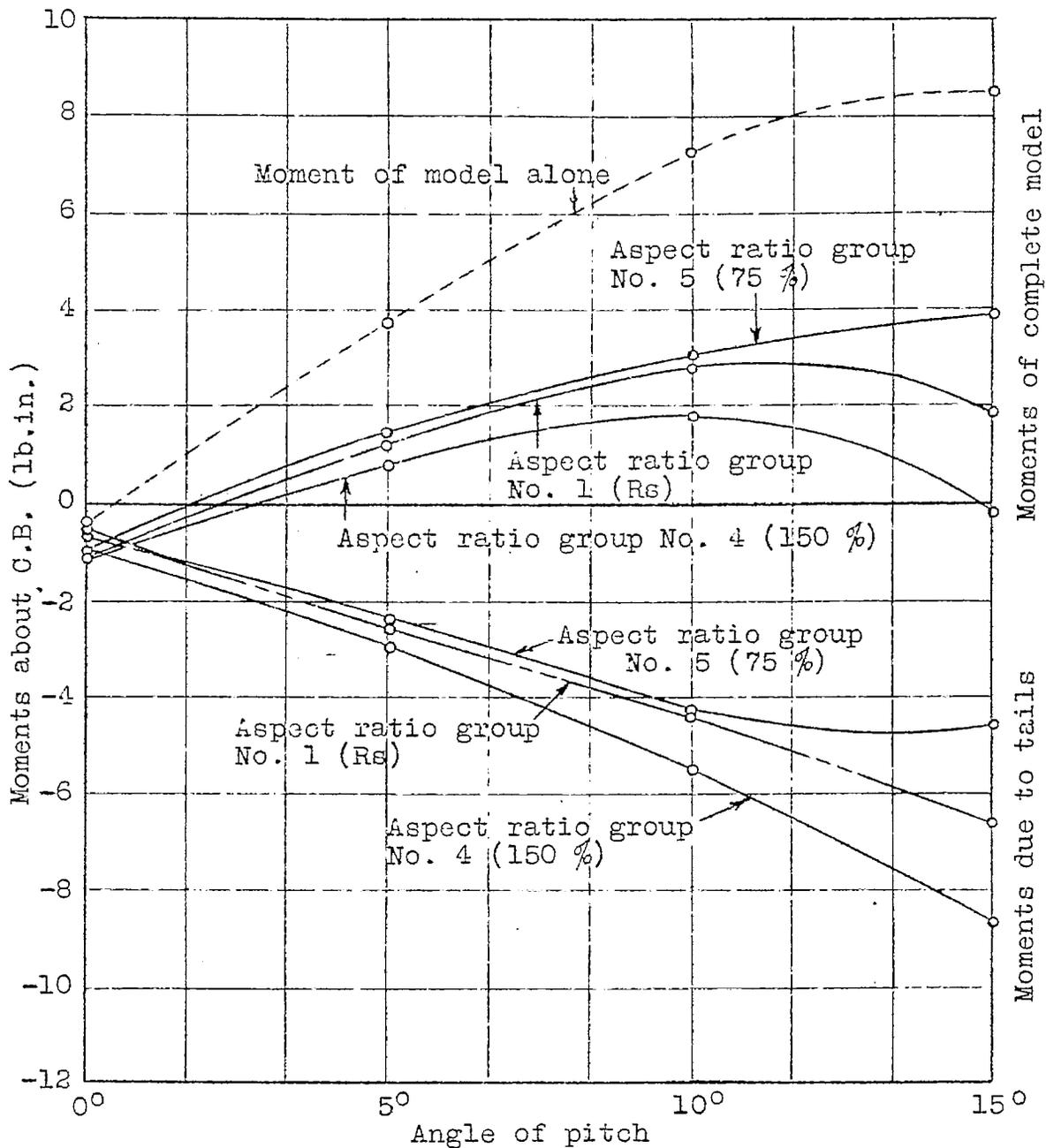
Fig. 8a Moment curves for elevator angle 10°
