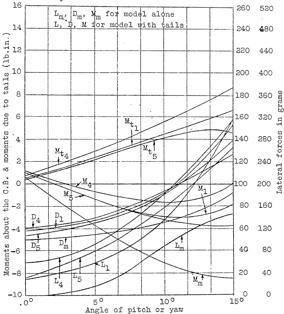
Fig. 17 Performance curves of an L-33 model fitted with aspect ratio tail surfaces. Elevators  $10^\circ$
