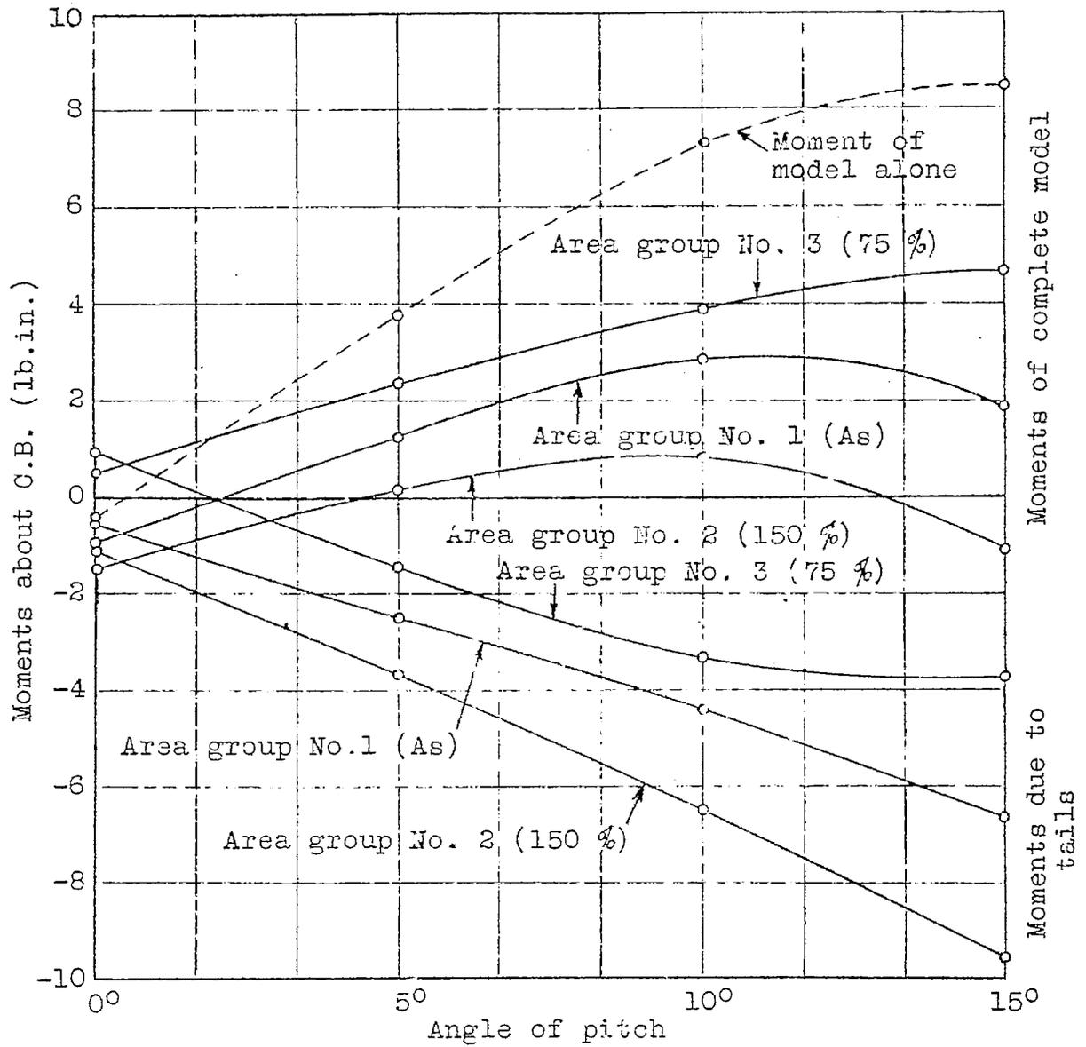
Fig. 8 Moment curves for elevator angle 10°
