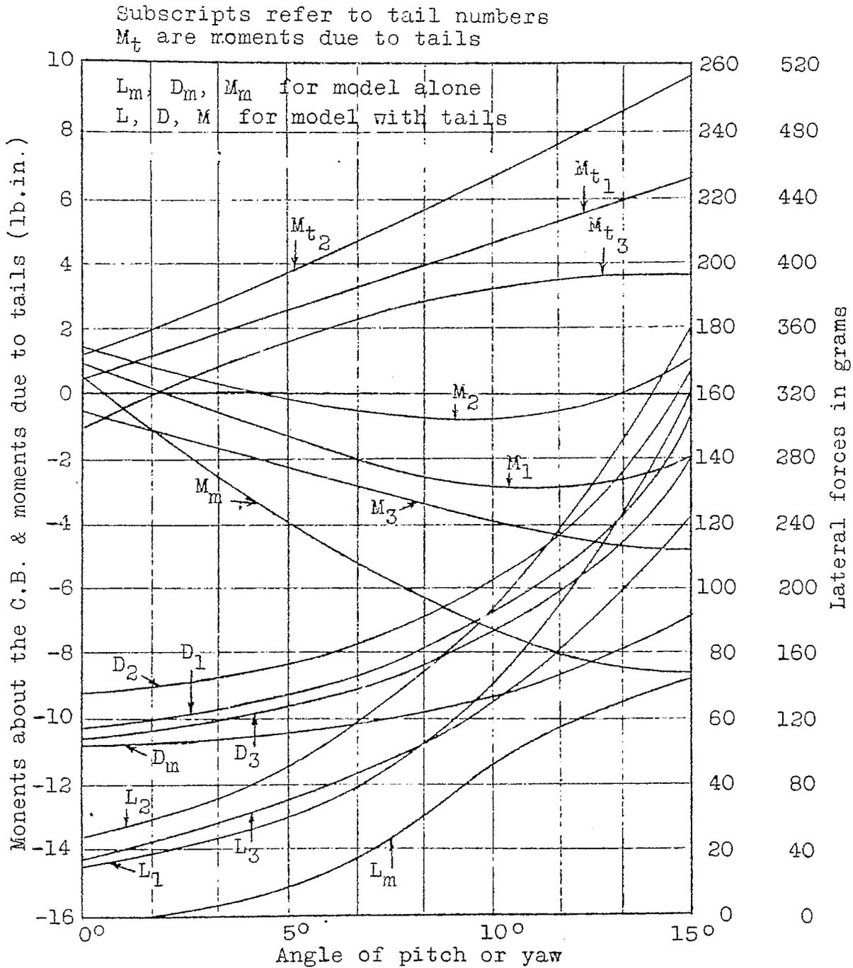
Fig. 16 Performance curves of an L-33 model fitted with area group of tail surfaces. Elevators 10°
