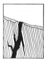
Fig. 82. — Fissure vein crossing the strata and throwing off stringers.
