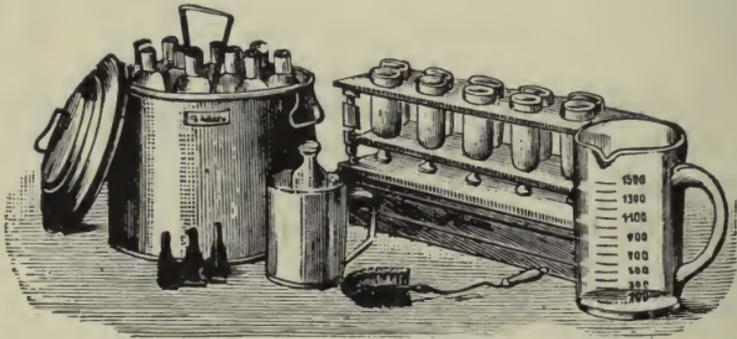
FIG. 198.—Soxhlet's milk steriliser.
