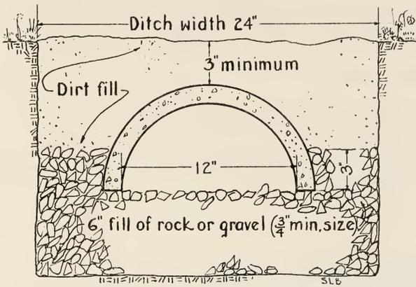
Fig. 16.—Cross section of half-section pipe drain line.
