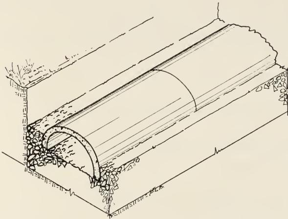
Fig. 17.—View of half-section concrete pipe in trench.
