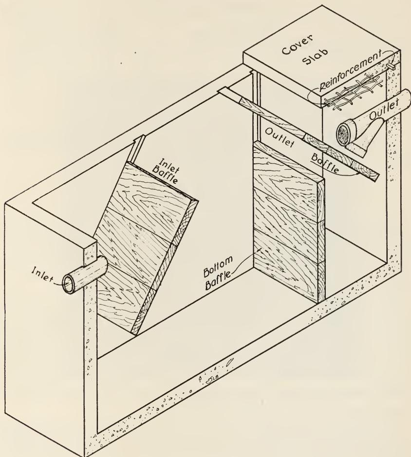
Fig. 3.—Half-section view of septic tank.
