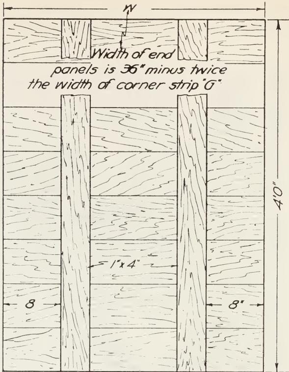
Fig. 10.—End panel. Four 6d nails, one at each corner, hold the end panels to the 2×3 inch studding B, figure 5.
