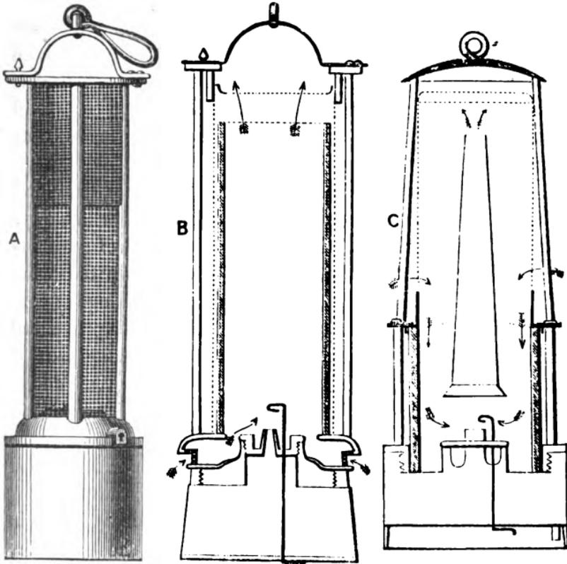
Fig. 50.—Safety-lamps. Scale—One-third true size.
