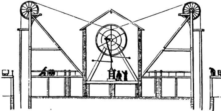
Fig. 40.—Drawing-engine, placed between two Pits.
