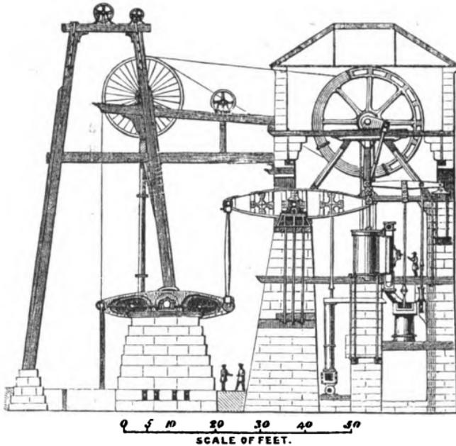
Fig. 49.—Engine and Apparatus for Winding and Pumping, Cambois, Northumberland.
