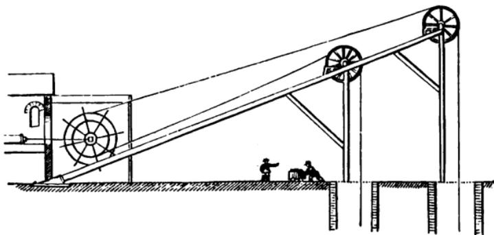
Fig. 41. — Engine on one side of a pair of Pits.
