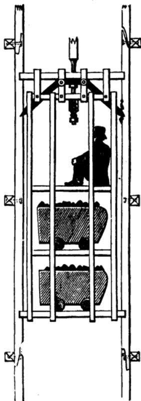
Fig. 44.—Fontaine's parachute as it appeared at the colliery of Boussu, when the flat wire rope broke with a weight of 2 tons.
