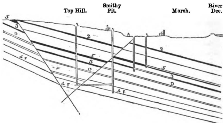
Fig. 21.—Section of Coal seams at Bagillt—160 yards to the inch.
