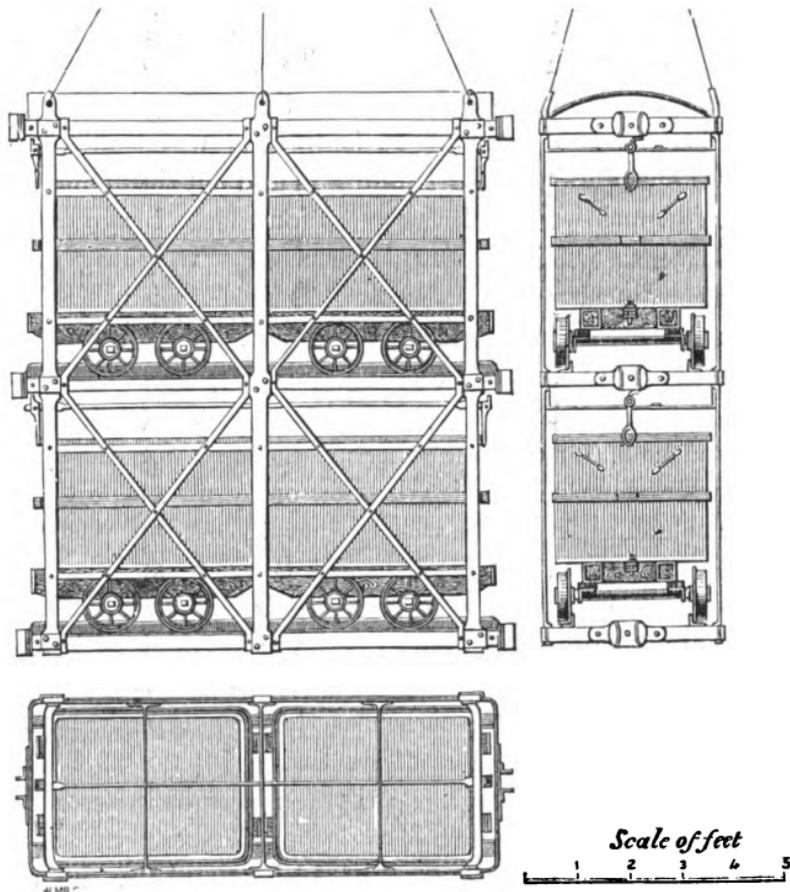
Fig. 38.—Steel Cage, North Seaton, with four tubs, in elevation and plan.
