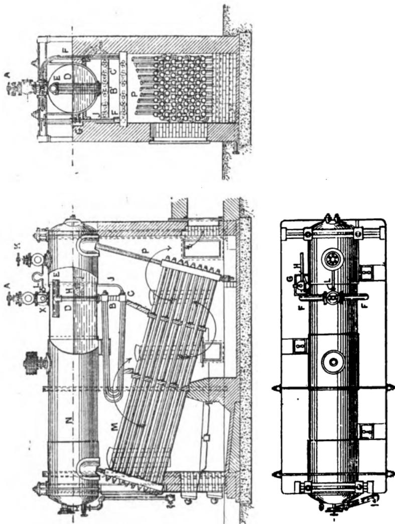
Fig. 34.—Pabcock and Wilcox Water-tube Boiler.
