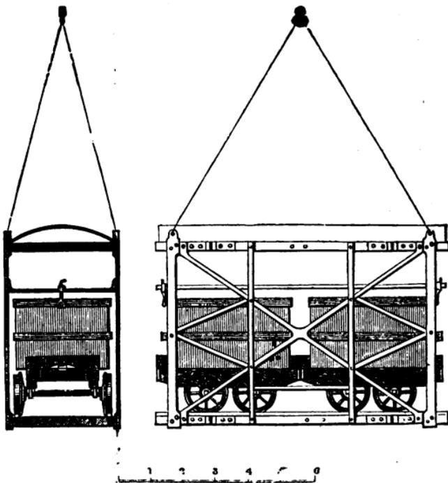
Fig. 37.—Single-deck Iron Cage, Newsham, for rolled iron guides.
