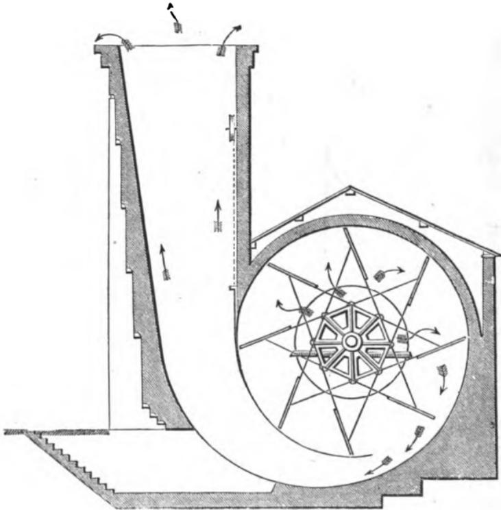
Fig. 56.—Guibal's Ventilating Fan. Scale—1 inch to 20 feet.
