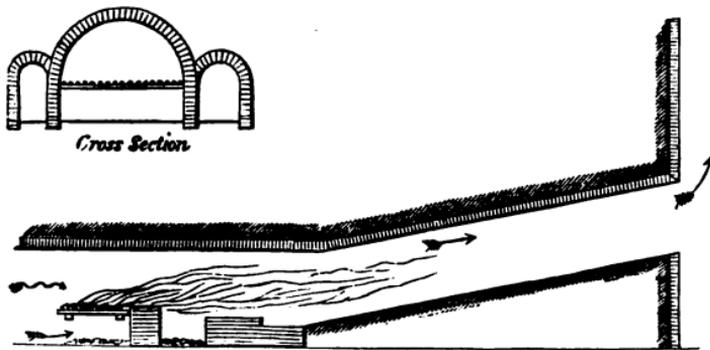
Fig. 53.—Ventilating Furnace, in longitudinal and cross-section.
