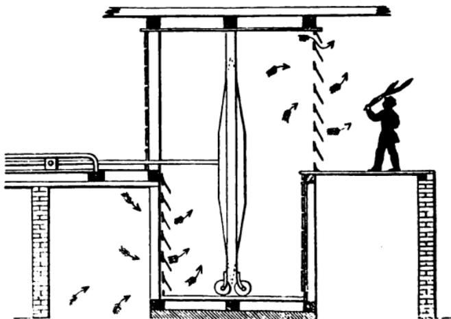
Fig. 55.—Nixon's Ventilator, Aberdare. Scale— $\frac{1}{4}$ -inch to 10 feet.
