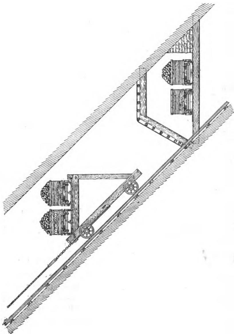
Fig. 32.—Platform for Colliery Tubs in inclined seams.
