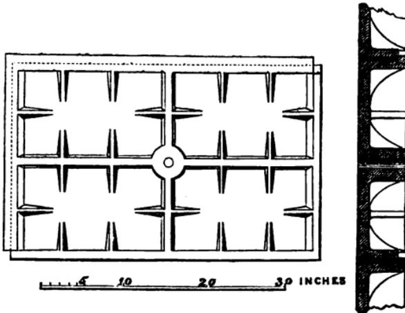
Fig. 20.—Cast-iron Tubbing Plate, in elevation and cross-section.
