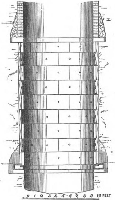
Fig. 19.—Cast-iron Tubbing, resting on two wedging curbs, the upper one hollow cast-iron, the lower one of wood.
