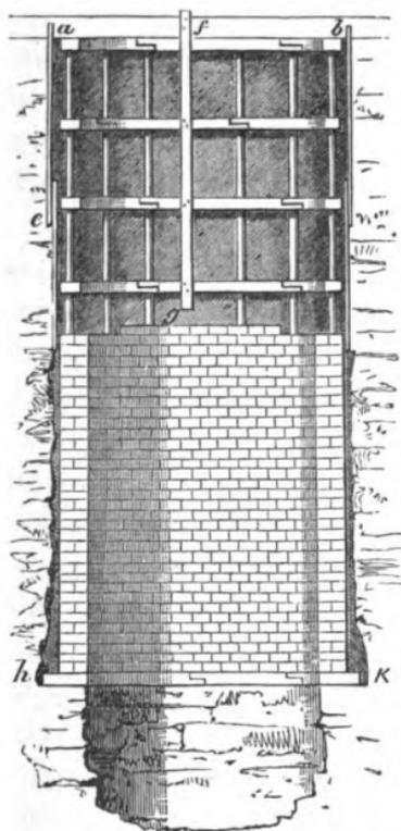
Fig. 17.—Lining of Shafts.
