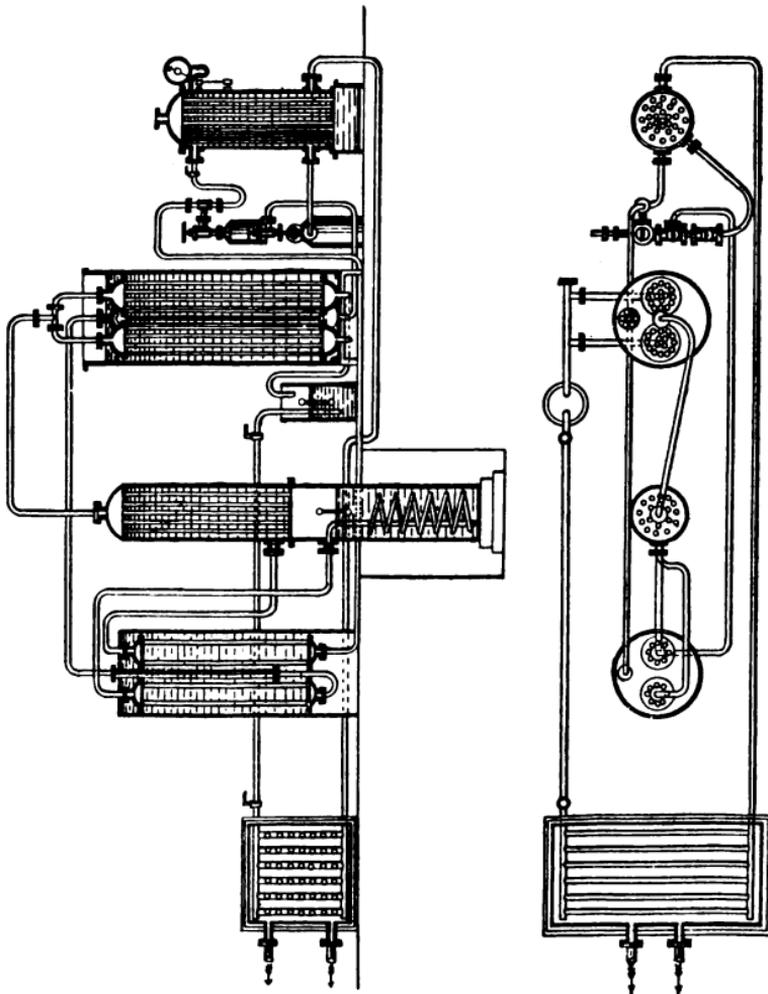
Fig. 18a.—Refrigerating Appliance used in Shaft-sinking.
