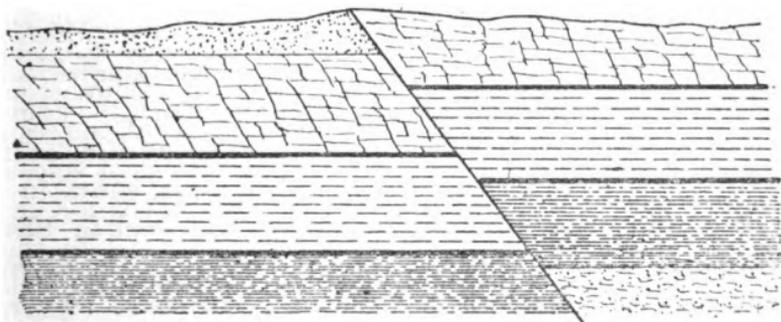
Fig. 4.—Reverse Fault.
