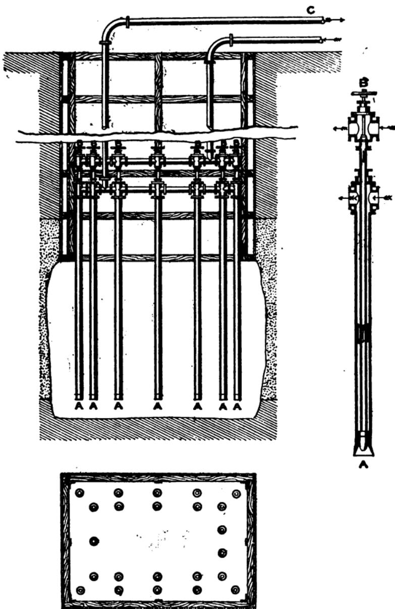
Fig. 18.—Refrigerating Method in Shaft-sinking.
