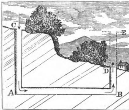
Fig. 52.—Diagrams illustrating Natural Ventilation.
