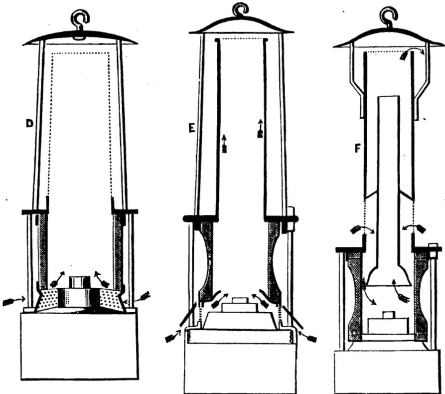
Fig. 51.—Safety-lamps. Scale—One-third true size.
