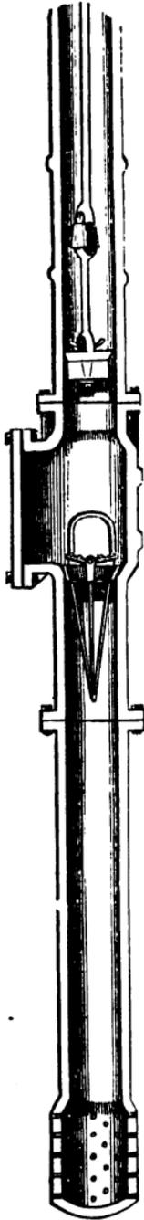
Fig. 47.—Bucket, or Drawing Lift.
