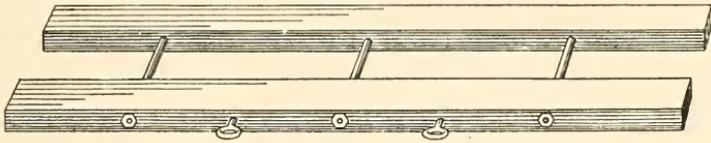
FIG. 1.—Implement used for leveling the land.
