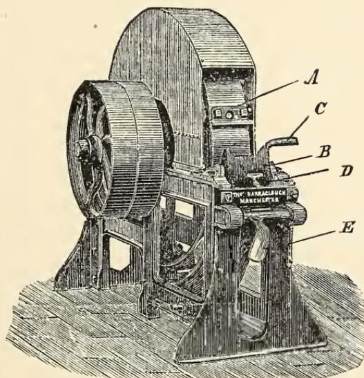
FIG. 18.—The Barraclough cleaning machine.
