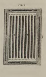
door; k is a pipe for drawing off the water melted from the ice.
