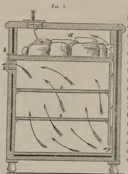
Preserver, showing the manner of admitting the air into the ice chamber. over and around the surface of ice, thence through an opening, and descending thro' a flue into the lower part of the Preserver up through the shelves, and out at the sides as denoted by the spears.
