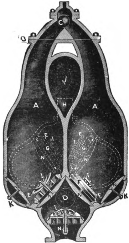
FIG. 120.—SECTION OF PULSOMETER.
