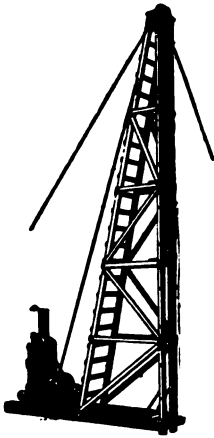
FIG. 36.—LIDGERWOOD PILE-DRIVING DERRICK.
