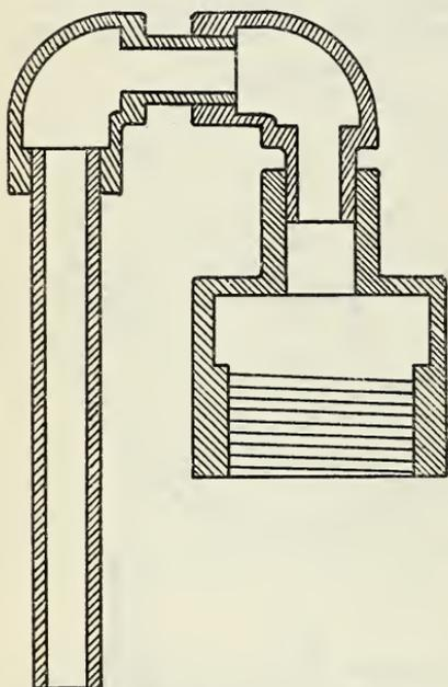
FIG. 2.—Cross section of the vent cap. It consists of a  $\frac{3}{4}$ -inch to  $\frac{1}{2}$ -inch reducer, into which fit successively two  $\frac{1}{2}$ -inch elbows and a  $\frac{1}{2}$ -inch pipe 3 inches long and open at the end. The elbows and upper two-thirds of the  $\frac{1}{2}$ -inch pipe are closely packed with asbestos wool.
