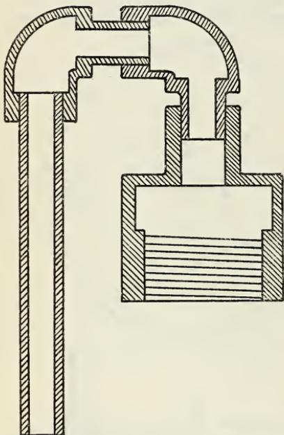
FIG. 2.—Cross section of the vent cap. It consists of a  $\frac{3}{4}$ -inch to  $\frac{1}{2}$ -inch reducer, into which fit successively two  $\frac{1}{8}$ -inch elbows and a  $\frac{1}{8}$ -inch pipe 3 inches long and open at the end. The elbows and upper two-thirds of the  $\frac{1}{8}$ -inch pipe are closely packed with asbestos wool.
