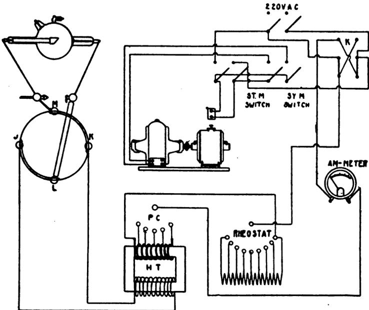
FIG. 20.—Diagram of connections of an "interrupterless" apparatus operating on an alternating current.
