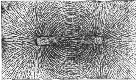
FIG. 4.—Action of bar magnet on iron filings.
