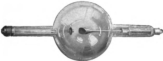
FIG. 11.—The Coolidge tube.
