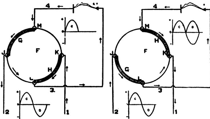
Figs. 18 and 19.—Illustrating rectification of current by revolving discs.
