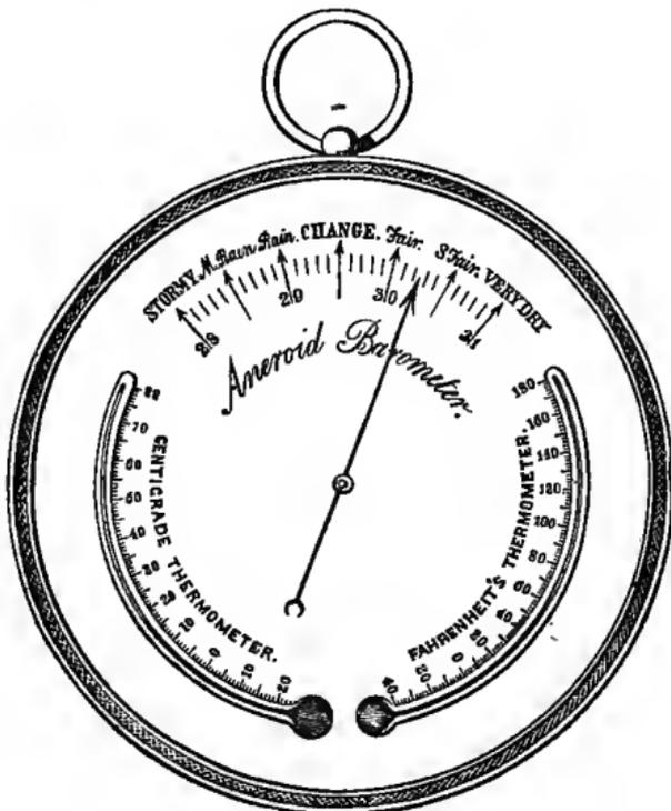
Fig. 1 represents the external appearance of the instrument. It is four inches and three-quarters in diameter across the face, and one inch and three-quarters in thickness. The pressure of the atmosphere is indicated by a hand pointing to a scale, which is graduated to correspond with the common barometer: thermometers are placed on the face, one of which is essential.
