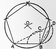
describe arcs cutting at O, which is the centre of the circle. Step off A B around the circumference and draw straight lines connecting the points.
