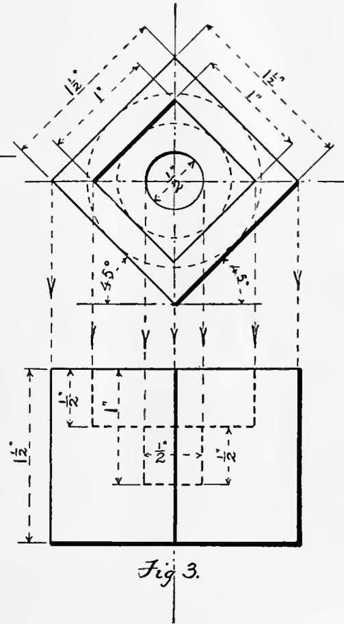
FIG. 3.—A cube resting upon one of its edges with sides at angles of  $45^\circ$  to horizontal. In one face of the cube is a depression 1" square,  $\frac{1}{2}$ " deep, while in the centre of this depression is a further depression, round  $\frac{1}{2}$ " diameter,  $\frac{1}{2}$ " deep, the cube being  $1\frac{1}{2}$ " square on each face.
