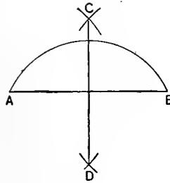
**2** To draw a perpendicular to a straight line from a given point in that line. Let  $C$  be the given point in the line  $A B$ . With  $C$  as a centre, draw the arcs at  $A$  and  $B$ , making  $A C$  and  $C B$  equal; then with  $A$  and  $B$  for centres, and radius greater than  $A C$ , draw the intersecting arcs at  $D$ . Join  $C$  and  $D$ .
