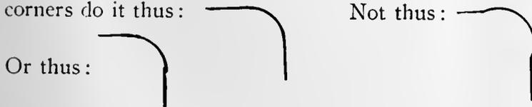
In drawing or finishing a drawing with ink it is best to fill in the circles and arcs first, afterwards drawing the straight lines, the reason being that it is easier to fit a tangent or straight line to an arc or curve than is the reverse process.
