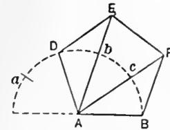
Draw line from A through the divisions D, b and c, omitting one point a. With D and B for centres and radius A B cut A b at E and A c at F. Draw D E, E F and B F.
