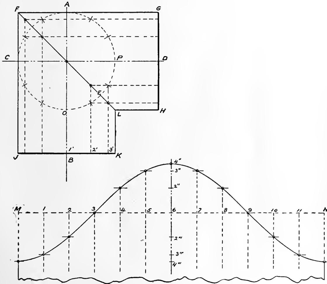
PLATE 31. *To Lay Out an Elbow of Several Sections and to Develop a Section.*
