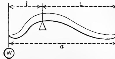
Bent levers are treated the same as straight levers, as in the figure annexed.
