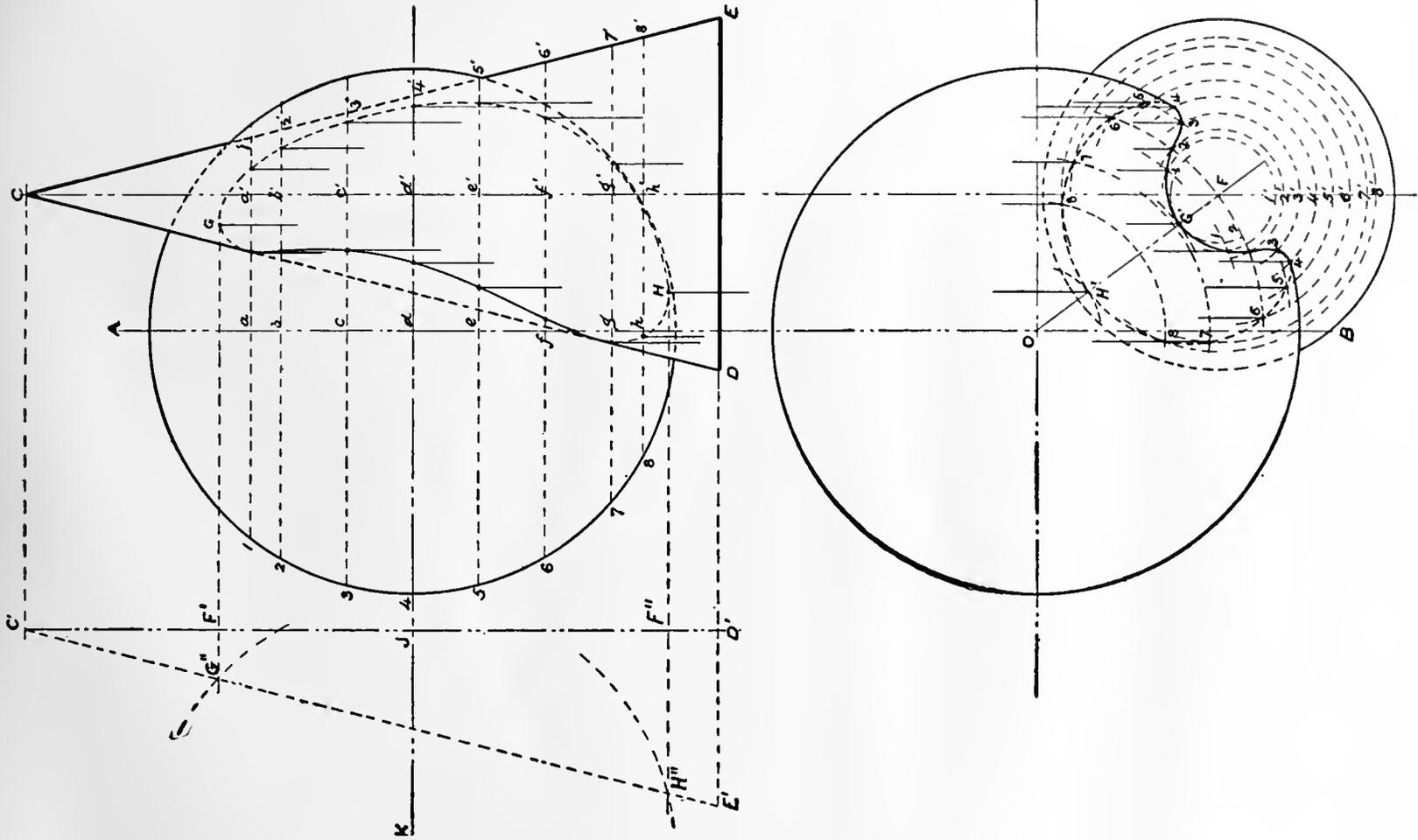
PLATE 30. *Intersection of Two Cylinders of Equal Diameter at Angle of  $90^\circ$ , and Development of Envelope.*
