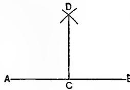
**3** From the end of a straight line to draw a perpendicular to that line. From some point without the line as  $C$ , draw the arc  $D A E$ , passing through  $A$  at the extremity of the line and cutting the line at  $E$ . From  $E$  draw  $E D$  through  $C$ , draw  $D A$ , which will be the required perpendicular.
