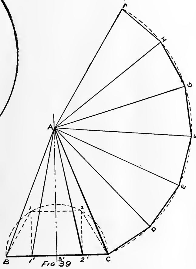
PLATE 34. *To Draw a Hemispherical Dome and to Develop in the Flat Sheet the Sections.*
