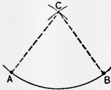
**10** To find the centre of a circle or of an arc of a circle. Take any three points in the circumference well separated as A, B and C. With these points as centres draw the intersecting arcs, and through these intersections draw straight lines intersecting at D. D will be the required centre.
