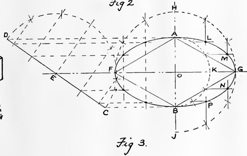
ting A produced in D, draw C D and bisect in E and erect perpendicular. With E for centre and E C for radius draw semi-circle and subdivide, and project the
