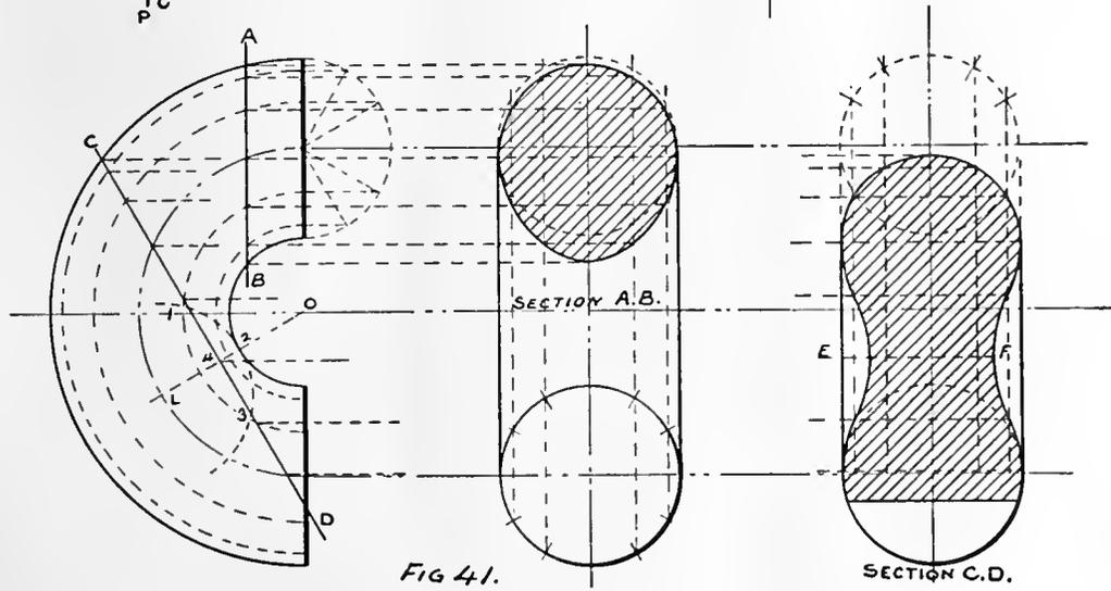
PLATE 37.—A sphere cut by a plane at an angle to its vertical axis. In the side elevation a straight line drawn to the required angle will represent the plane.
