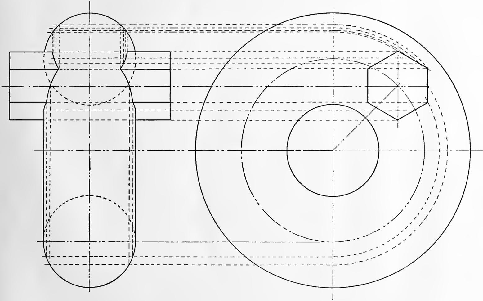
PLATE 27. *Intersection of Cone and Cylinder.*
