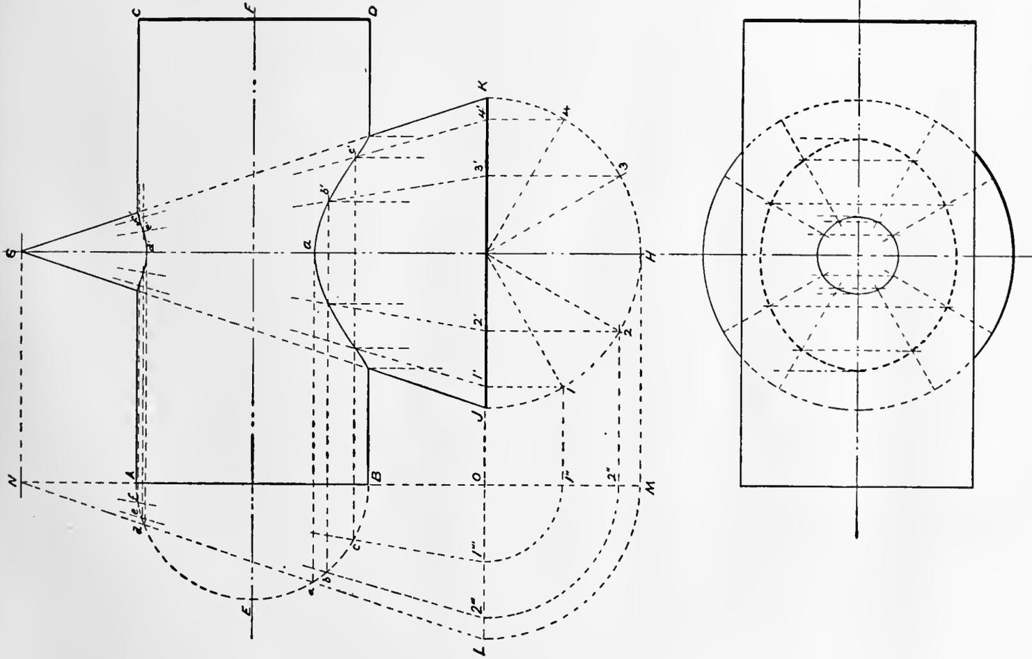
PLATE 28. *Intersection of Two Cones.*
