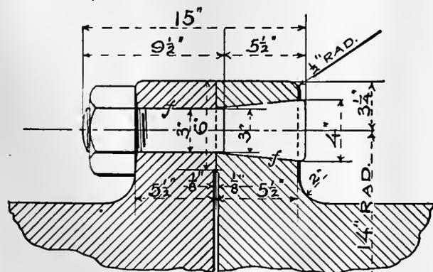
SECTION SHOWING COUPLING BOLT.
