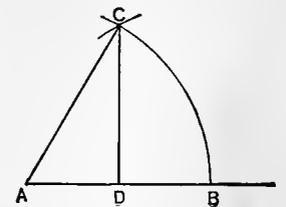
**7** To lay off an angle of  $45^\circ$ . Draw A C perpendicular to A B, with A for centre and radius A B draw arcs B and C, draw B C. Then will angles A C B and C B A be angles of  $45^\circ$ .
