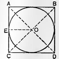
**20** To describe a square about a circle. Draw diameters  $A B$  and  $C D$  perpendicular to each other, with  $A, B, C$  and  $D$  as centres and  $A O$  for radius, draw arcs cutting each other at  $E, F, G$  and  $H$ . Draw  $E F, F G, G H$  and  $H E$ .
