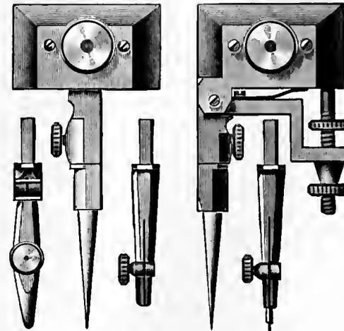
clamped to a wood bar or beam. It is fitted with pen, pencil and needle points.
