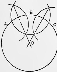
**11** To draw a circle through three given points use the same construction as used for No. 10, the centre D being found by the same method.
