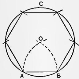
**24** To inscribe a hexagon in a circle. Draw diameter A B and with radius equal to the radius of the circle step off points around the circumference; connect these points with straight lines to complete the hexagon.
