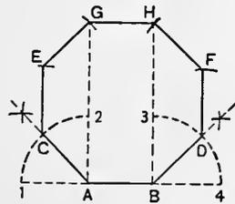
radius A B draw arcs E and F, and draw C E and D F parallel to A G and B H. With E and F as centres and radius A B draw arcs cutting A G and B H. Draw E G, F H and G H.
