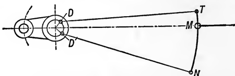
Fig. 94.—Link Motion “Notched up.”
