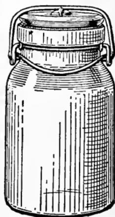
FIG. 128.—Position of clamp after sterilization.
