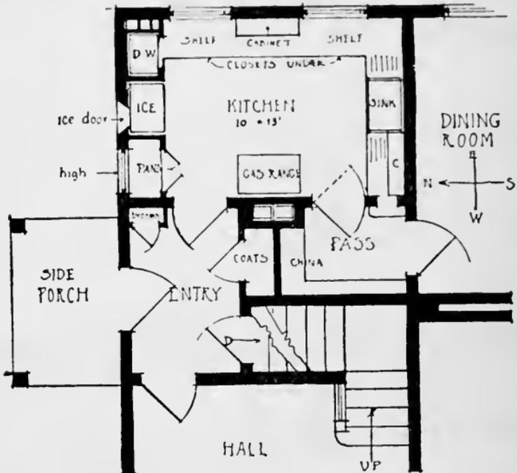
FIG. 36.—A kitchen for a suburban house, developed in accordance with the principles of good arrangement.
