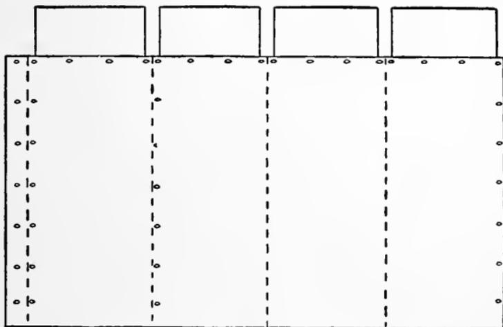
FIG. 51.—Removable canton flannel cover for the refrigerator. The buttonholes are placed to correspond with the buttons on the framework.
