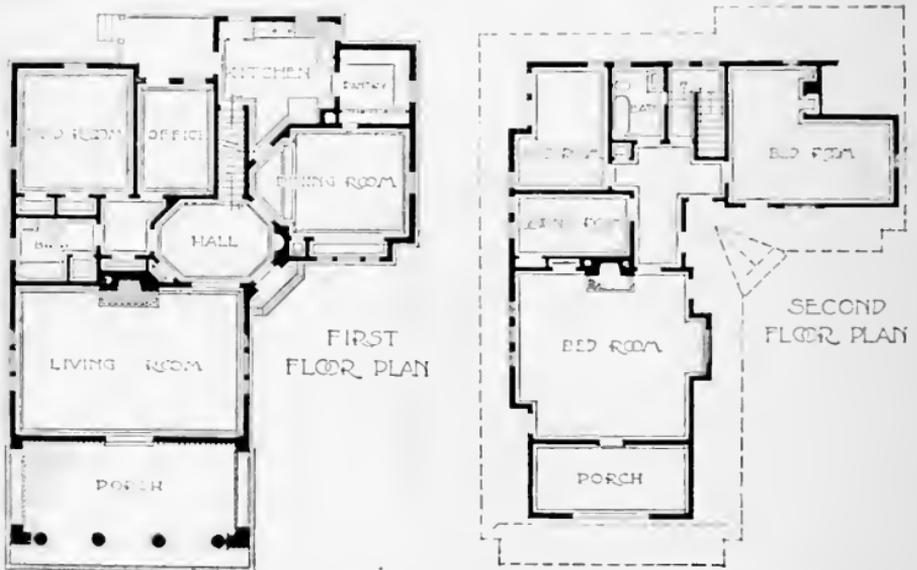
FIG. 8.—A farmhouse plan, showing diagonal corners used deliberately for purpose of design.
