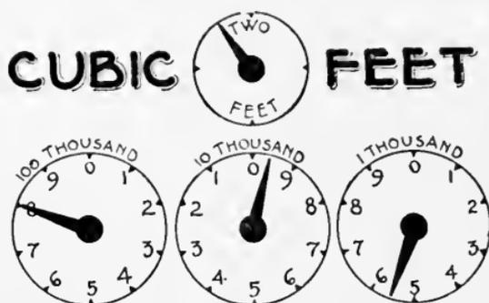
FIG. 42.—Gas meter index reading 79,500 cubic feet.
