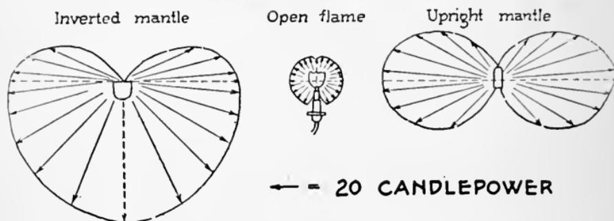
FIG. 46.\*—Comparison of amount of light given by different gas lamps. Each lamp is supposed to burn 5 cubic feet an hour, costing  $\frac{1}{2}$  cent if gas is \$1.00 a 1000 cubic feet. Note that the mantle lamp gives four or five times as much light as the open flame. The inverted mantle gives more light downward and less upward than the upright mantle.
