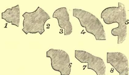
6. Wave-molding, or swelled chamfer.
