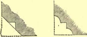
1. The plain or hollow chamfer of two or more orders, which, properly speaking, is only the step preparatory to molding, and stopping short of that ulterior process.
