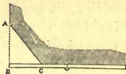
which may generally be done very easily by placing the rule against one plane and sighting the end of it to a line with the other, as in diagram, where the rule is placed against one plane, the end just meeting the other,
