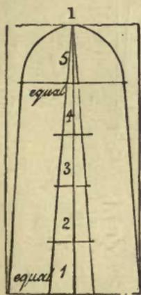
Plate 1 will shew you what sub-division to proceed with previous to forming the exterior line of the leaf; and better to prove it, we will suppose that I have a given size to execute an Acanthus foliage, height 2 feet, base
