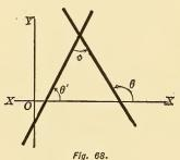
$\phi = \theta - \theta'.$   $\therefore \tan \phi = \frac{m - m'}{1 + mm'}.$ If the lines be  $\parallel, \phi = 0,$   $\therefore m - m' = 0, m = m'.$ If the lines be  $\perp$ ,  $\tan \phi = \infty,$  $\therefore 1 + mm' = 0.$
