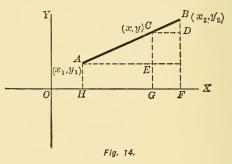
A and B are the given points, C, (x, y) is the required point. Draw the ordinates as in the figure.
