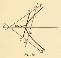
To prove AA' = BB'. Let A be  $(x_1, y_1)$ , B  $(x_2, y_2)$ . Then the chord AB meets the [axes] asymptotes in B'  $(x_1 + x_2, o)$ and A'  $(o, y_1 + y_2)$ .
