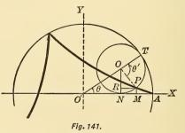
To find its equation: Take O', the center of the fixed circle, as origin, and the  $\perp$  diameters OAX, OY, as axes. Let A be the initial point of the curve.
