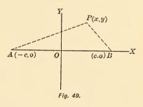
$\sqrt{(x+c)^2 + y^2} + \sqrt{(x-c)^2 + y^2} = 2 a \quad . \quad . \quad (1)$  $\sqrt{(x+c)^2 + y^2} = 2 a - \sqrt{(x-c)^2 + y^2}.$
