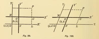
OX, OY are the old axes; O'X', O'Y' are the new axes. P is any point in the plane whose co-ordinates are (x, y) to the old axes (x', y') to the new axes.
