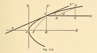
SN is the given diameter, ST a tangent at its extremity S. We shall first find the equation referred to SN and SY' perpendicular to it.
