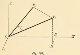
Then, the projection of  $OP_1$  on  $OP_2 = projection of the broken line <math>ONMP_1$  on  $OP_2$ .
