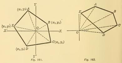
CASE II. Origin without the polygon. Area ABCDE =  $\triangle$ s OAB + OBC + OCD + OAE - ODE. But  $\triangle$  ODE =  $-\frac{1}{2} [x_5y_4 - x_4y_5]$ . Hence, in all cases, the signs of the  $\triangle$ s are positive.  $\therefore$  Area ABCDE =  $\frac{1}{2} \{ [x_2y_1 - x_1y_2] + [x_3y_2 - x_2y_3] + [x_4y_3 - x_3y_4] + \text{etc.} \}$ =  $\frac{1}{2} \{ x_2y_1 - x_1y_2 + x_3y_2 - x_2y_3 + x_4y_3 - x_3y_4 + \text{etc.} \}$ . The order of the subscripts is cyclic.
