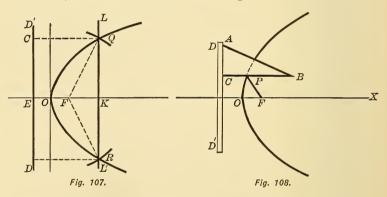
any point K of EF (produced if necessary) erect the  $\perp$  LL'. Now with F as center and EK as radius, cut this  $\perp$  in Q and R. These are two points on the curve. For FQ = EK = CQ. In this manner any number of points may be found and joined by a continuous curve.
