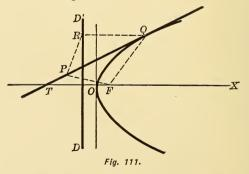
(2) To draw a tangent to a parabola from an external point P. With P as center, and PF as radius, cut the directrix in R. Draw RQ parallel
