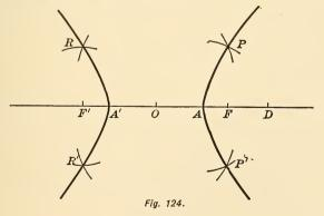
radius, describe two arcs. Then with F as center, AD as radius, describe two arcs cutting the former in P and P'. These are evidently points on the curve. By interchanging radii, R and R' are found. After a sufficient number of points have thus been found, they are joined by a smooth curve.
