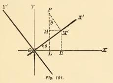
P is any point (x, y) old axes, and (x', y') new axes. PM' is  $\perp$  to OX' and M'M is  $\perp$  to PL. Now x = OL = OL' - LL' = OL' - MM'  $= OM' \cos \theta - PM' \sin \theta.$  $\therefore x = x' \cos \theta - y' \sin \theta.$
