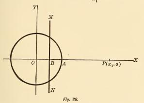
construct it, find B so that  $OP \times OB = \overline{OA}^2$ , *i.e.*, a third proportional to OP and OA (r). Then  $MN \perp$  to OP at B is the polar required.
