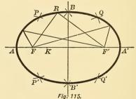
Bisect FF' in O, and take OA = OA' = a. Then A and A' are points on the curve. [Why?] Now between F and F' take any point K. With F as center and AK as radius, describe arcs; with F' as center and A'K as radius, describe arcs intersecting the former in P and P'. By interchanging radii, Q and Q' are found. These all lie on the curve because the sum of the focal distances of each is 2a. After finding enough points we join them by a smooth curve.
