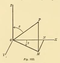
and cutting the latter in the line OM. The position of P is then known if the line OP, the radius vector, and the angles  $\phi$  and  $\theta$ , the vectorial angles, are given. These three magnitudes together constitute the polar co-ordinates of the point P.
