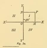
Thus, in Fig. 2*a*, the point P is determined if its distances PM, PN, from the axes are known. In Fig. 2*b*, it is determined if the lines PN, PM, drawn parallel to the axes, and the angle  $\phi$  between the axes, are given; X'X is called the axis of **abscissas**, or the **x**-axis; Y'Y, the axis of **ordinates**, or **y**-axis. The line PN, measured parallel to the
