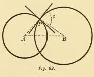
Tangents at P, the point of intersection of the two circles, are  $\perp$  to the radii AP and BP. Hence the angle between the tangents is equal to angle APB.
