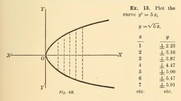
For negative values of x the value of y is imaginary; hence no point of the curve lies to the left of the y-axis. When  $x = \infty$ ,  $y = \infty$ , hence the curve extends to the right without limit. It passes through the origin. The curve is called a **parabola**.
