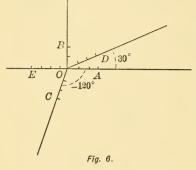
is designated in polar co-ordinates by  $(\rho, \theta)$ . The vectorial angle  $\theta$  is positive or negative according as we suppose the line OP to revolve in the counter-clockwise or clockwise direction. The radius vector  $\rho$  is positive if measured from O along the revolving line OP, and negative if measured in the opposite
