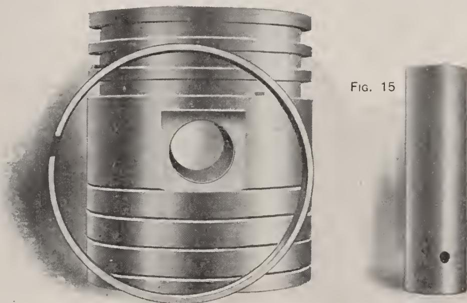
Fig. 15—A Piston, Piston Ring, and Piston Pin
