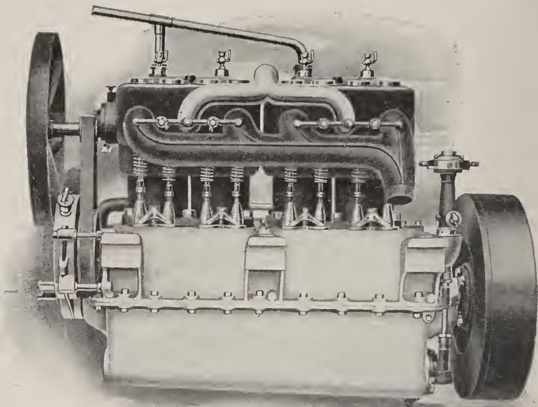
Fig. 35 - Valve side of a Four-cylinder Motor.
