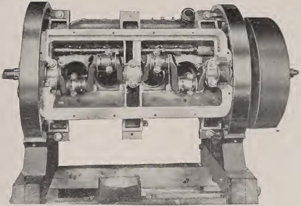
Fig. 37—Bottom view of same Motor with oil pan removed showing Crank Shaft, and Connecting Rods.
