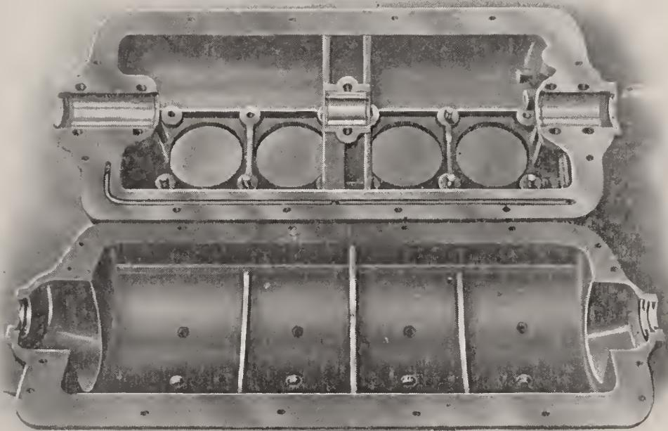
Fig. 20—The two halves of a Four-cylinder Crank Case.
