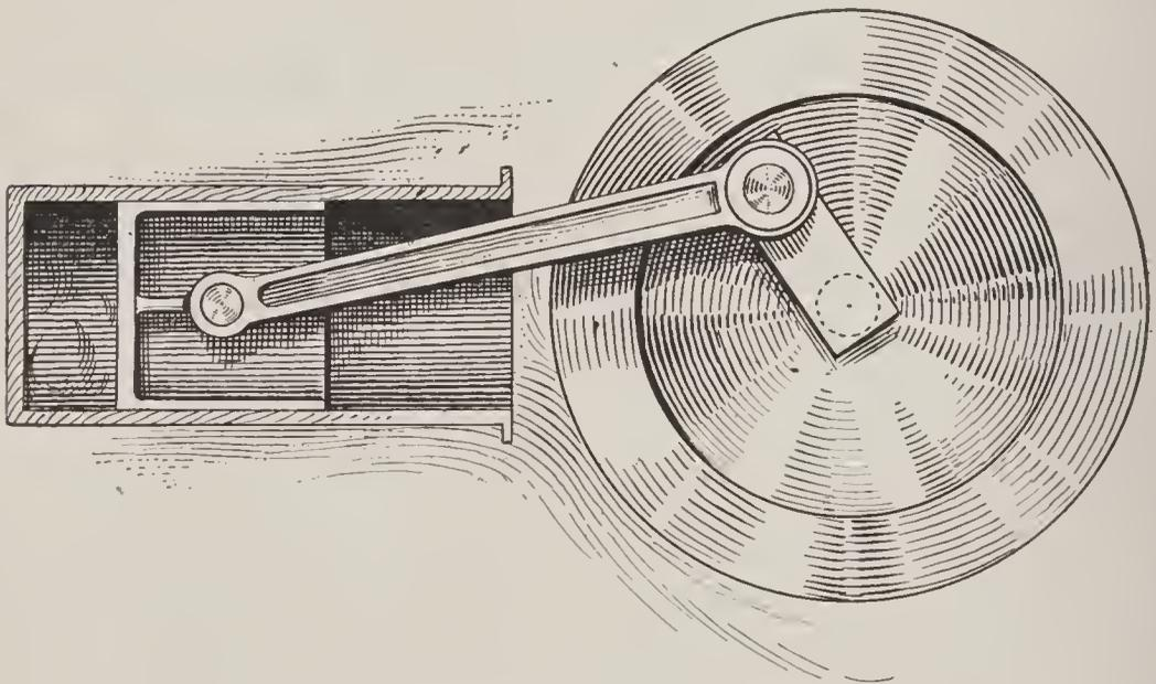
Fig. 1—The Essential Parts of a Gas Engine.
