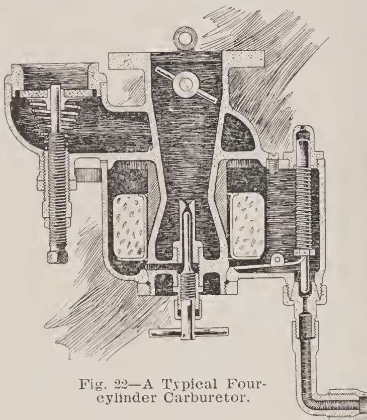
Fig. 22—A Typical Four-cylinder Carburetor.
