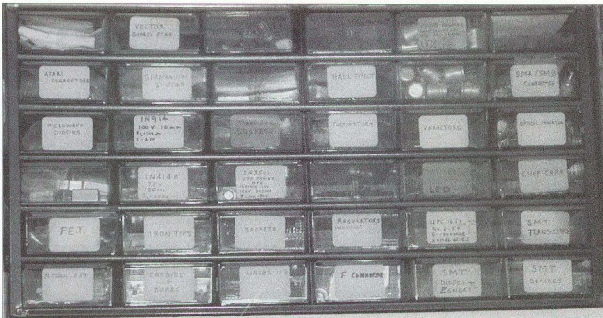
**Photo D.** Example of a cabinet containing plastic drawers. Drawers are labeled to indicate the part within along with cursory technical data.
