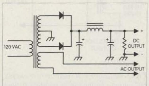
Fig. 1. Typical AC-powered supply.
