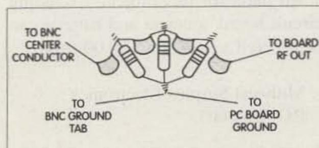
Fig. 2. Layout of the bandpass filter.
