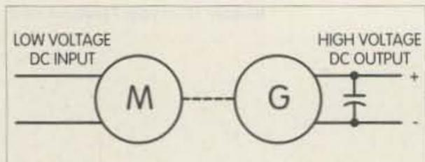
Fig. 2. Typical dynamotor or rotary transformer.
