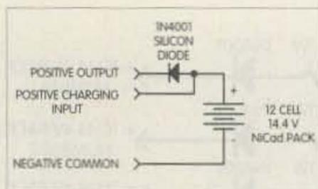
**Fig. 2.** Typical 12-cell, 14.4 volt battery pack showing one positive wire for charging the pack and another positive wire for discharging the pack into the operating load through a diode.
