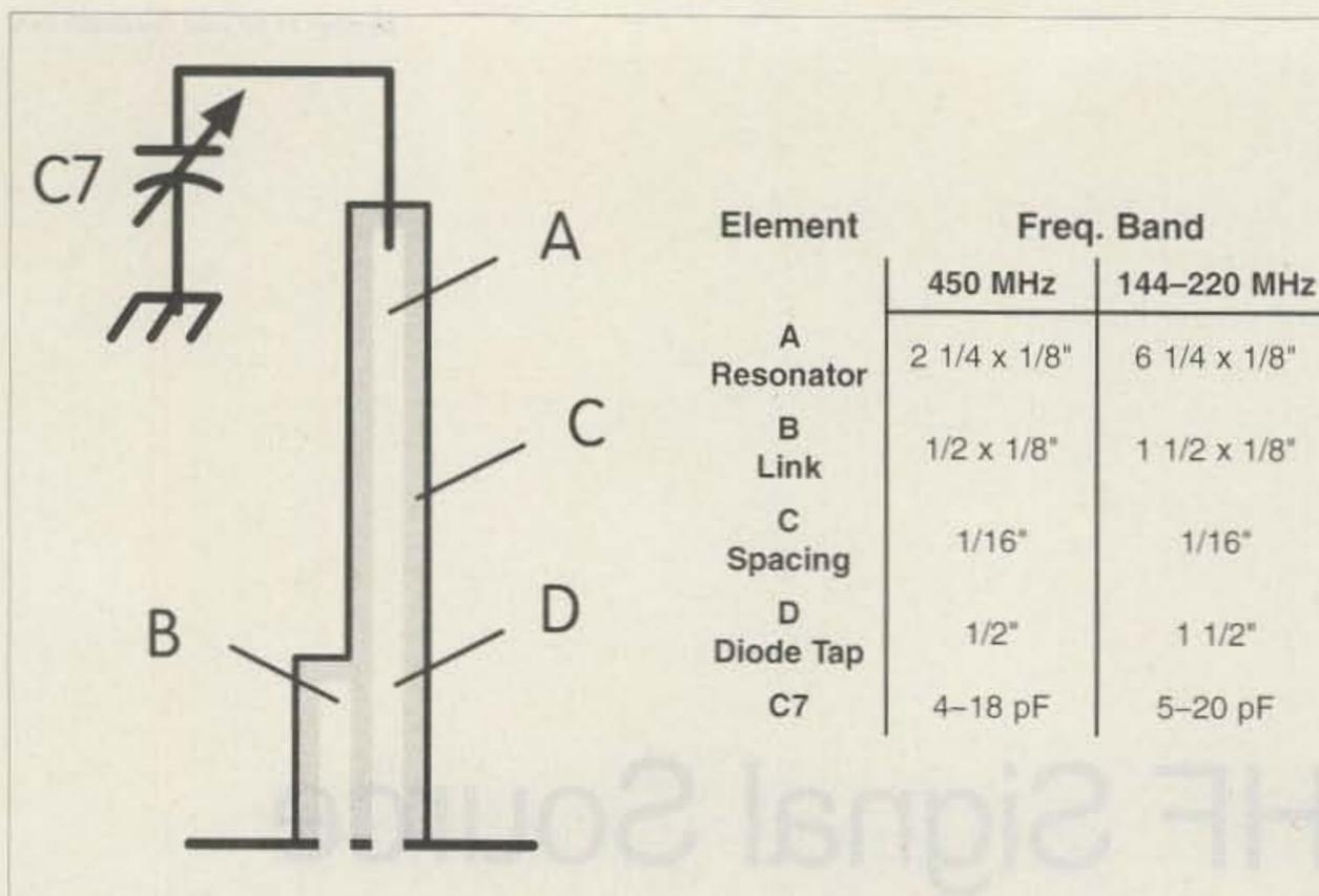
Fig. 2. Stripline dimensions and lengths for different frequency bands.
