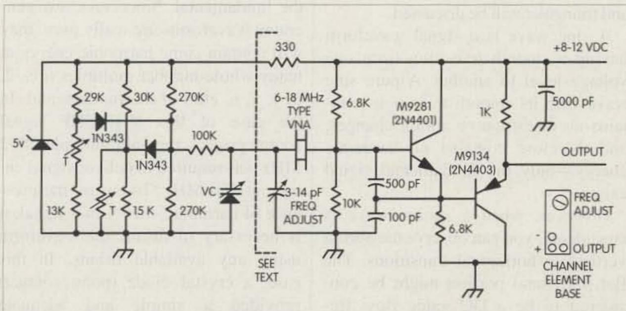
Fig. 1. Motorola TLN 1086/87 channel element.
