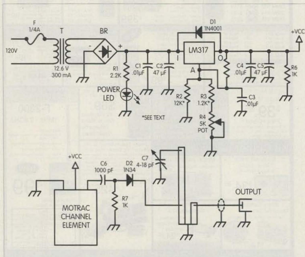
Fig. 4. UHF signal source.
