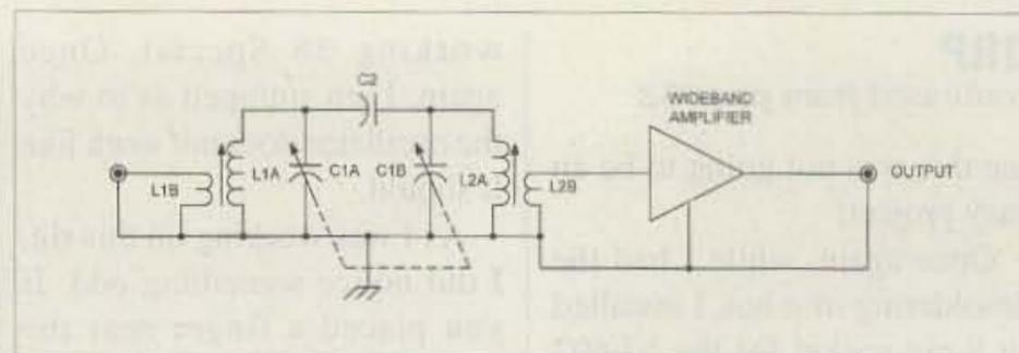
Fig. 2. Preselector schematic.
