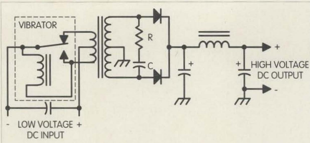
Fig. 4. Vibrator power supply used in early car radios. Typical rectifier was an 0Z4, 6X5, or 6X4 tube.
