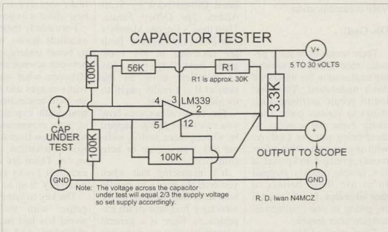
Fig. 1. Schematic for N4MCZ's capacitor checker. Note: The voltage across the capacitor under test will equal 2/3 the supply voltage, so set supply accordingly.
