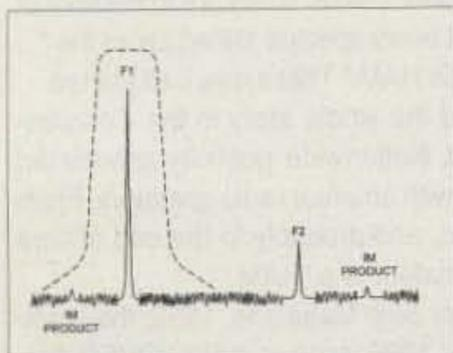
Fig. 4. A preselector can reduce the IM products.
