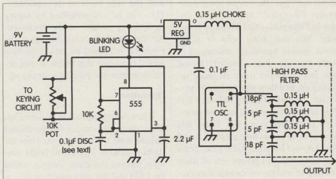
Fig. 1. Schematic of FoxTTL 2-meter transmitter.
