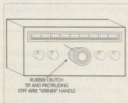
**Fig. 3.** A rubber crutch tip with a short, stiff piece of wire inserted and glued to one side can be used as an inexpensive vernier tuning adapter for many older radios. See text for more details.
