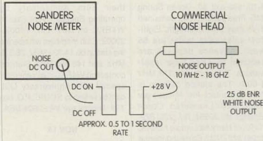
**Fig. 1.** Basic noise test instrument from Sanders, covering a frequency spectrum of 10 MHz to 18 GHz. Heart of unit is noise head driven by 28-volt power supply.
