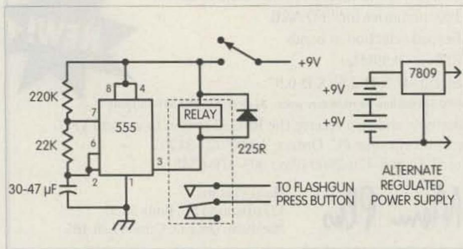
Fig 1. Pulse circuit.
