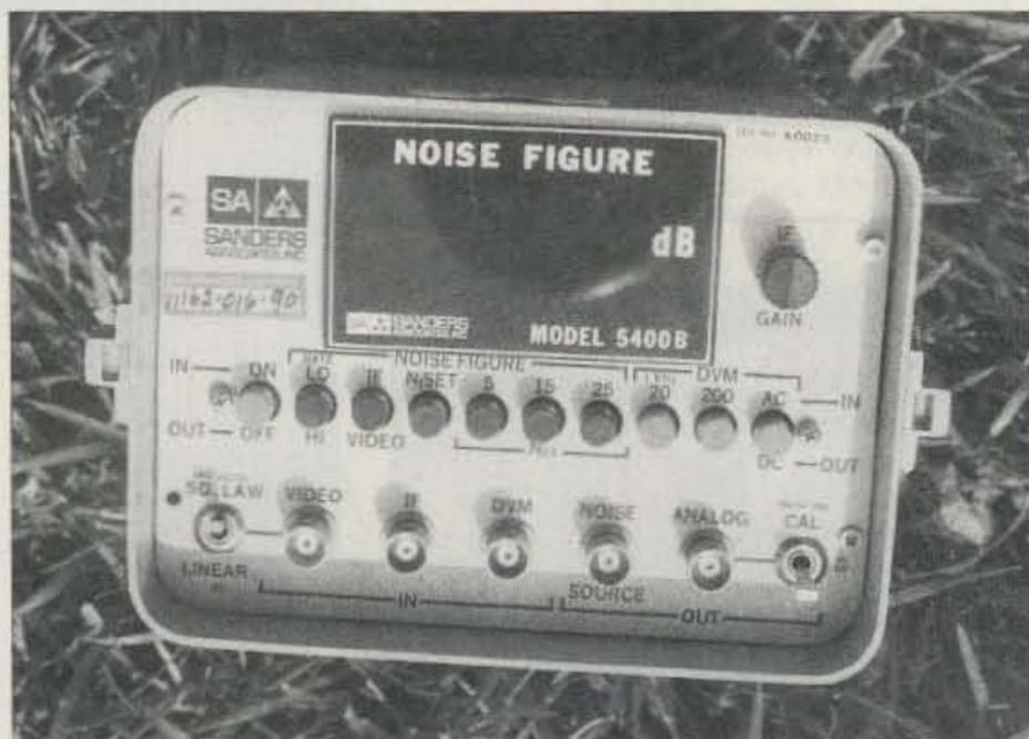
**Photo A.** Sanders noise figure meter, 10 MHz to 18 GHz operation frequency range. Capable of 25 dB excess noise output and can be used with external 10 or 20 dB attenuator to reduce noise for more sensitive systems. With a 20 dB attenuator attached to noise head, this will reduce the noise output to 5 dB ENR (excess noise ratio). Permits noise figure in the 1 to 10 dB range to be measured.
