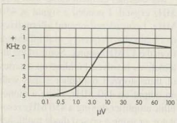
Fig. 3. Frequency shift relative to output voltage setting.
