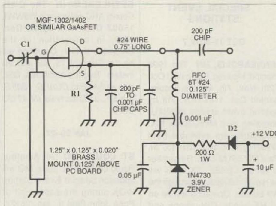
**Fig. 2.** GaAsFET preamplifier by WA5VJB from 1986 ARRL Handbook, used as test circuit. This circuit selected because of simplistic design, low noise figure, ease of construction, and modest cost. C1 = 0.3- to 3-pF piston trimmer capacitor. R1 = 100  $\Omega$ , 1/8 or 1/4 W, carbon. D2 = 1N914 or 1N4148, or any with ratings of 25 PIV and 50 mA or greater.
