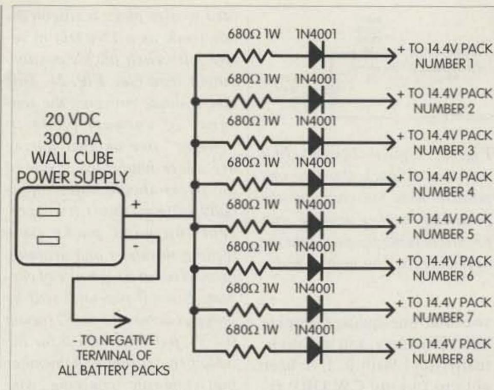
**Fig. 1.** The wall cube power supply and current limiting resistors should be chosen so that about 28 milliamperes is delivered to each of the 14.4 volt DC battery packs. The values shown represent just one such combination; the ones you select should be measured with a milliammeter to make sure that the proper one-tenth-capacity current is present.
