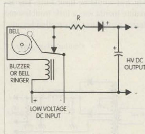
Fig. 3. Buzzer or bell ringer power supply, DC output obtained from rectified flyback voltage.
