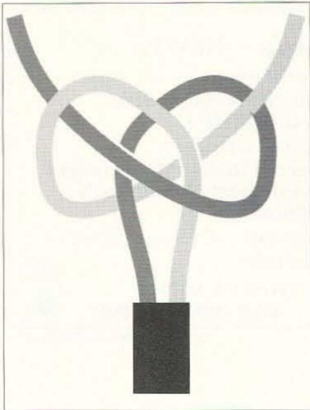
Fig. 3. The "Electrician's" or "Underwriter's" knot.
