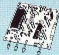
**COR-3.** Inexpensive, flexible COR module with timers, courtesy beep, audio mixer. .... only \$49/kit, \$79 w/t.
