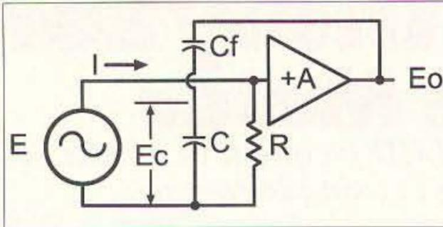
Fig. 1. A negative capacity can be generated.
