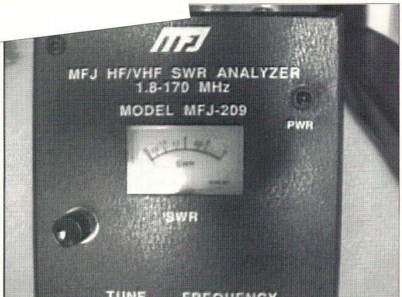
Photo C. The momentary push-button is mounted just to the left of the meter face.
