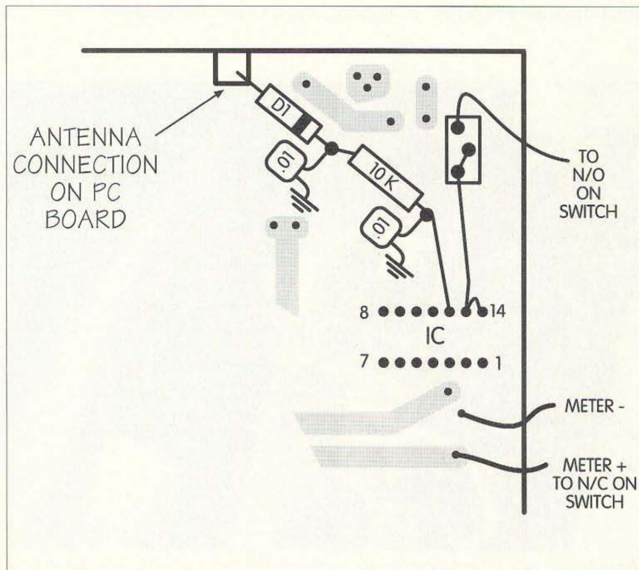
Fig. 2. Board connections.
