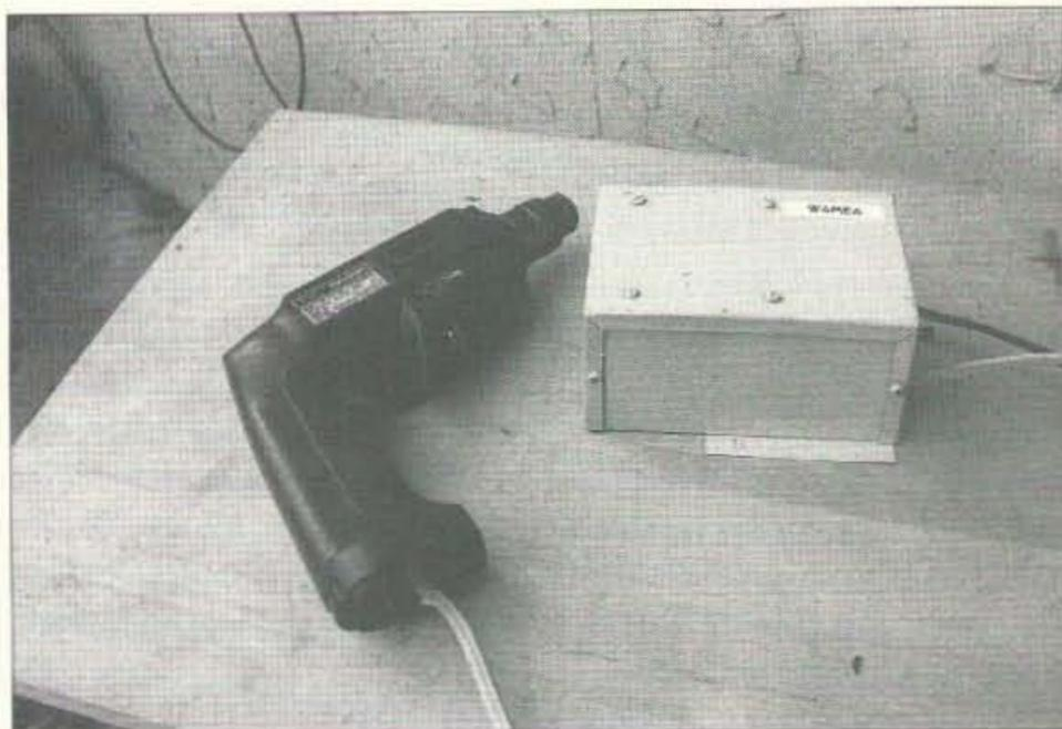
Photo A. W4MEA's "recycled" cordless drill alongside its home-brew 120 VAC to 12 VDC power supply.
