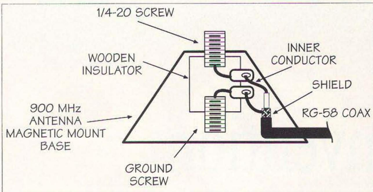
Fig. 2. Internal magnetic base connections.
