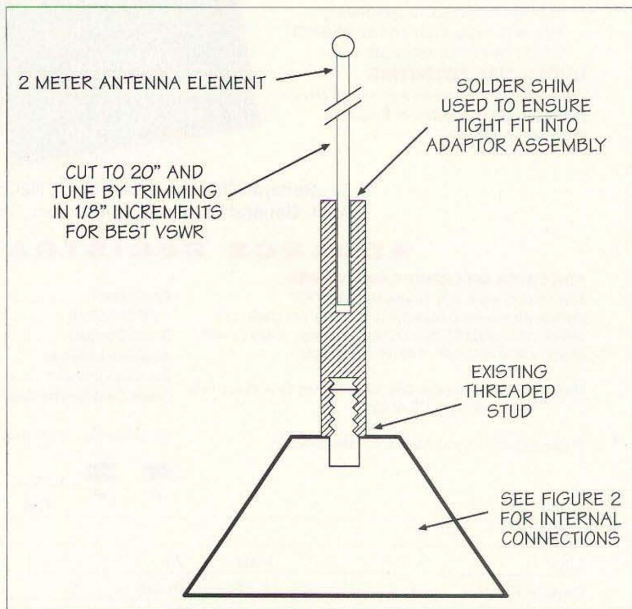
Fig. 3. Whip assembly and tuning details.
