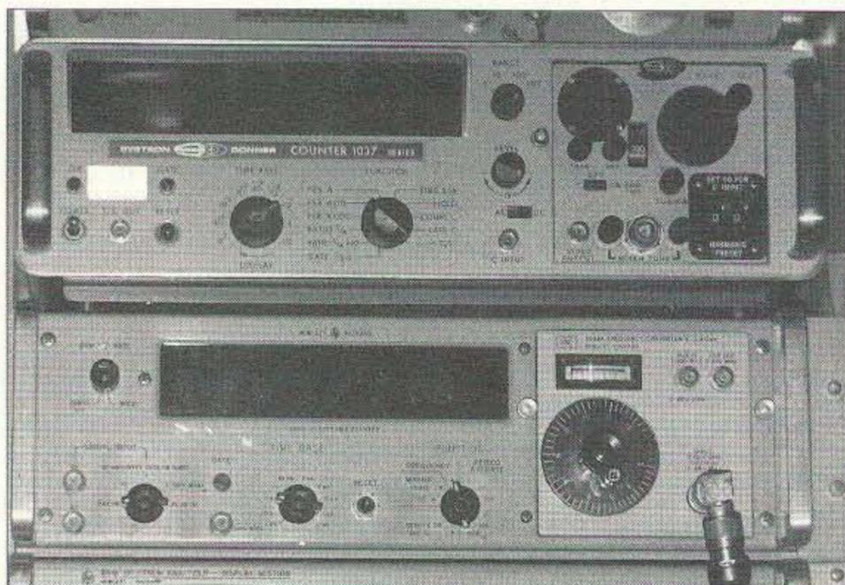
**Photo A.** The old reliable HP-5245 base counter on bottom, shown with the Systron Downer 1037 on top. Not a match but quite similar in operation for main units and plug-in units. (Note: Plug-ins not interchangeable between units.)
