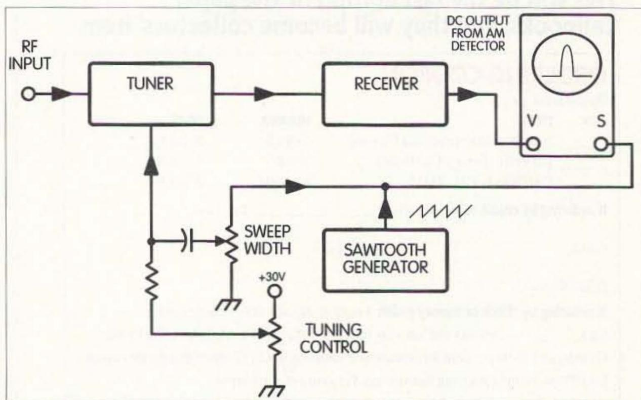
Fig. 1. Spectrum analyzer block diagram.
