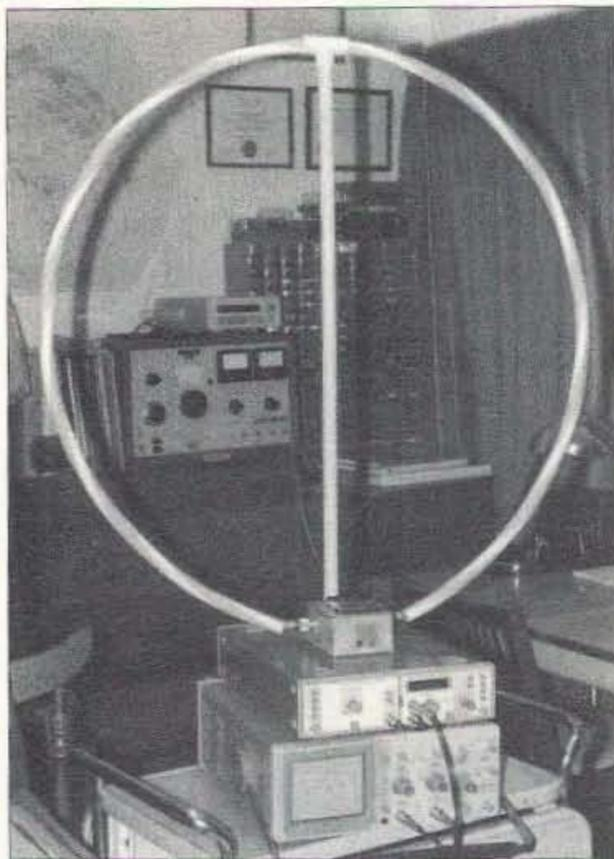
**Photo B.** Calibration was done by substituting the hula hoop for a standard calibrated loop located on top of a spectrum analyzer. The signal generator in the background was used to establish a calibration reference point for each band.
