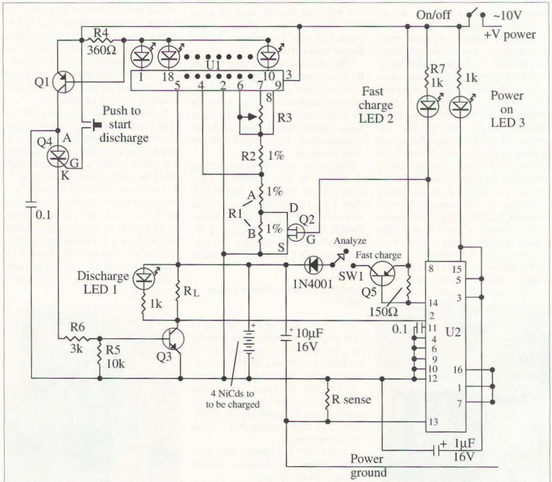
Fig. 1. The NiCd Health & Fitness Center schematic. Q1 = PN2907. Q2 = ZVNL110A MOSFET. Q3 = PN2222. Q4 = SCR EC103B. Q5 = TIP32 with heat sink. R1A = 2.94k 1%. R1B = 1.82k 1%. R2 = 2.94k 1%. R3 = 2k multiturn. R sense = 1Ω 1W. RL = 33Ω 1W. All resistors 5% unless noted. U1 = LM3914. U2 = MAX713.
