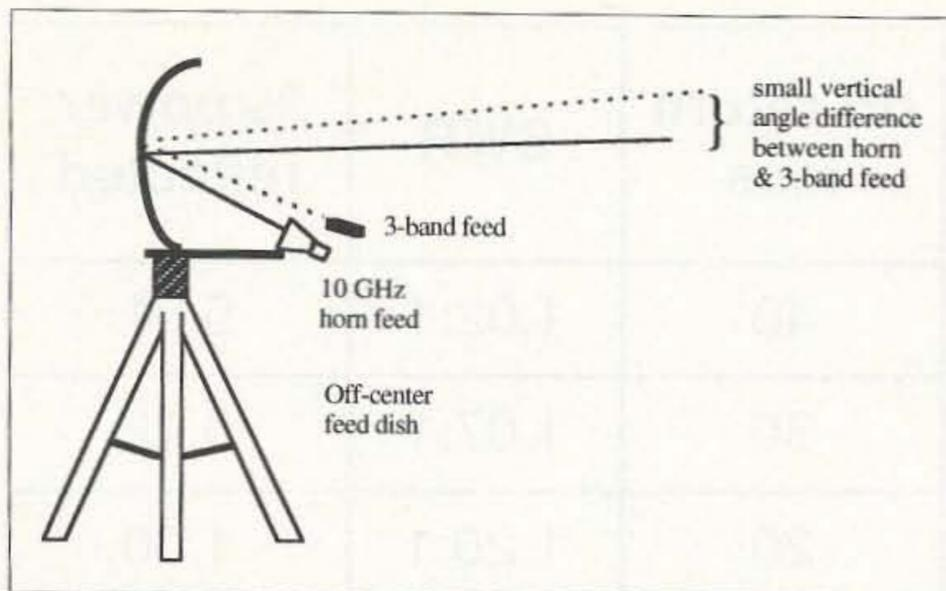
**Fig. 3.** Drawing of triband feed mounted on my off-center-feed dish with 10-GHz horn feed attached. The WA3RMX triband feed is held in place with a length of RG-141 semi-rigid solid copper jacket microwave coax. The RG-141 coax is bent and formed to position the 3-band feed just above the 10-GHz horn at the focus point. Slight vertical realignment is necessary to align either the horn or the tri-band feed. No repositioning is required in horizontal position.
