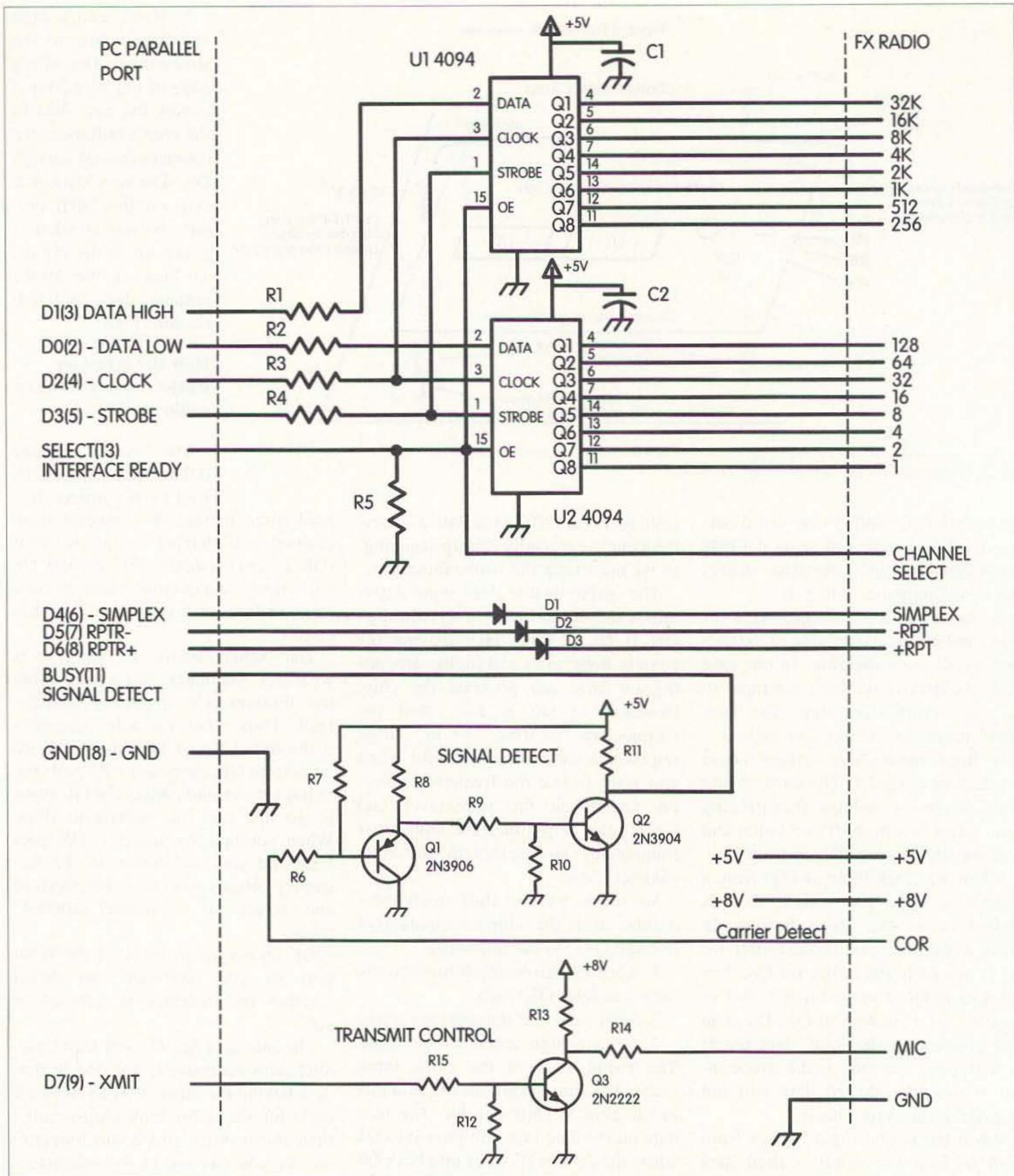
Fig. 3. Ramsey FX radio/PC interface.
