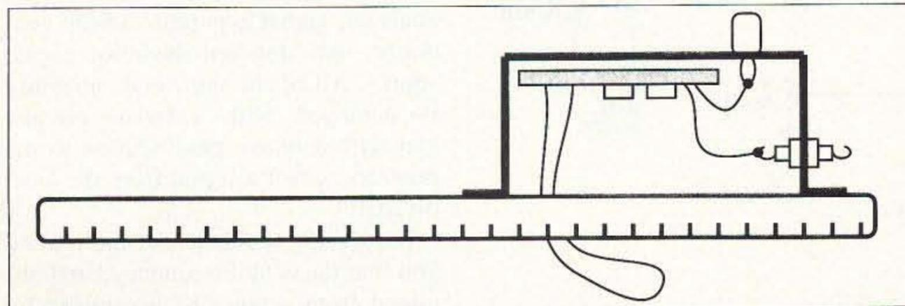
Fig. 3. Amplifier mounting and coupling. The pickup loop feeds signal from the oscillator to the amplifier board.
