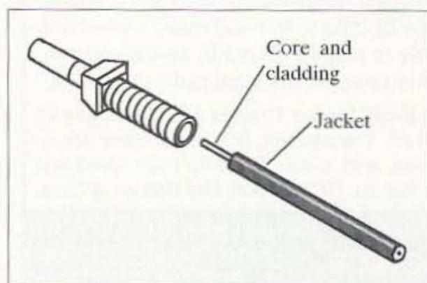
Fig. 1. One type of plug for plastic fiber.
