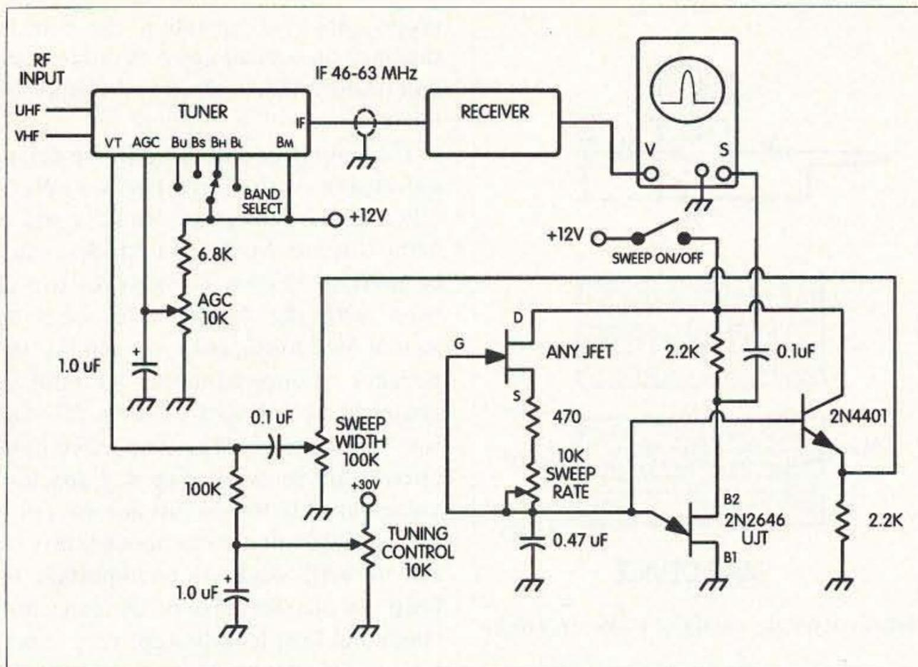
Fig. 2. Spectrum analyzer schematic.
