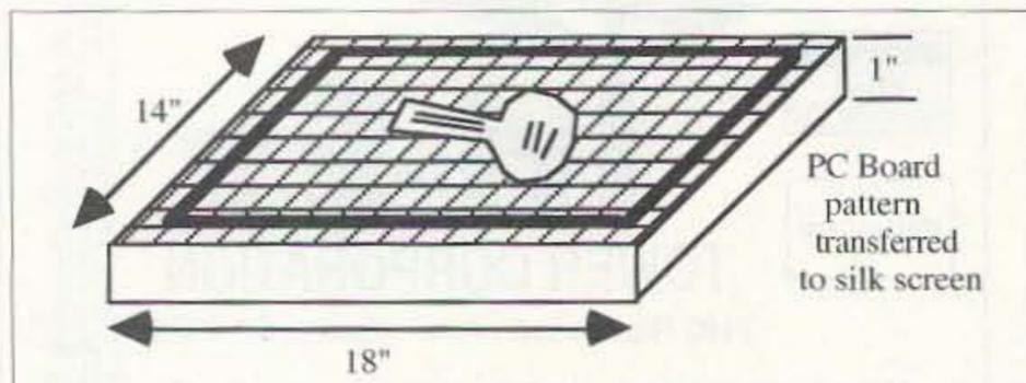
**Fig. 1.** A typical silk-screen showing a home-made wooden frame made from 1- by 2-inch pine. Black line is window screen tubing to hold fine-mesh silk-screen material in cut in bottom of wood. Make screen taut like a GI bunk. Screen material is actually nylon with 306 mesh threads per inch. The original process used silk, hence the name.
