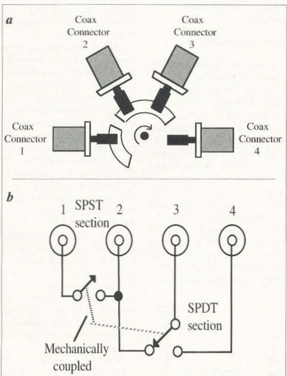
Fig. 4(a). Rear internal view of the B&W Model 551A coaxial bypass switch showing its inner construction. It's basically an SPDT switch (via connectors 2, 3, and 4) ganged with an SPST "secondary" switch (via connectors 1 and 2). The switch is shown in its normal (nonbypassed) position.
