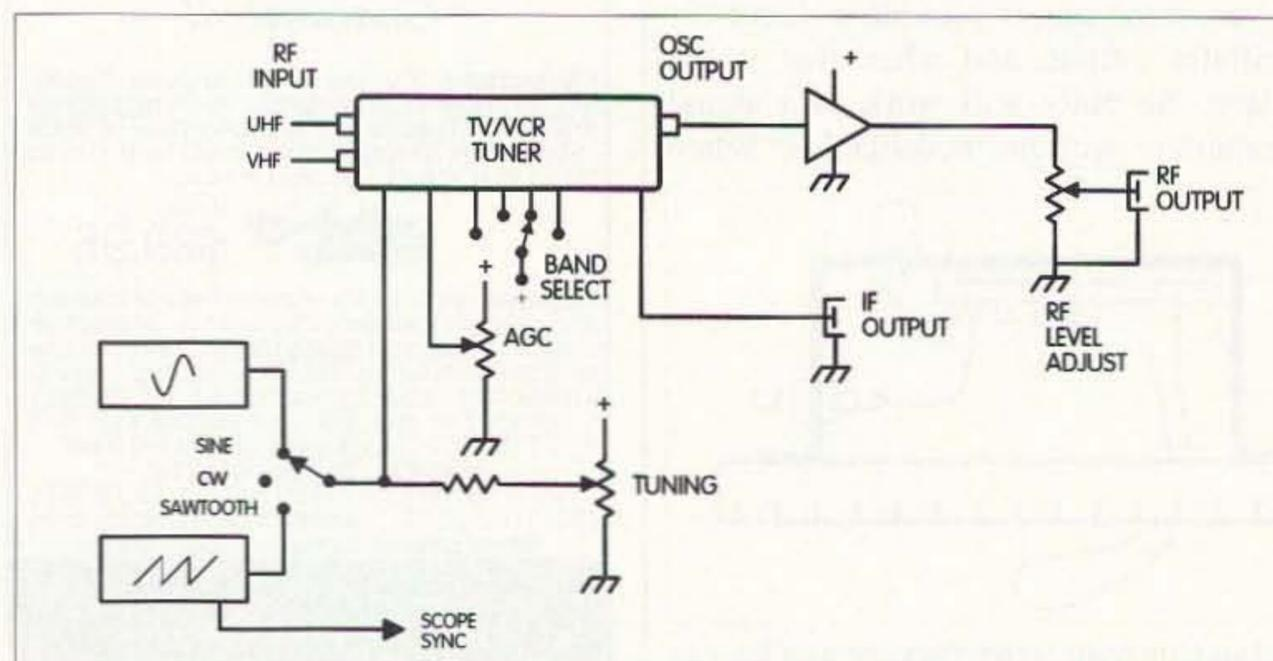
Fig. 5. Multifunction signal device block diagram.
