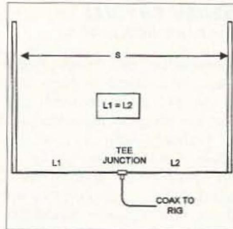
**Fig. 3.** Configuration of antennas using phasing box.
