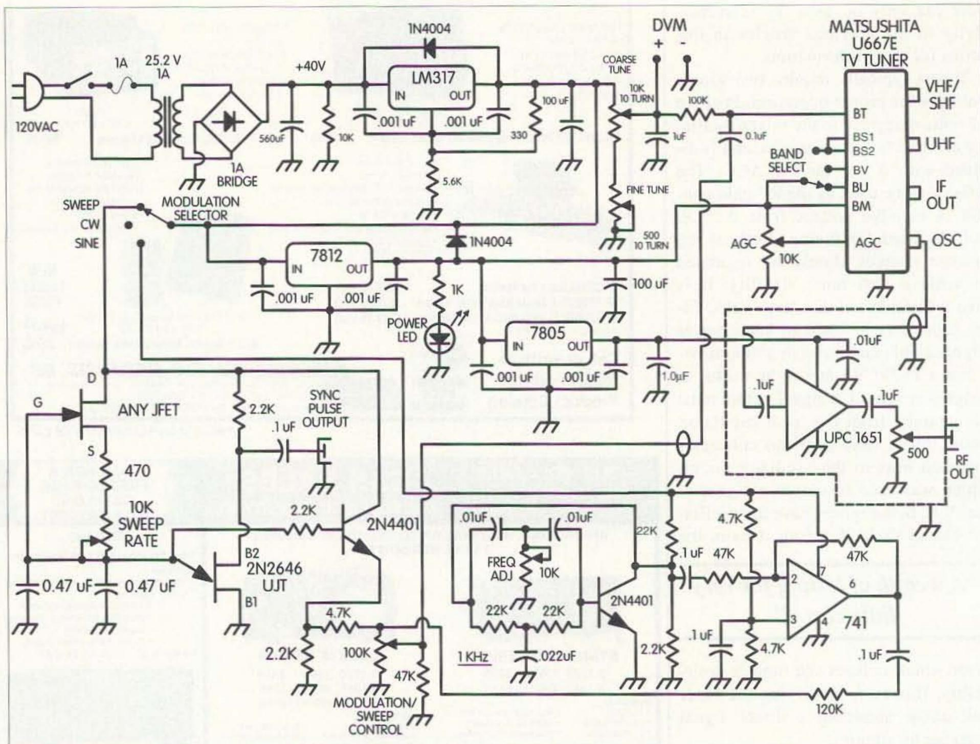
Fig. 6. Multifunction signal device schematic.
