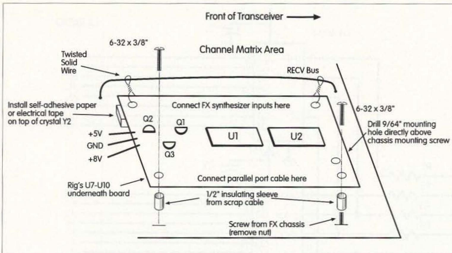
Fig. 2. Mounting details, view from the left side.
