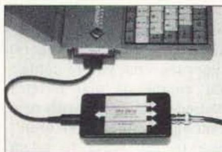
The Viking is a high-performance computer-controlled synthesized VHF satellite receiver—in a miniature low-cost (\$445 with software) unit made for use in harsh mobile, portable and base station environments. It works with the companion PC
