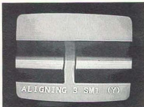
Fig. 5. TV display from the automatic splicer.
