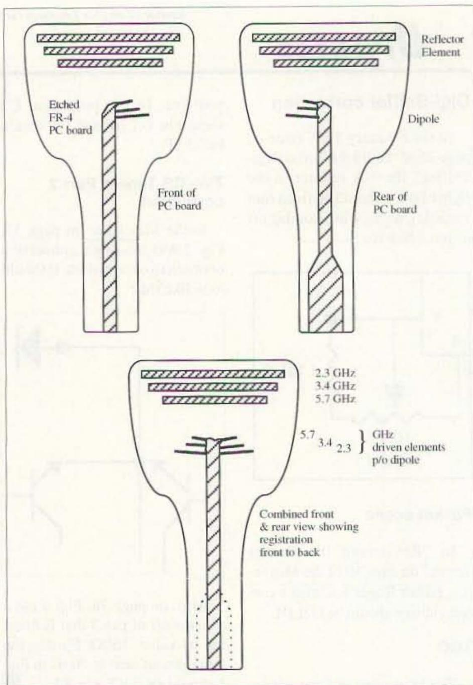
**Fig. 2.** Diagram of WA3RMX tri-band feed showing the rear and front sides of the PC board. Double-sided PC board is required, with an exact registration between both sides. Solder rear side wide trace to shell of RF connector, narrow trace to center pin. Scale artwork is available in The ARRL UHF/Microwave Projects Manual.
