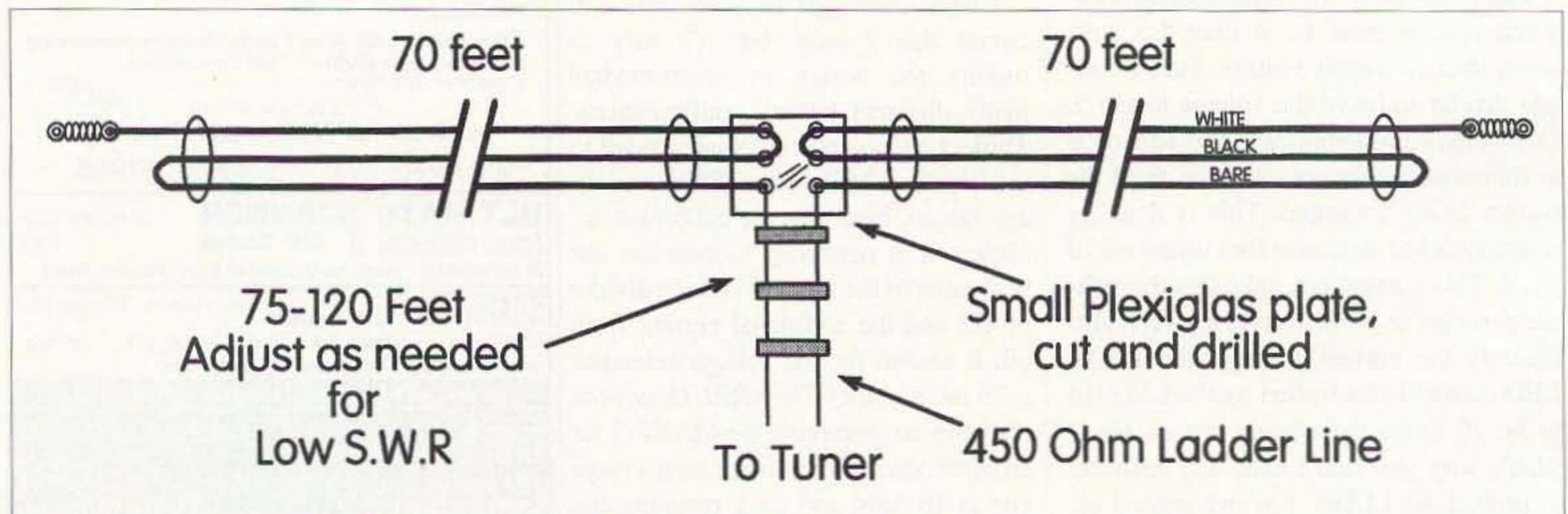
Fig. 1. The configuration for the "Cobra."
