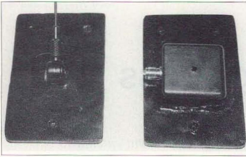
**Photo C.** Baseplates with epoxied antenna pad and coupler. The Plexiglas was painted black after construction.
