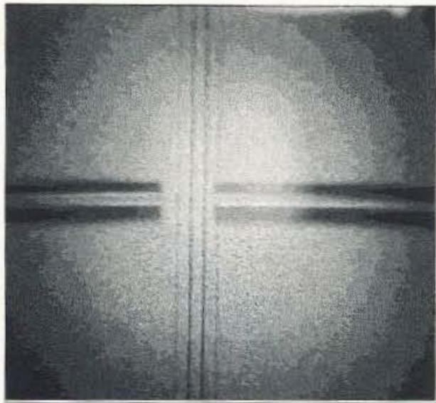
Fig. 3. Microscope display on semi-automatic splicer.
