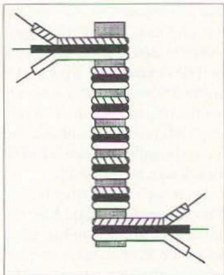
Fig. 5. Trifilar winding scheme for toroids.
