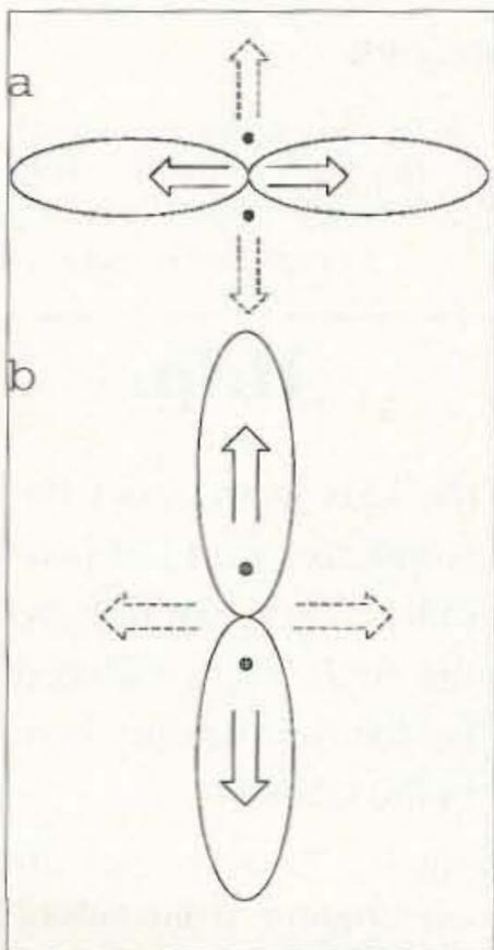
**Fig. 1.** Direction patterns for two verticals a half wavelength apart: (a) antennas in-phase ( $0^\circ$ ); (b) antennas out-of-phase ( $180^\circ$ ).
