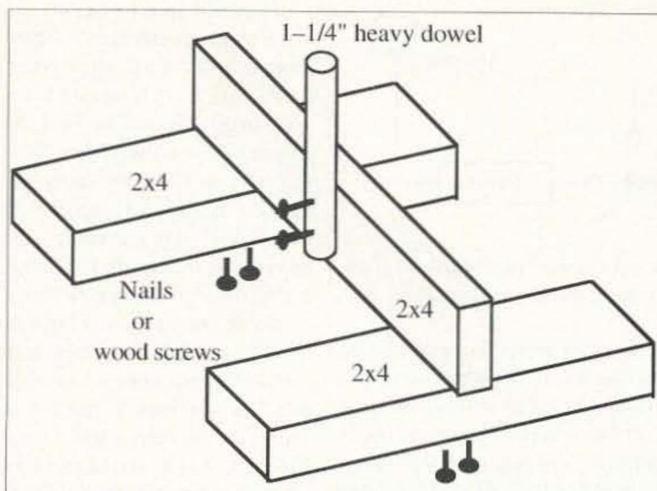
Fig. 3. AD1B's attic beam antenna suggestion.
