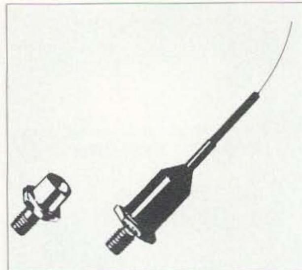
Fig. 6. Semiconductor laser diodes.
