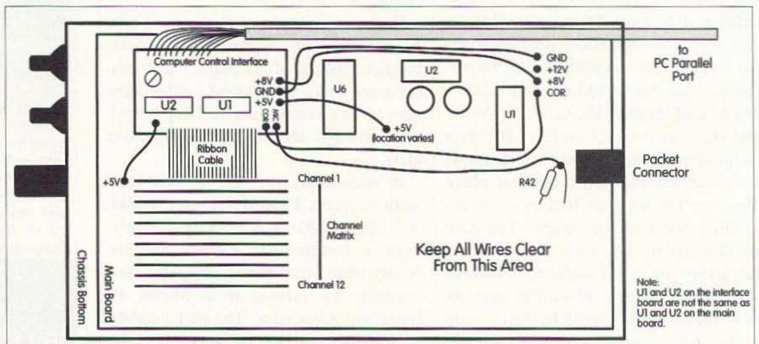
Fig. 1. The Computer Control Interface mounted above the Ramsey transceiver's address chips.
