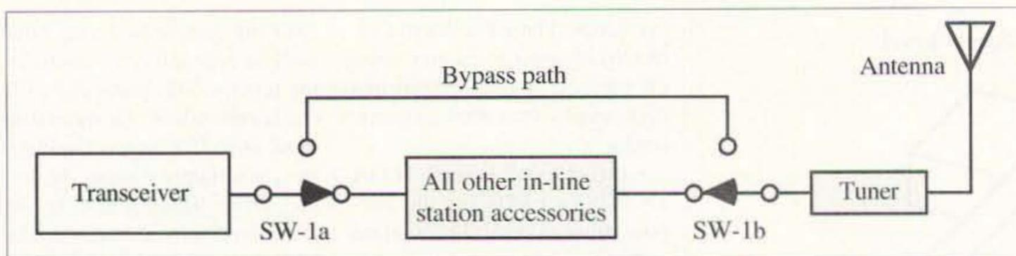
**Fig. 5.** Coaxial bypass switch being used to completely bypass all in-line accessories (with the exception of an antenna tuner) to eliminate potential sources of trouble quickly... without having to sign off the air.
