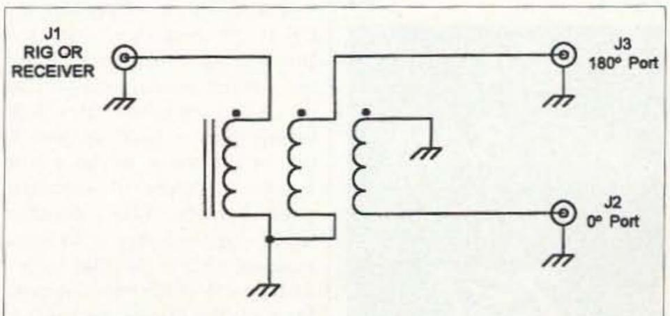
**Fig. 4.** Circuit of phasing box.
