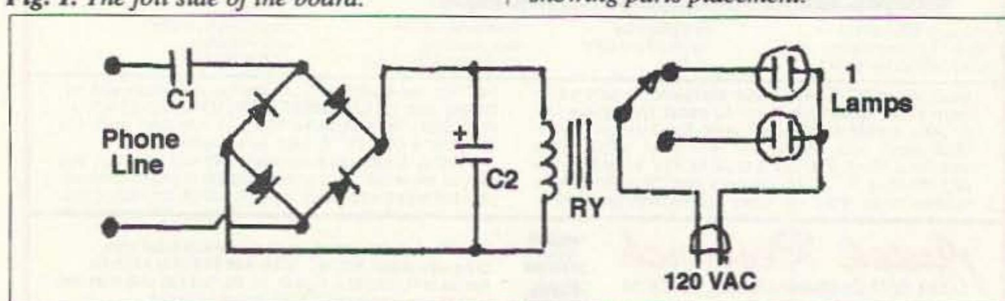
Fig. 3. The circuit diagram.
