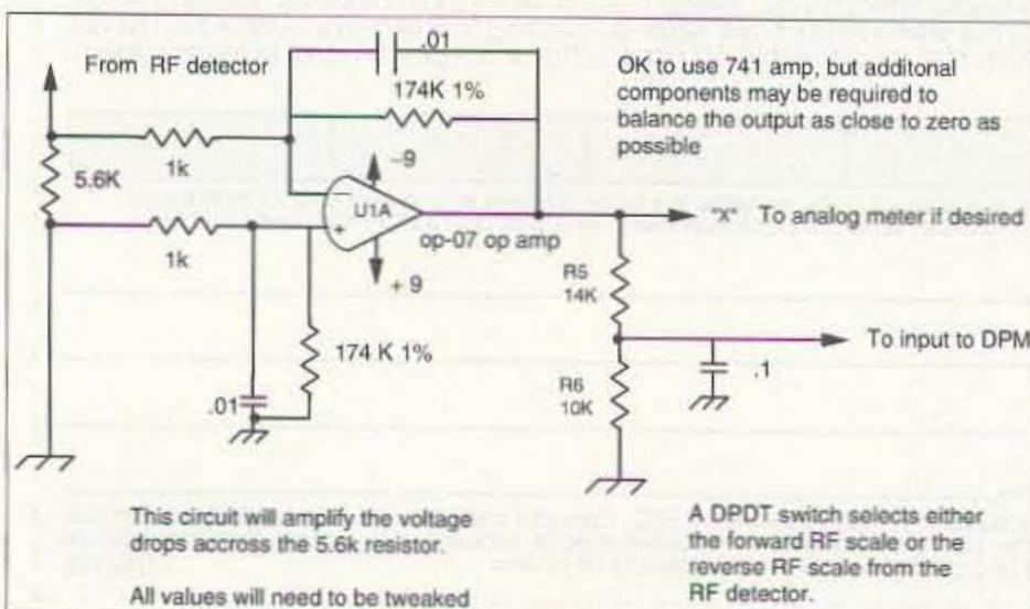
Fig. 1. Schematic of the DPM.
