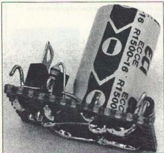
Photo B. The on-delay timer construction details.
