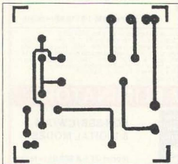
Fig. 1. The foil side of the board.
