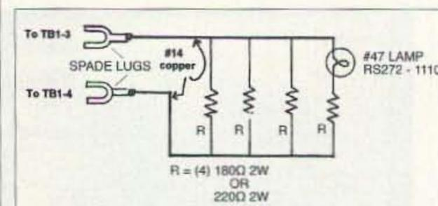
Fig. 5. Terminating RF detector.
