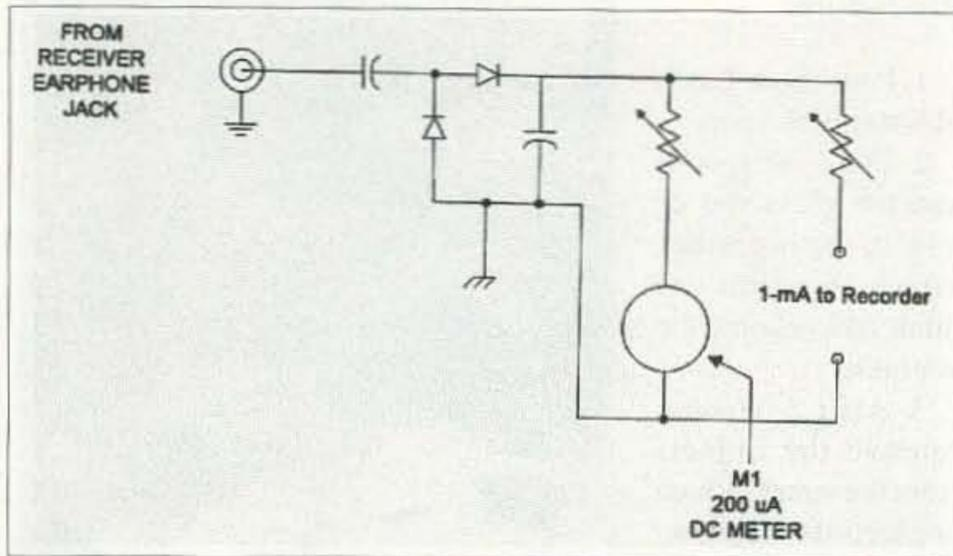
Fig. 1. Audio-to-DC converter for recording signal levels.
