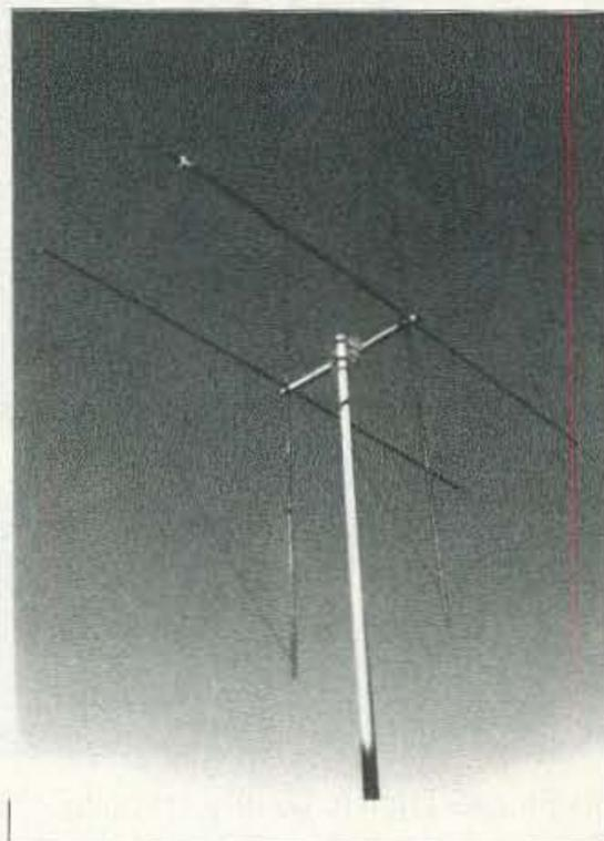
driven element pre-marked for a resonant frequency of 50.4 MHz, giving the antenna a bandwidth of 1.5 MHz at an SWR of less than 1.7 to 1. The antenna can be rotated for horizontal or vertical polarization, and has a boom length of 27 inches. The best feature is the price of \$69.95 F.O.B. BREA CA, PLUS \$12 S & H. Circle Reader Service No. 202.
