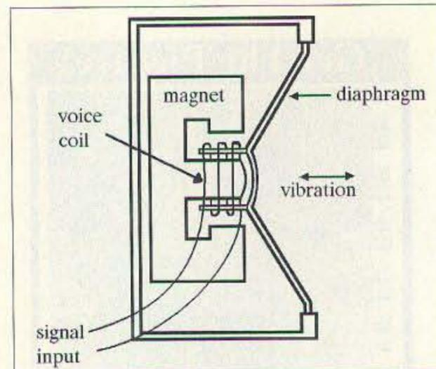
Fig. 3. A telephone-type earphone.
