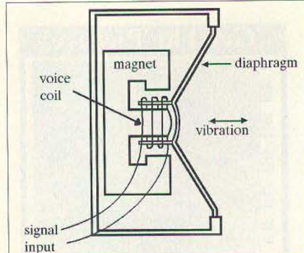
**Fig. 3. A telephone-type earphone.**
