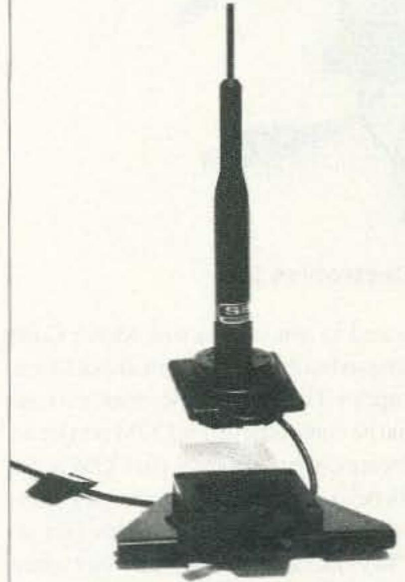
The COMET "Quick-Disconnect" Mobile Antenna Mount, Model CQ-5M consists of two separate sections: A trunk-mount base that is attached to the trunk edge with four set screws, and an antenna-mount base that fits inside the trunk-mount base. Sliding a lever wedges the antenna-mount base securely in place. To remove the antenna, simply slide the lever to unlock. The antenna can then be placed inside the trunk. Comet's 17-foot
