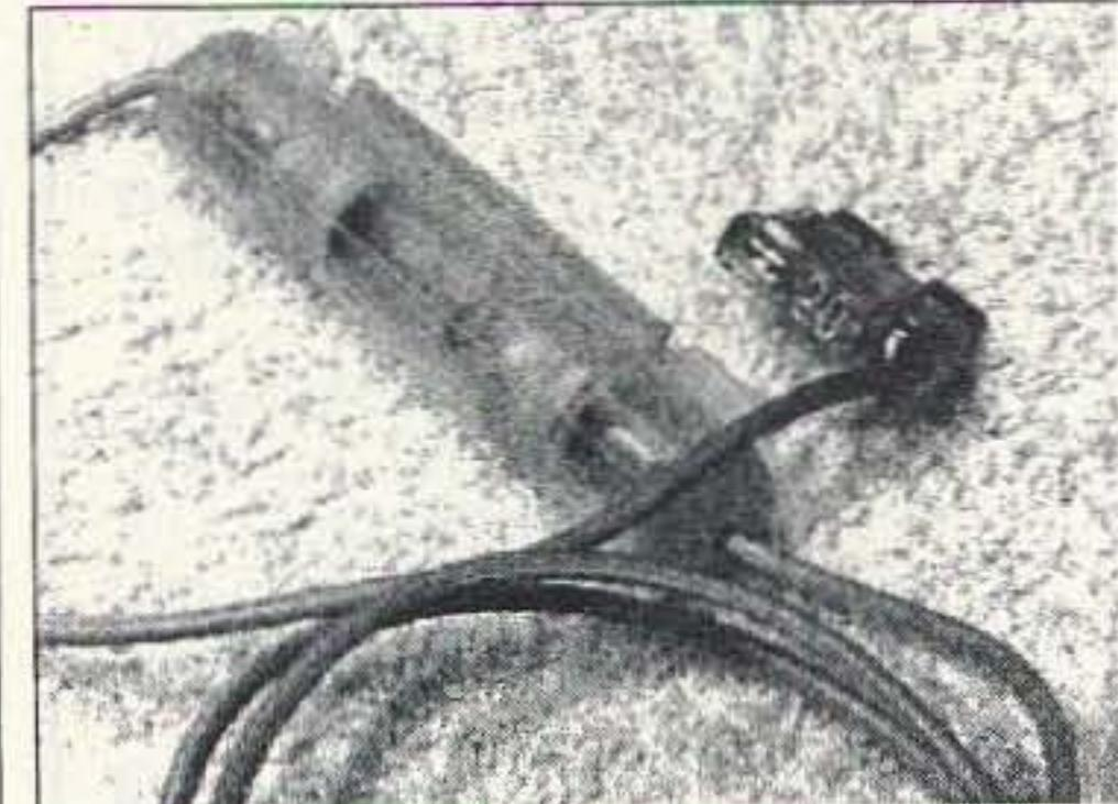
**Photo C.** Modified "blade-type" fuse useful in connecting to a car's key-switch circuit.
