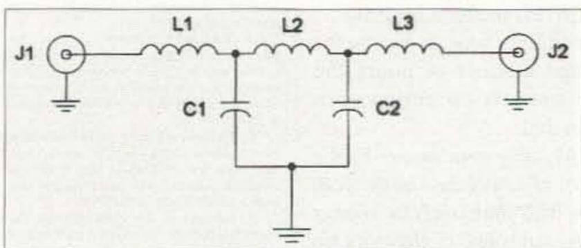
Fig. 2. Low-pass filter circuit.
