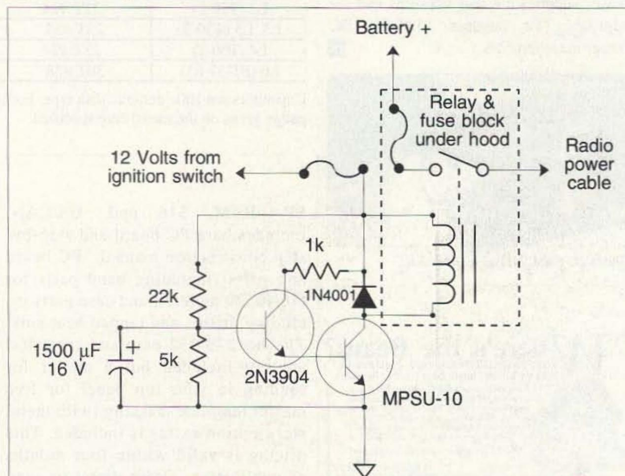
Fig. 1. The on-delay timer circuit.
