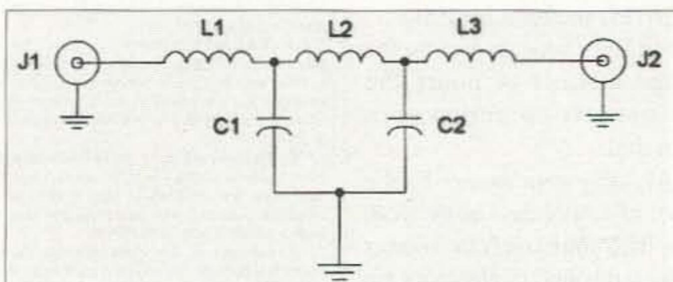
Fig. 2. Low-pass filter circuit.
