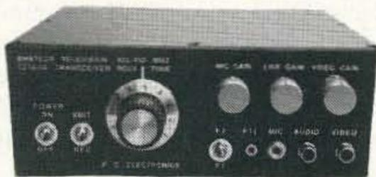
Snow free line of sight DX is 90 miles - assuming 14 dBd antennas at both ends. 10 Watts in this one box may be all you need for local simplex or repeater ATV. Use any home TV camera or camcorder by plugging the composite video and audio into the front phono jacks. Add 70cm antenna, coax, 13.8 Vdc @ 3 Amps, TV set and you're on the air - it's that easy!
