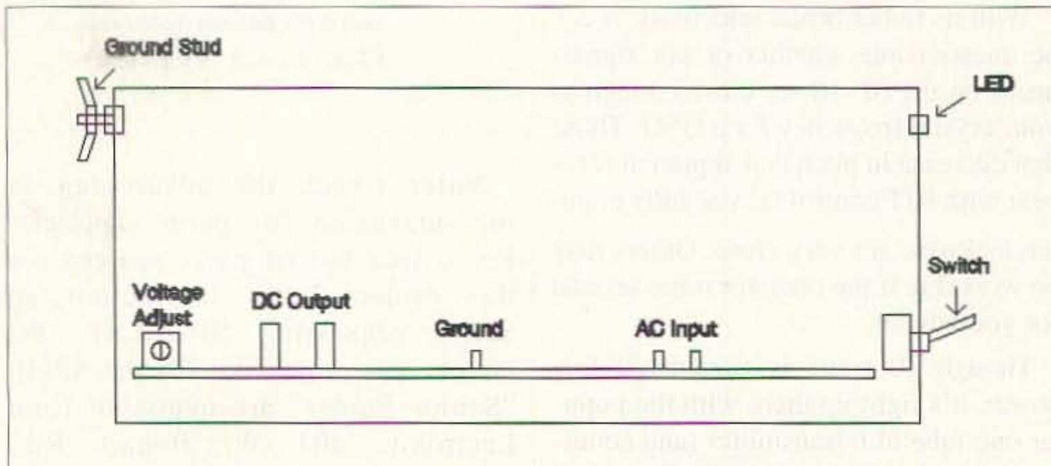
Fig. 1. Switching power supply side view.
