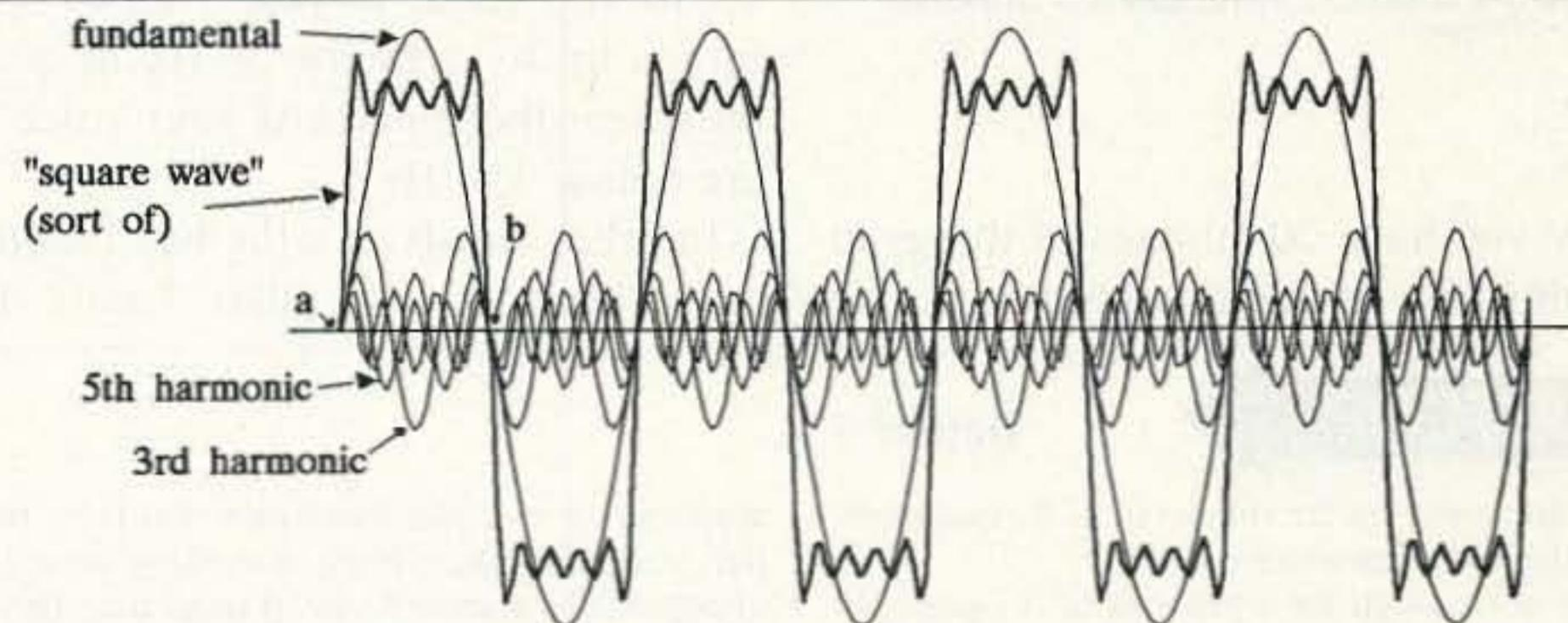
Fig. 10. Making a square wave out of a sine wave.
