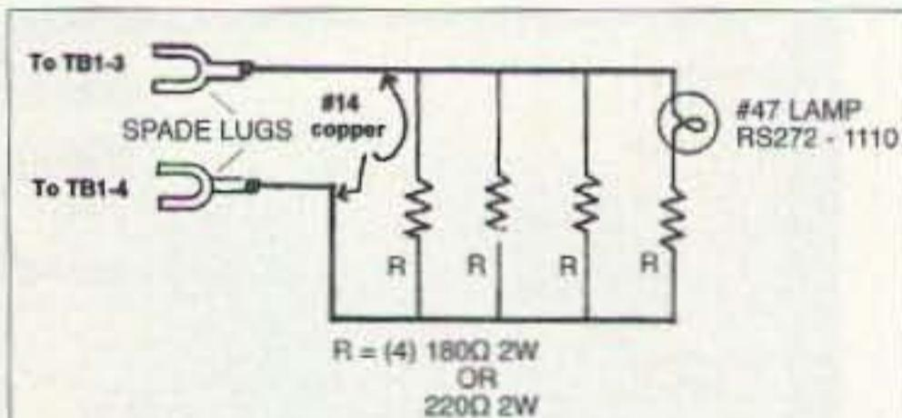
Fig. 5. Terminating RF detector.
