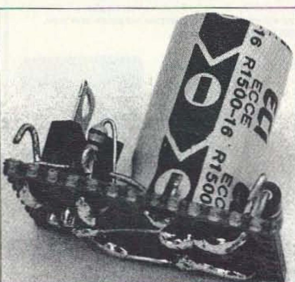
**Photo B.** The on-delay timer construction details.
