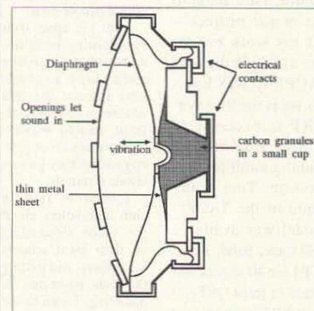
Fig. 1. Telephone-type carbon microphone.
