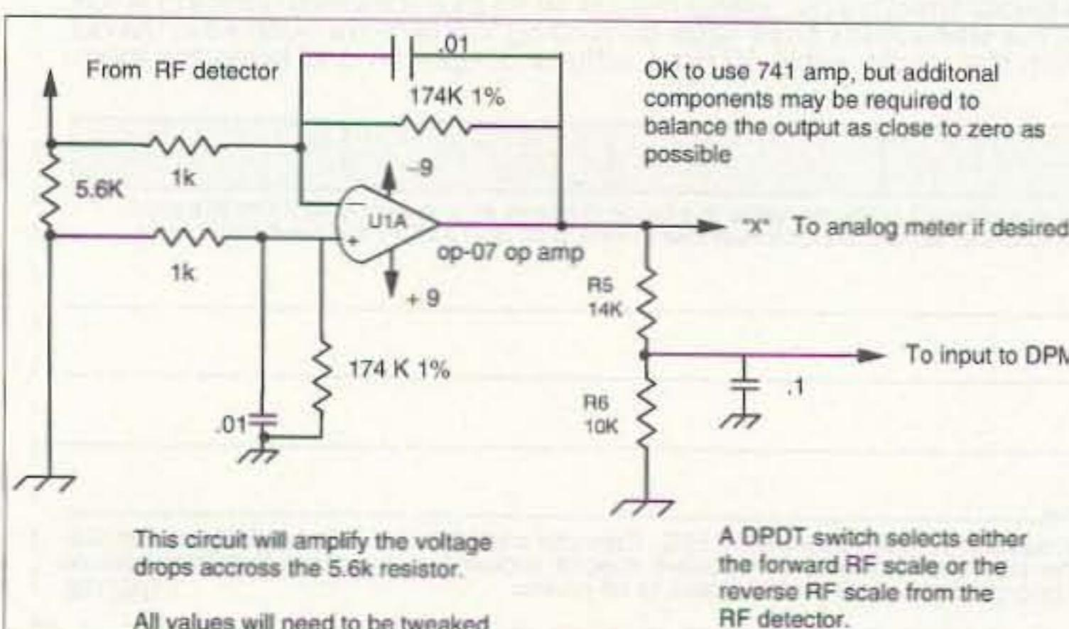
*Fig. 1. Schematic of the DPM.*
