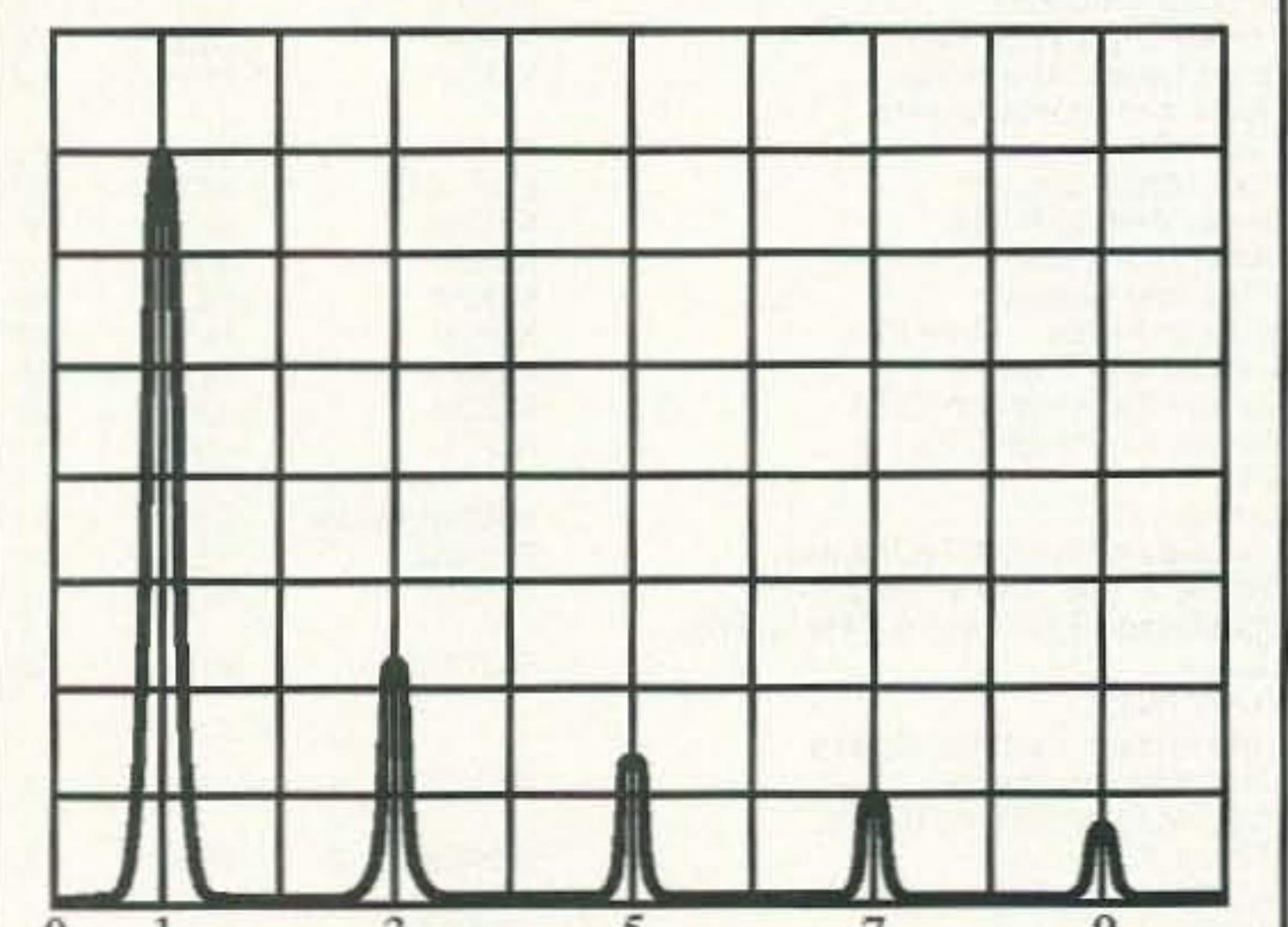
Fig. 12. Spectrum of a 1,000-Hz square wave.
