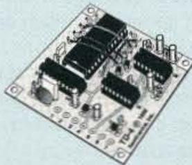
TD-3 CTCSS DECODER/ENCODER. Prevents access to repeater or receiver unless proper tone is present. Tone output for transmitters, too. .... kit \$29, w/t \$59
