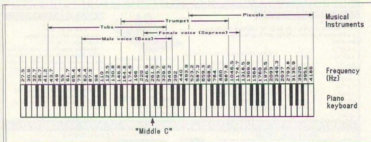
Fig. 7. Frequencies produced by musical instruments.
