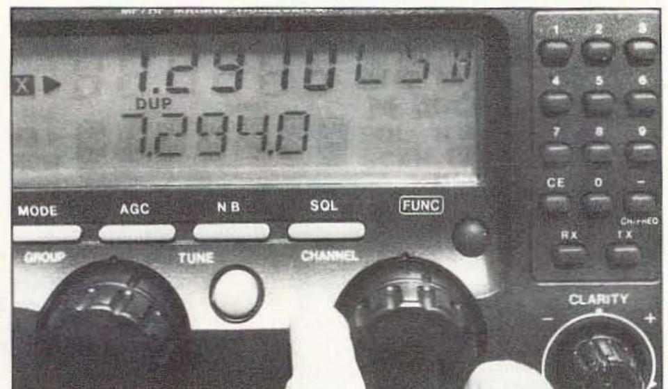
Photo B. Now the IC-M7100 is a ham set, tuned to a 40 meter net on lower sideband.
