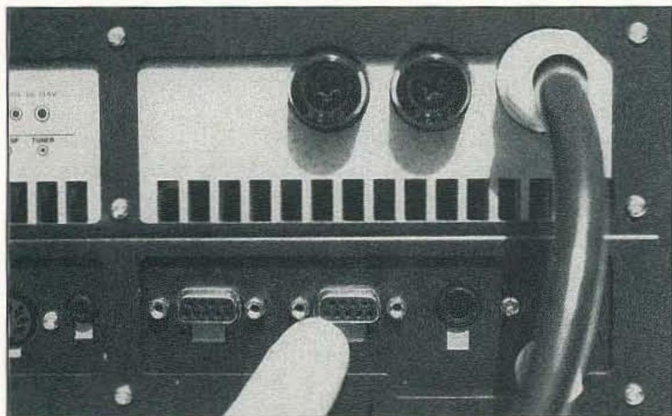
Photo C. The rear of the Icom marine transceiver offers output jacks for weather fax, data, and the APRS positioning service.
