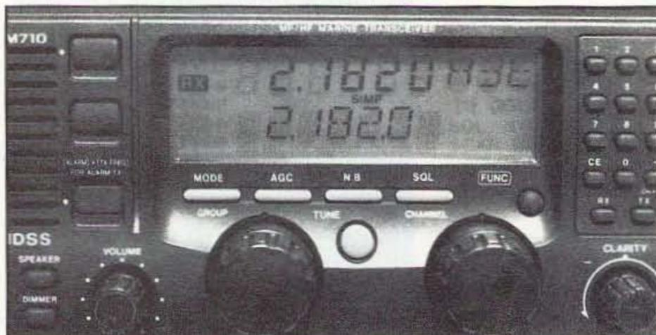
Photo A. The Icom IC-M710 is in the marine SSB mode, set to distress frequency 2182 kHz.
