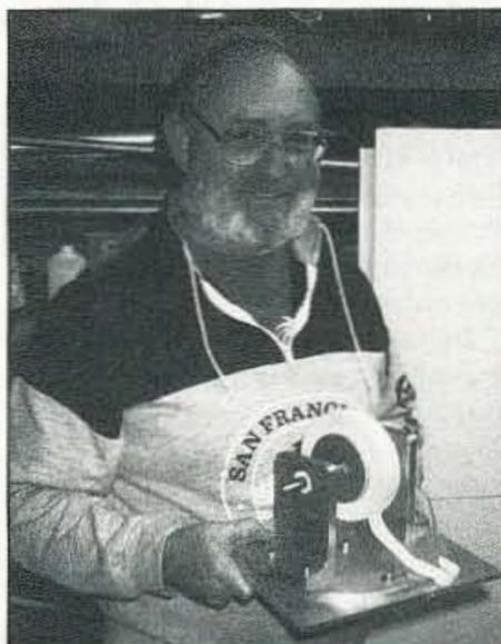
Photo C. Lou McFadin W5DID and the tape spooler used to cover the iron torque rods prior to the coil-winding process.
