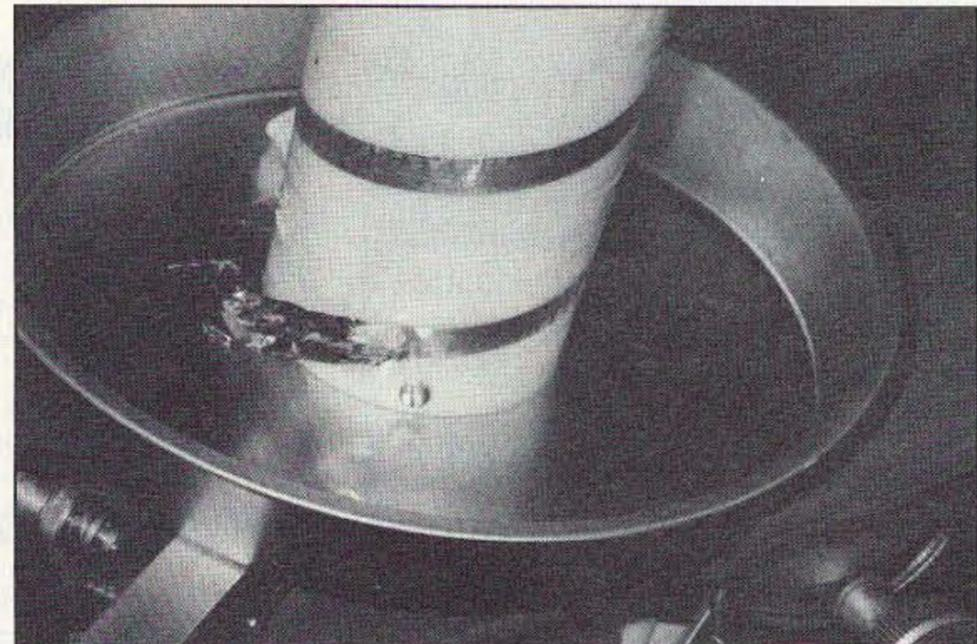
Photo B. Close-up of helical antenna matching section. Use length of copper to adjust match, by varying capacitance to ground (pie tin). Section of copper foil soldered near coax connector and on helical line.
