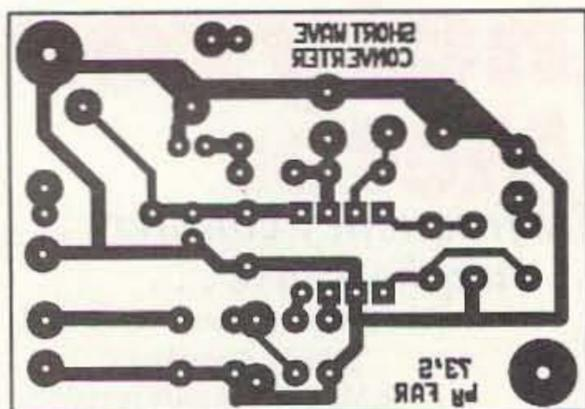
Figure 3. PCB layout and parts placement diagram.
