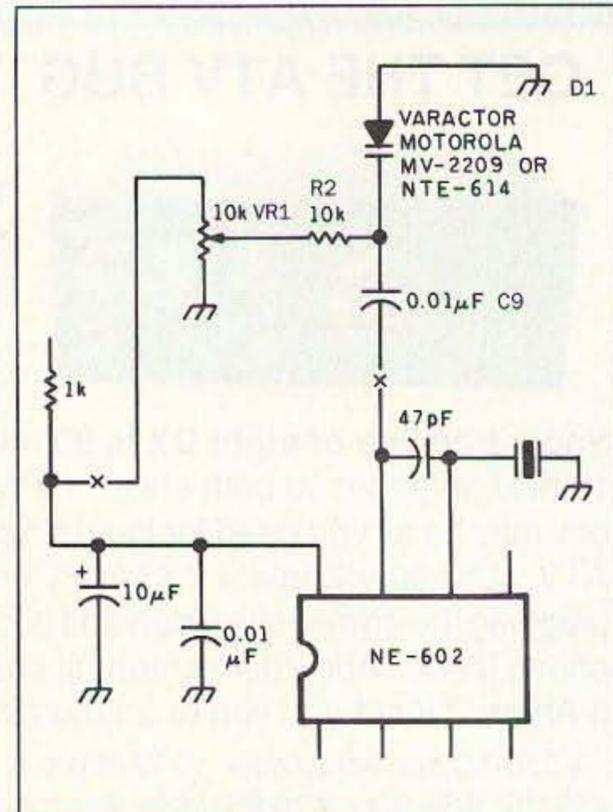
Figure 2. Schematic variation using a crystal tuning circuit with a varactor.
