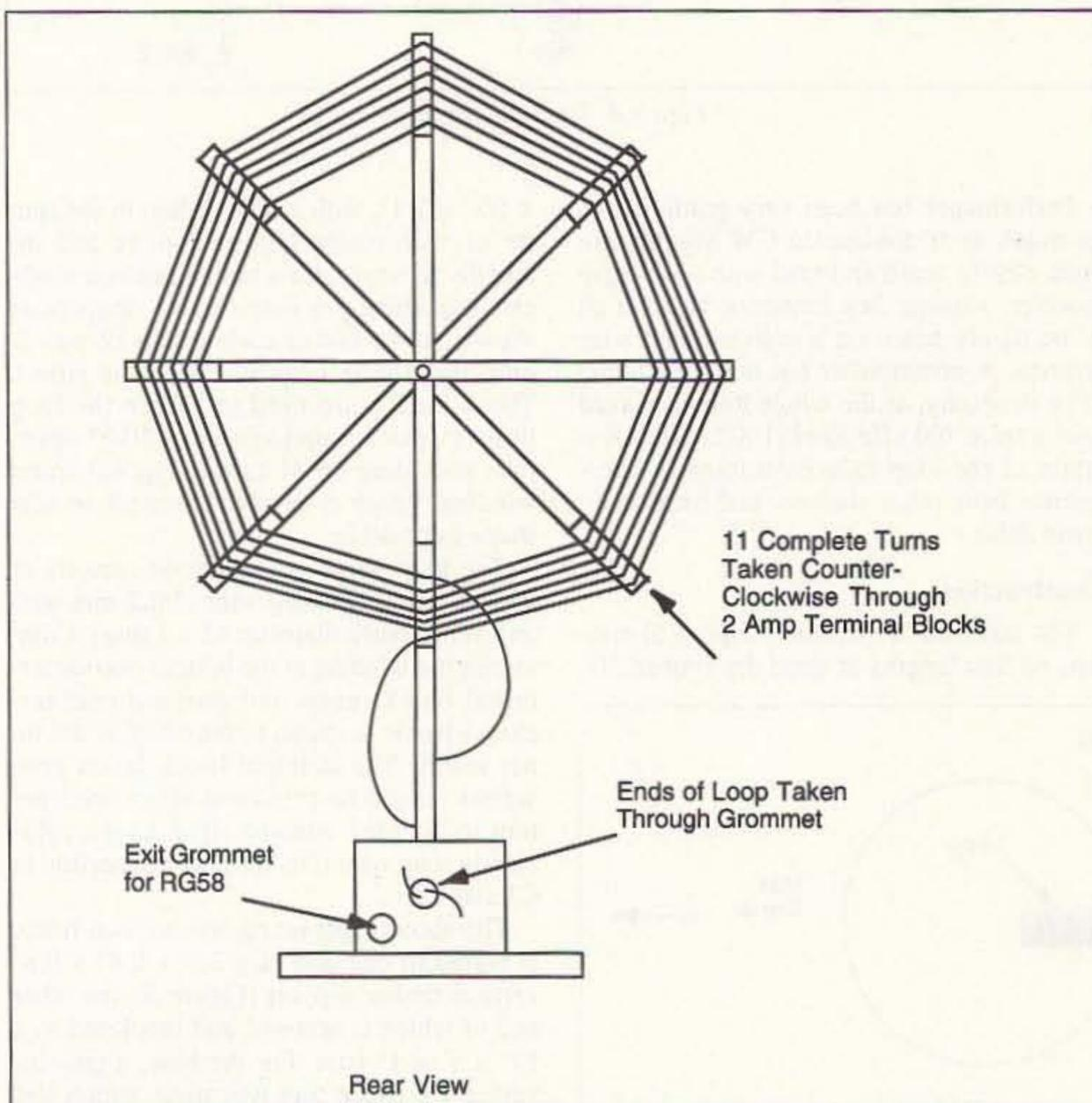
Figure 6. Loop winding detail.
