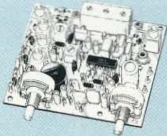
**R76 MONITOR FM RCVR Kit** for 10M, 6M, 73 MHz, 2M, hi-band, or 220 MHz. IF selectivity 60dB at ±12kHz. Great for monitoring repeaters, amateur calling frequencies, or packet radio frequencies, and for listening to commercial two-way radio, police/fire frequencies, or weather forecasts. **Good starter kit, too; easy to assemble and align.** .... **Kit only \$59!**
