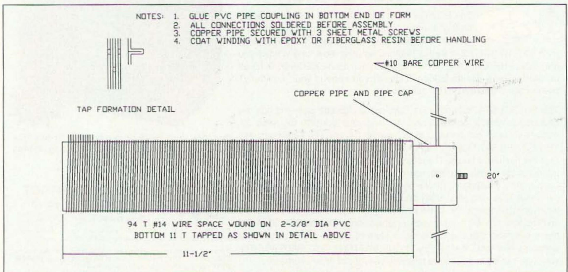
Figure 2. 75 meter resonator.
