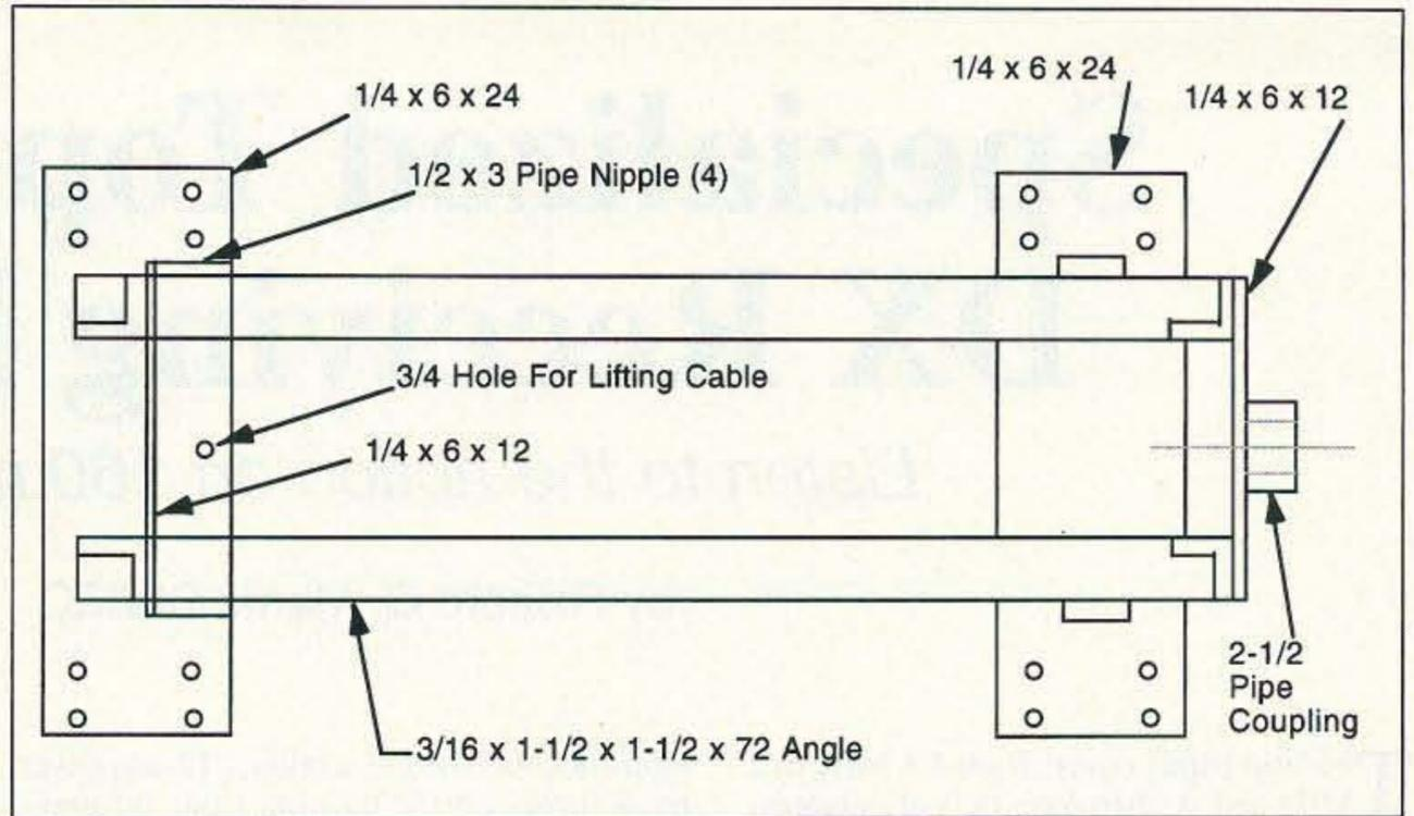
Figure 1. Top view of the elevator.
