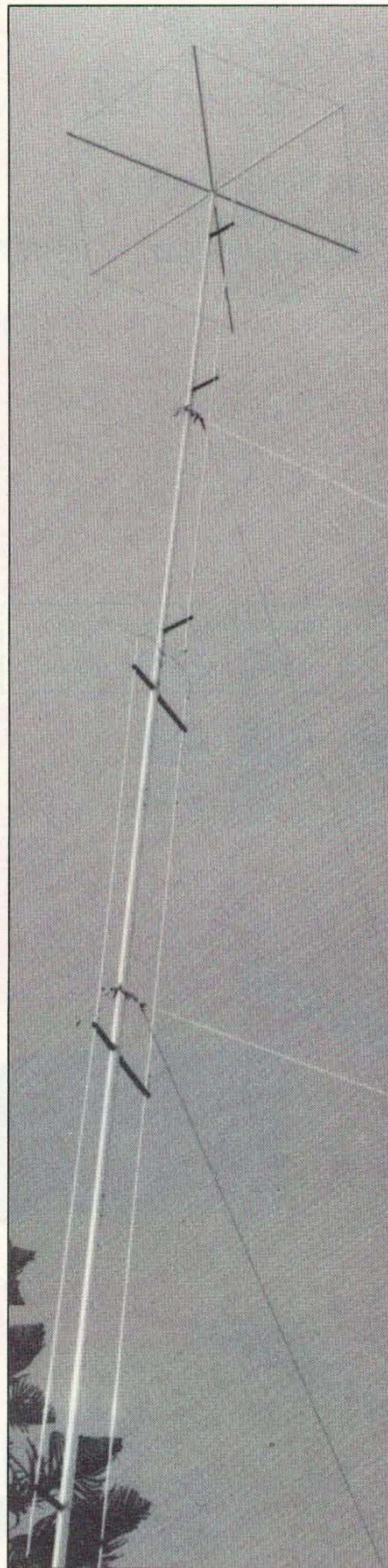
Photo E. The Voyager in place on the roof. Different measurements must be applied to roof mounting—40 meters needed a specific quarter-wave radial.
