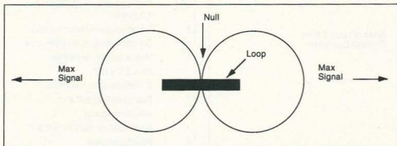
Figure 3. Typical polar diagram of reception.
