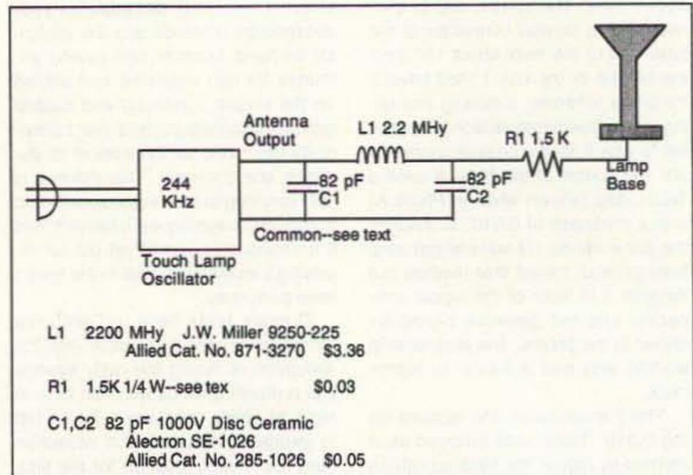
Figure 1. A solution for a 244 kHz touch lamp (see text).
