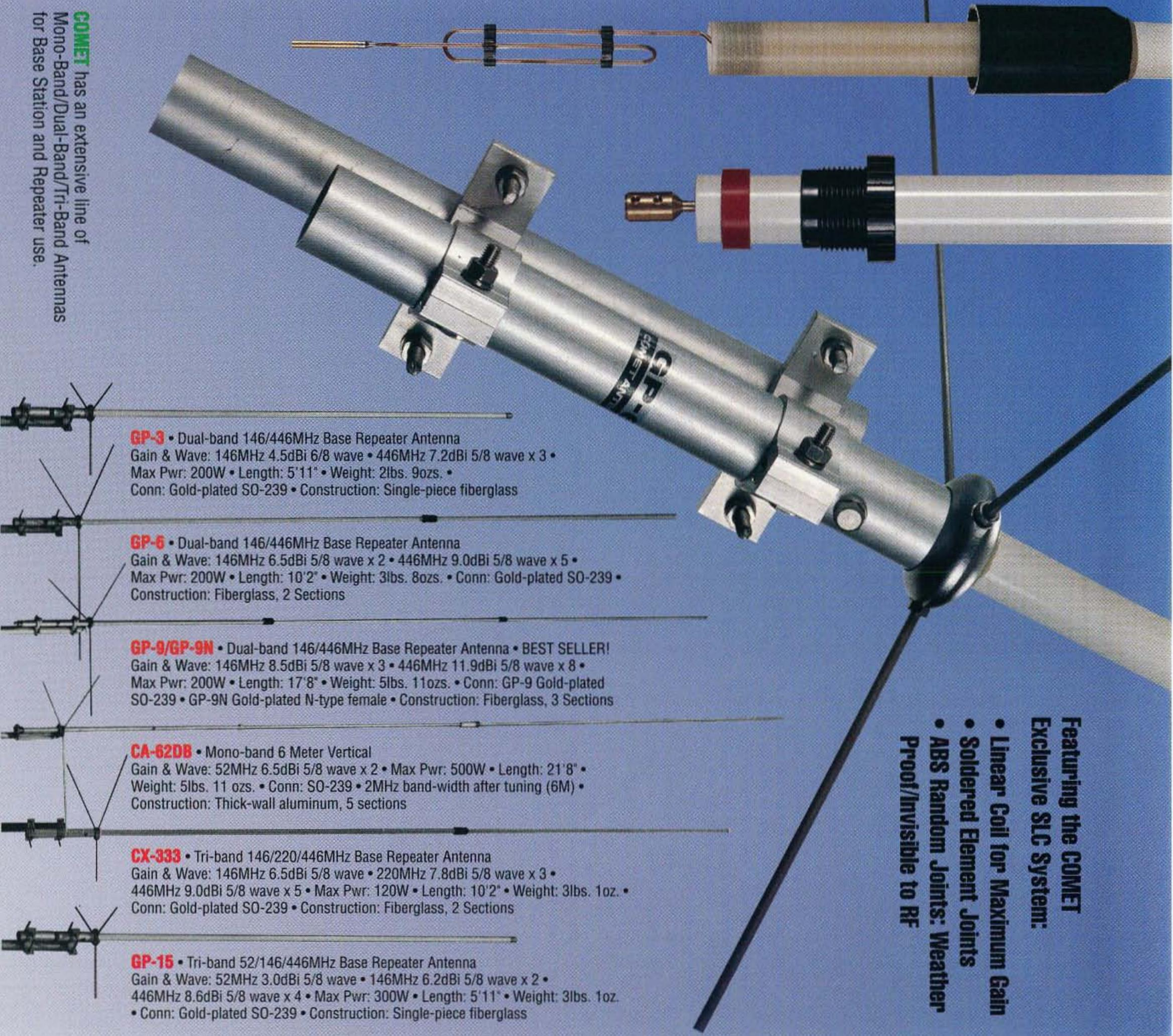
**GP-3** • Dual-band 146/446MHz Base Repeater Antenna
