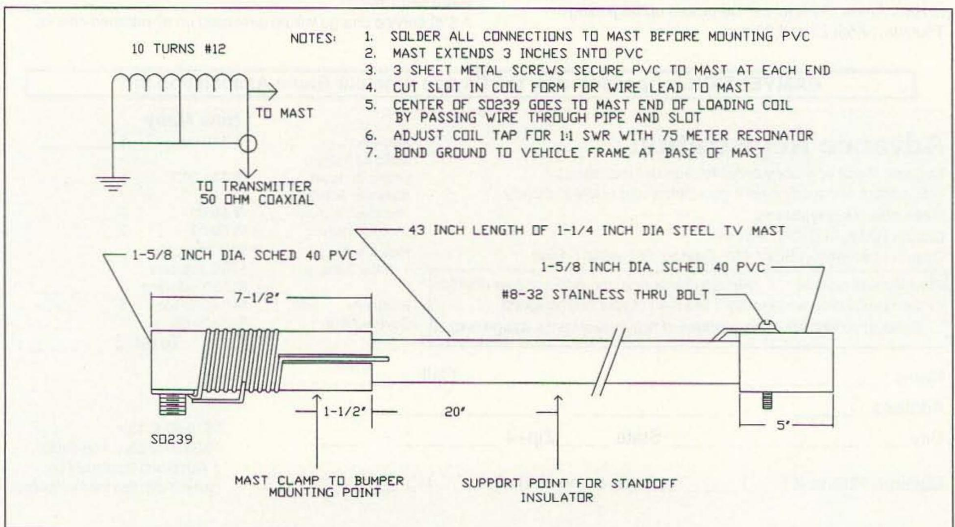
Figure 1. Mobile mast construction detail.
