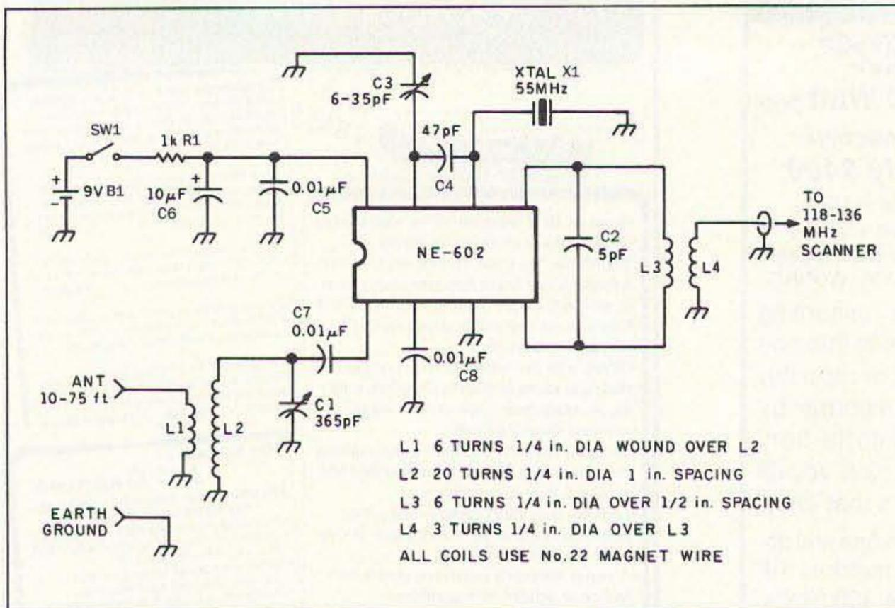
Figure 1. Schematic for the shortwave converter for your scanner.
