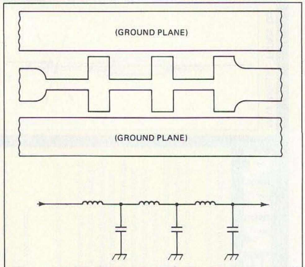
Figure 2. Printed circuit low-pass filter and equivalent circuit.
