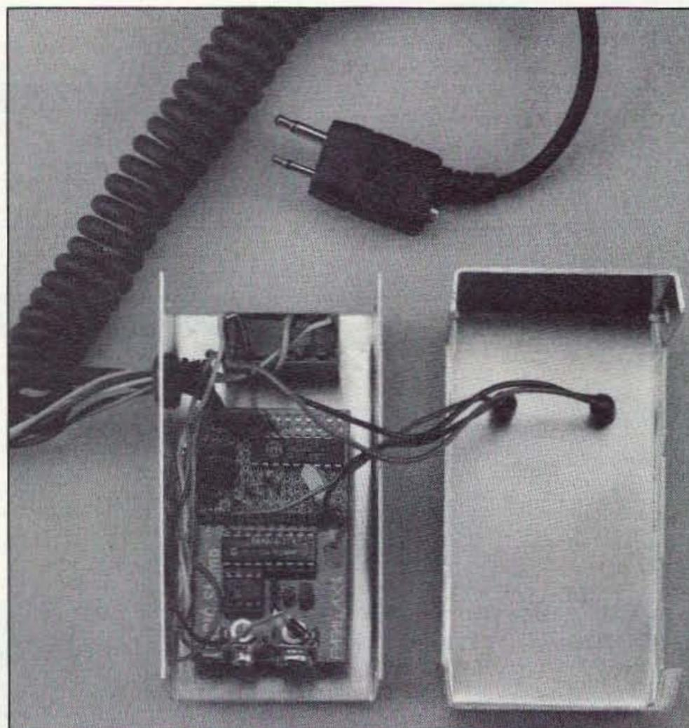
Photo B. The finished Intelligent Relay.
