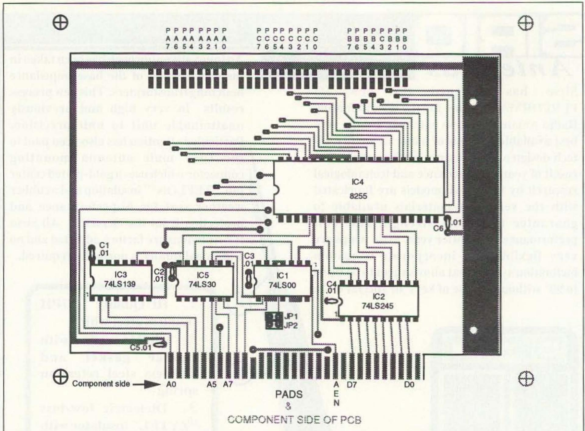
Figure 2. 1:1 PCB component overlay.
