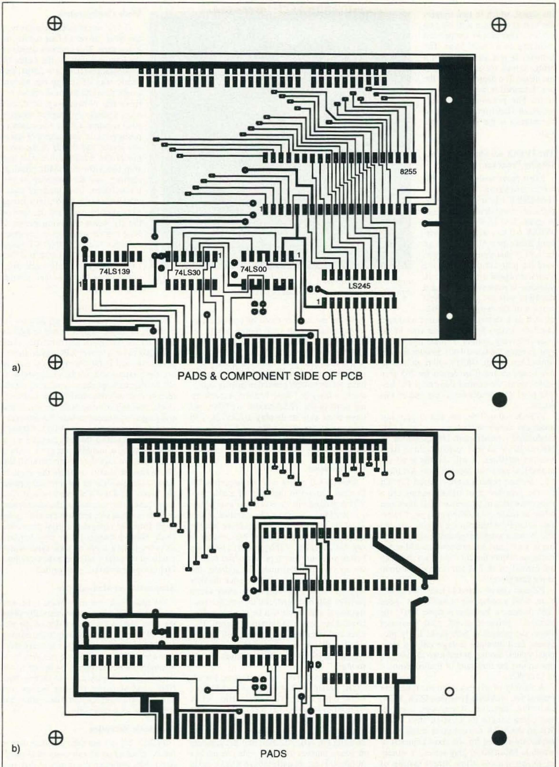
Figure 3a.) 1:1 PCB layout, component side; b) 1:1 PCB layout, solder side.
