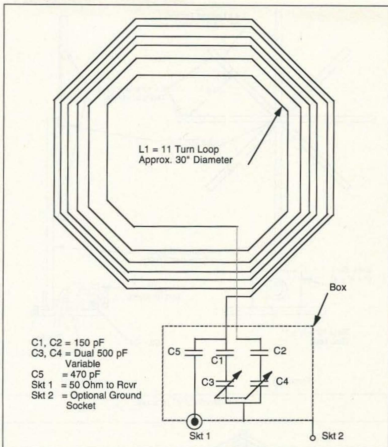
Figure 4. Topband circuit.
