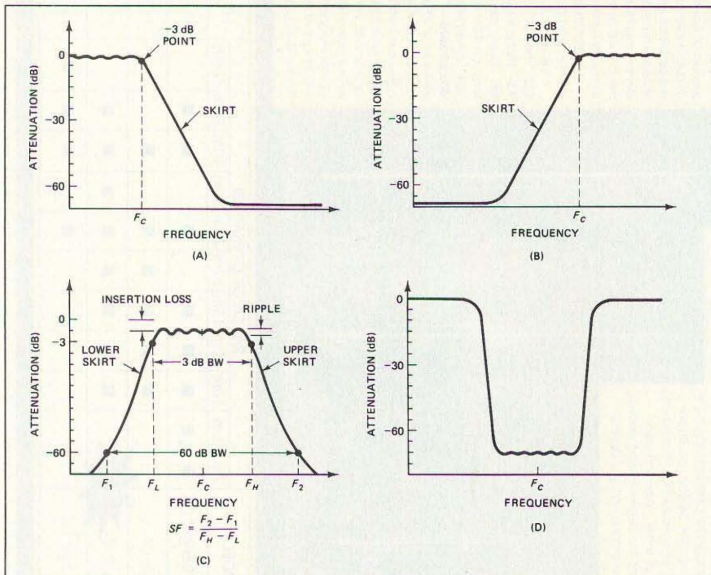
Figure 1. Filter frequency response characteristics.
