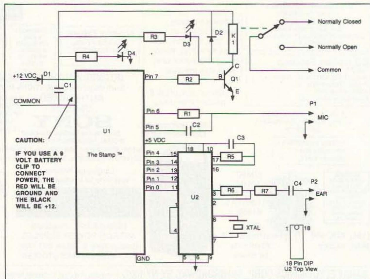
Figure 2. The Intelligent Relay Schematic.
