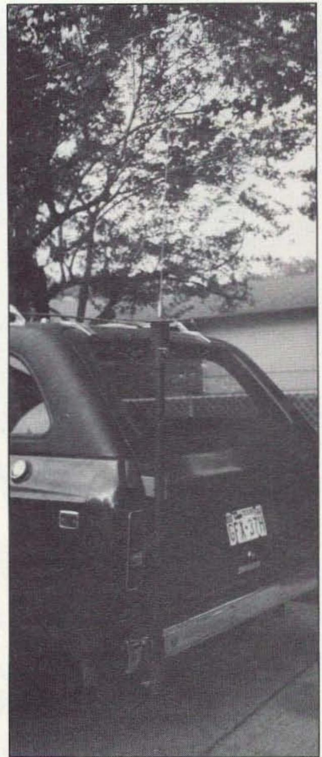
Photo C. 20 meter resonator mounted on the mobile mast.
