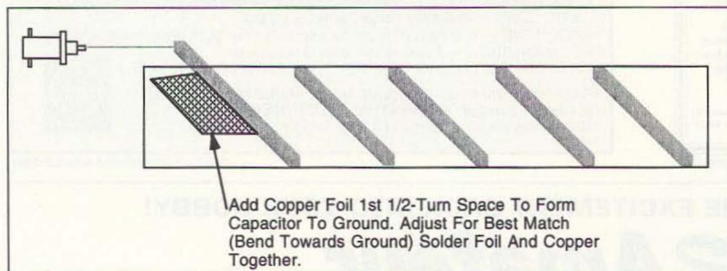
Figure 3. Matching capacitor and coax connection section for the helical antenna (matches 140-ohm helix to approximately 50 ohms for coax feed).
