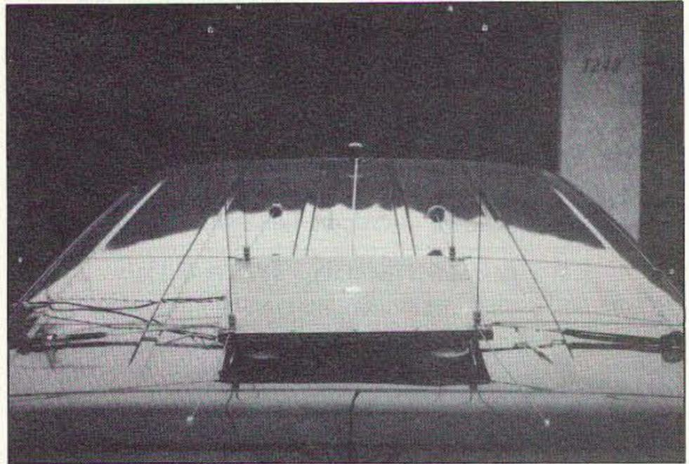
Photo A. The Roanoke Doppler antenna array has four quarter-wavelength whips on a 20 X 20 inch metal plate with eight radials to provide a ground plane under each whip.
