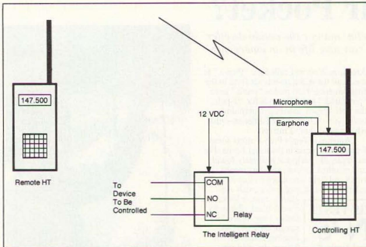
Figure 3. Block diagram of the Intelligent Relay.
