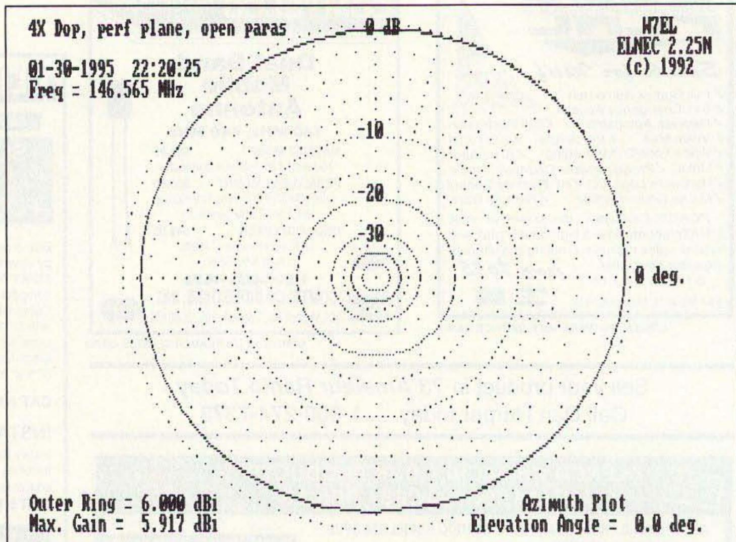
Figure 2. The undesirable lobe disappears and a nearly perfect circular pattern with no phase anomalies is achieved when the switched-off whips are open-circuited to minimize parasitic effects.
