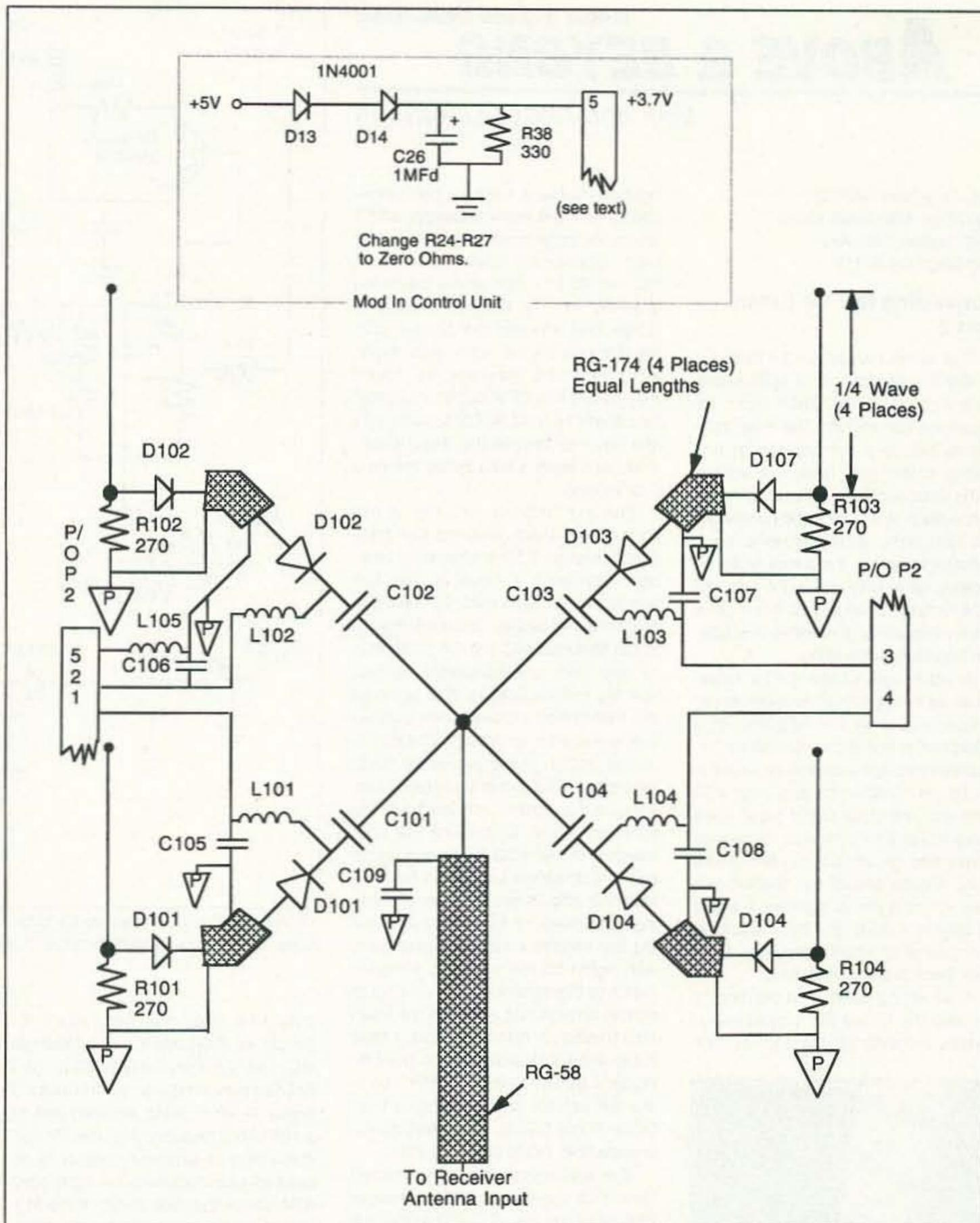
Figure 3. Schematic diagram of the new wideband switcher for the Roanoke Doppler. The P-in-a-triangle symbol denotes a connection to the ground plane sheet. Components values are for an array centered on 2 meters. All capacitors except C26 are 680 picofarads. See text for data on D101-D108 and L101-L105.
