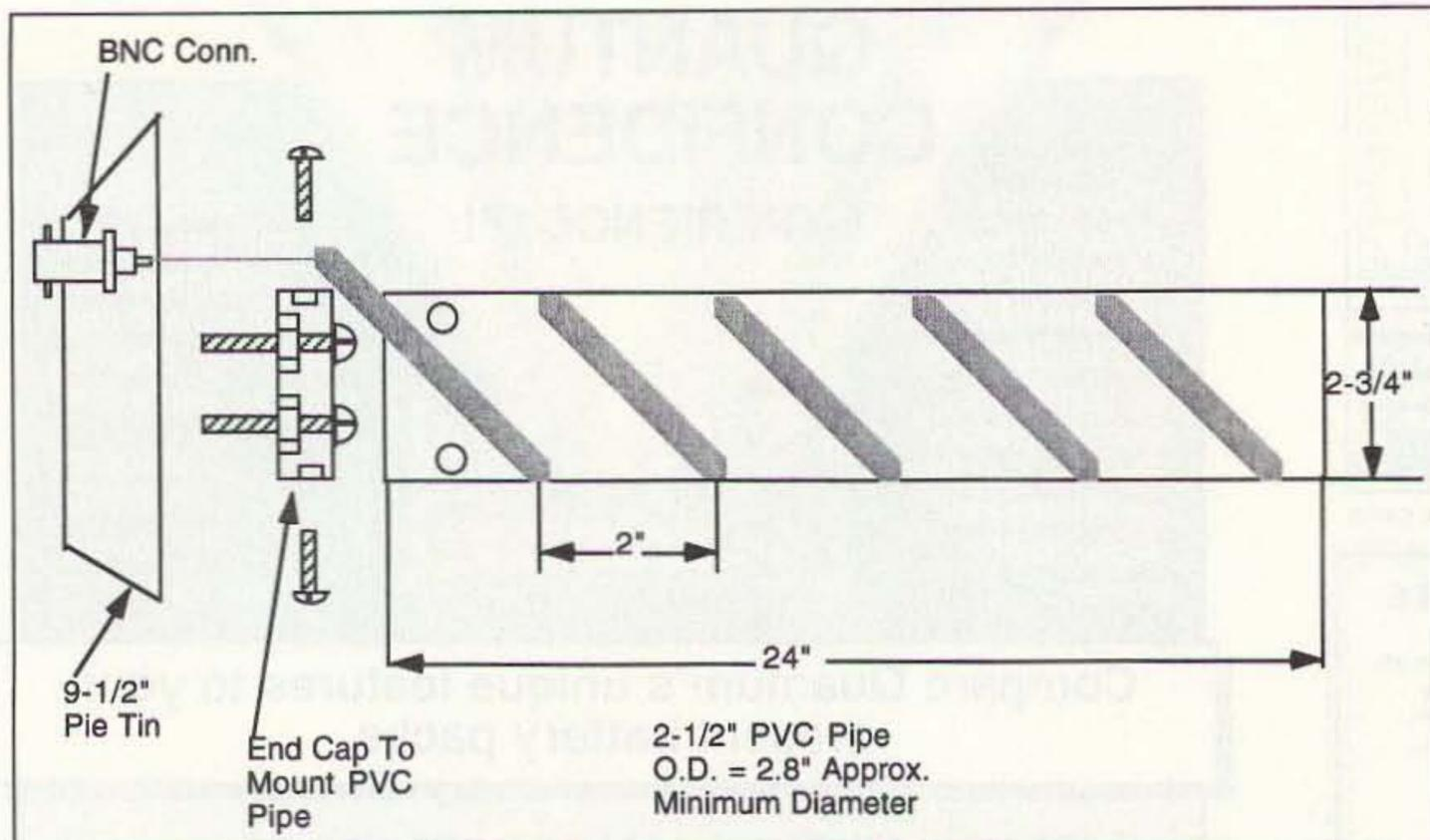
Figure 2. Construction details for the helical antenna for 1240 MHz. Wind a helix right-hand spiral spaced 2" between turns. Use copper foil tape 3/8" wide. Mark off 2" lines to aid in positioning tape on the PVC pipe.
