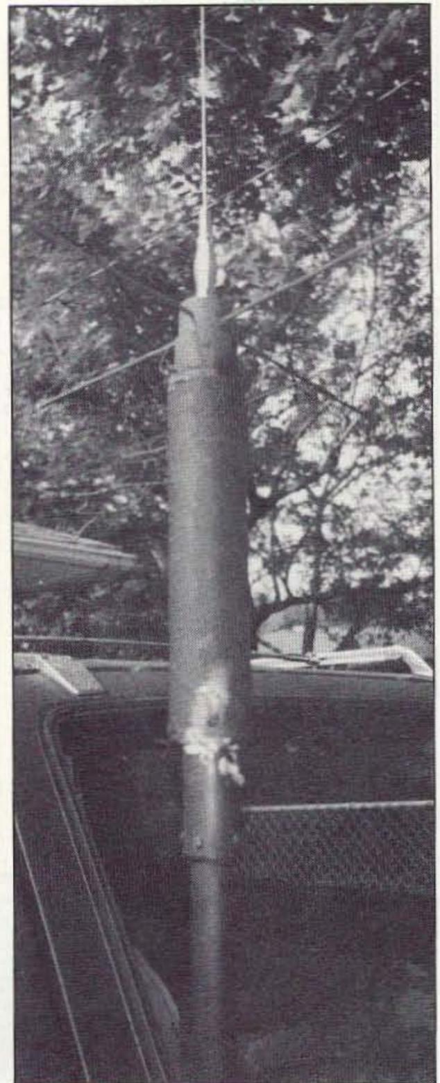
Photo B. Close-up of the 75 meter resonator.
