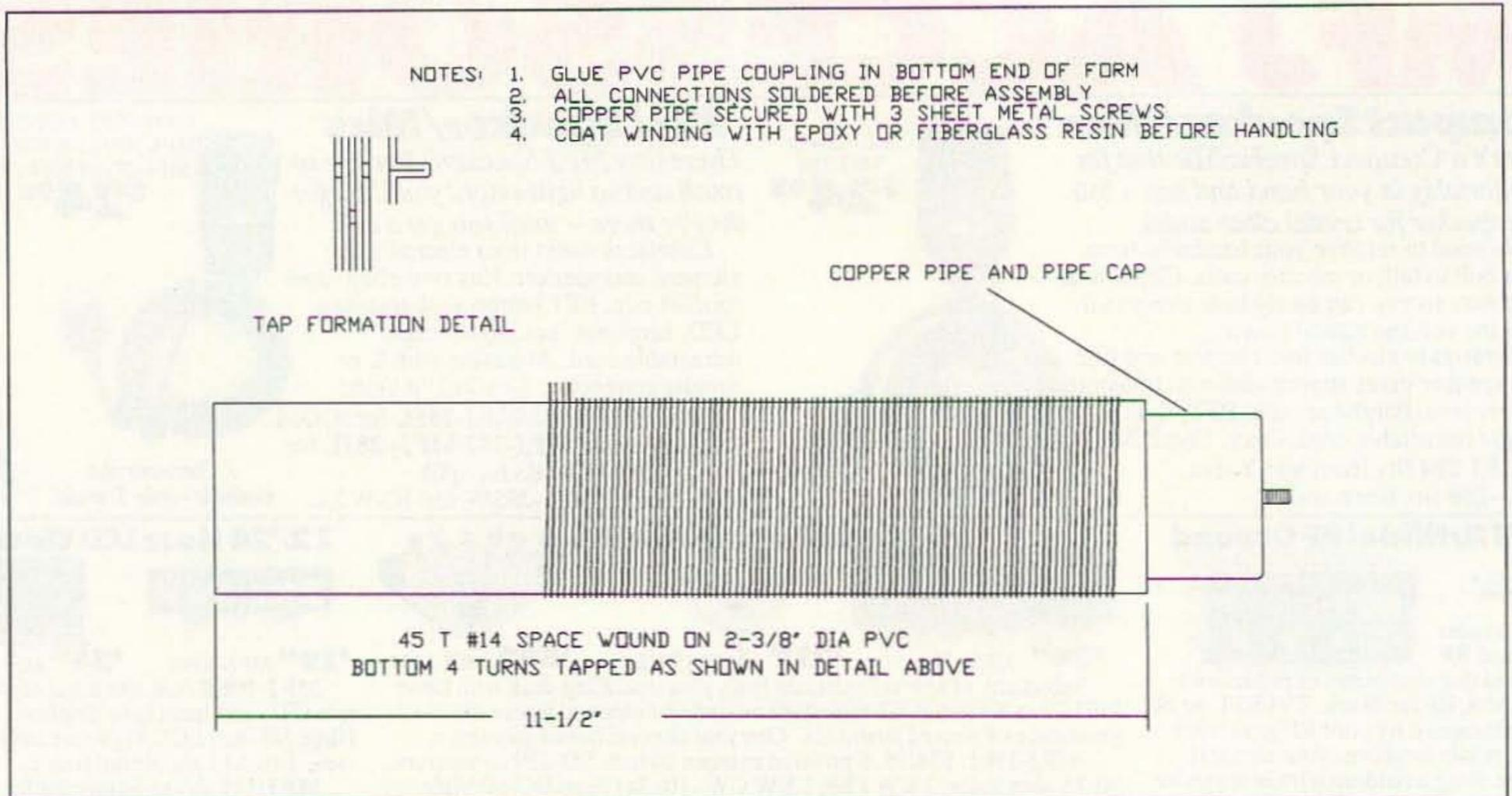
Figure 3. 40 meter resonator.
