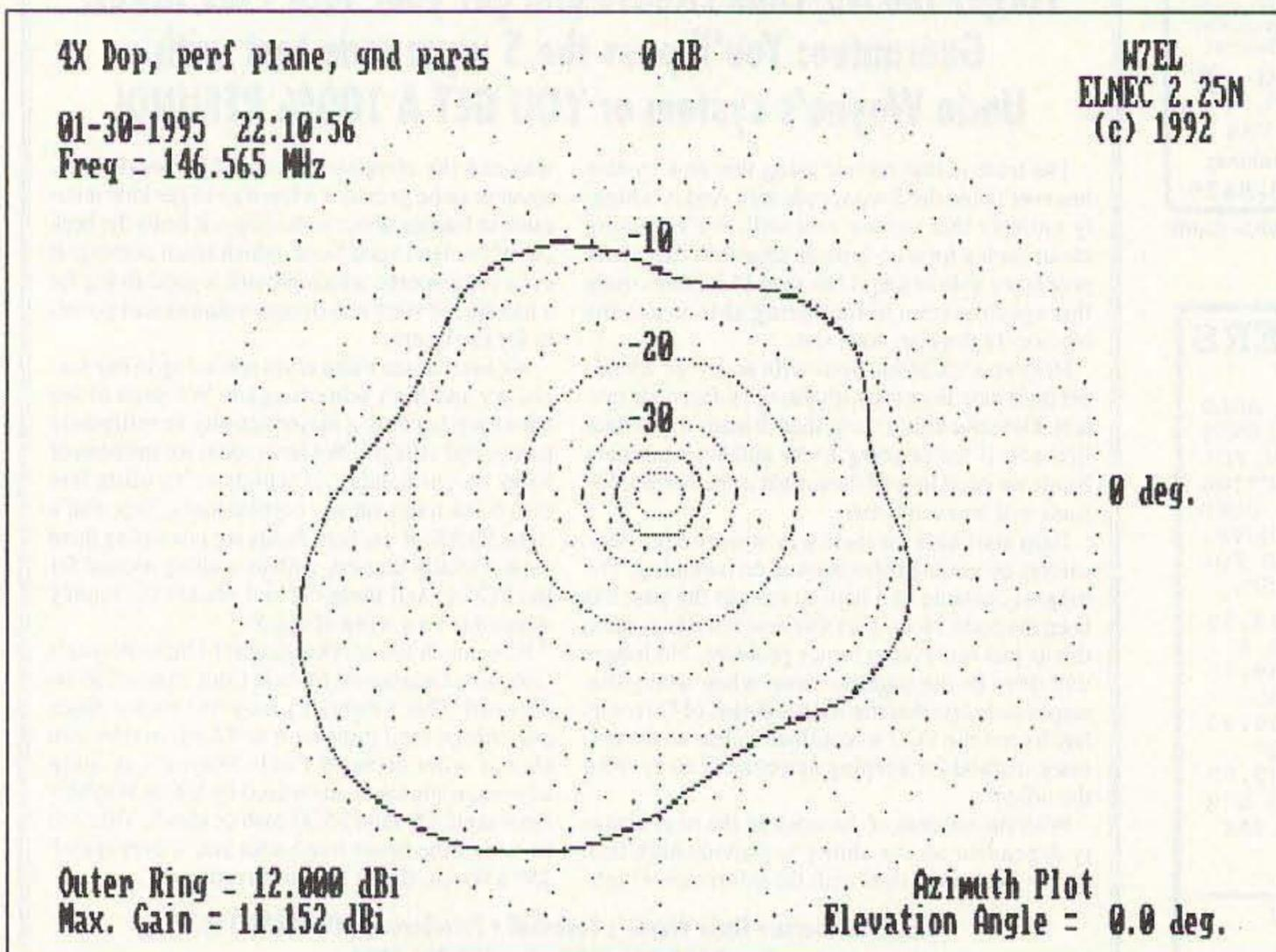
Figure 1. ELNEC azimuth pattern plot of a four-whip doppler array with three whips grounded and one connected to the feed-line. The large lobe is in the direction of the active whip, which is in the lower left of the array.
