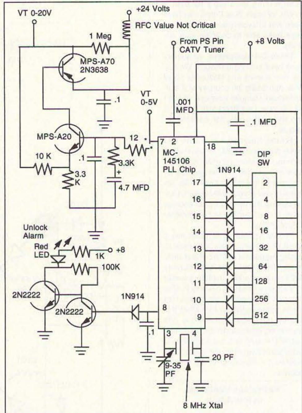
Figure 1. Schematic diagram for Motorola MC-145106 synthesizer control. Refer to the text for an explanation of the "\*" on pin 7.
