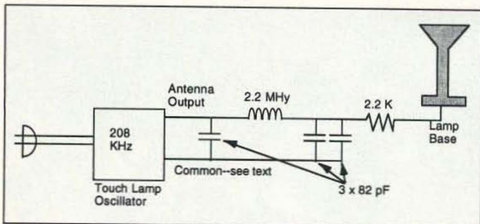
Figure 2. A solution for a 208 kHz touch lamp (see text).
