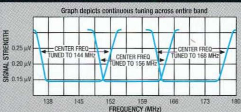
**3-Stage Advance Track Tuning (ATT)** – The exclusive 3-Stage Advance Track tuning front end automatically adjusts band width sensitivity across the entire receiver range, while maintaining selectivity specifications. ATT significantly reduces interference from inter-modulation and front end overload.
