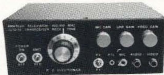
Snow free line of sight DX is 90 miles - assuming 14 dBd antennas at both ends. 10 Watts in this one box may be all you need for local simplex or repeater ATV. Use any home TV camera or camcorder by plugging the composite video and audio into the front phono jacks. Add 70cm antenna, coax, 13.8 Vdc @ 3 Amps, TV set and you're on the air - it's that easy!
