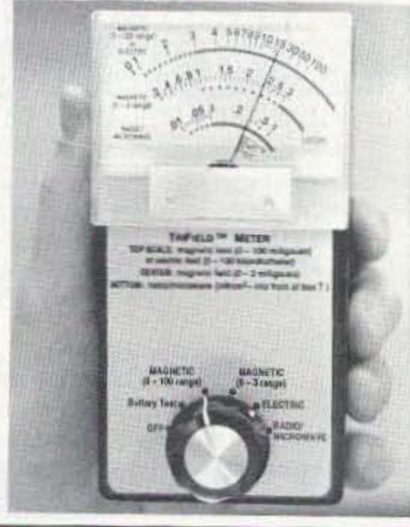
Electric and magnetic settings are omnidirectional, measuring full magnitude of fields without the need to reorient the meter. Price of \$145 includes delivery and one-year warranty.
