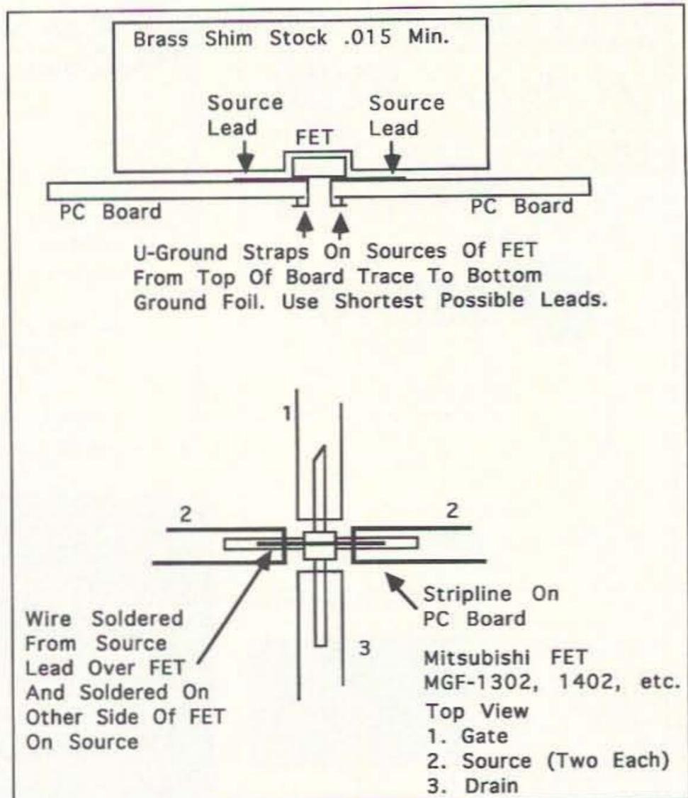
Figure 3. FET shielding details.
