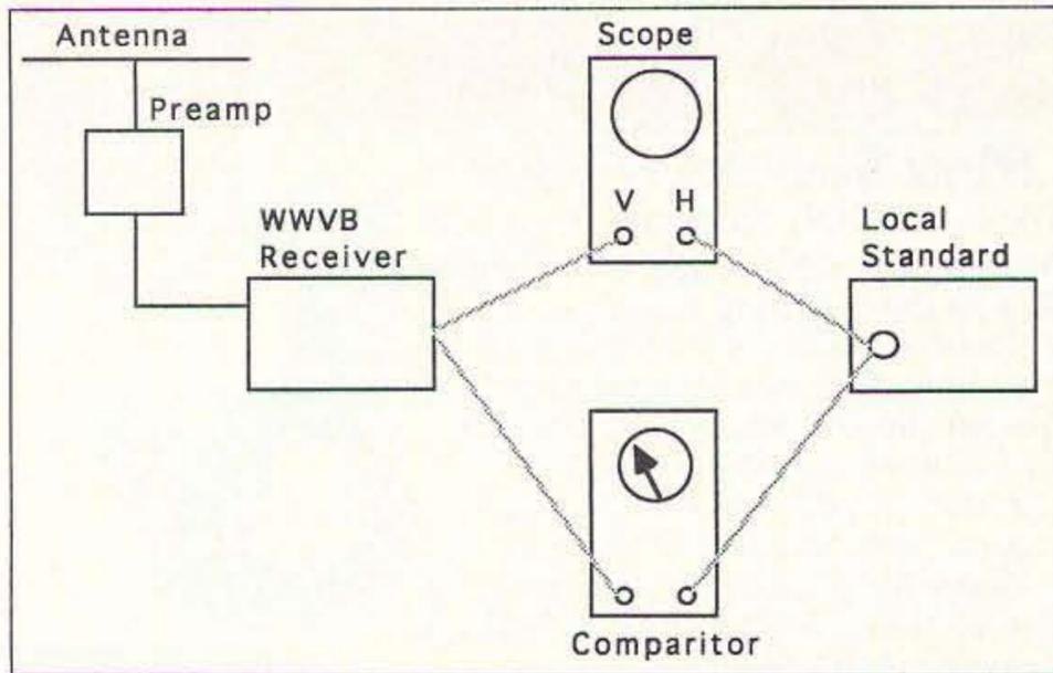
Figure 1. Block diagram of the WWVB receiver/comparator.
