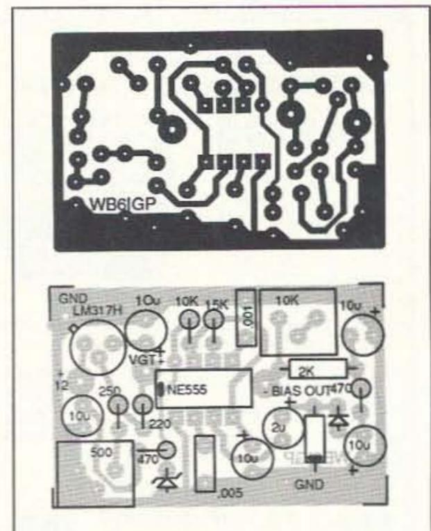
Figure 4. PC board layout and parts placement diagram. Drilled and etched PC boards are available for \$3.50 plus \$1.50 S&H from FAR Circuits, 18N640 Field Ct., Dundee IL 60118.
