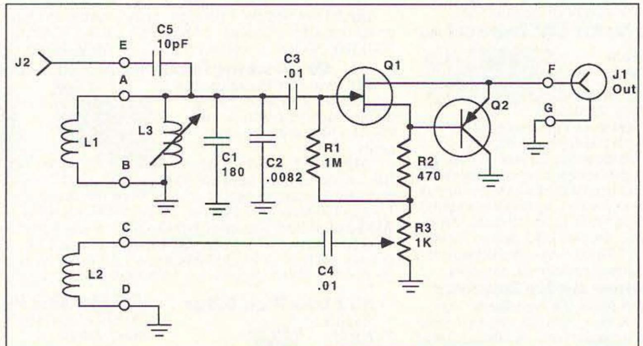
Figure 2. The antenna/preamp circuit.
