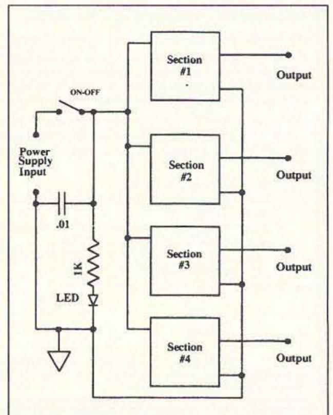
Figure 2. Quad Charger system schematic.
