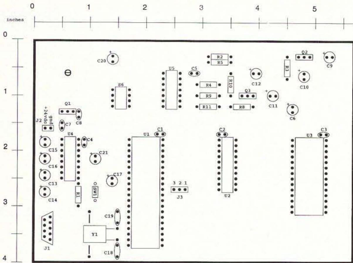
Figure 4. Programmer parts placement @ 70%.
