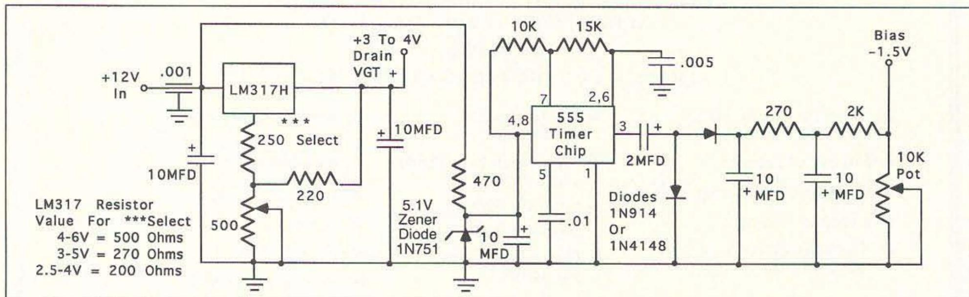
Figure 1. Schematic for bias power supply. Adjust positive voltage with selection of LM317 resistor as indicated by \*\*\*. Note: 470 ohm resistor at the input of the 555 chip (pins 4 & 8) is mounted on the PC board to +12 volts. This maintains a stiff -1.5 volts bias output at minimum pot output from the negative bias supply.
