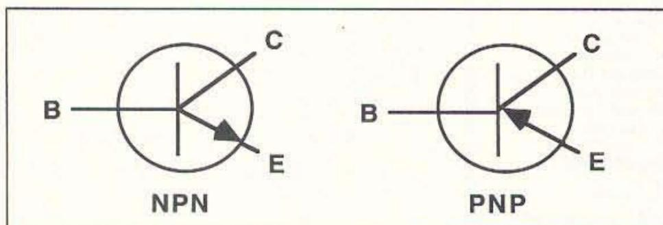
Figure 1. Schematic symbols for NPN and PNP transistors. Note the arrow's direction for each.
