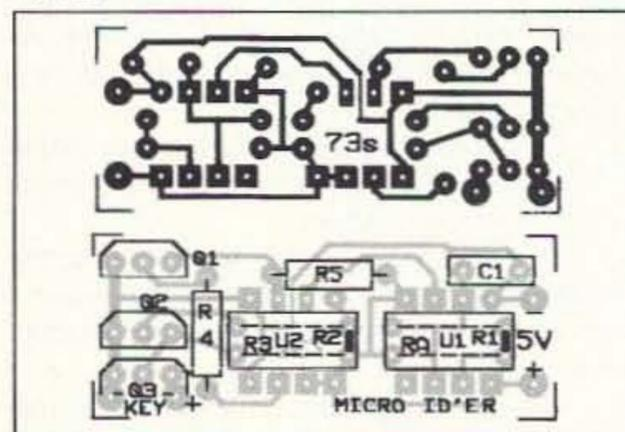
Figure 2. Parts placement outline and circuit board pattern.
