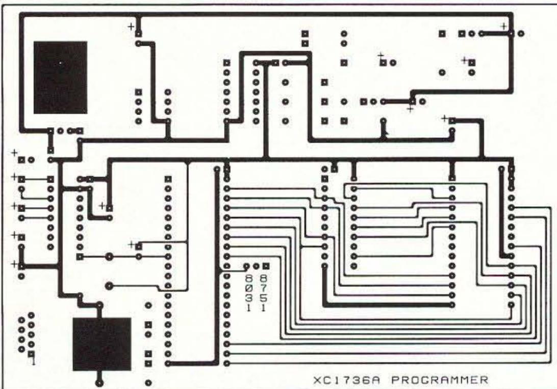
Figure 6. Programmer component side circuit pattern @ 70%.
