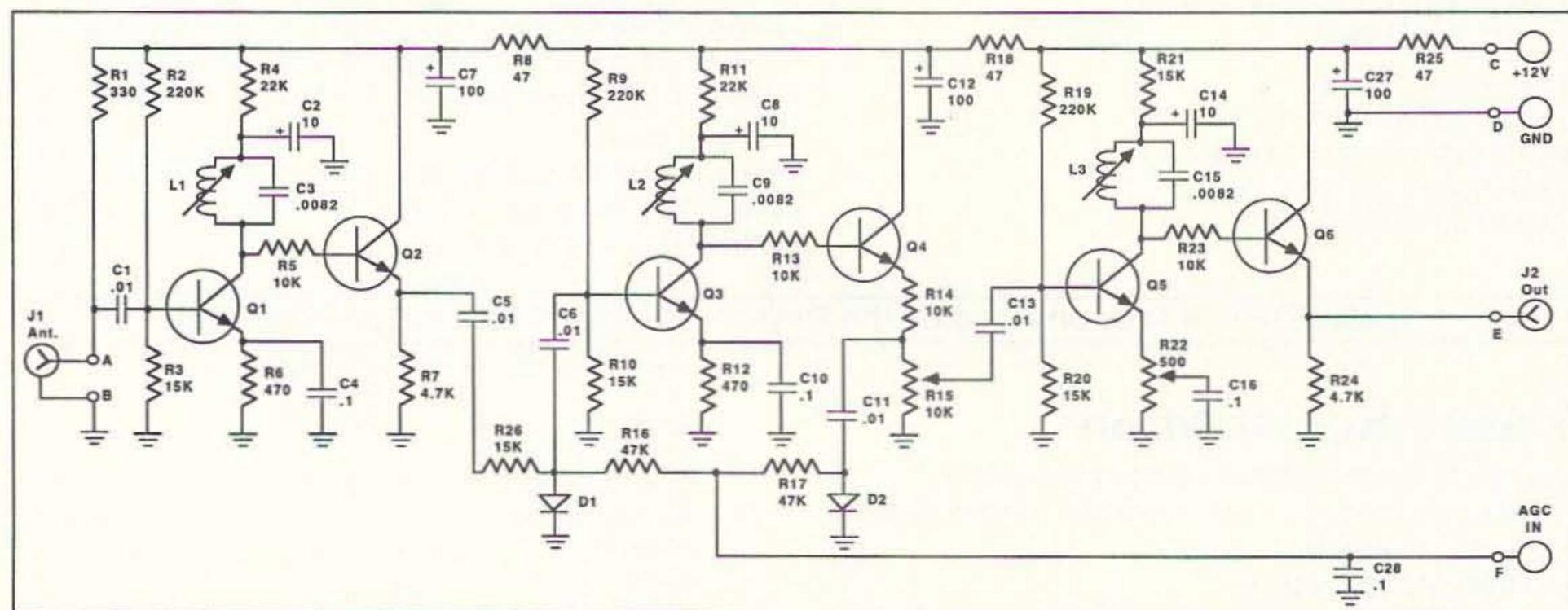
Figure 4. RF amplifier portion of the receiver.
