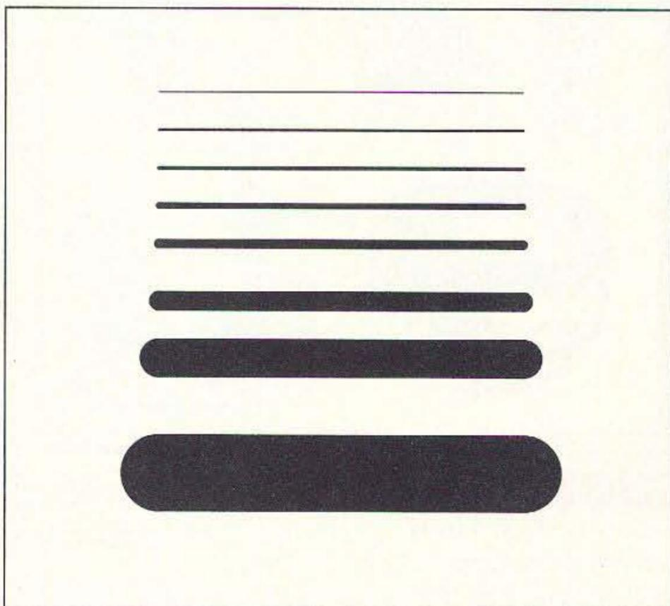
Figure 1. Track widths available on EASY-PC.
