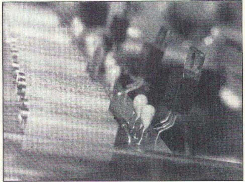
Photo C. LM317 mounting, showing off-set arrangement.
