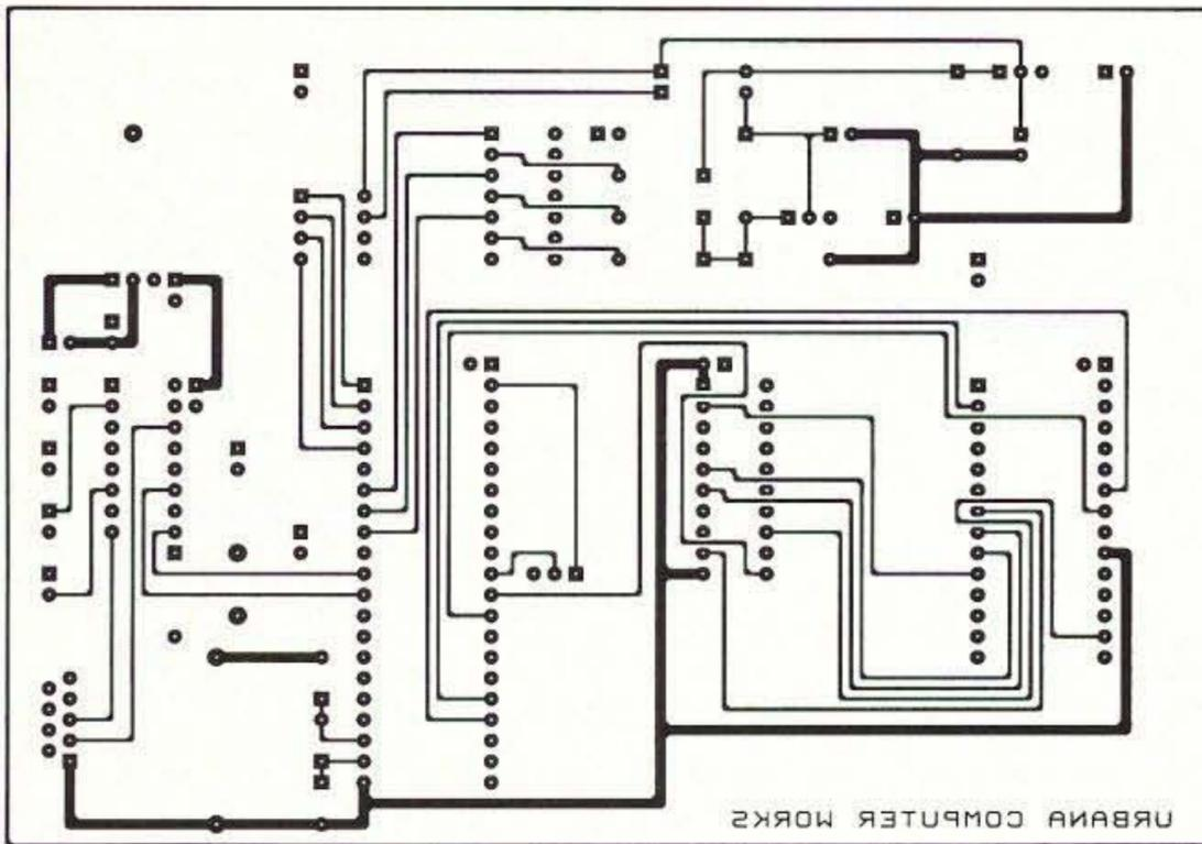
Figure 5. Programmer solder side circuit pattern @ 70%.
