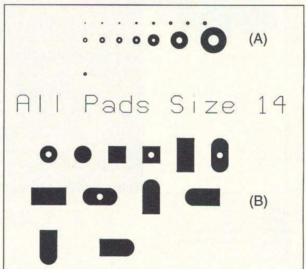
Figure 2. A) Pad widths available on EASY-PC; B) Pad variants available.
