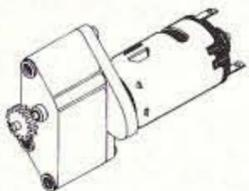
Excellent motor for displays, robotics and other mechanical applications. No load ratings: 48 RPM @ 6 Vdc 92 RPM @ 12 Vdc. Motor dimensions: 1.08" diameter X 1.4" long. Gearhead dimensions: 1.34" X 0.93". Final drive shaft is 1/8" diameter X 0.35" long. A 0.55" diameter gear is press-fit onto the shaft.
