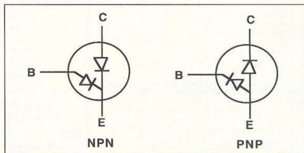
Figure 2. Theoretical NPN and PNP transistors, each composed of two diodes.
