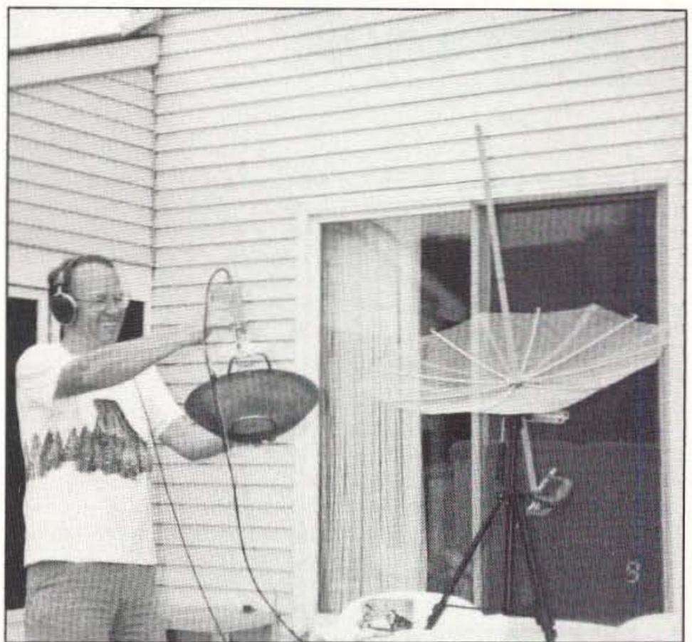
Photo E. Ed Krome KA9LNV at home with the three-foot dish for SSB reception using OSCAR-13 and his 15-inch "WOK" reflector for successful CW reception via 2.4 GHz, Mode "S." (KA9LNV photo.)
