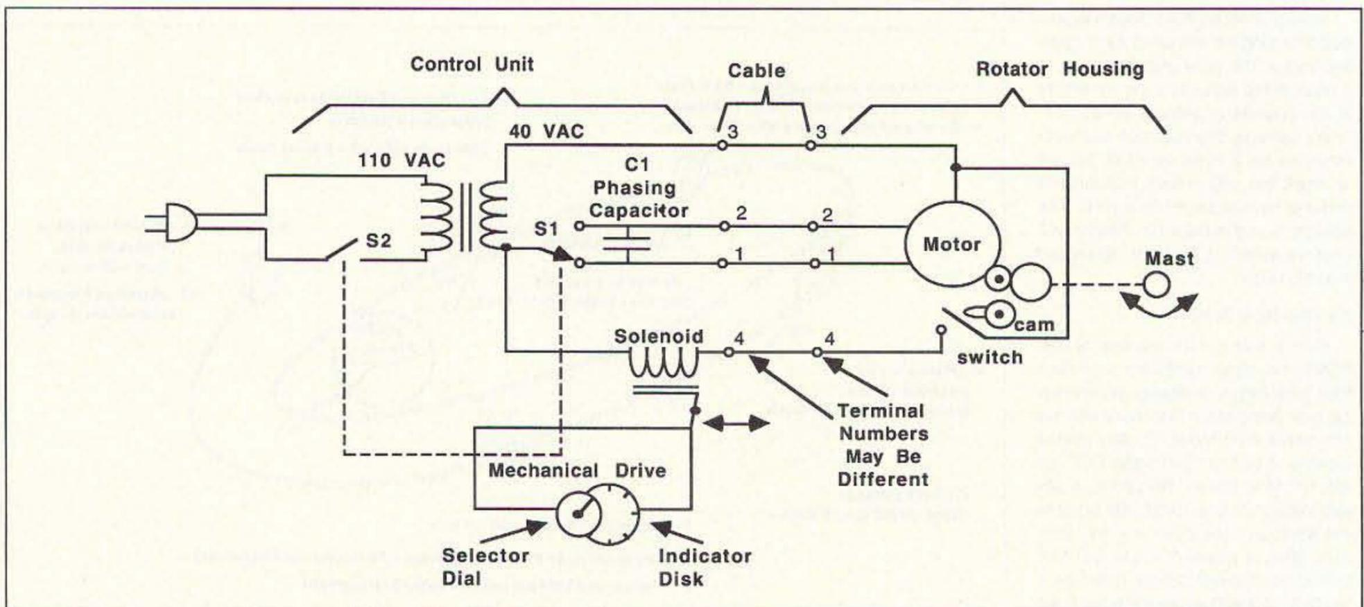
Figure 1. Typical rotator and control box.
