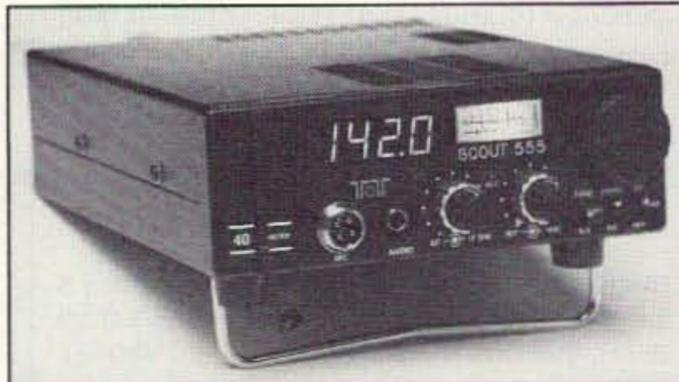
kHz. A built-in microprocessor keeps the VFO virtually drift-free and handles the built-in iambic keyer. For more information contact *TEN-TEC, Inc., P.O. Box 8010, Sevierville TN 37864; (615) 453-7172, FAX (615) 428-4483.* Or circle Reader Service No. 203.
