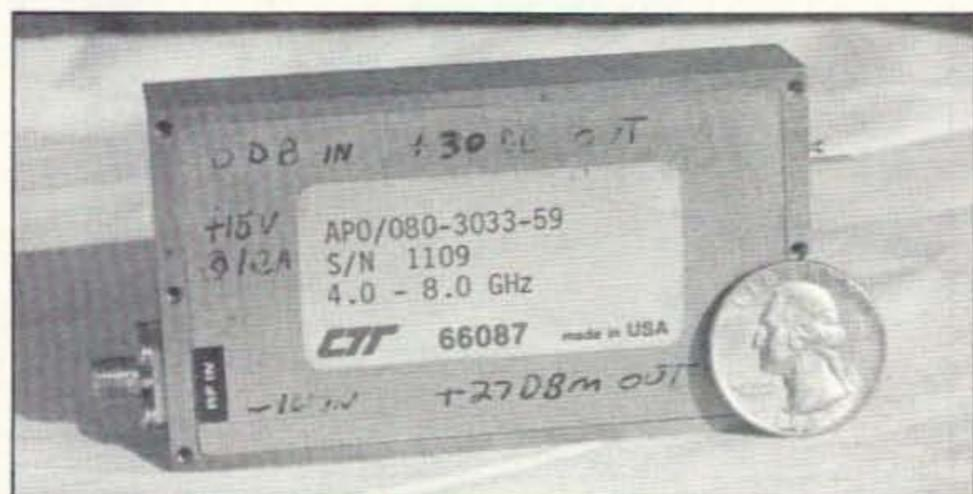
Photo C. A compact CIT 4.0 to 8.0 GHz, 1 watt amplifier.
