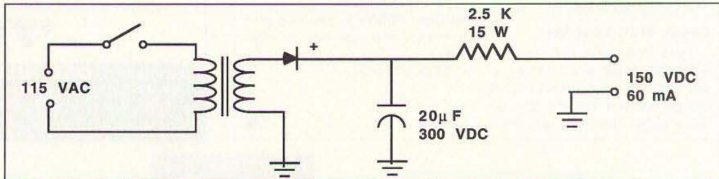
Figure 3: Basic RTTY Loop supply circuit.
