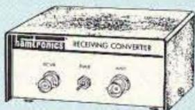
Low noise converters to receive vhf and uhf bands on a 10M receiver.
