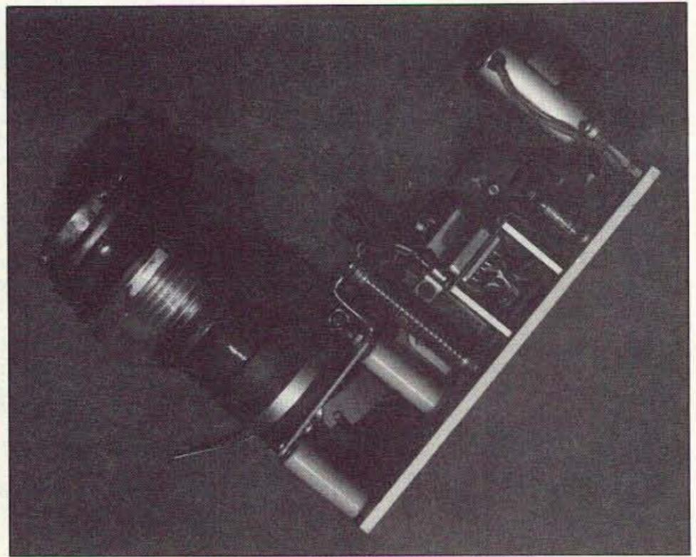
Photo D. Vacuum variable (10-1000 pF) capacitor.
