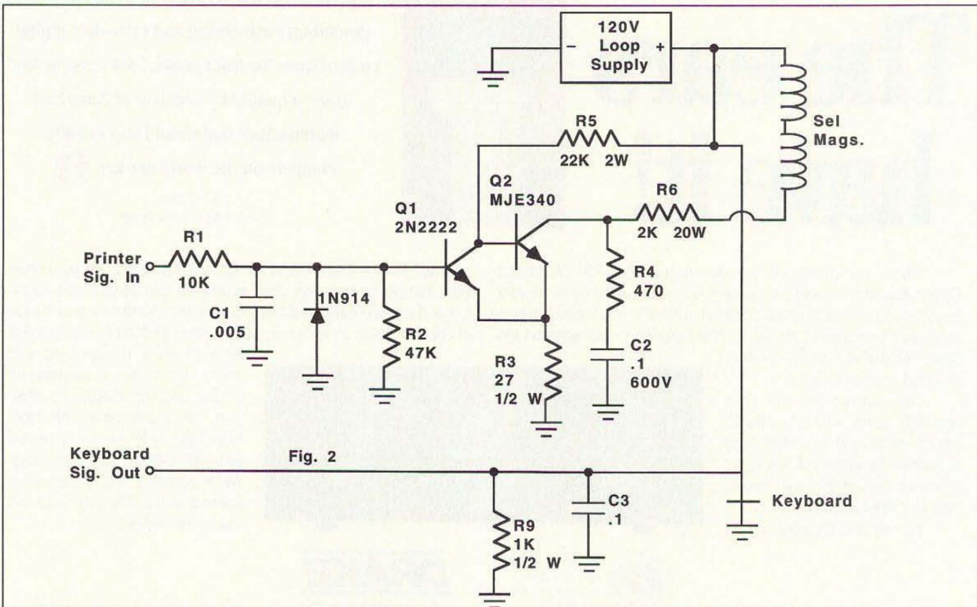
Figure 1: Selector Magnet Driver Circuit.
