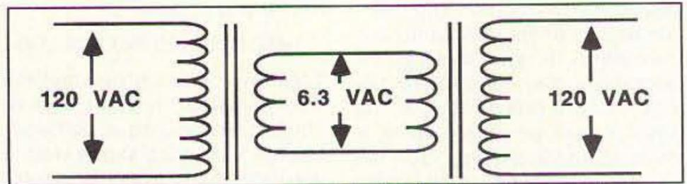
Figure 2: Line Isolation with back-to-back transformers.
