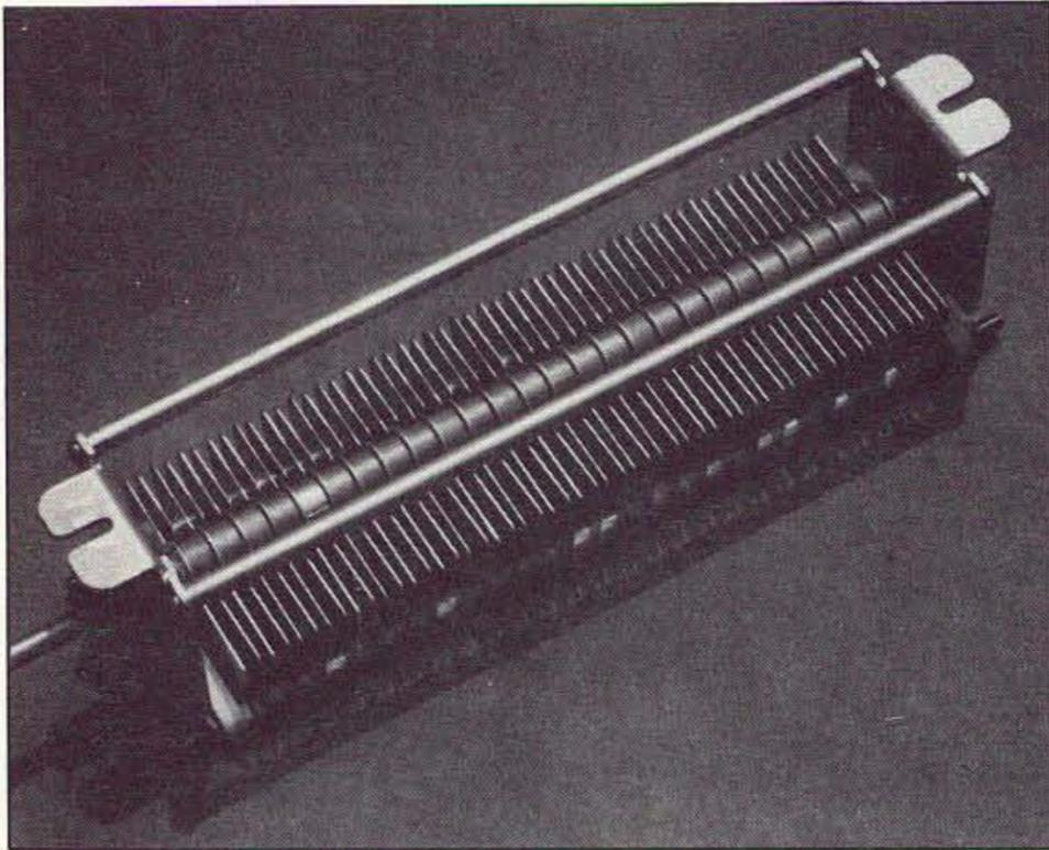
Photo C. Transmitting air variable capacitor.
