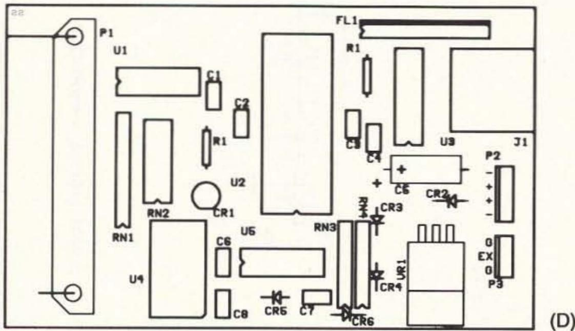
C) PC drilling template; D) parts placement diagram.
