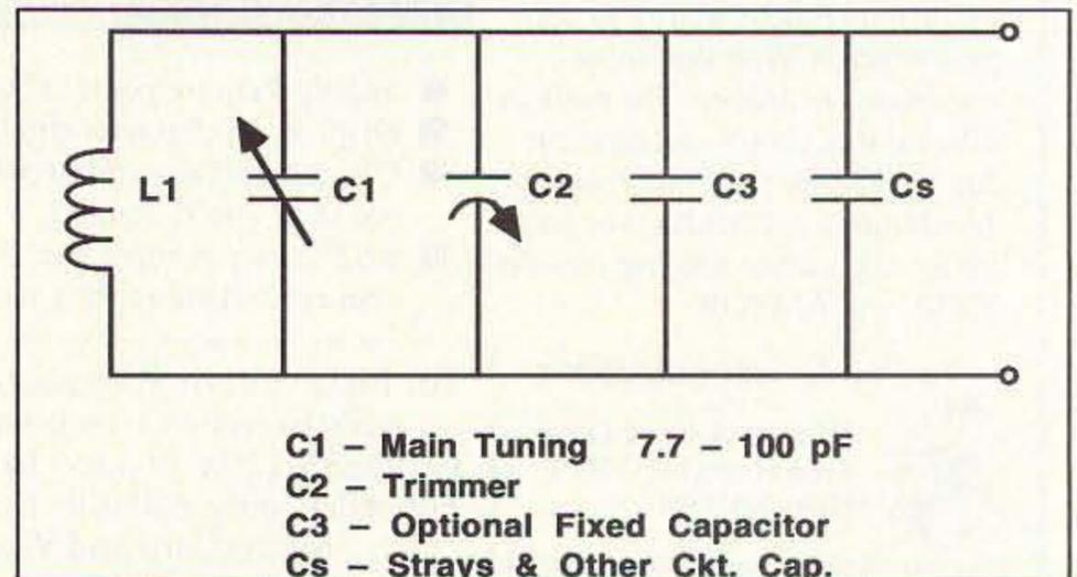
Figure 3. L-C resonant tank circuit for example calculations.
