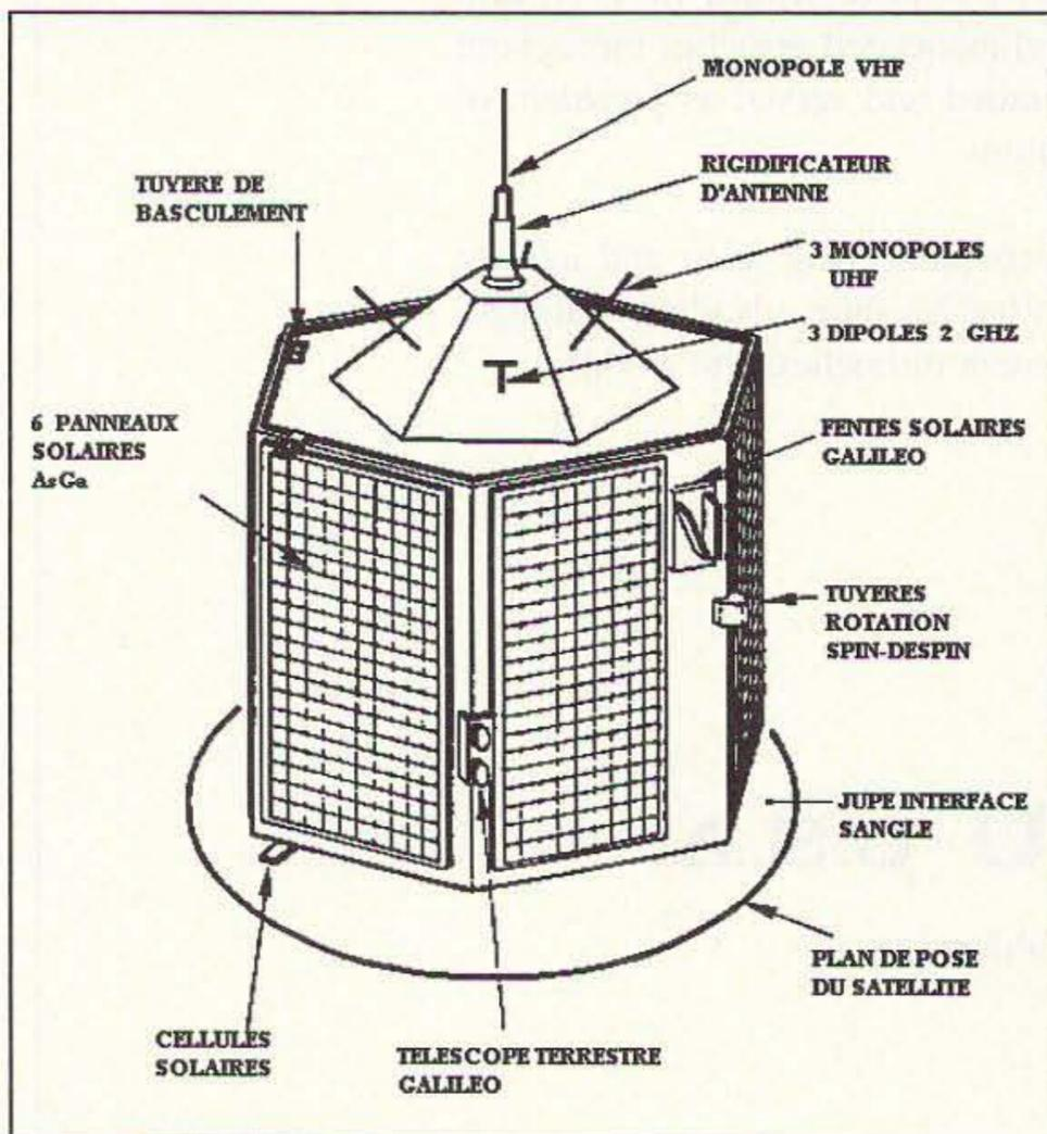
Figure 1. External ARSENE configuration.
