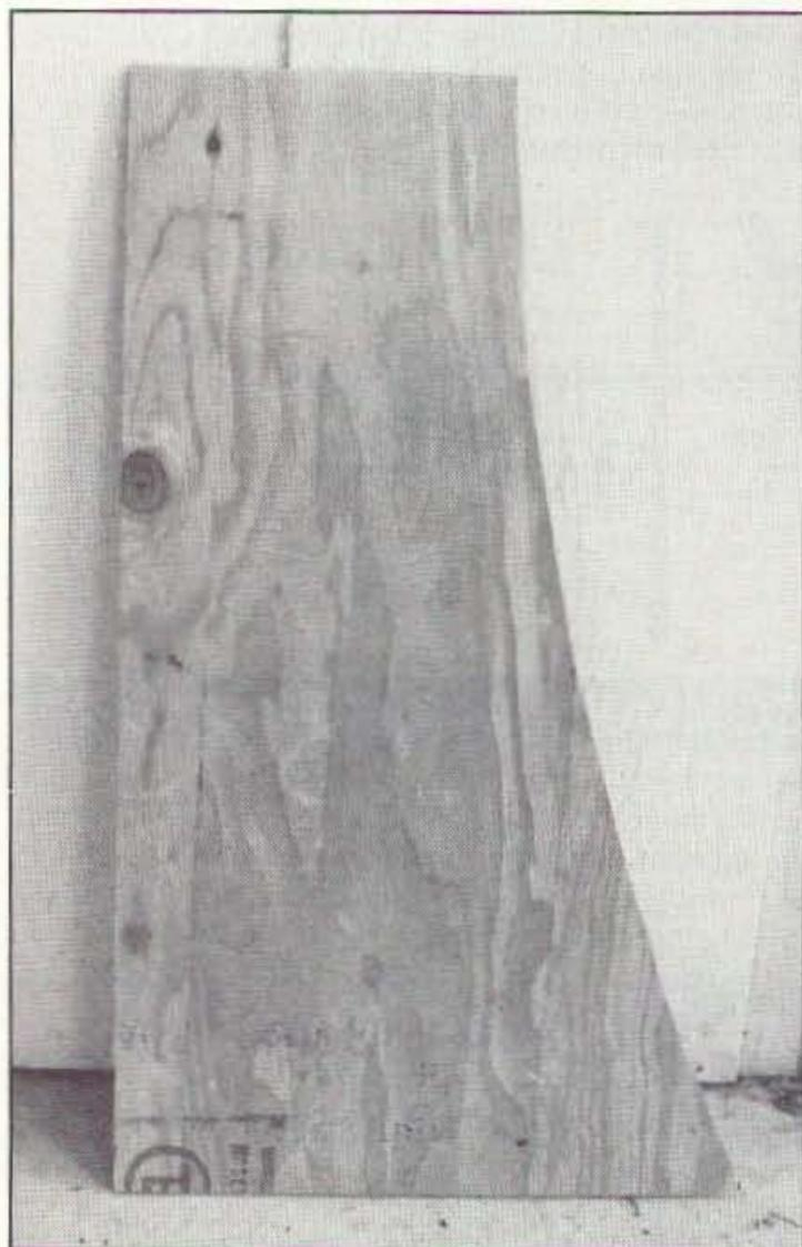
Photo A. Plywood bending fixture.
