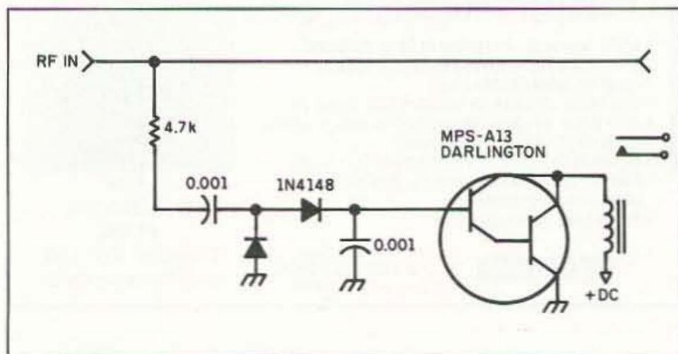
Figure 1. Basic RF switching circuit.
