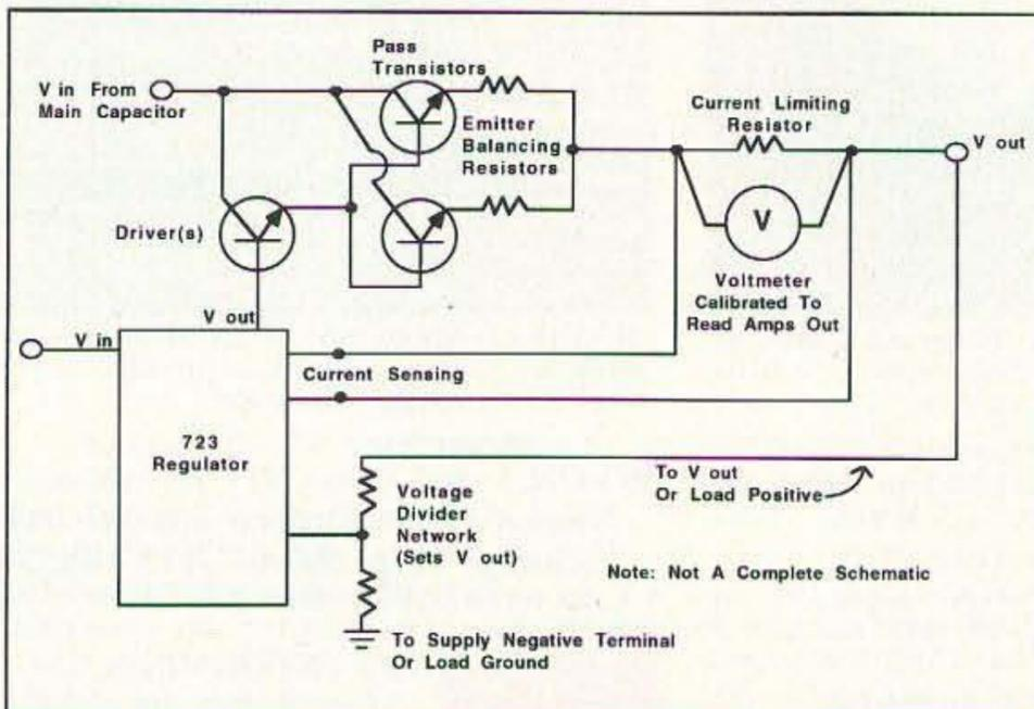
Figure 1. 723 circuit components.
