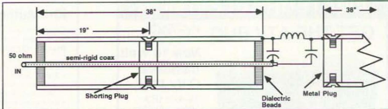
Figure 5. Basic construction.
