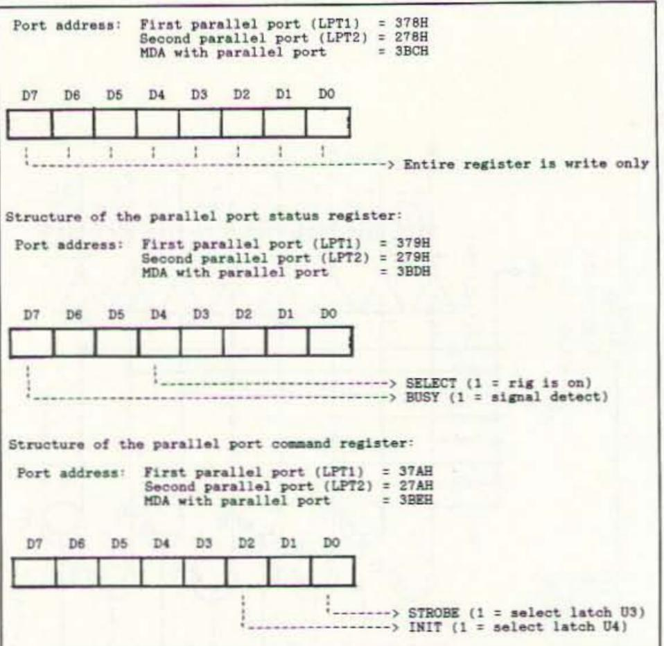
Figure 3. PC parallel port layout.
