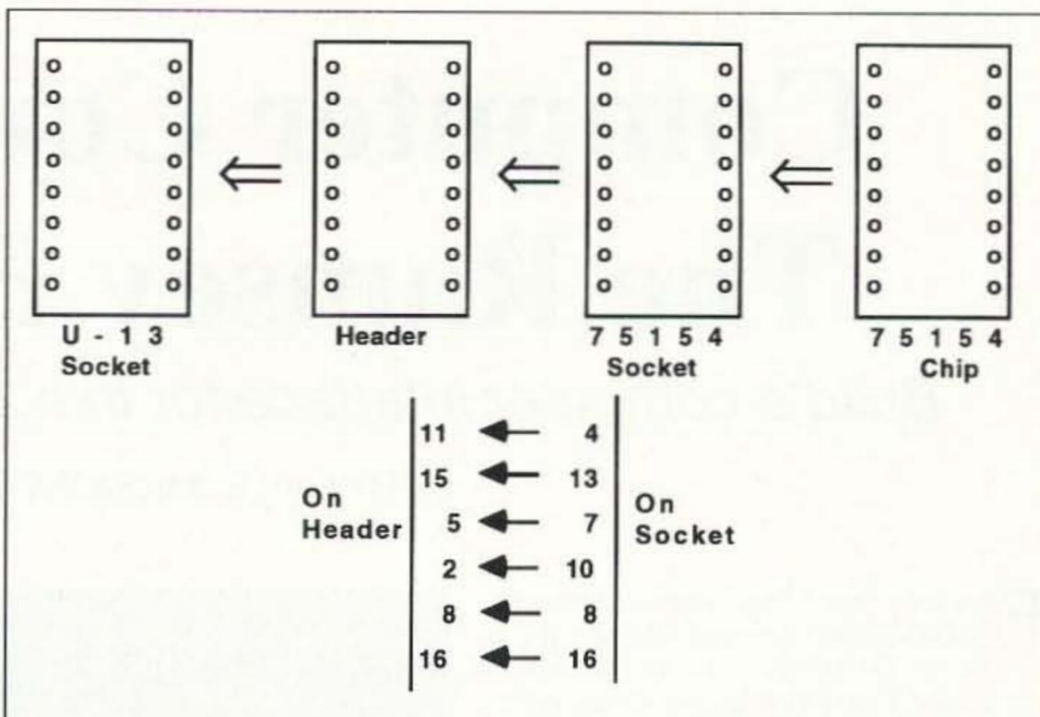
Figure 1. Interface wiring for the CP-1.
