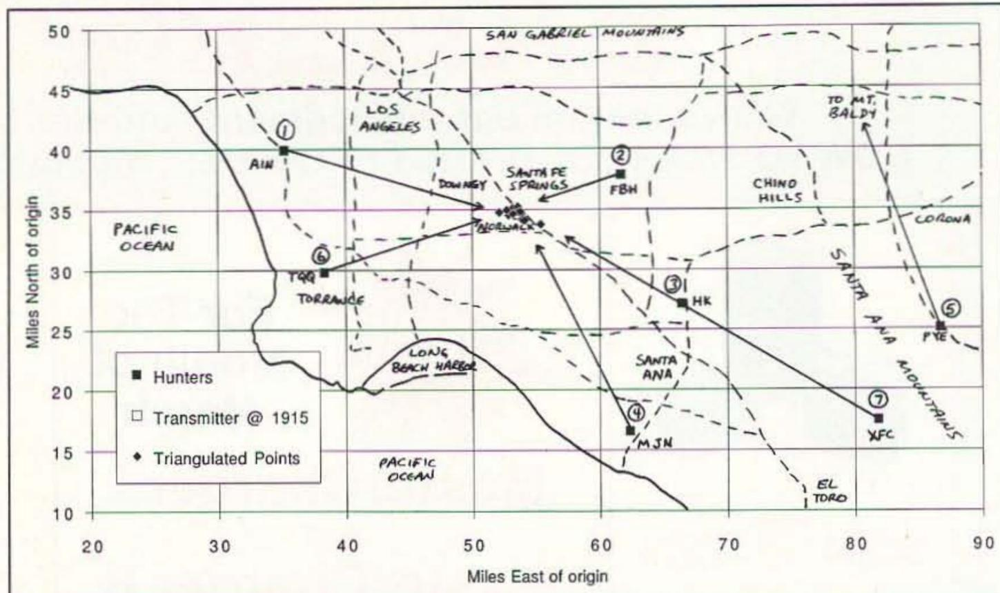
Figure 2. After triangulations are complete, WB3JZV's program produces an Excel chart of the hunters and their fixes on the fox. In this case, the final position estimate is almost buried under them. I drew in the coastline (solid) and major freeways (dashed) for reference.
