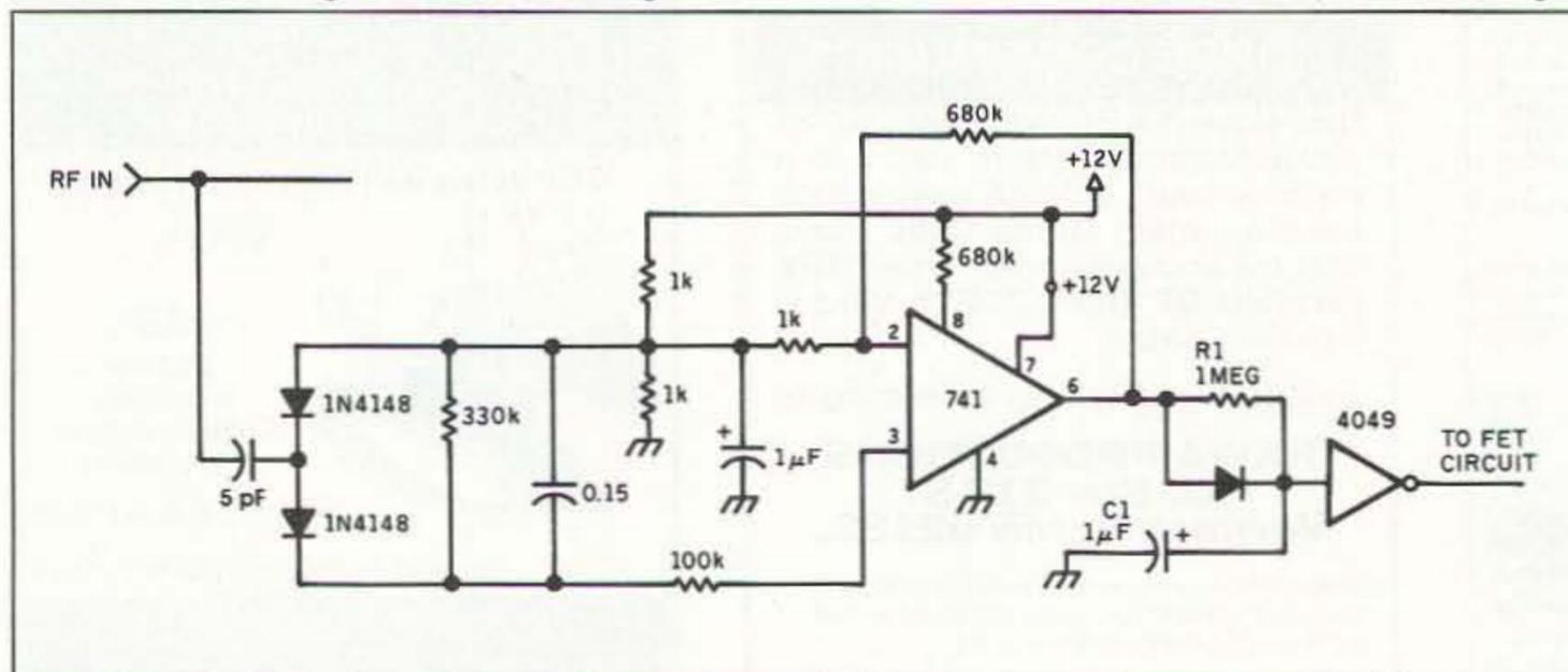
Figure 2. Sensitive RF circuit for SSB.
