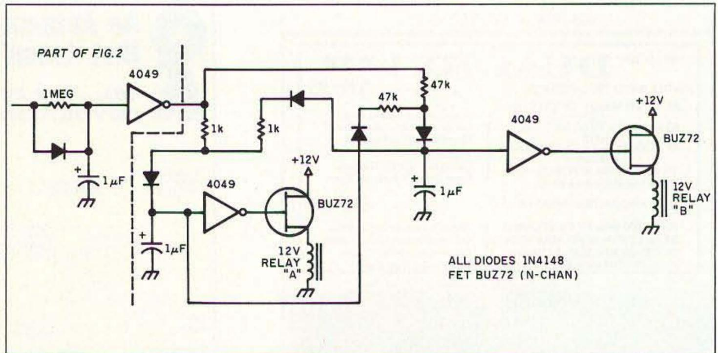
Figure 3. Timed FET switching circuit.
