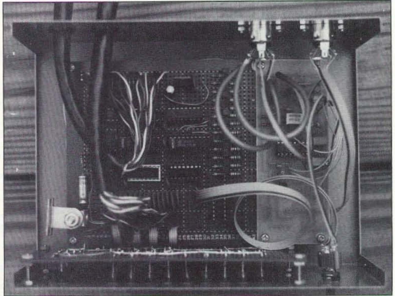
*Photo A. Parts placement of the interface on a Radio Shack 276-147 board inside an RS 270-274 cabinet. The LEDs are installed on another RS 276-147 (cut in half) and mounted inside the front panel. The circuit on the right side of the board is a packet modem interface, described in "Poor Man's Packet," 73 Amateur Radio Today, August 1991.*
