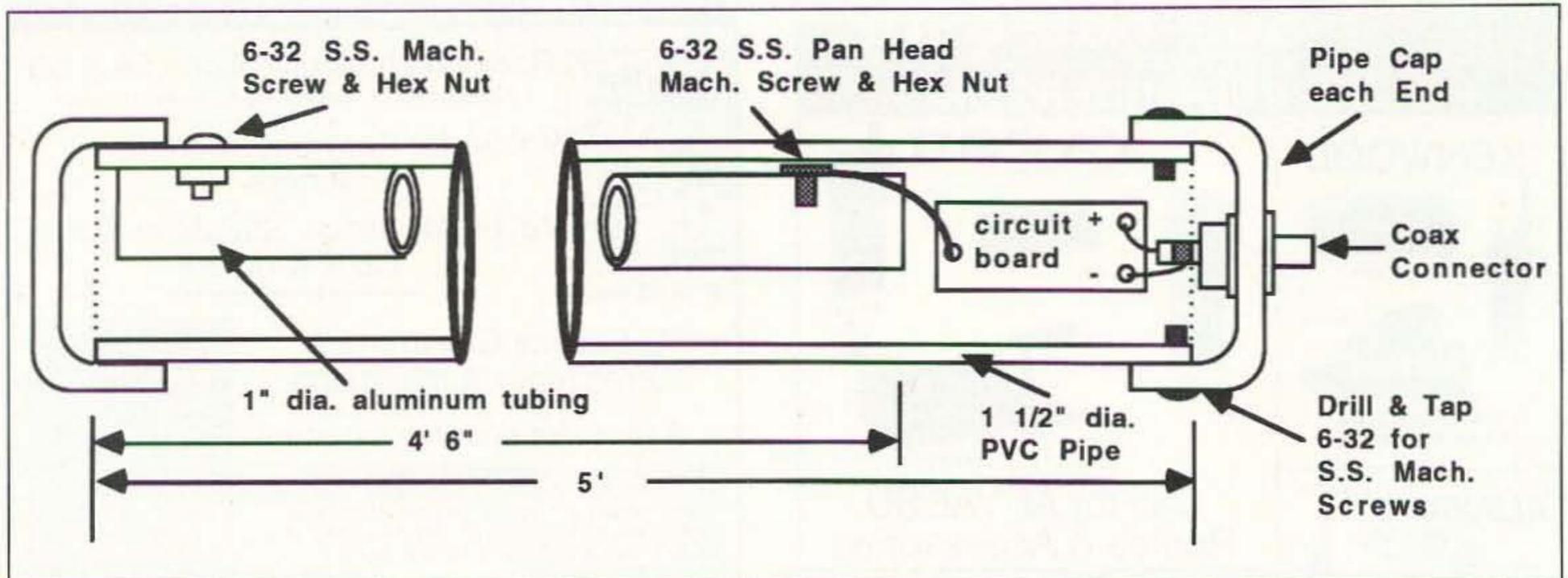
Figure 3. Active antenna assembly.
