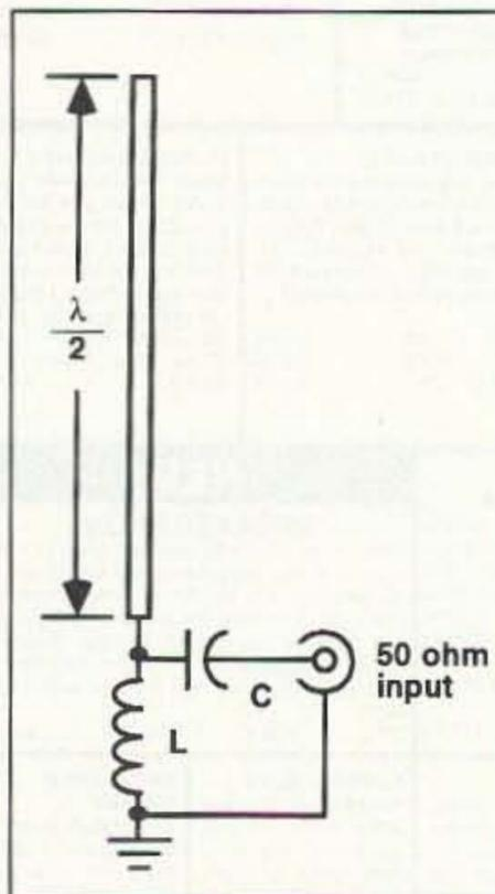
Figure 1. The ground-independent vertical half wave.
