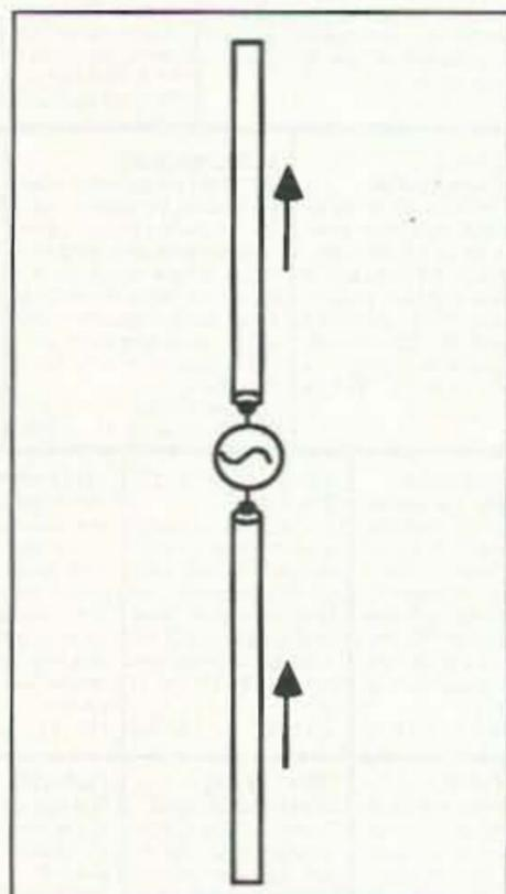
Figure 2. Two half waves in phase.
