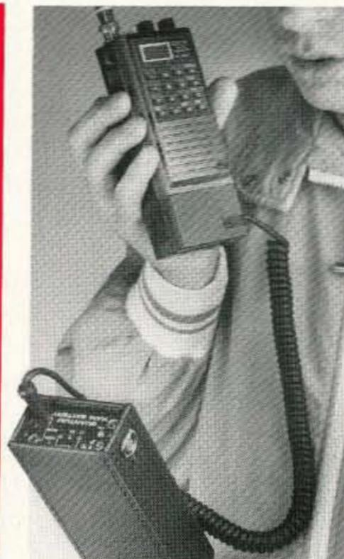
The Quantum Ham Battery™ may be the last rechargeable battery you'll purchase. Its 12 volt 2.1 amp hour capacity packs up to six times the power of H-T nicad packs.
