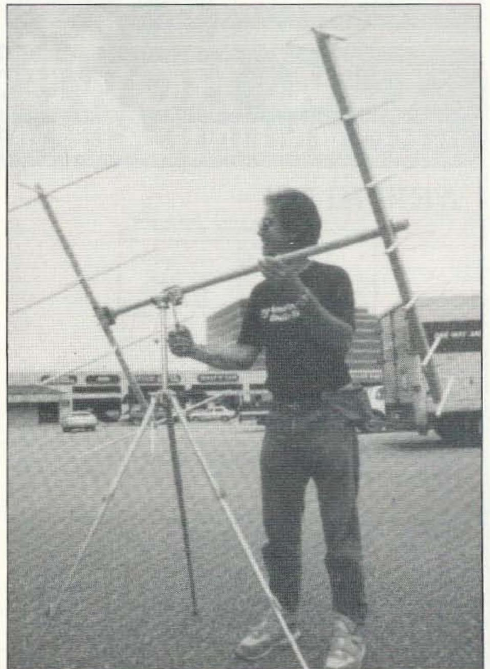
Photo B. Allan N5LKJ checks the array balance and camera tripod controls for the Lightning Bolt OSCAR antenna system. (Photo by WB5RTT.)
