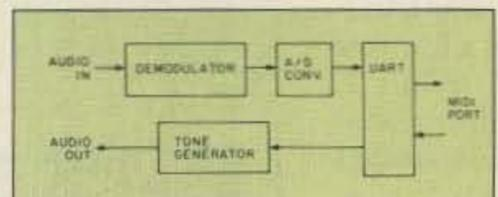
Figure 9. Block diagram of high performance interface.
