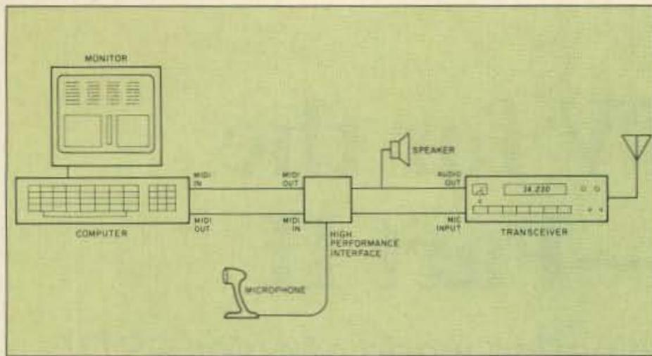
Figure 8. Station layout using the high-performance interface.
