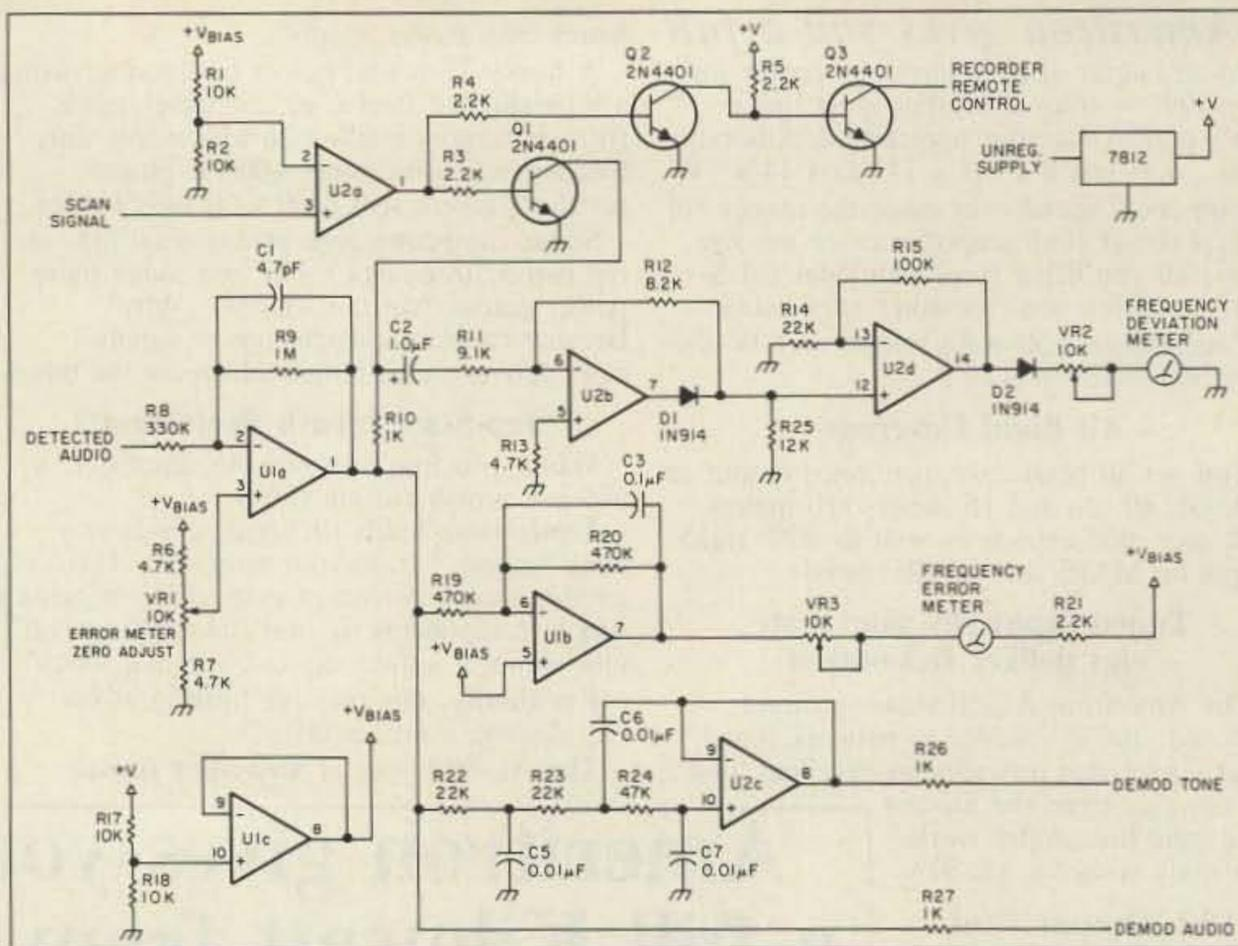
Figure 1. Schematic of the Poor Man's Service Monitor.
