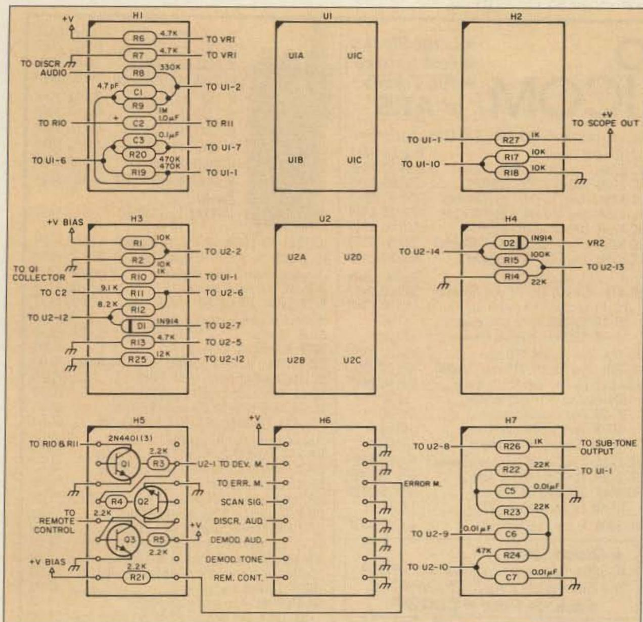
Figure 2. Parts placement for the Monitor.
