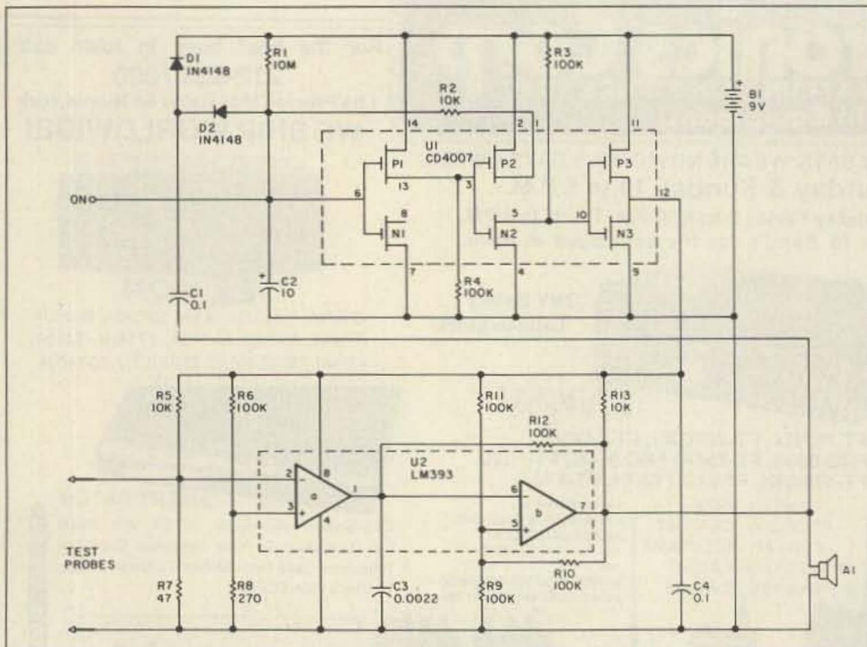
Figure 1. Continuity beeper schematic.
