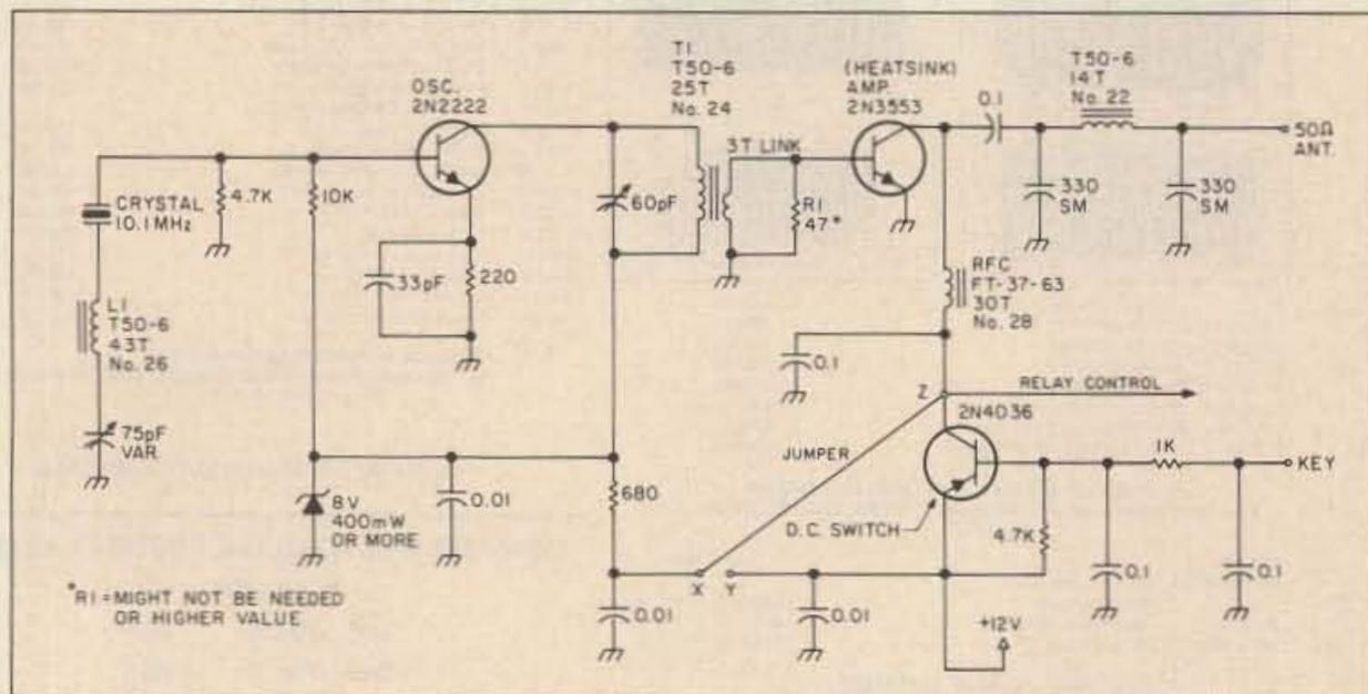
Figure 1. Schematic for the 30m QRP transmitter.
