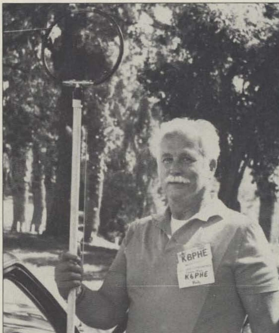
Photo A. Bob Hastings K6PHE uses a 6 meter T-hunting loop on his vehicle and on foot.
