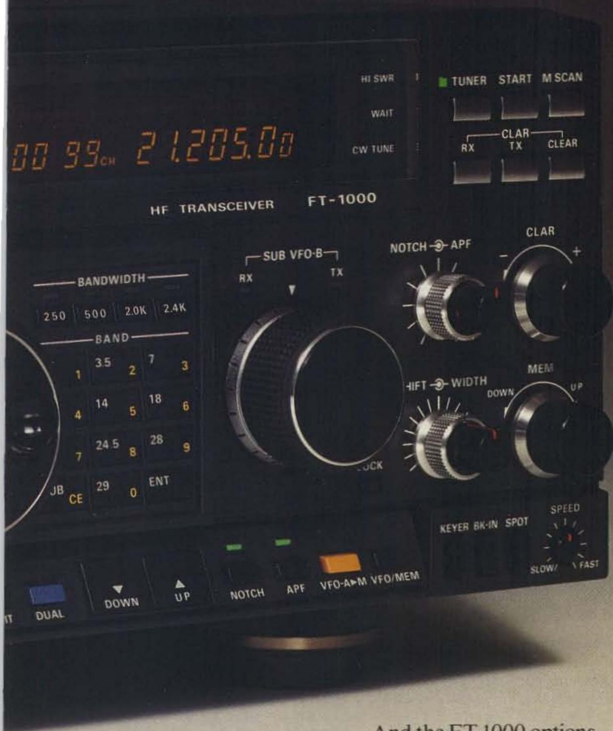
features and options that other manufacturers still have on their drawing boards: Like **200 watts RF power output**; **Built-in TCXO**, for superior frequency stability; **Independent filter selection**; **Dual receive with balance control** and **two tuning knobs** for simultaneous reception in tough pile-up situations. Using **BPF-1** allows cross-band dual receive.
