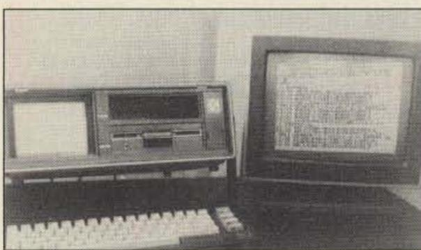
Photo A. This SX-64 (left) is running Digicom > 64 Version 2.10 with an internally mounted packet modem. External video monitor (right) displays incoming packets, with Digicom in monitor mode.
