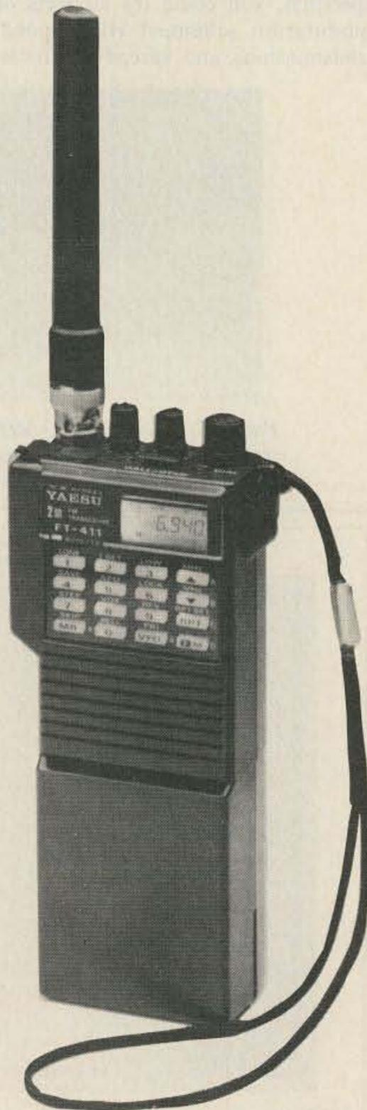
I've ever seen, and a few new ones. Frequencies may be entered in several ways. You may use the tuning knob, the UP/DOWN arrow keys, or you may key in the frequency directly from the keypad (my favorite method). When using the knob or arrow keys, a press of the FUNCTION key makes them step the VFO in 1 MHz steps. I should say VFOs, because there are two of them! Emulating modern HF rigs, VFOs A and B are identical in function and can be toggled between with a press of the VFO button.
