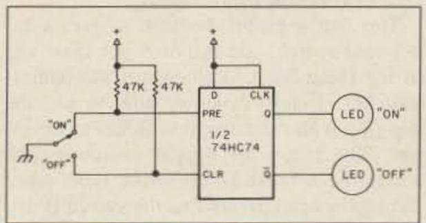
Figure 5. Flop-flop chip used as a debounced switch.
