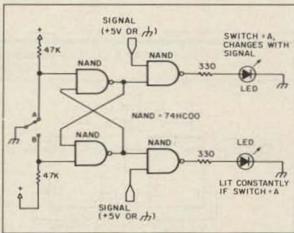
Figure 3. NAND flip-flop controlling pass/block gates.
