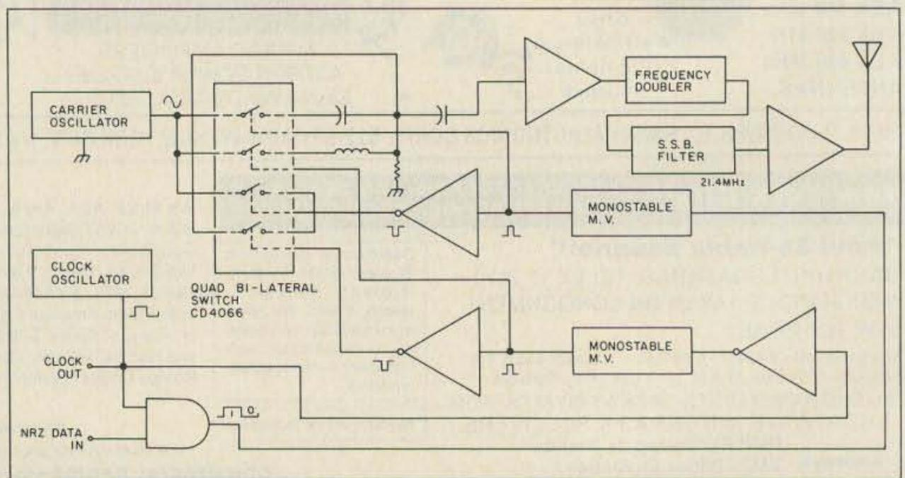
Figure 2. Transmitter block diagram.
