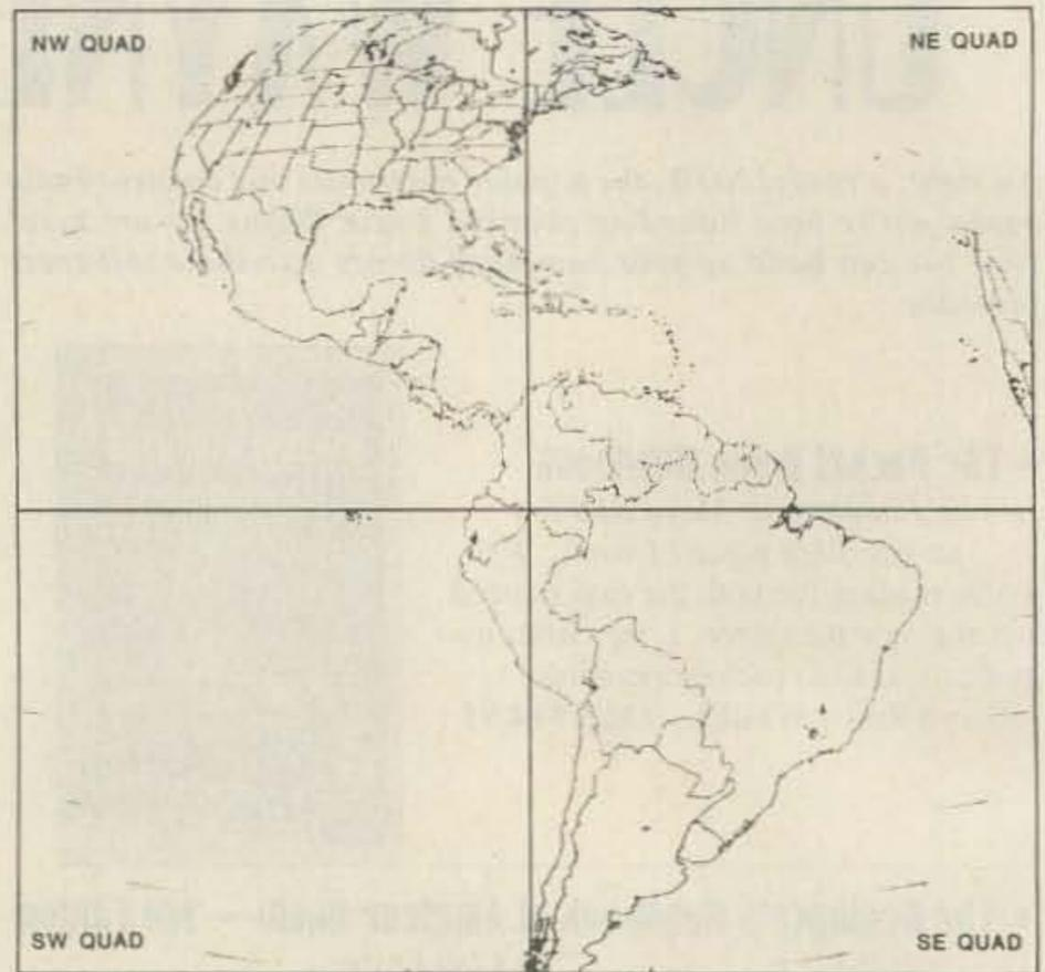
Figure 1. Diagram of the arrangement of WEFAX quads that make up the mosaic of the full earth disc as imaged by one of the GOES spacecraft. This particular diagram shows the coverage from GOES E and is reproduced from Clark, R.M. and E.W. Feigel. 1981. *The WEFAX User's Guide*. Nat. Earth Sat. Serv., NOAA, U.S. Dept. of Commerce.
