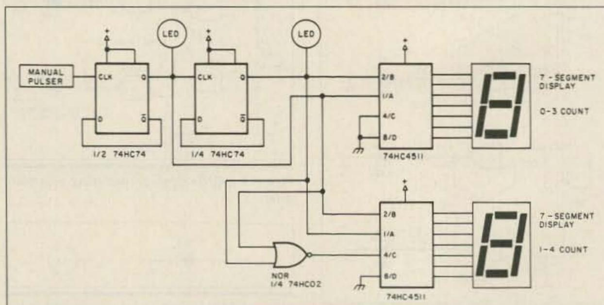
Figure 9. A flip-flop binary counter-controller-indicator.
