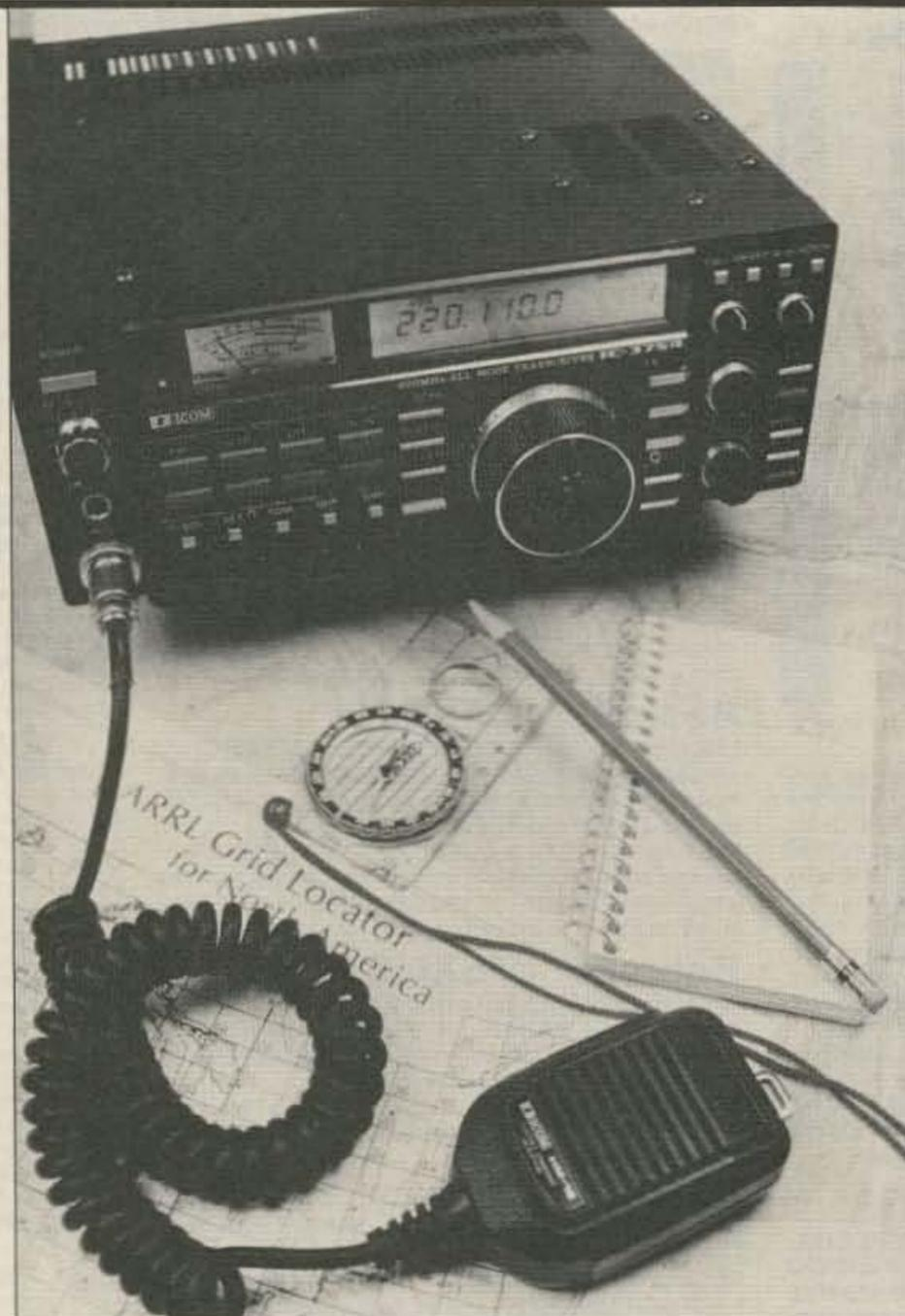
The ICOM IC-375 220-MHz multimode transceiver.
