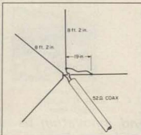
Fig. 4. 10m ground plane antenna.
