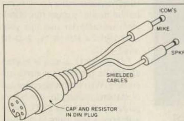
Fig. 1. (top left) How to configure the circuit parts for "Connecting Circuit" to fit inside the DIN plug.
