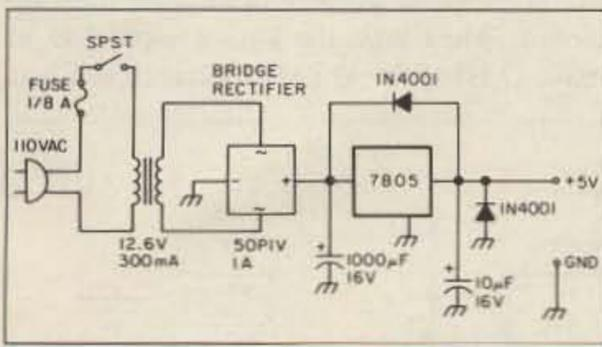
Figure 1. 5-volt test power supply.
