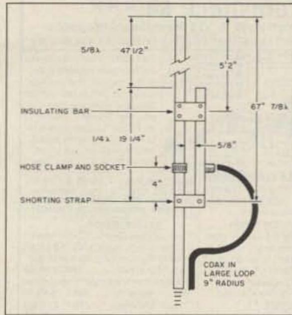
Fig. 6. Construction details of the improved J-Pole match.
