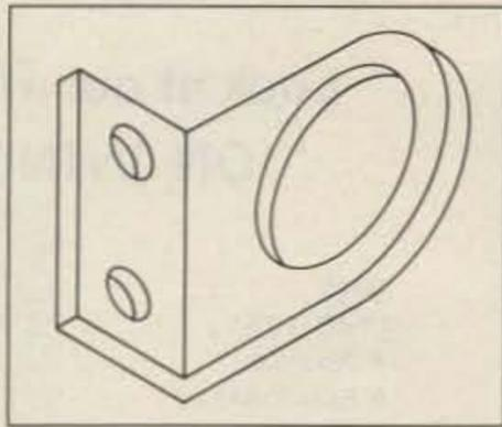
Fig. 5. Bracket for coax socket.
