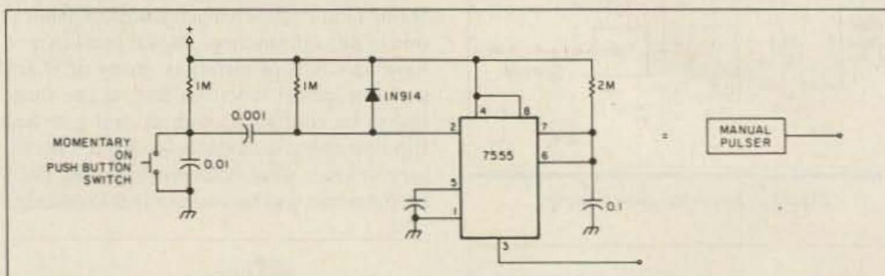
Figure 8. A handy manual pulser (pulse duration 1/3 second).
