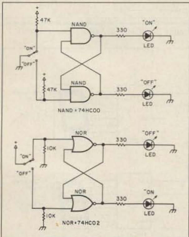
Figure 2. NAND and NOR flip-flop switches.
