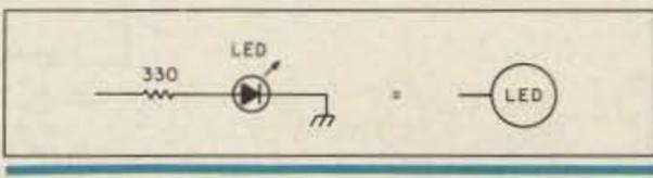
Figure 4. LED indicator symbol to simplify drawings.
