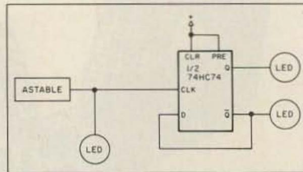
Figure 7. Basic divide-by-2 flip-flop circuit.
