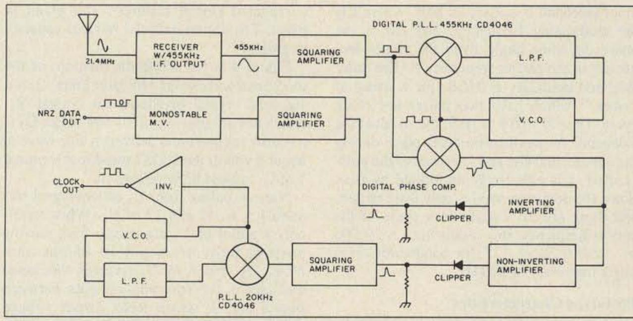
Figure 3. Block diagram of the pulsed BPSK demodulator.
