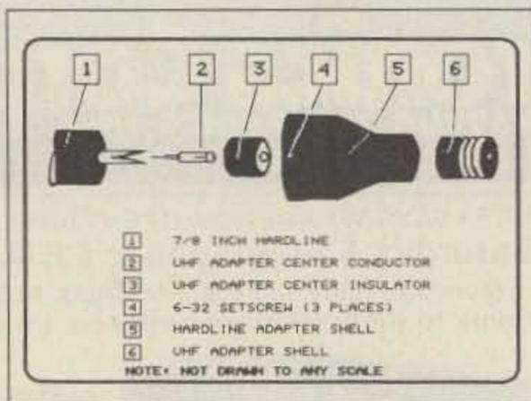
Figure 1. Hardly-Hard hardline connector assembly component parts.
