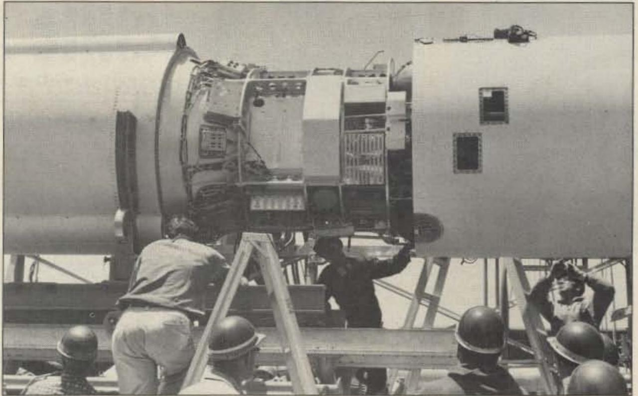
*Photo C. Assembly of the launch housing on the Agena spacecraft. The top side of OSCAR 2 shows on the right side of the rack, in the exposed section of the rocket.*
