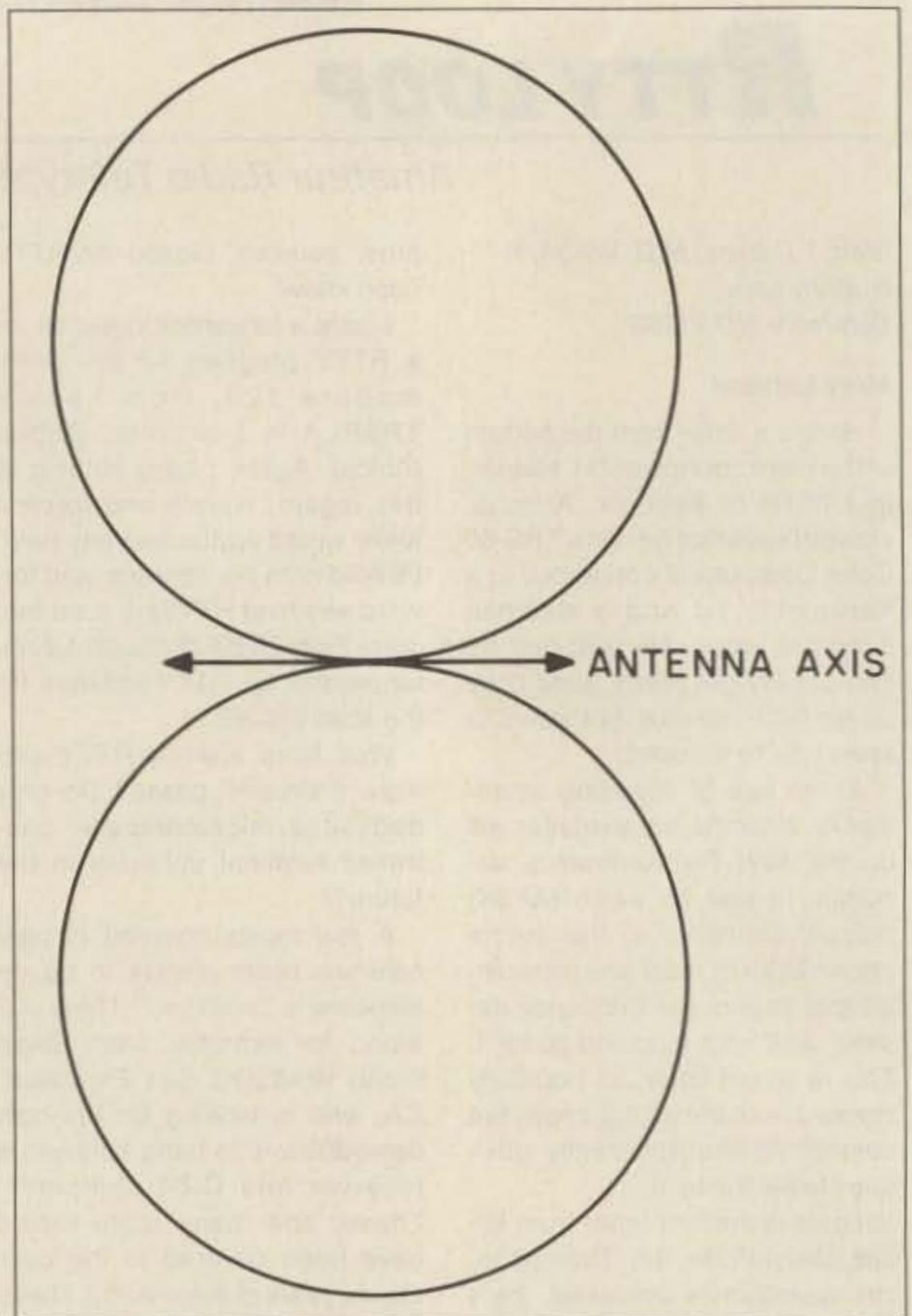
Figure 1. Horizontal directional pattern of a half-wave dipole.
