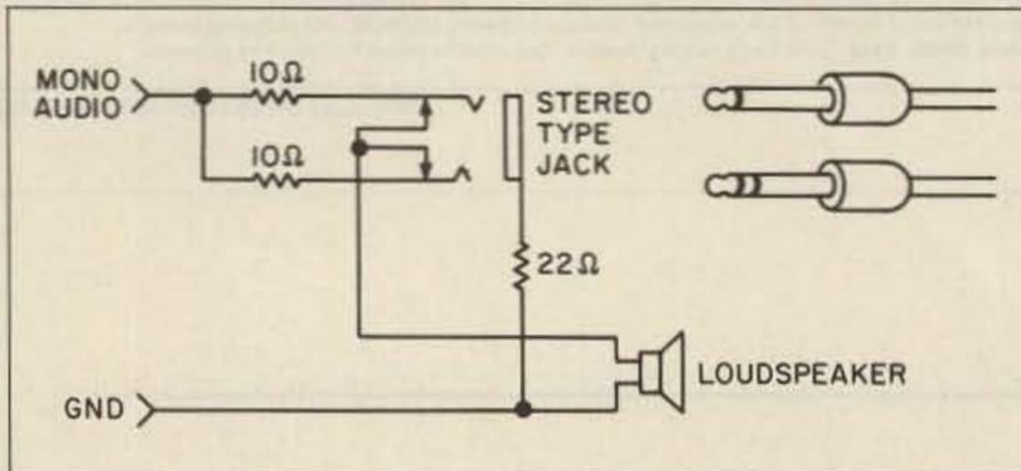
Figure 1. Adaptable monophonic output.
