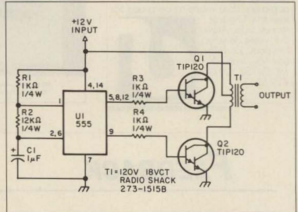
Figure 2. Low power inverter.
