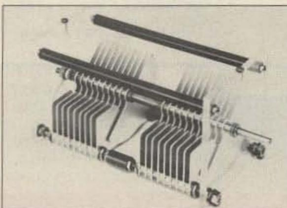
construction with gold anodizing and high voltage acrylic. These capacitors are suitable for high-power antenna matching units, power amplifiers, and transmitters. They are presently available in two values, 500pF and 250pF. The TC-250 retails for approximately
