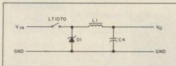
Figure 2. Positive buck converter.
