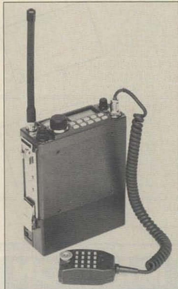
Photo B. The FT-290R II configured for portable operation with a rubber duck and an FBA-8 battery pack.
