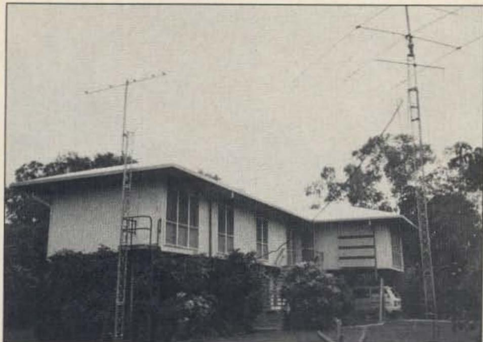
VK8LM's QTH. Left: 5-element 6m yagi; 8-element 2m yagi and 3-element triband TH3JK on right. Tower has been winched down for the wet (cyclone) season.
