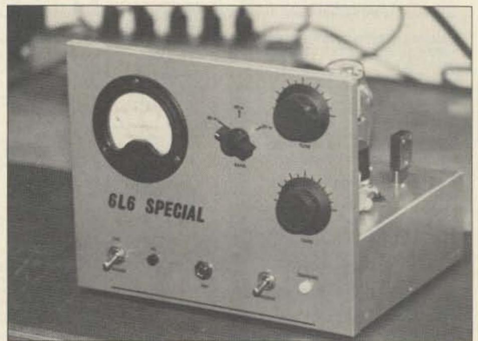
Photo B. Here it is, the 6L6 Special. A crystal-controlled 6L6 transmitter. Output of 12 Watts on 80 meters.
