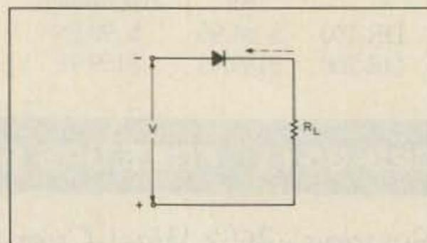
Fig. 2(b). Reverse-biased half-wave rectifier.
