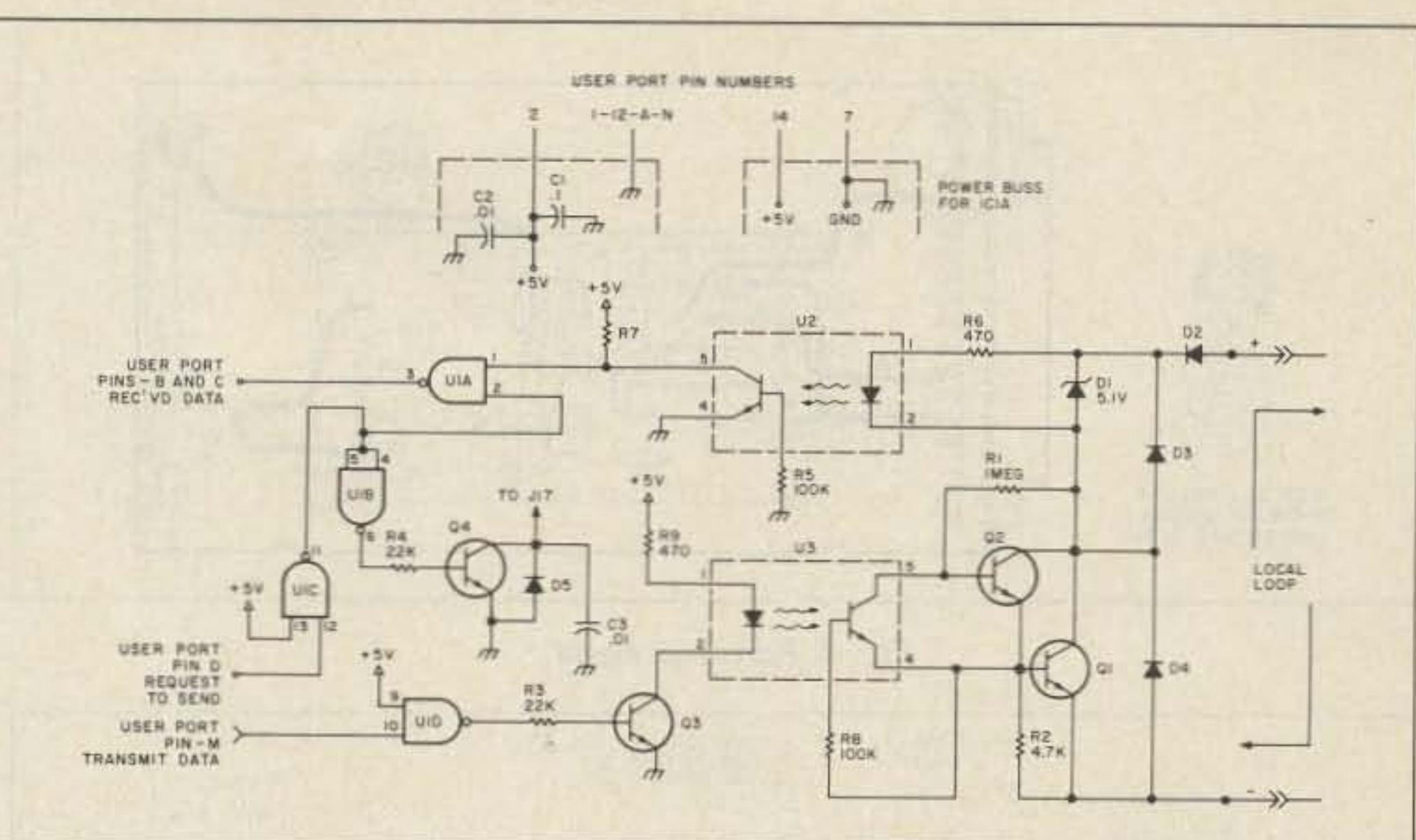
Fig. 2. RTTY/C-64 interface schematic.
