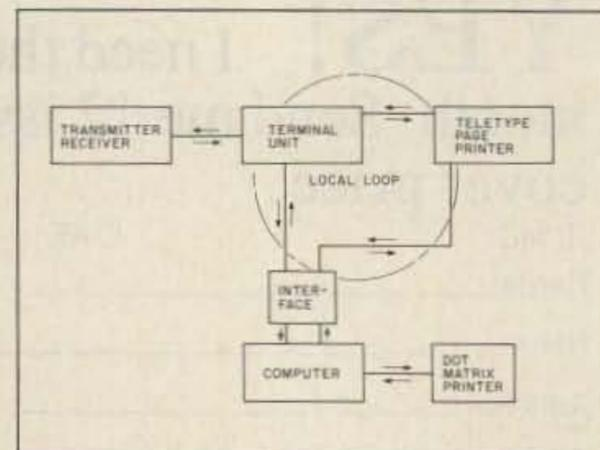
Fig. 1. Block diagram, RTTY local-loop configuration.
