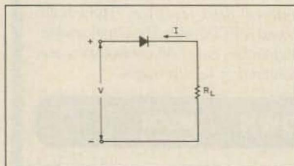
Fig. 2(a). Forward-biased half-wave rectifier.
