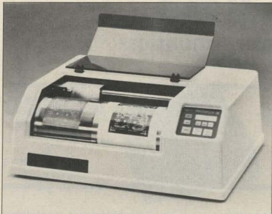
The Girard Prototflex-III printed-circuit system.
