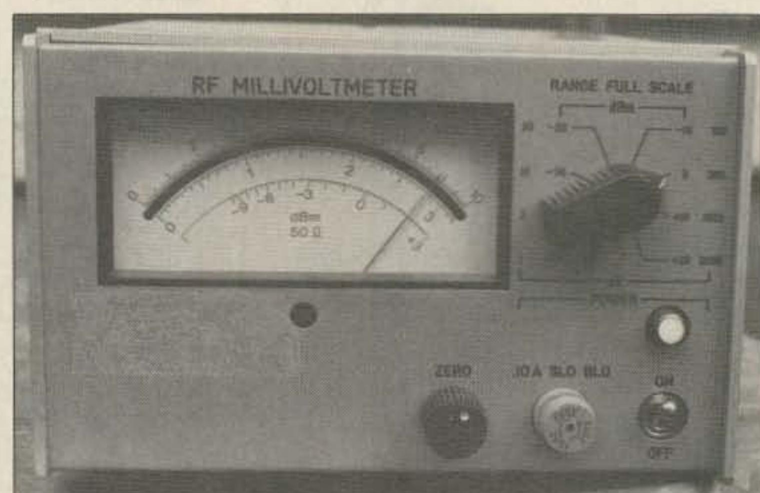
Photo C. Rf millivoltmeter measuring output from the 5/8-wave Larsen antenna in a vertical plane.
