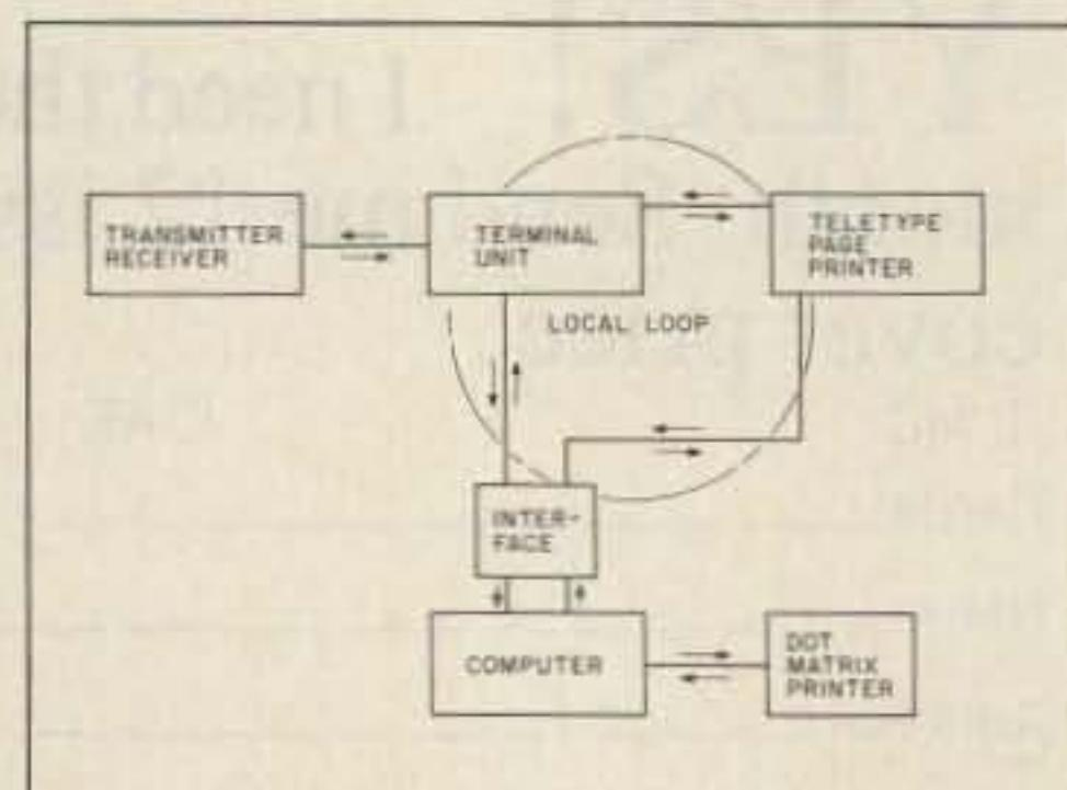
Fig. 1. Block diagram, RTTY local-loop configuration.
