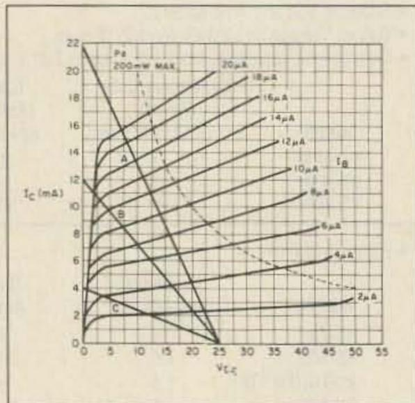
Fig. 2.  $V_{ce}$  vs.  $I_c$  characteristic curves.
