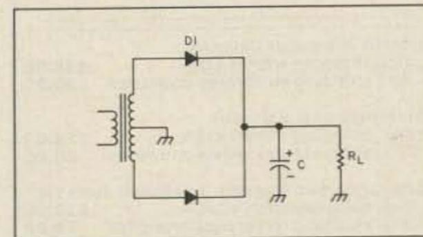
Fig. 6(a). Capacitor C smooths out the pulsating wave.
