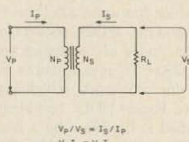
Fig. 1. The transformer is essentially a voltage converter.
