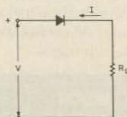
Fig. 2(a). Forward-biased half-wave rectifier.
