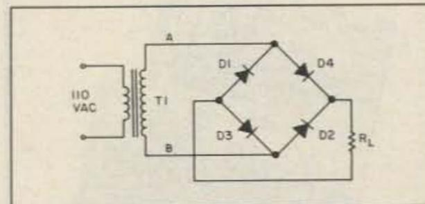
Fig. 4. The bridge rectifier requires no center tap on the transformer.
