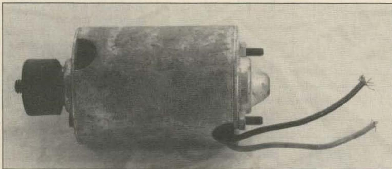
Photo A. The 1/10-horsepower, 12-V-dc bicycle pedal-assist motor.
