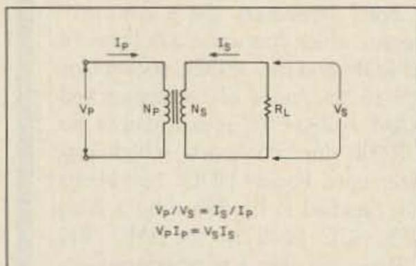
Fig. 1. The transformer is essentially a voltage converter.
