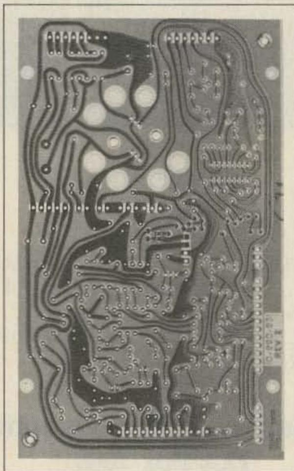
Photo B. Foil side of the "Tuner Interface" analog PC board. The power supply section is in the upper left portion of the board.
