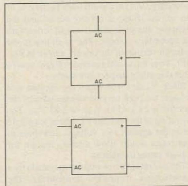
Fig. 5. Circuit symbols for integrated bridge-rectifier assemblies.
