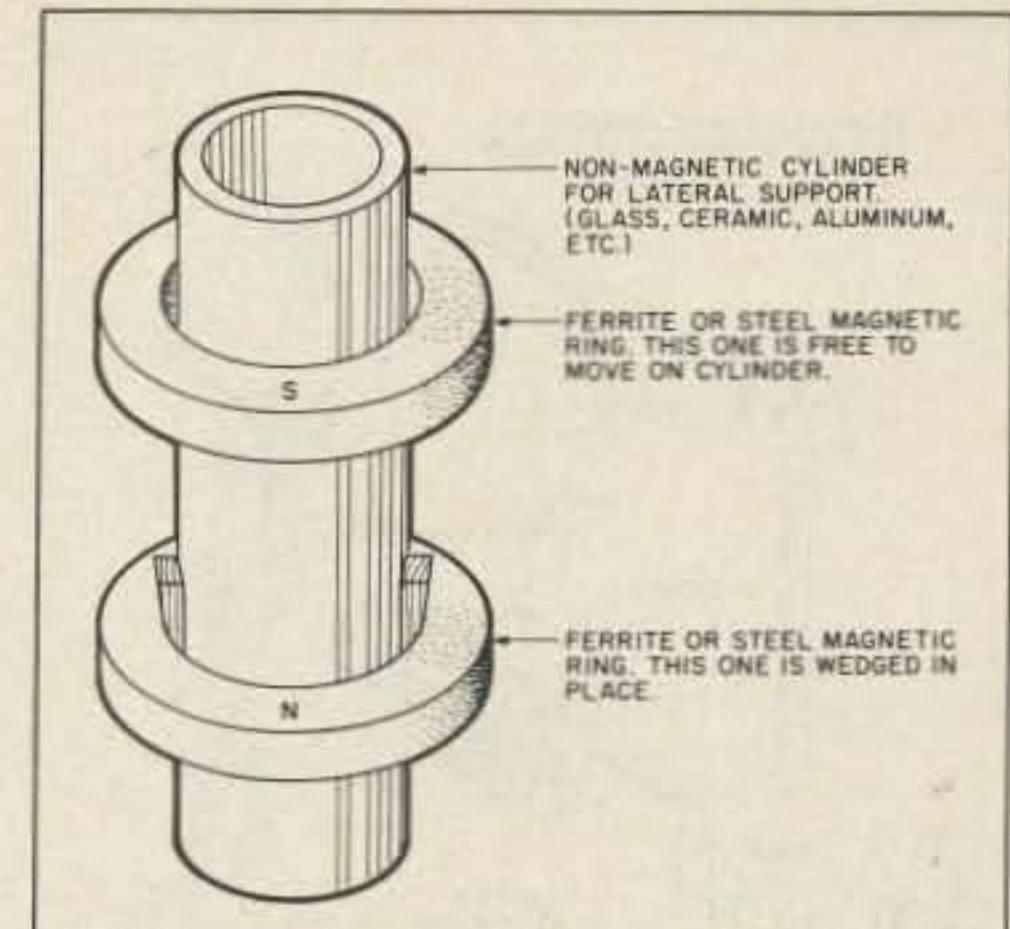
*Fig. 4. A "food-for-thought" experiment. No external energy supply is needed for the levitated ring. The upper ring remains levitated indefinitely; neither ring loses magnetic strength. The constant repulsive force from the north poles of the magnetic rings overcomes gravity. If this experiment were simulated by electromagnets, it is obvious that electrical energy would have to be supplied (but only to overcome Ohmic resistance).*
