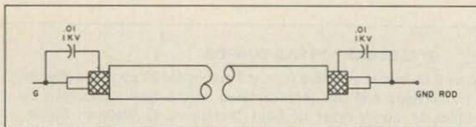
Fig. 1. The coax ground couldn't be simpler.
