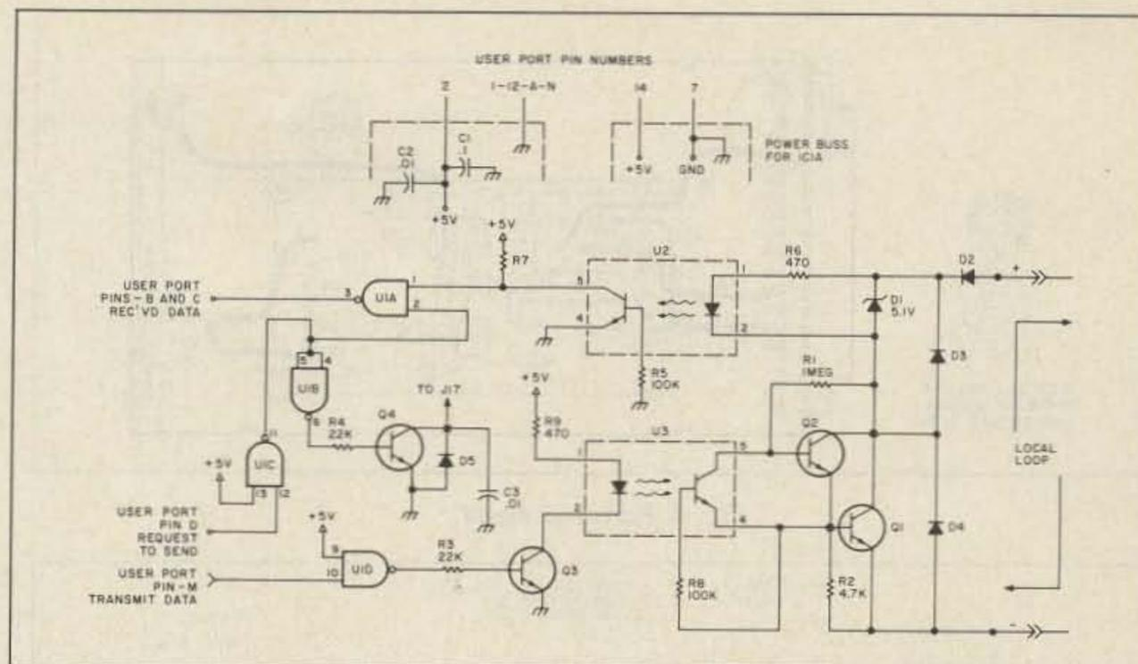
Fig. 2. RTTY/C-64 interface schematic.
