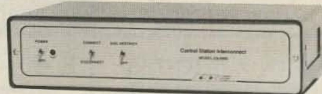
For exemplary simplex performance, the CS-9500 control station interconnect incorporates a full 1/2 second of landline to mobile electronic voice delay. Voice delay assures compatibility with the slowest CTCSS or trunked repeater systems.
