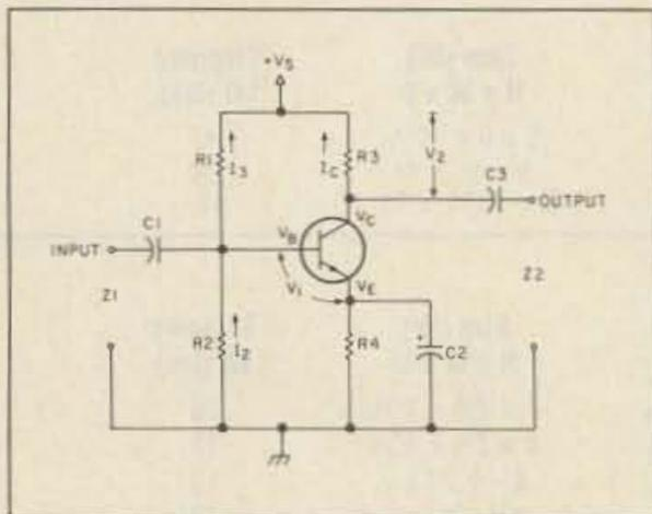
Fig. 1. Class-A common emitter amplifier.
