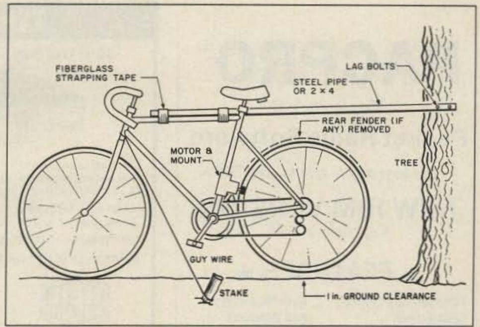
Fig. 2. The test stand. You may want to find a jockey to do the pedaling.
