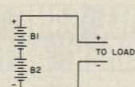
C) TWO PM MOTOR-GENERATORS IN SERIES TO CHARGE BATTERY OF 12V OR GREATER (CHECK POLARITY AND DIRECTION OF ROTATION)
