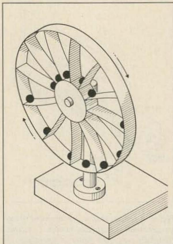
Fig. 6. Perpetual-motion wheel for providing free energy from gravity. This is a typical application of the unbalanced or over-balanced wheel. The radius arm of the steel balls is supposed to shift in such a manner as to keep the wheel turning.
