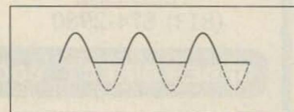
Fig. 2(c). Output waveform of a half-wave rectifier.
