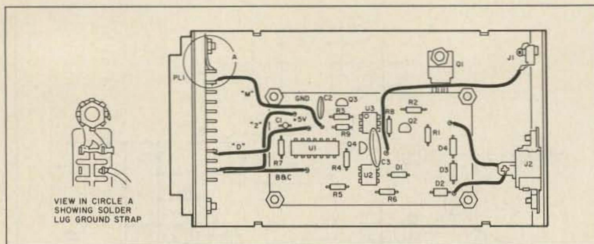
Fig. 4. Parts placement.
