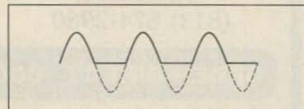
Fig. 2(c). Output waveform of a half-wave rectifier.
