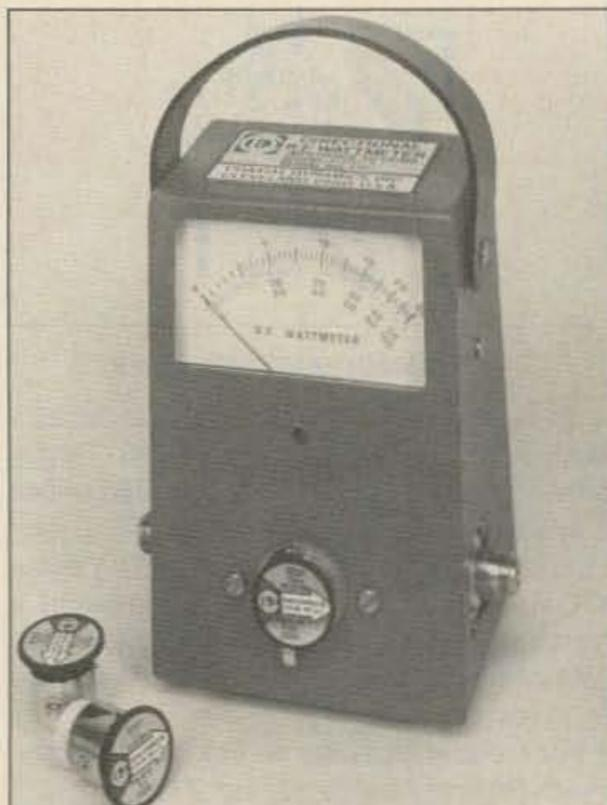
Coaxial Dynamic's model 81000-A rf wattmeter.
