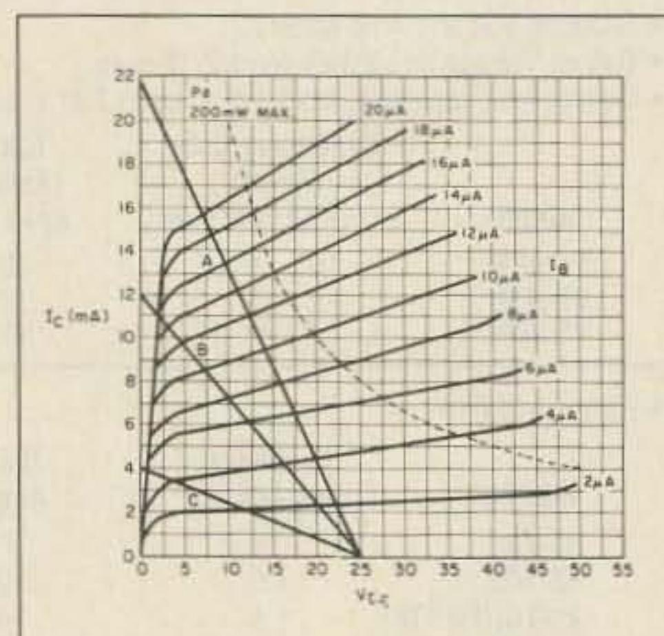
Fig. 2.  $V_{ce}$  vs.  $I_c$  characteristic curves.
