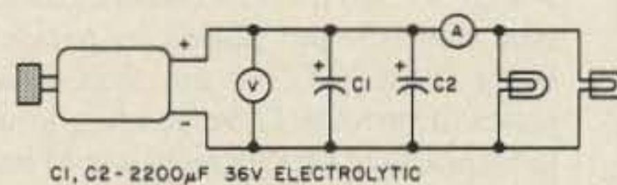
Fig. 3. Modified test circuit, with two 2,200-uF capacitors in parallel with the armature and the load.
