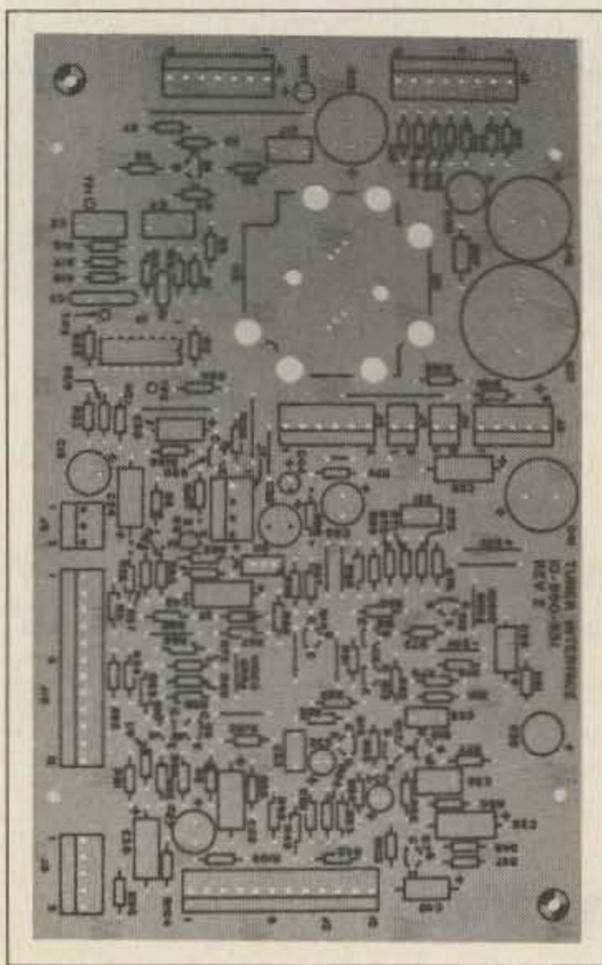
Photo A. Component side of the "Tuner Interface" analog PC board. The power supply section is in the upper right portion of the board.
