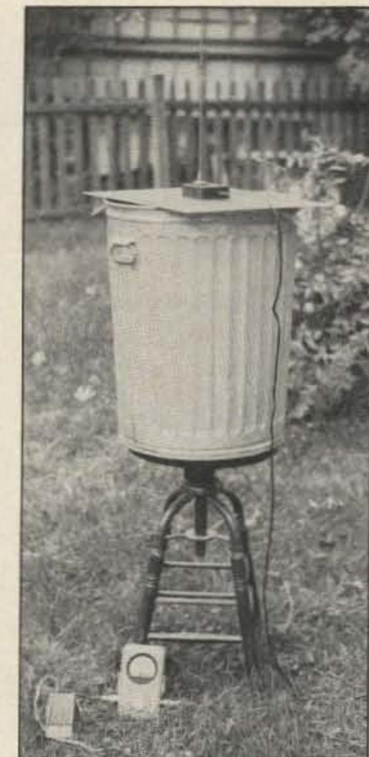
*Photo E. The test rf source, an IC-2AT, feeds a Larsen quarter-wave antenna. A Bird 43 monitors steady output.*
