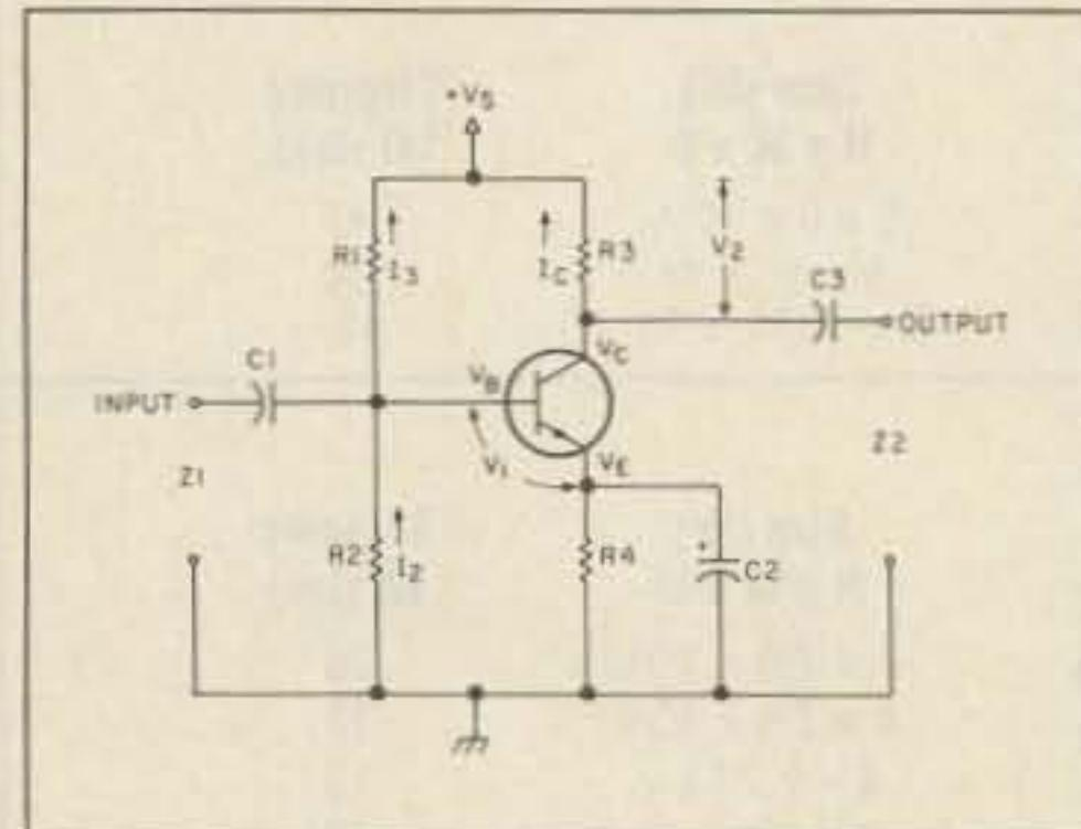
Fig. 1. Class-A common emitter amplifier.
