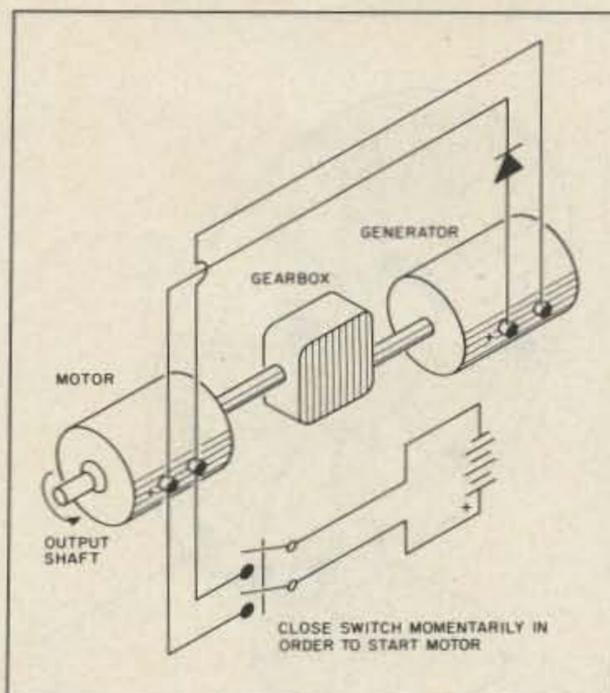
Fig. 3. A representative arrangement of motor-generator perpetual-motion systems. Hopefully, once the motor is operating, its continued operation will be sustained from the output of the generator. The switch, dc source, and the rectifier comprise the startup circuit. Hopefully, too, the gear box ascertains that the motor will be able to drive the generator fast enough to develop high output from the generator.
