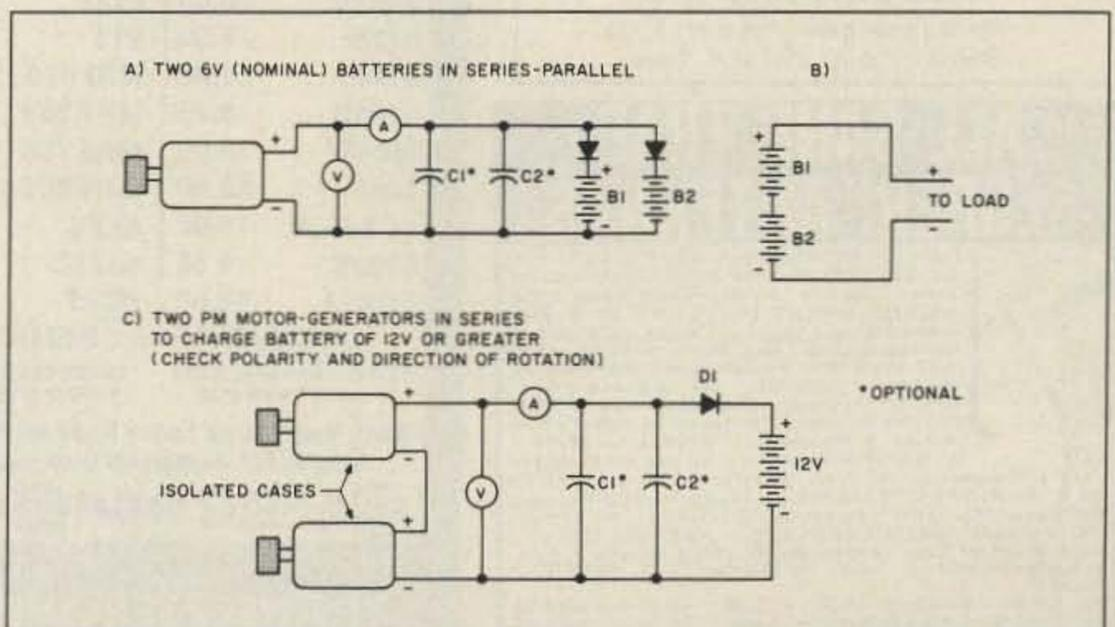
Fig. 5. (a) Two 6-V batteries in parallel while being recharged and (b) switched to series while in use. (c) Two motor generators in series.
