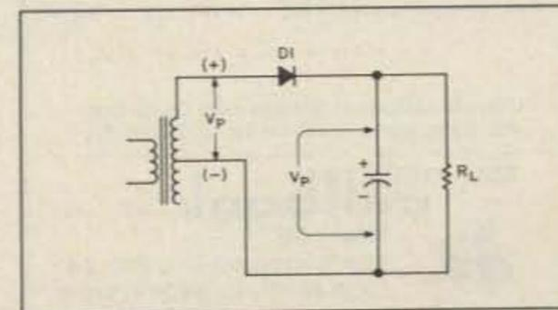
Fig. 6(b). This is what D1 sees on the alternate half-cycle.
