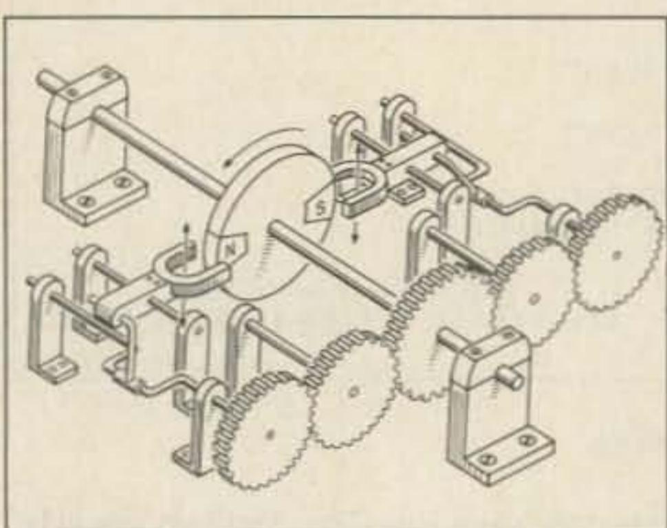
Fig. 1. Hitherto, attempts to secure continuous rotation in motors using only magnets have not been successful. An obstacle has been a condition of latchup wherein the arrangement quickly comes to a standstill after very limited motion. In this invention, a mechanical-feedback system is claimed to prevent such stoppage. The inventor promises to demonstrate such a self-running motor as soon as certain frictional losses can be reduced to a satisfactory level.
