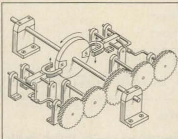
Fig. 1. Hitherto, attempts to secure continuous rotation in motors using only magnets have not been successful. An obstacle has been a condition of latching wherein the arrangement quickly comes to a standstill after very limited motion. In this invention, a mechanical-feedback system is claimed to prevent such stoppage. The inventor promises to demonstrate such a self-running motor as soon as certain frictional losses can be reduced to a satisfactory level.
