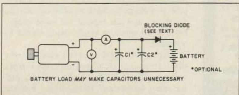
Fig. 4. Substitute a germanium diode for the silicon one and you can save a half volt or more because of the lower forward voltage drop.
