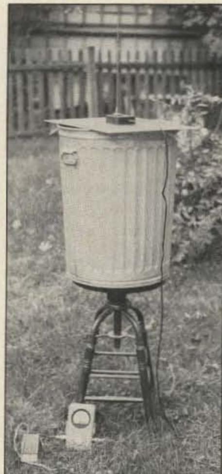
Photo E. The test rf source, an IC-2AT, feeds a Larsen quarter-wave antenna. A Bird 43 monitors steady output.
