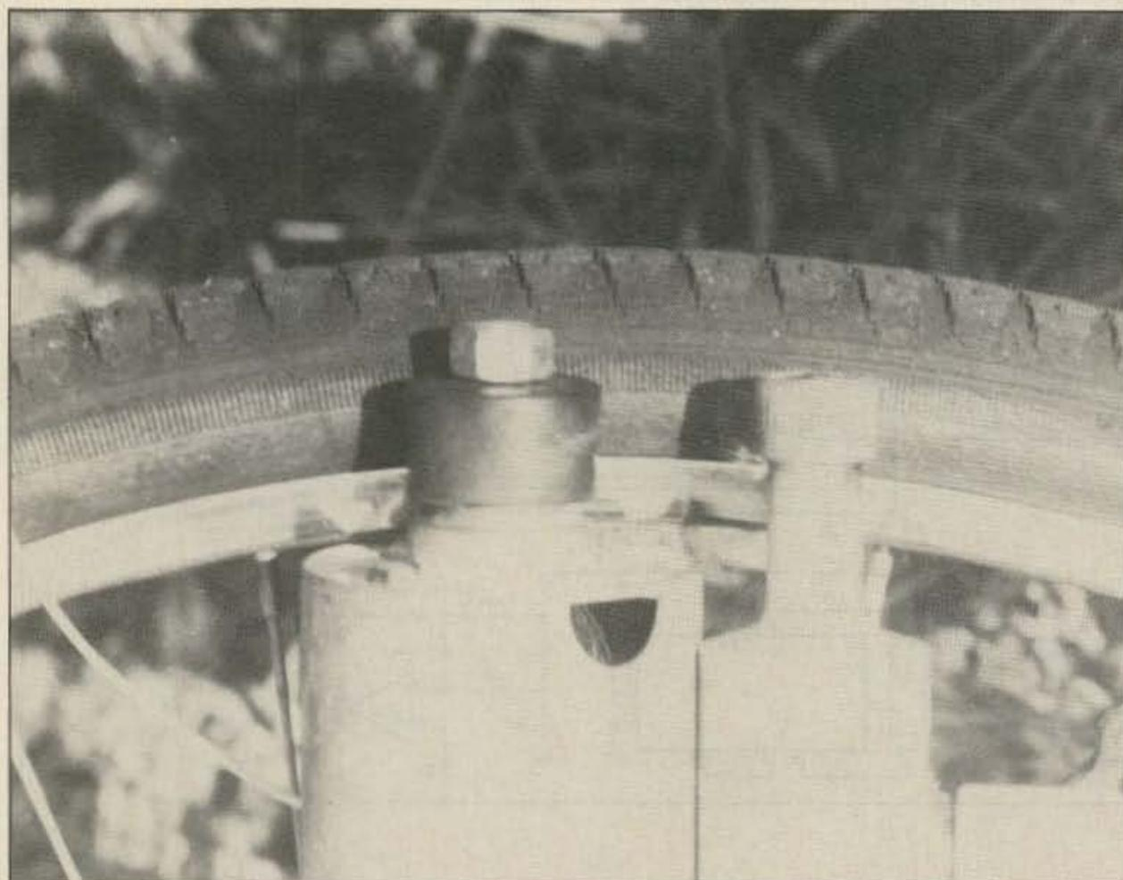
Photo B. The motor with the home-brew friction roller mounted against the bicycle tire rim. The smaller roller is the regular bicycle headlight generator.
