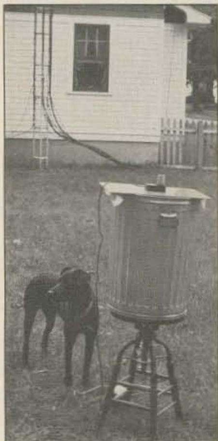
Photo A. The horizontal vs. vertical polarization test range. The 5/8-wave vertical is in the foreground and the KLM beam is in the background. Crescent, VHF/UHF's most famous dog, guards the test setup.
