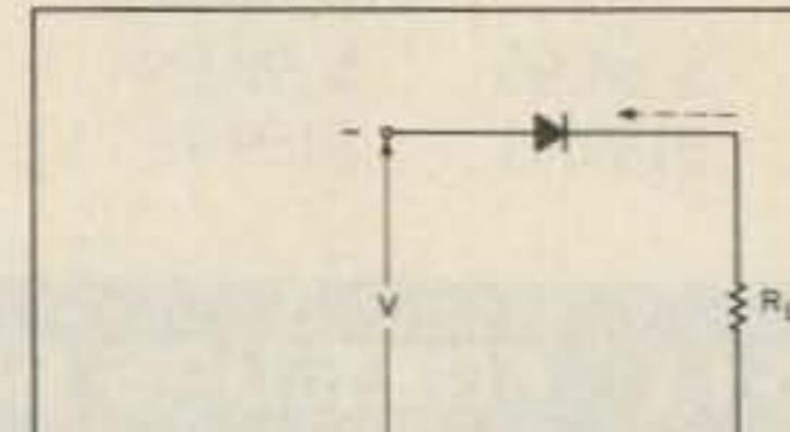
Fig. 2(b). Reverse-biased half-wave rectifier.
