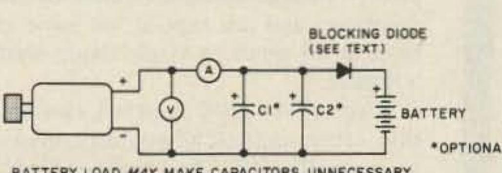
Fig. 4. Substitute a germanium diode for the silicon one and you can save a half volt or more because of the lower forward voltage drop.
