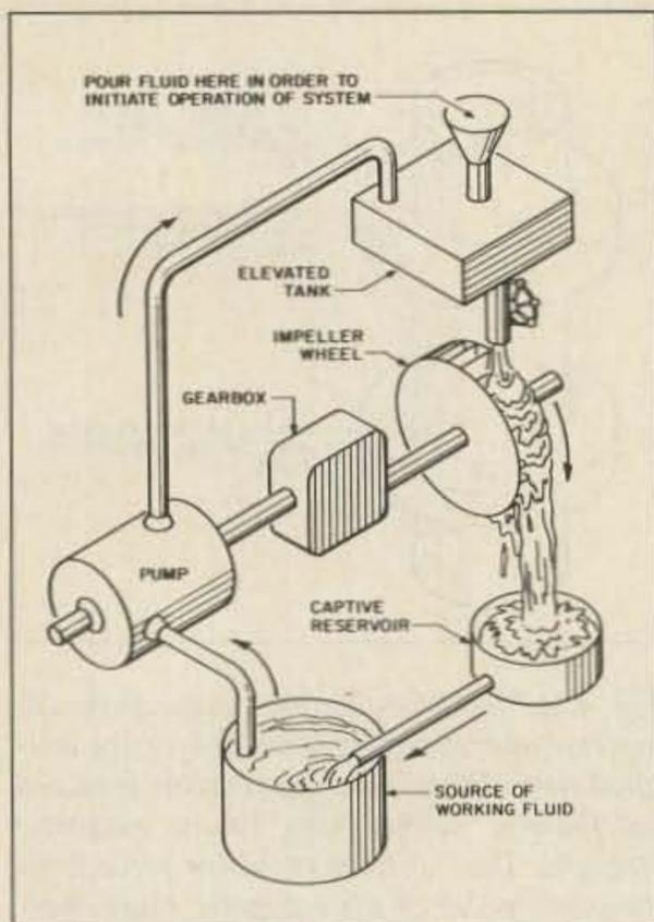
Fig. 5. Basic theme of many hydraulic perpetual-motion systems. Operation of a closed-cycle system is supposed to be self-sustained after initial startup. The gear box represents inventor's attempt to obtain more vigorous pumping action, thereby "fooling" the system to overcome its losses.
