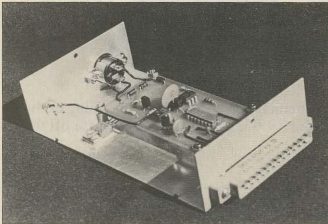
Photo A. The fully assembled interface with top cover removed.
