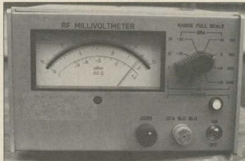
Photo C. Rf millivoltmeter measuring output from the 5/8-wave Larsen antenna in a vertical plane.
