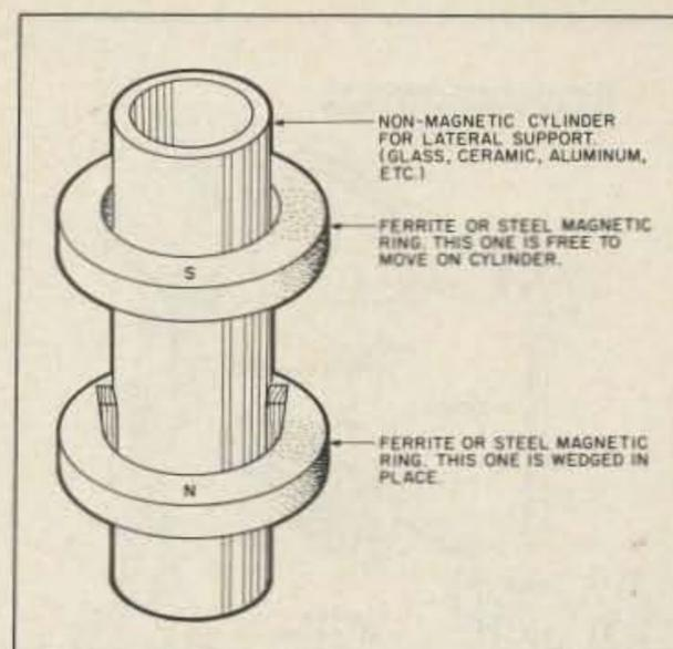
Fig. 4. A "food-for-thought" experiment. No external energy supply is needed for the levitated ring. The upper ring remains levitated indefinitely; neither ring loses magnetic strength. The constant repulsive force from the north poles of the magnetic rings overcomes gravity. If this experiment were simulated by electromagnets, it is obvious that electrical energy would have to be supplied (but only to overcome Ohmic resistance).
