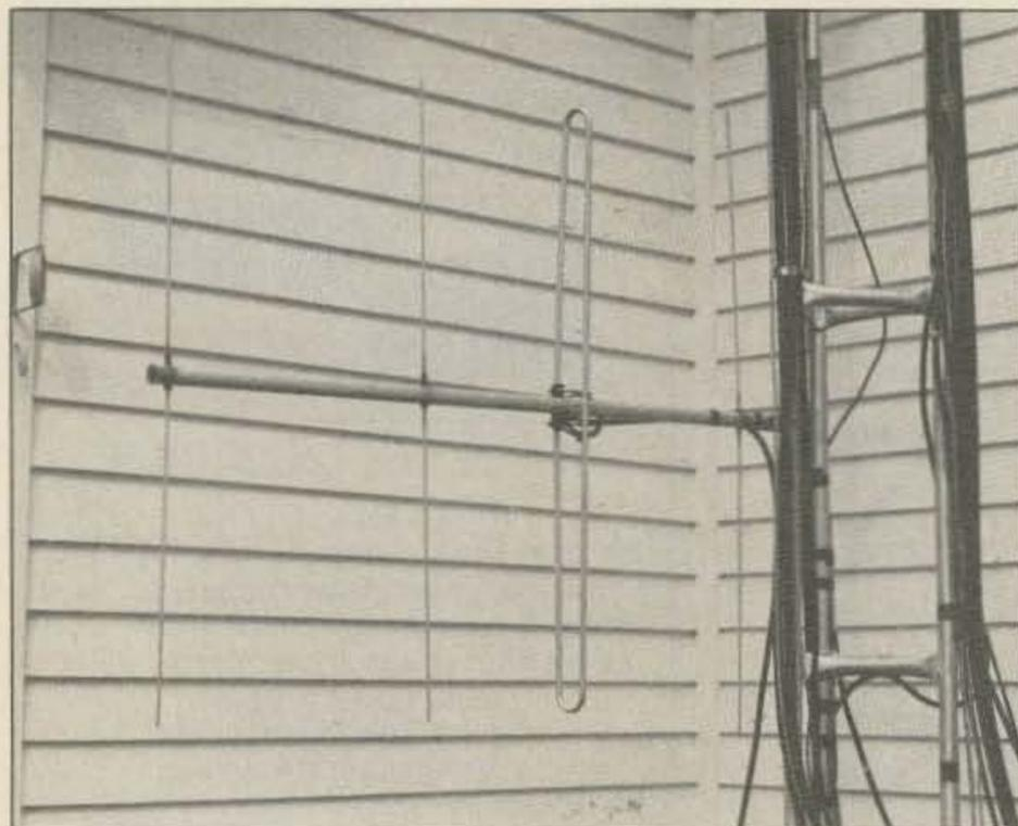
Photo B. The four-element KLM beam is connected to the tower and is vertically polarized. Output from the KLM beam is fed to an rf millivoltmeter.
