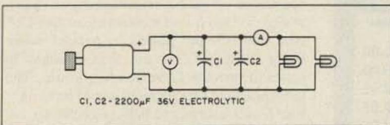
Fig. 3. Modified test circuit, with two 2,200-uF capacitors in parallel with the armature and the load.
