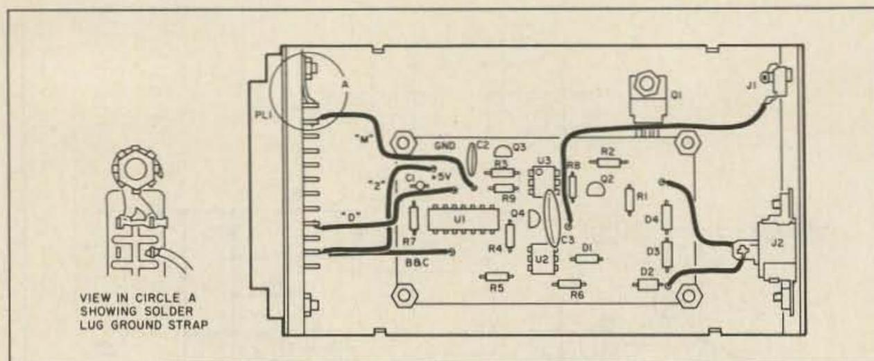
Fig. 4. Parts placement.
