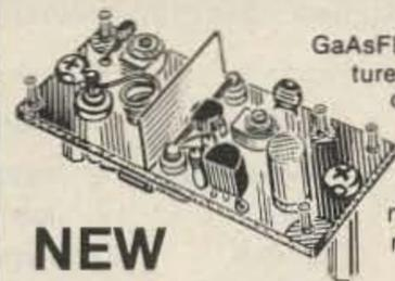
GaAsFET Preamps with features similar to LNG, except designed for LOW COST and SMALL SIZE: only 5/8"W x 1-5/8"L x 3/4"H. Easily mounts inside many radios.
