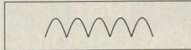
Fig. 3(b). Characteristic double-humped waveform of full-wave rectifier.
