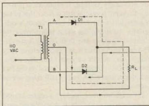
Fig. 3(a). Basic full-wave rectifier using a center-tapped transformer.
