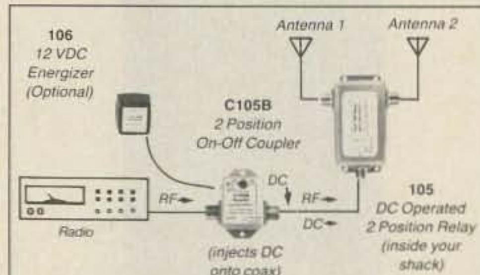
Antennas Etc.'s remote switching system.
