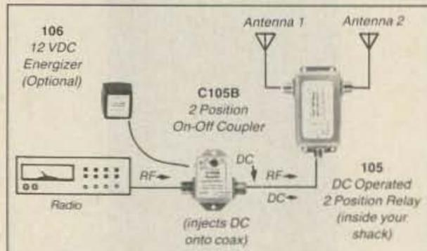
Antennas Etc.'s remote switching system.
