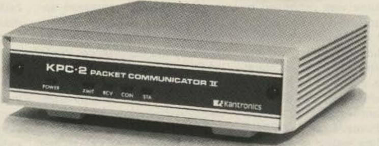
KPC-2 Kantronics AX.25 Version 2 TNC features a built-in HF modem, full duplex operation, multiple connects, and over 100 software commands. A serial RS-232 or TTL (C-64/ VIC-20) port gives universal compatibility. The enhanced generic command structure fits any computer, even PC compatibles. All this combines to make KPC-2 the only TNC you'll ever need. Suggested retail \$219.00.
