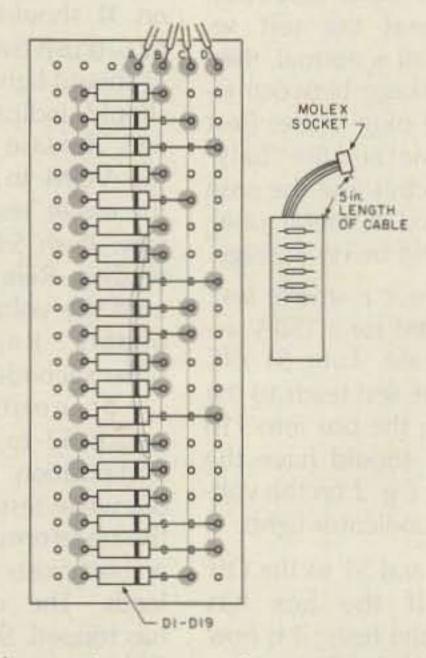
Fig. 4. Diode-matrix construction, component side.
