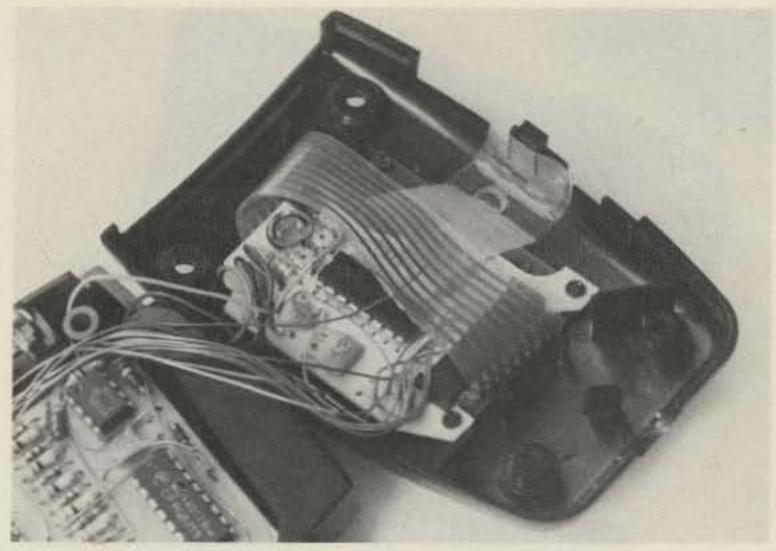
Photo C. In the PCM-369 microphone, the row-and-column leads are connected to the existing solder pins of the plastic bus connector. Route the wires underneath the flat printed-bus cable. Be careful not to burn or melt this printed bus or the connector when soldering in this cramped area.
