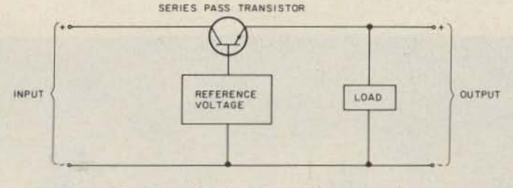
Fig. 1(a). Simplified series voltage regulator.
