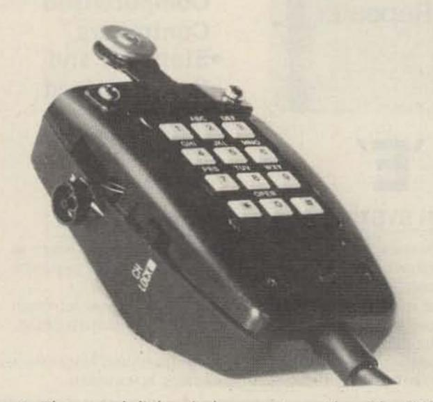
Photo A. The speed-dial switch mounts on the side of the microphone near the area where the remote volume control used to be. A protection ring around the dial button eliminates any accidental dialing sequences while handling the microphone.
