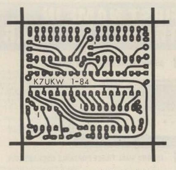
Fig. 11. Circuit pattern, full size, foil side.
