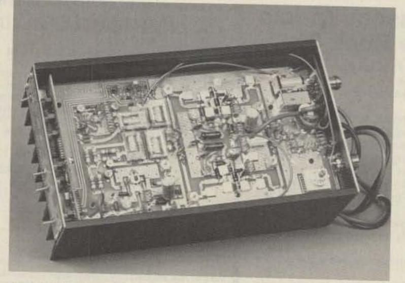
Photo B. Underside of the MML/200-S showing input-selector switch, lower right.
