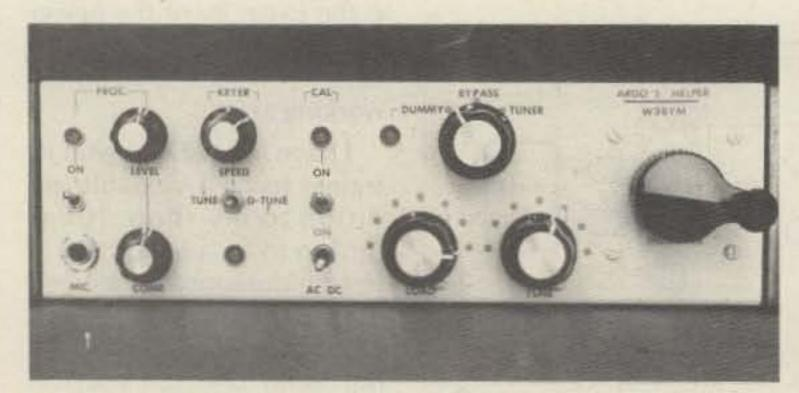
Photo A. Front-panel view — notice arrows indicating direction for tune and delay tune. LED colors are red for power and CAL, green for dummy load and processor.
