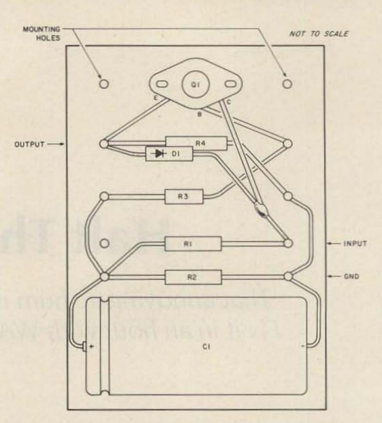
Fig. 3. Pictorial layout of the hum eliminator.
