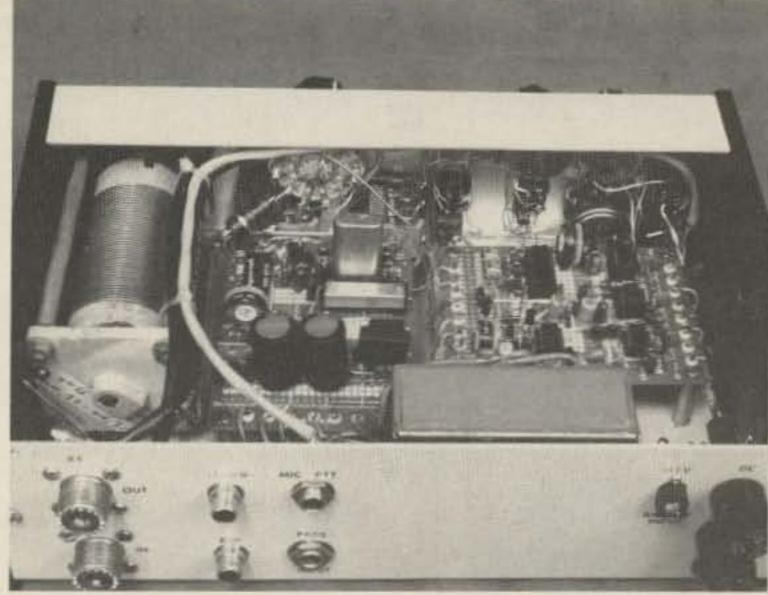
Photo D. Internal front portion showing board layouts and rotary inductor. Notice the RG-58/U routing.
