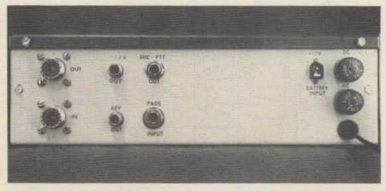
Photo B. Rear-panel view—rf connectors are SO-239, plus 13.8 and key-out are RCA phono types. Plus 12-V-dc battery input is a panel-mount coaxial power connector.
