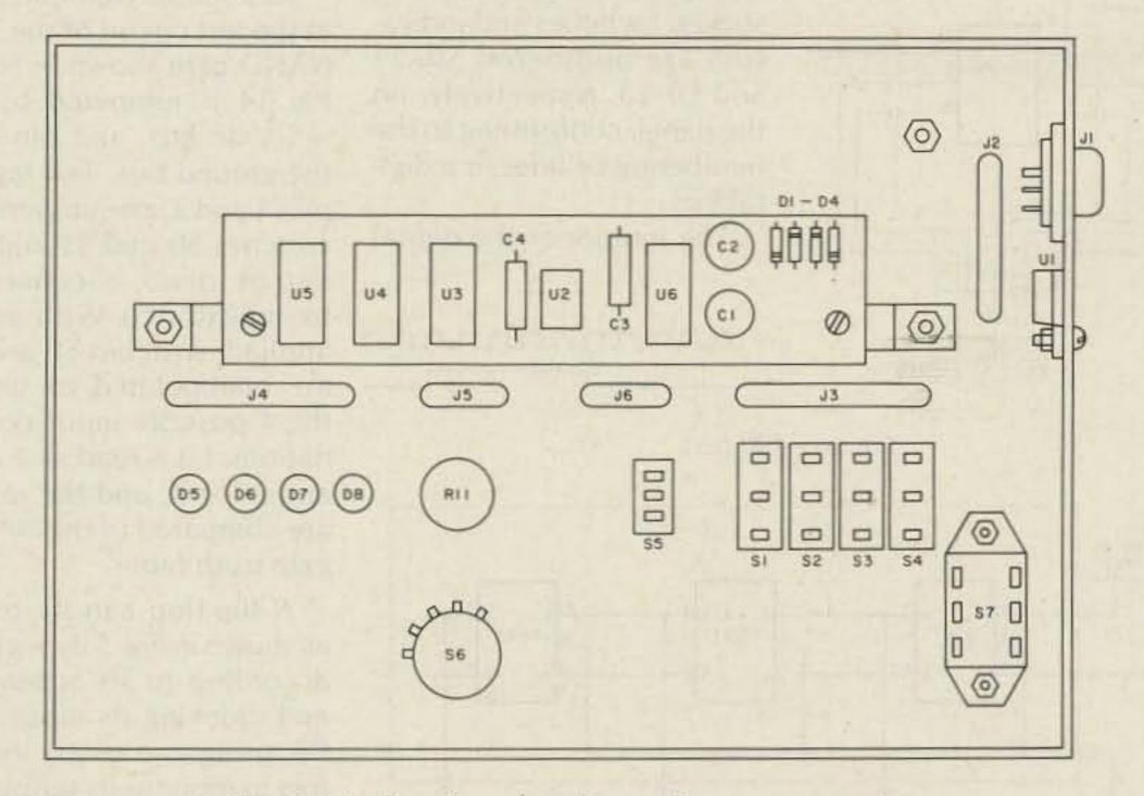
Fig. 3. Interior view showing major components.
