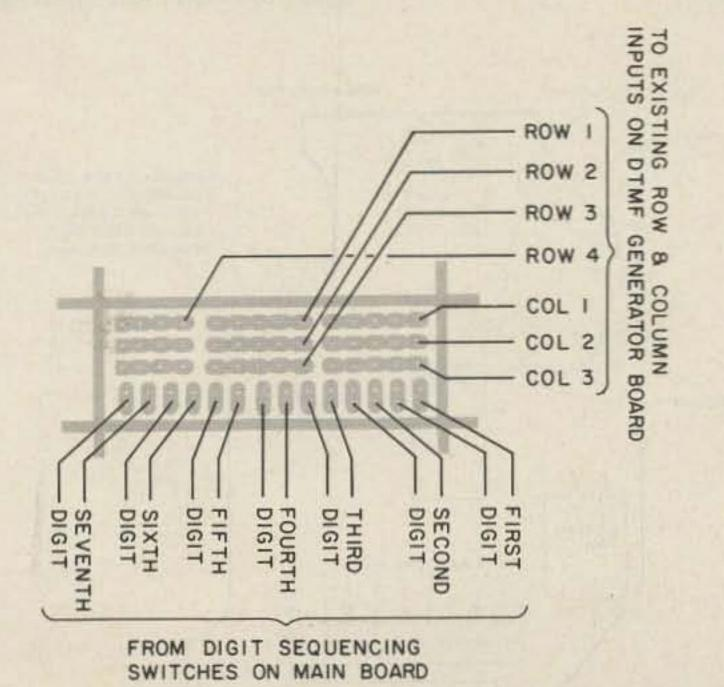
Fig. 7. Solder side of the program board, showing interconnect routing.
