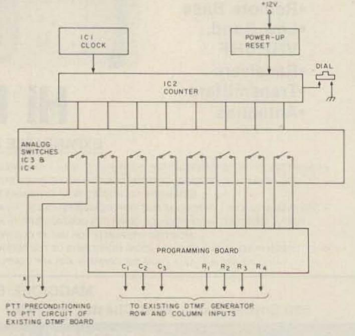
Fig.1. Block diagram of the speed-dial circuit.
