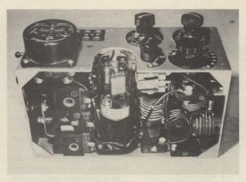
Photo D. At the right, tuning capacitor C5, and around it coils L1, L2, and L3. Left of the tube, the connectors for two antennas (or antenna and counterpoise), and at the extreme left, the Morse key.
