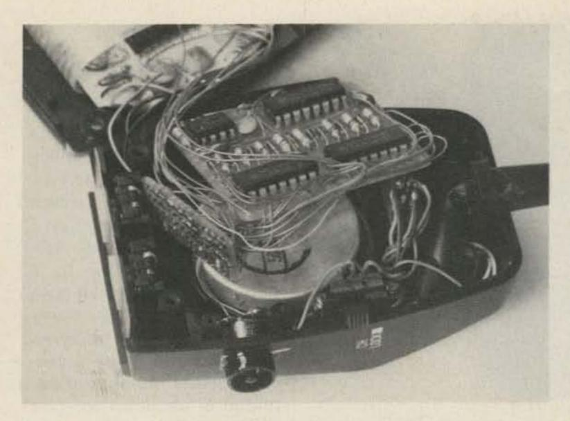
Photo E. Packing it all inside the microphone case looks impossible at first glance. The little program board slips vertically between the mike element and the two up/down switches; cover the solder side with electrical tape first. The main board then overlaps it and lies flat against the mike element, insulated with Kraft paper.
