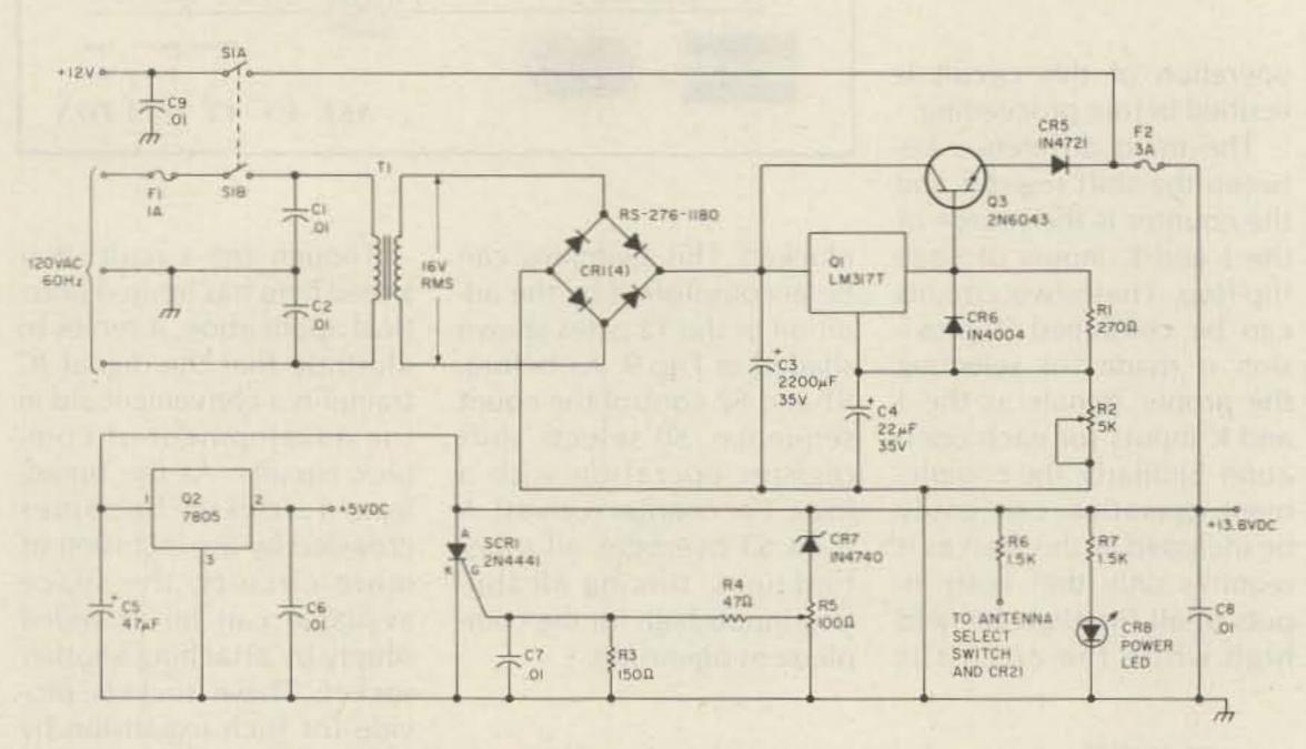
Fig. 1. Power supply and crowbar protection circuit.
