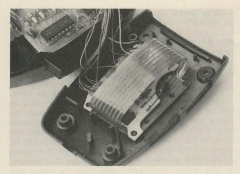
Photo B. In the newer-style microphone (Model PCM-369), capacitor C3 must be changed to a physically smaller tantalum type. Leave its leads long and let it hang over the edge of the board. The older-style PCM-2000 microphone does not need this change.
