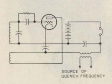
Fig. 1. An elementary superregenerative circuit as shown in the ARRL Radio Amateur's Handbook of 1936.
