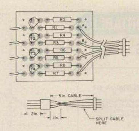
Fig. 6. Inverter/level translator board, component side.
