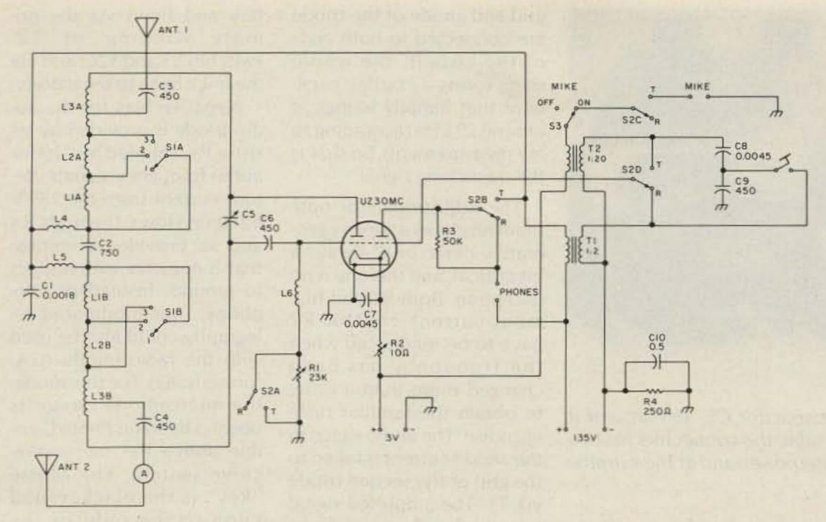
Fig. 4. Circuit diagram of radio type 94-6. The transmit/receive switching is somewhat simplified.
