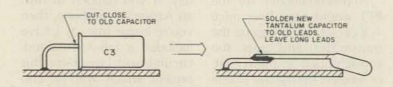
Fig. 4. For the PCM-369 microphone, replace C3 with a smaller tantalum capacitor. Leave long leads and let it hang over the edge of the encoder board.
