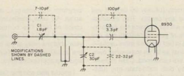
Fig. 2. Modifications necessary for putting 144 MHz on your AM-6155 amplifier.
