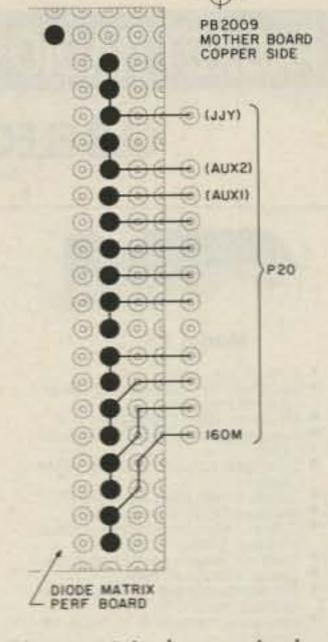
Fig. 7. Diode-matrix board pinout.
