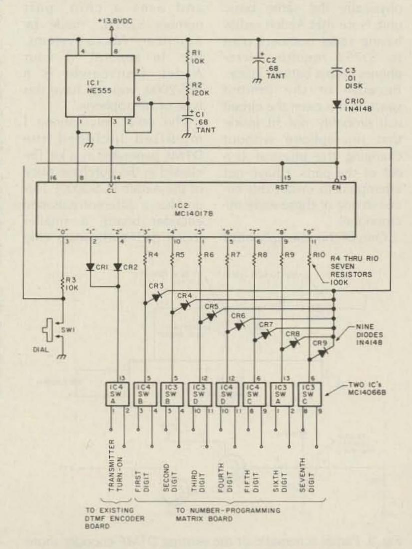
Fig. 2. Schematic of the speed-dial circuit.
