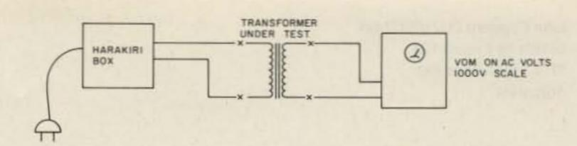
Fig. 5. Setup for using the Hara-Kiri box.
