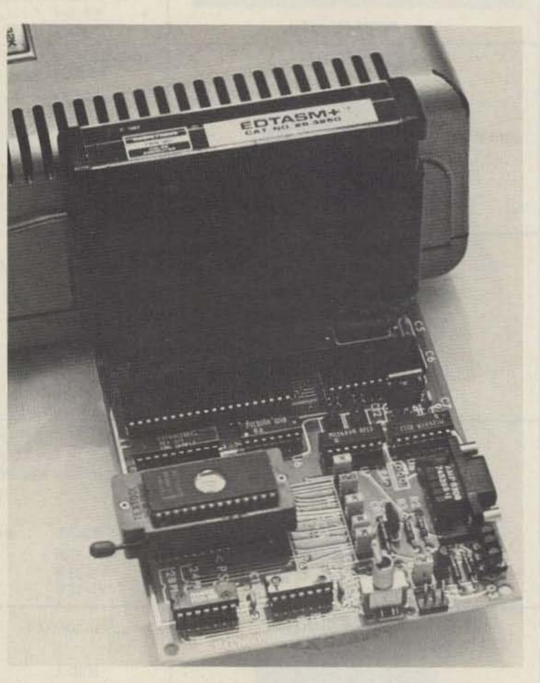
Photo C. The CRA and Associates Universal EPROM Programmer. This unit can be considered a complete development system. It also offers protection to the CoCo via full buffering.
