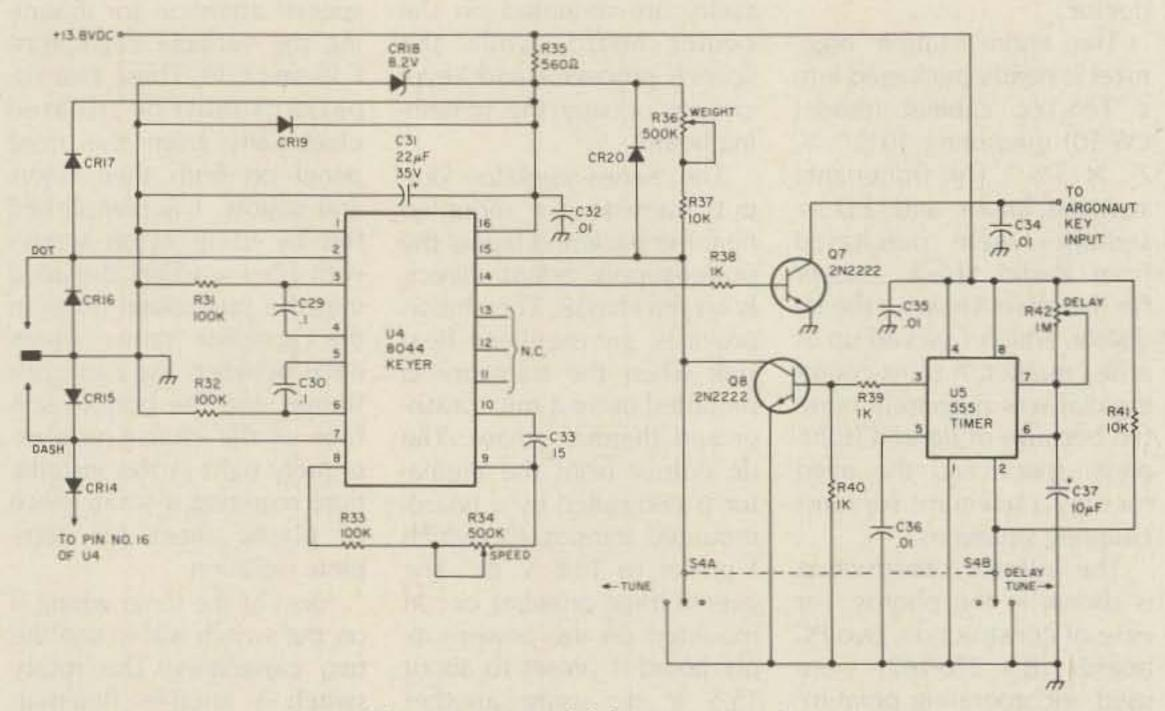
Fig. 4. Keyer and delay-tune circuit.
