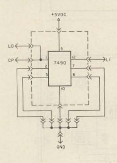
500 Hz to 50 kHz, adjustable by R11, so the CP output is 2.5 Hz to 250 Hz in low range and 250 Hz to 25 kHz in high range.
