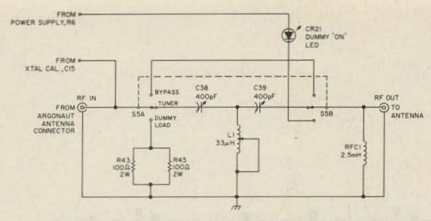
Fig. 5. Antenna tuner, bypass, and dummy-load circuit.
