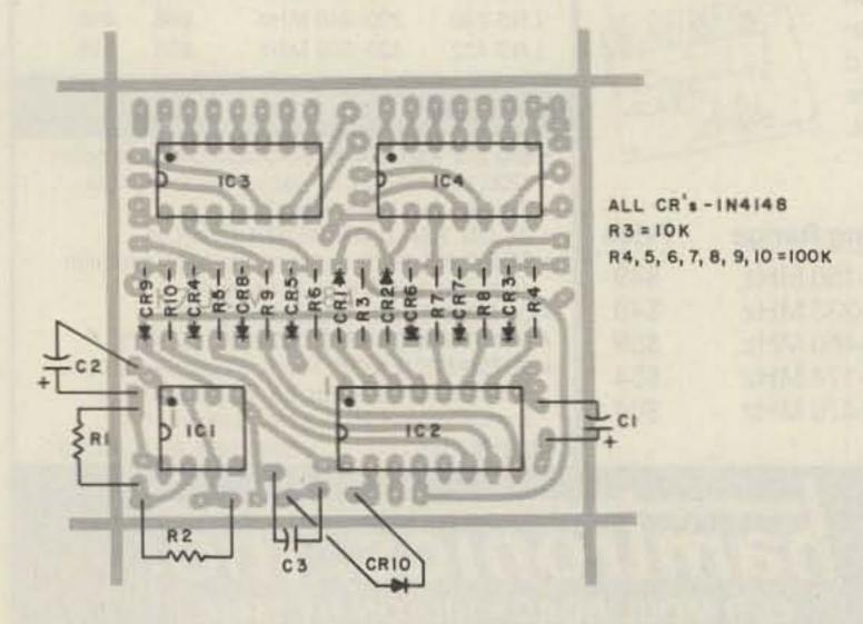
Fig. 6. Parts placement guide as seen through the board.
