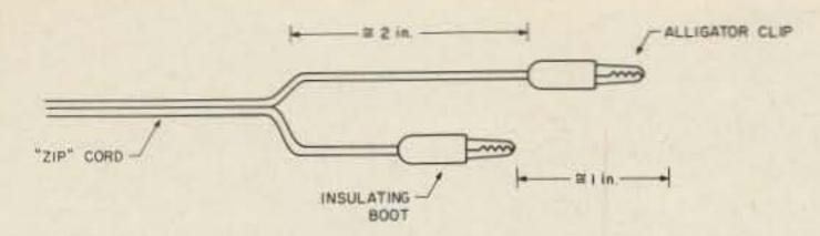
Fig. 4. Preparation of the test leads.
