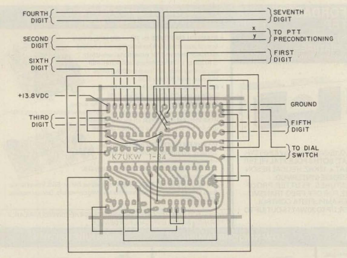
Fig. 5. Layout of the main board, shown from the foil side, detailing jumpers and interconnect wires.
