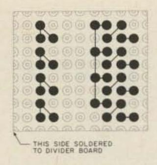
Fig. 5. Inverter/level translator board, foil side.
