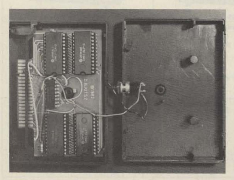
Photo A. A RAM pack configured to give 8K of RAM at the cartridge port. The switch is a "Comprise" auto-execute (see text).
