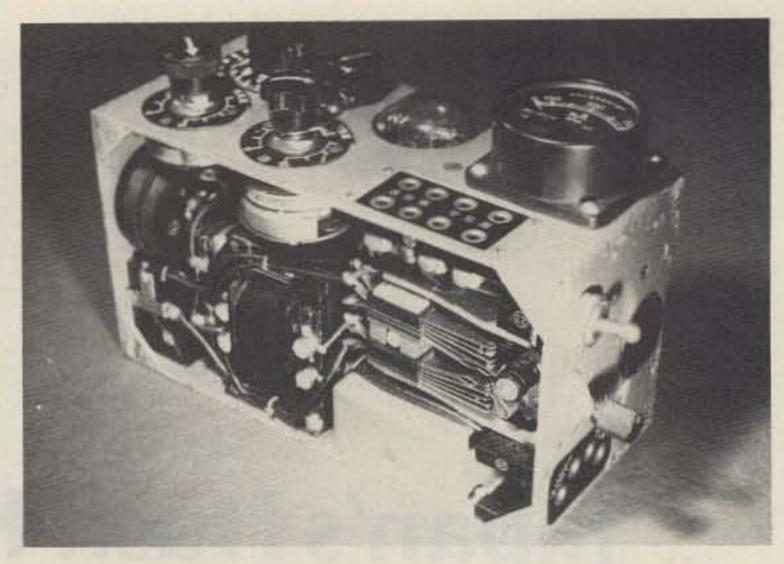
Photo C. At the right center, transmit/receive switch S2; above it, switch S3 to interrupt the microphone circuit when using telegraphy. Behind S2, the Morse "key" can be seen. At the bottom, the cable to the generator is plugged in. Inside the radio, transformer T1 is fastened to the bottom. Microphone transformer T2 is in a screened box below S2. The two round coils below filament-control R3 are L4 and L5, the tuning coils for the quenching oscillation.
