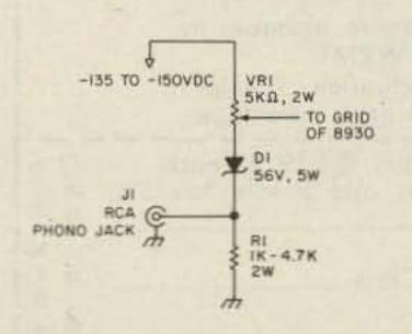
Fig. 1. The optional bias circuit as it should have appeared in December's column on AM-6155 amplifiers.
