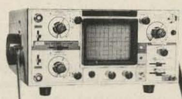
Ideal for field/bench applications, this scope can display up to 15 MHz signals. Internal battery pack allows up to 2 hours operation on a single charge. Features include . built-in battery charger • 5X horizontal magnification high brightness CRT • front panel trace rotator . internal rechargeable battery pack
