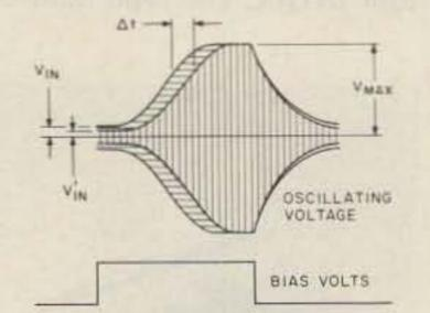
Fig. 2. Oscillating voltages in the superregenerative receiver ensuing from two starting levels,  $V_{in}$  and  $V'_{in}$  respectively, and finally building up to the same voltage,  $V_{max}$ . Lower section: Bias voltage as dependent on time, caused by the quenching oscillator. In reality the voltage is not rectangular but sinusoidal.
