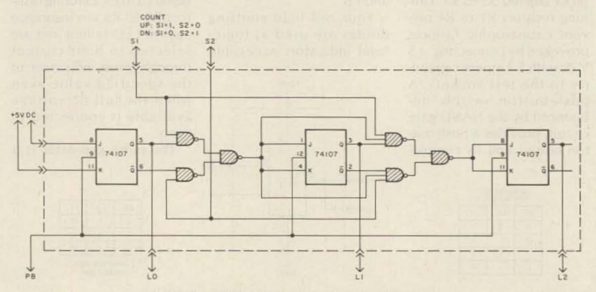
Fig. 8. Parallel up/down counter development.
