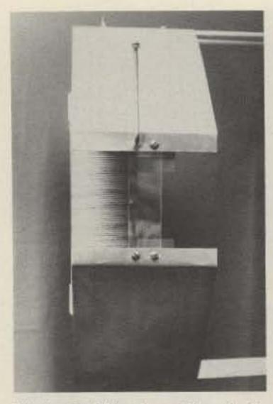
Photo C. Side view. The plastic holds the upper and lower wings together under slight tension.
