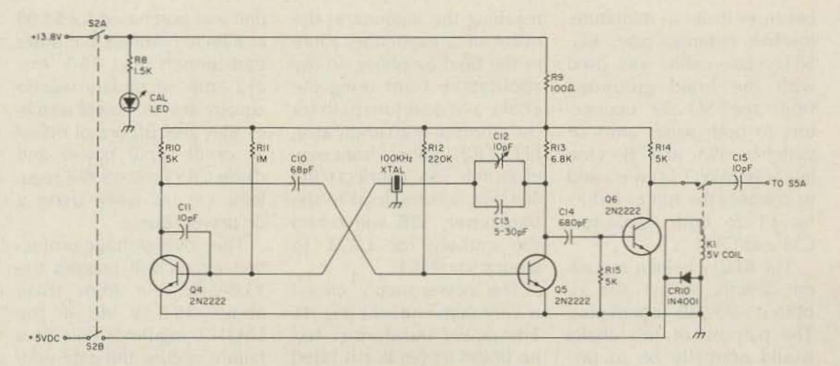
Fig. 2. Crystal calibrator circuit.
