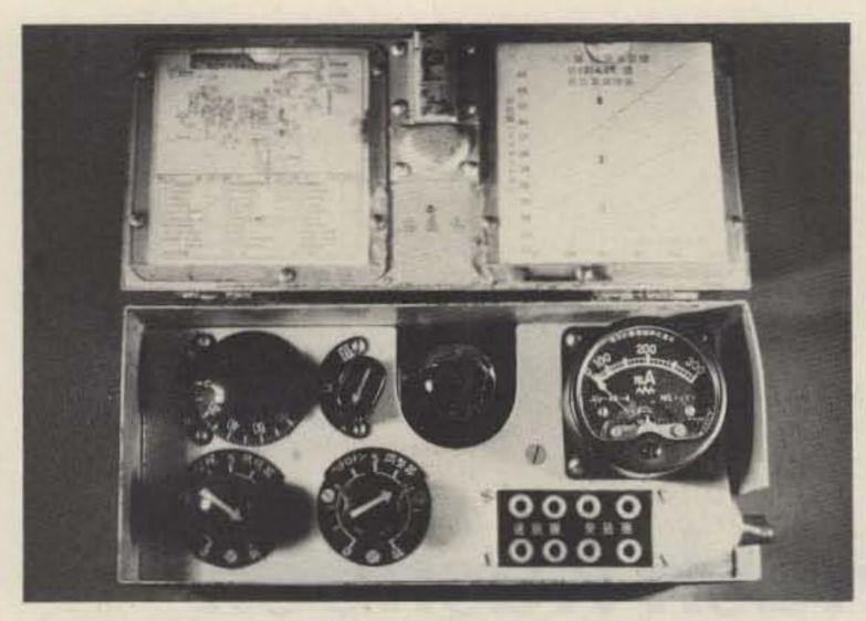
Photo B. Top view of the radio. Inside the lid are the circuit diagram and frequency calibration curves for the three ranges. On the radio, top row left to right: tuning capacitor C5 (see Fig. 4), frequency range switch S1, top of the tube, and antenna-current meter. Bottom: filament-current control R2, variable grid leak R1, and jacks for two handsets.
