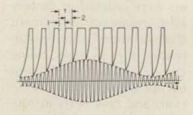
Fig. 3. Received signal, an amplitude-modulated carrier, and the variation of the rectified current through the tube. Starting from the amplitude of the recieved signal, the signal builds up during interval 1 and stays at the maximum level during interval 2. The sum of intervals 1 and 2 is t, the period of the quenching signal.
