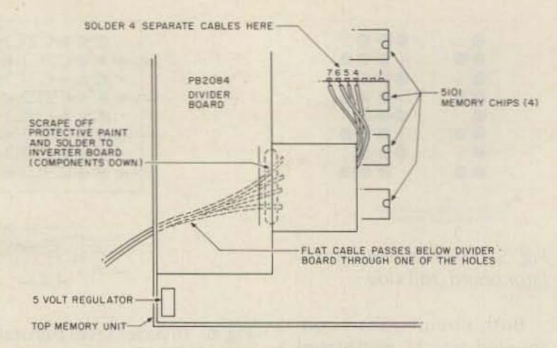
Fig. 8. Inverter board placement.
