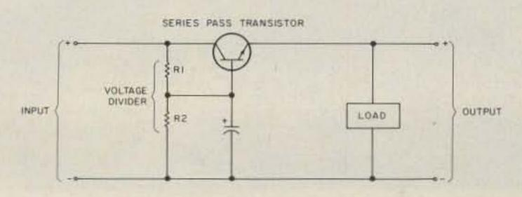
Fig. 1(b). Simplified hum-eliminator circuit.
