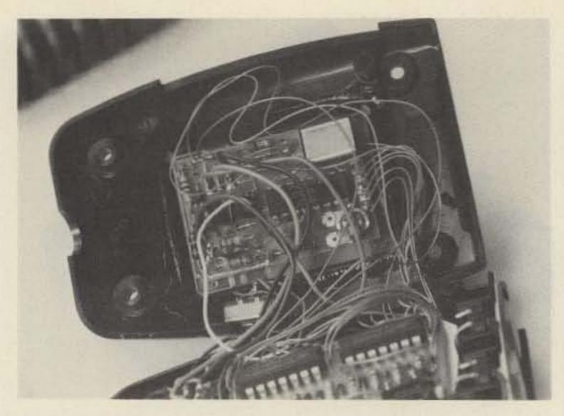
Photo D. In the older-style PCM-2000 microphone, the rowand-column leads are soldered to existing PC pads on the end of the DTMF board. The crystal must be bent up slightly while soldering. Use just a small amount of heat and do not disturb the existing wires which are poking through these pads from below the board.
