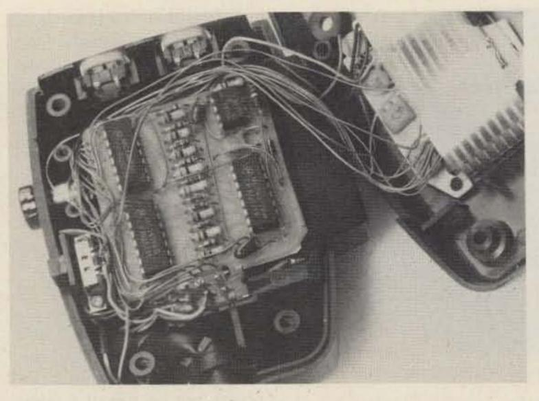
Photo F. When mounting the parts on the printed-circuit board, be sure to orient the three capacitors flat against the board—there is not enough room to allow them to mount vertically. The exact routing of the many connecting wires is not critical.
