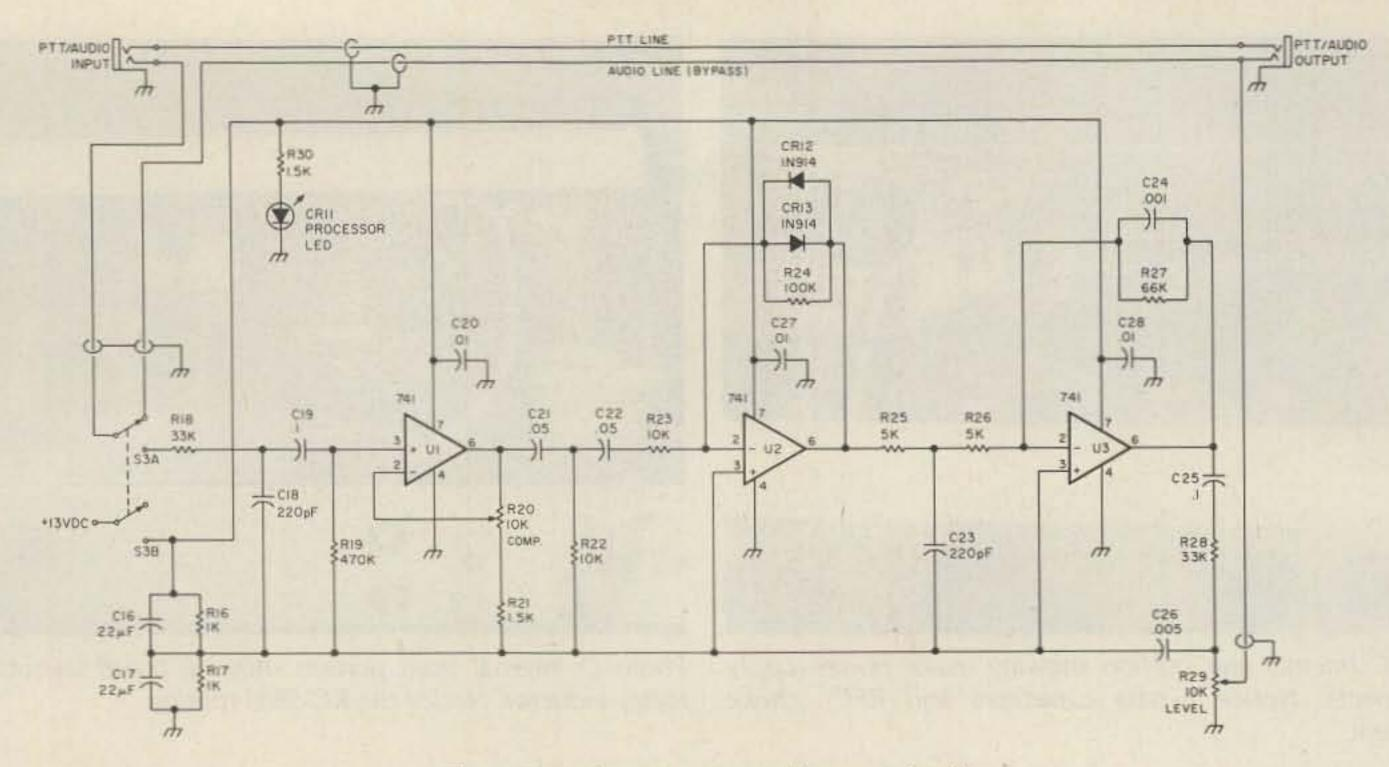
Fig. 3. Speech processor and bypass circuit.
