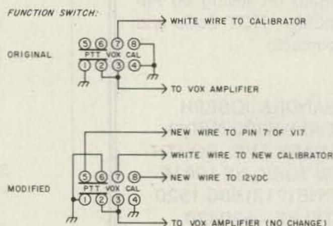
Fig. 1(b). Modified function switch.
