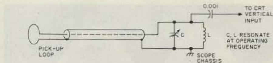
Fig. 5. Coupling rf to oscilloscope.
