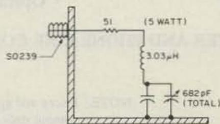
Fig. 3. Construction of special dummy load.
