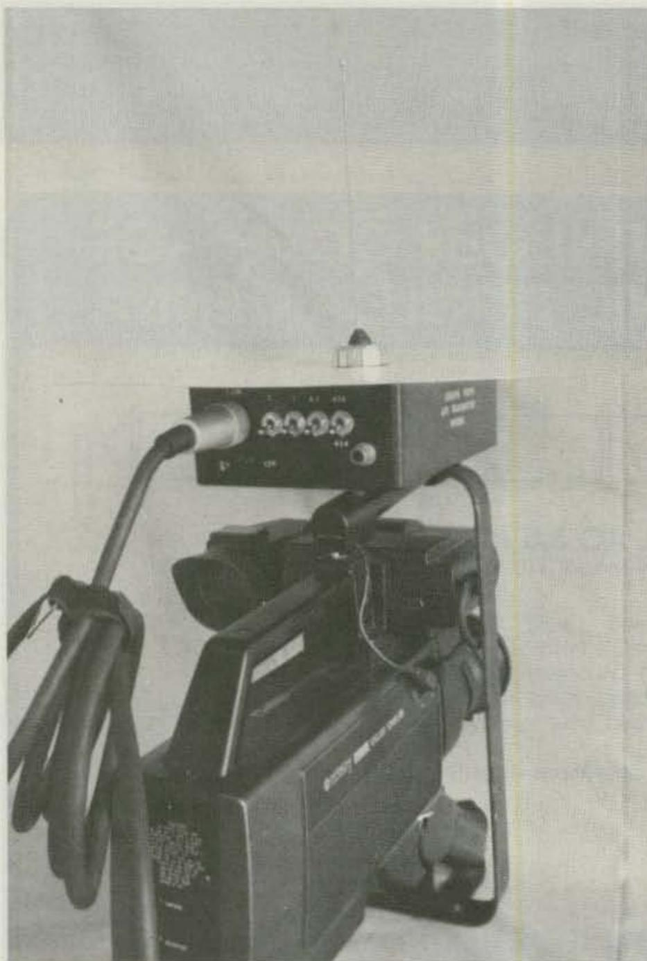
Photo A. Camera with transmitter in a Hammond #1590D housing. Also shown is the thirteen-inch ground-plane disc needed with most cameras for an rf shield. (Photo by P.C. Electronics)
