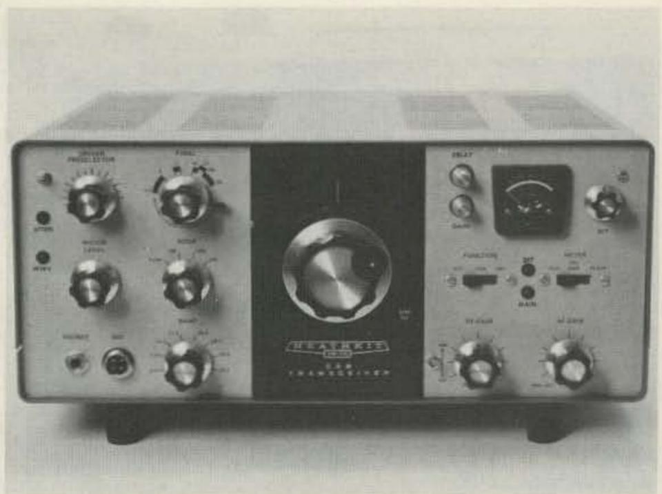
Photo A. The finished product with new controls, LED status indicators, and spinner knob.
