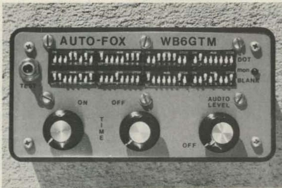
The Auto-Fox was built using point-to-point wiring on parts of a protoboard and put into a Radio Shack 270-233 experimenter's box. The top panel contains the callsign programming DIP switches, transmit speed, delay, and audio level/on-off pots, as well as the push-button switch which activates the monitor LED. The right side of the enclosure (not shown) has a subminiature mike jack, a miniature PTT jack, and an external power connector.
