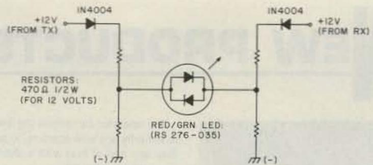
**TWO-WAY LED:** Here's a little bridge circuit that allows a front-panel LED to glow red or green from a switched positive voltage. Normally you would have to reverse the polarity across the LED, but this circuit does it for you. If your switched voltages are negative with respect to ground, simply reverse the diodes—Ron Johnson WA5RON, Austin TX.
