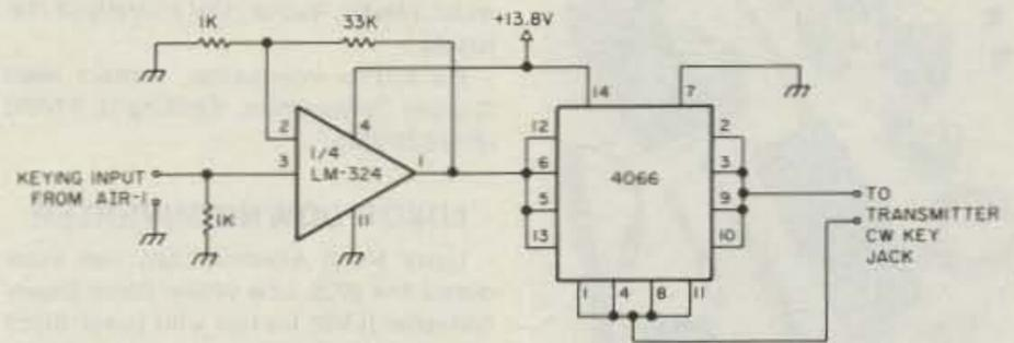
**COMPUTER-TO-RIG INTERFACE:** I needed a circuit to allow my VIC-20/AIR-1 to key an FT-707, which requires a set of closed contacts such as a straight key. The keying output of the AIR-1 is 0-0.6 V dc, which drives one quarter of an LM-324 op amp. The 13-V output of the LM-324 activates a CMOS switch, keying the rig. The four CMOS switch contacts are wired in parallel to reduce the "on" resistance.—Dave Ball WA4PQD, Barrington NH.
