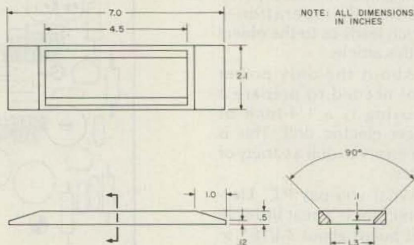
Fig. 3. Bezel dimensional drawing. This is an optional item which can be added at any time. Its basic purpose is to act as a switch guard, but it also improves the appearance.
