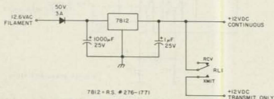
Fig. 7. Regulated power supply for modifications. Don't overlook the 1-µF capacitor at the 7812 output.
