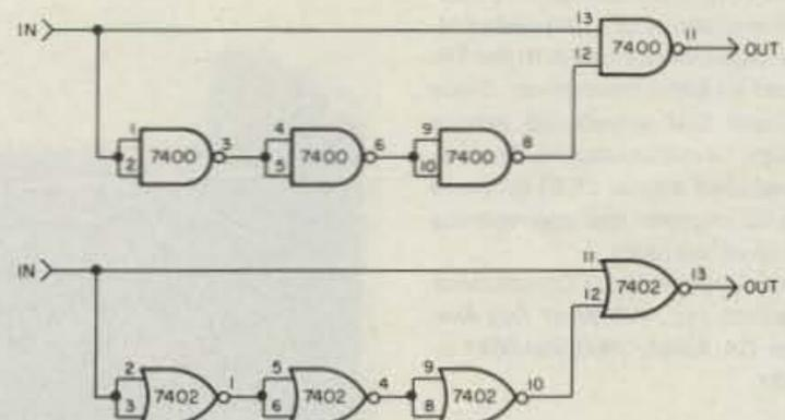
**TWO-WAY EDGE DETECTION:** When you need an edge-detector for a positive- or a negative-going change and don't want to use a one-shot, try this circuit. Using NAND gates will yield a single LOW pulse when the input goes from LOW to HIGH. Using NOR gates, a single HIGH pulse is generated when the input switches from HIGH to LOW. Any odd number of gates can be used in the delay leg feeding the final gate. The more delay gates used, the longer the output pulse.—Paul Selwa N9CZK, Brownsburg IN.
