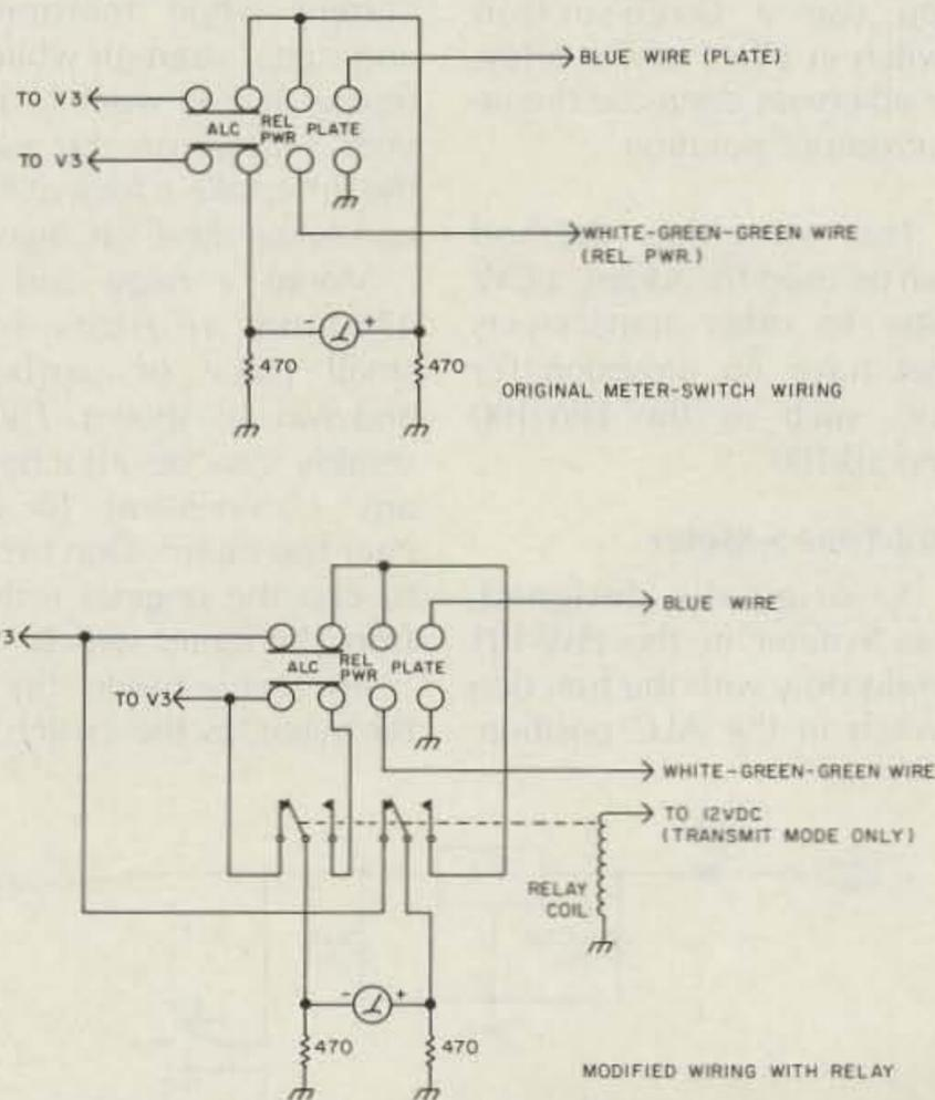
Fig. 6. The new relay makes the S-meter independent of the meter switch. Observe meter polarity when connecting relay to switch.
