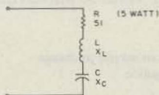
Fig. 2. Special dummy load.
