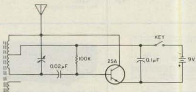
Fig. 1. The original rf oscillator circuit.
