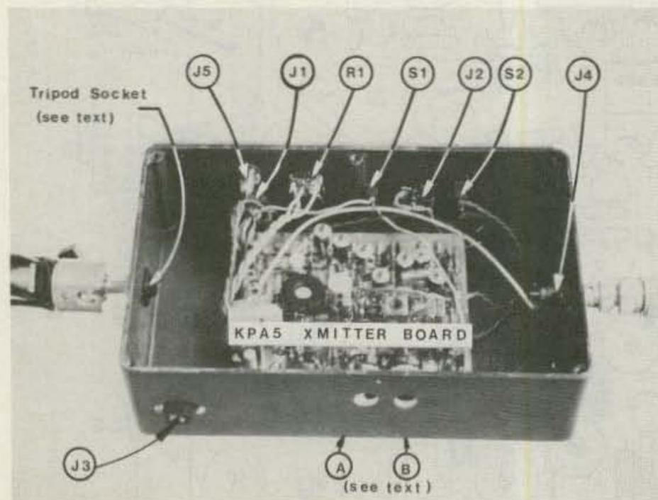
Fig. 2. A middle-of-the-road approach to packaging the transmitter board. Video-level control is brought out to the panel as are connector jacks and switches. Audio levels are screwdriver-adjusted through access holes A and B.
