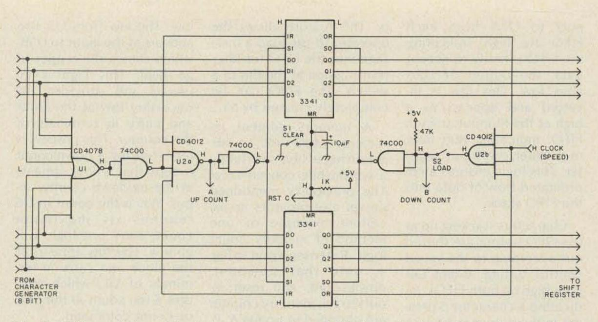
Fig. 4. FIFO parallel stacking to accommodate an 8-bit character. Logic indicated is with circuit at rest.
