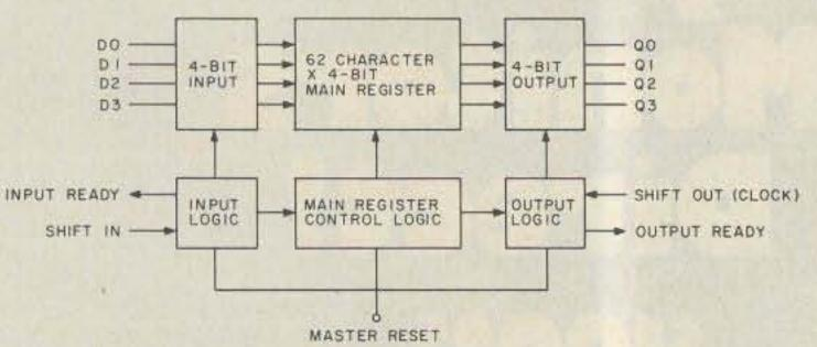
Fig. 1. The Fairchild 3341 MOS FIFO buffer block diagram.
