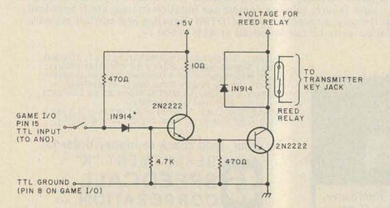
Fig. 1. No parts values are critical. \*Any small switching diode can be used.
