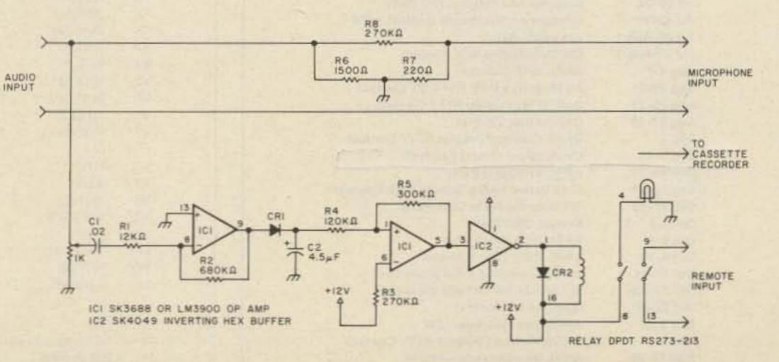
AUTOMATIC TAPE RECORDING: Don't miss the action while you're away from the rig. This circuit turns on a tape recorder whenever the receiver's squelch is broken. After signal loss, the recorder will shut off following a slight delay.—Gary Anderson KE7H, Nampa ID.
