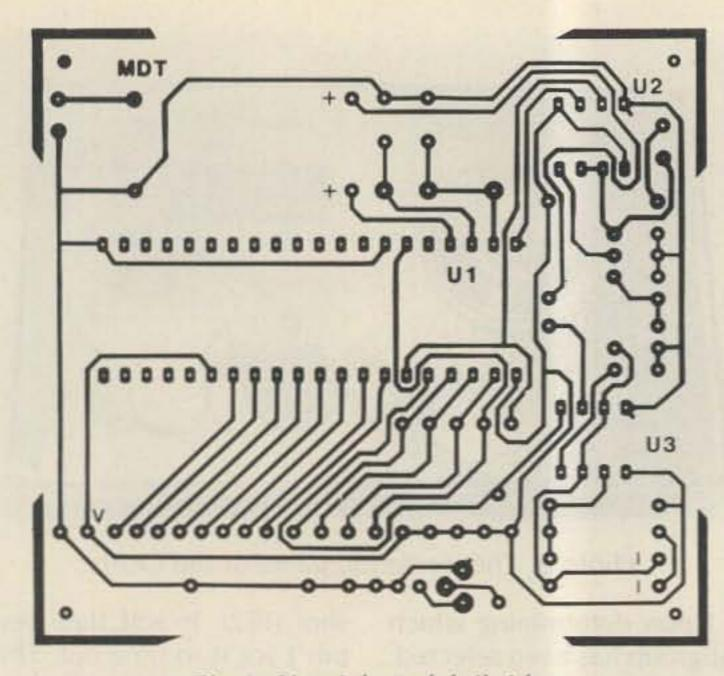
Fig. 3. Circuit board, foil side.
