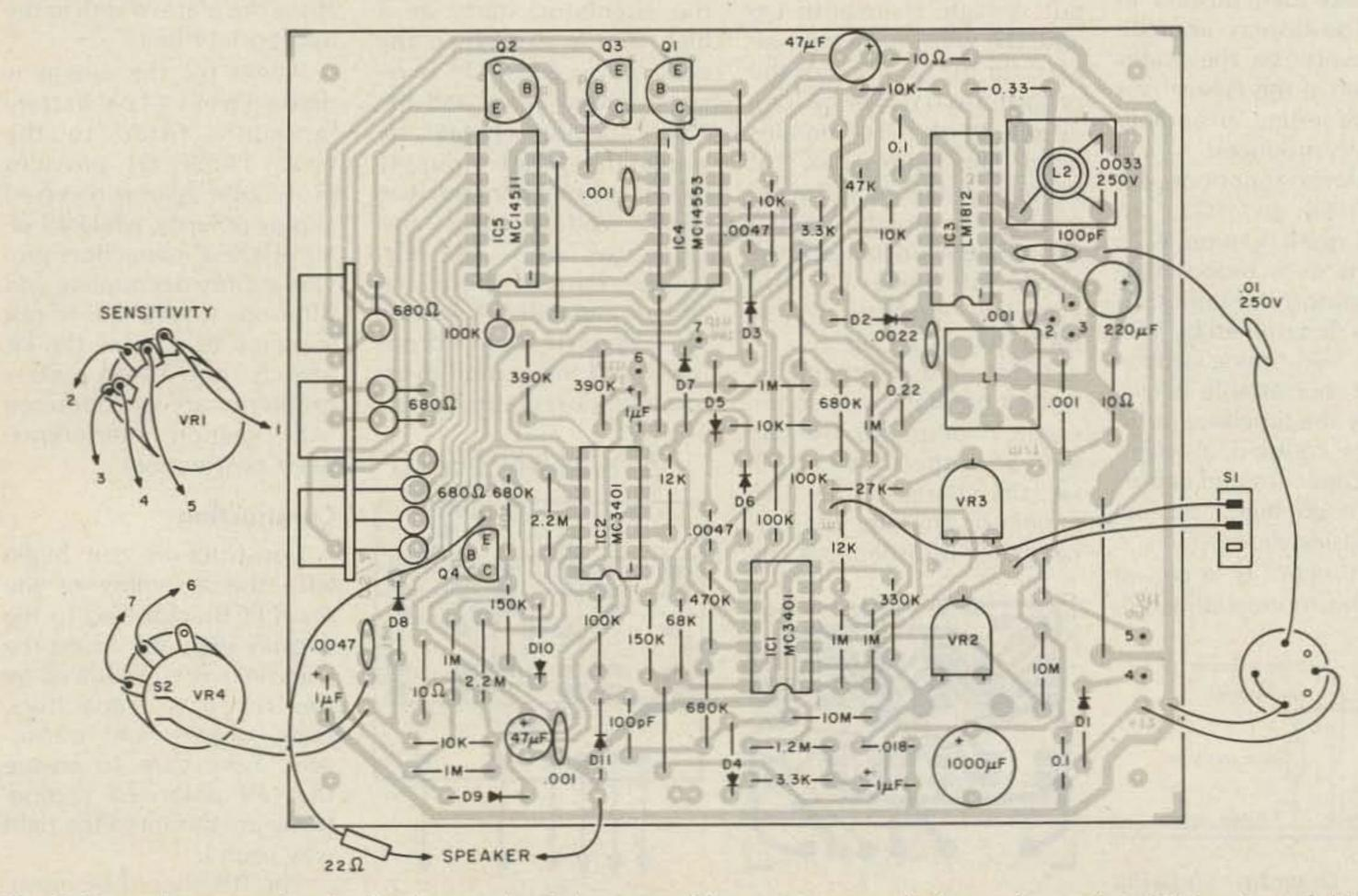
Fig. 4. Parts placement for the depth sounder. Take care with component polarity, and note that IC4 is oriented differently than the other ICs.
