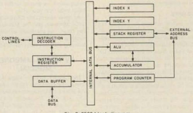
Fig. 3. 6502 block diagram.
