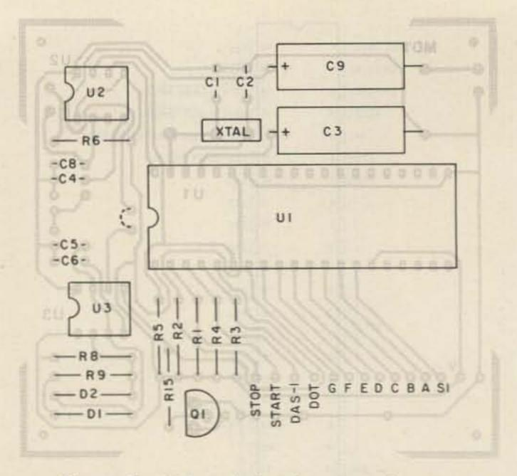
Fig. 4. Circuit board showing parts placement.
