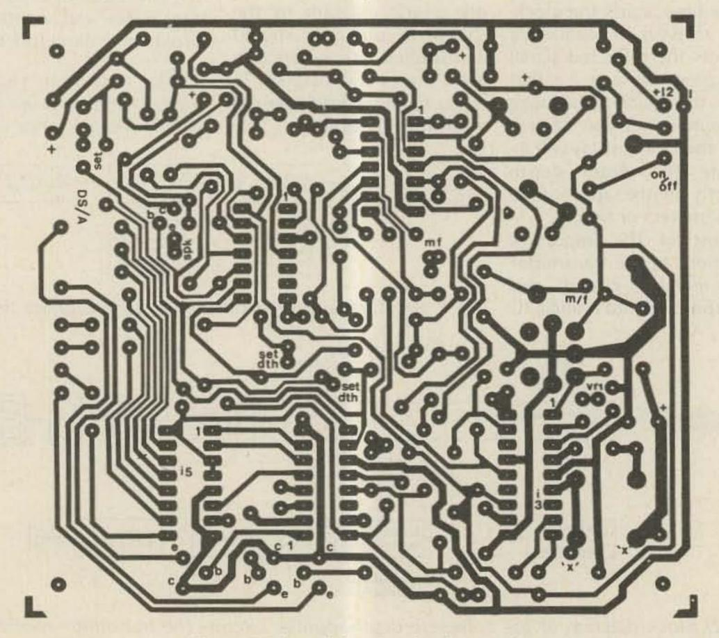
Fig. 3. PC board for the depth sounder.
