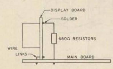
Fig. 5. Diagram showing how four of the 680-Ohm resistors are mounted.
