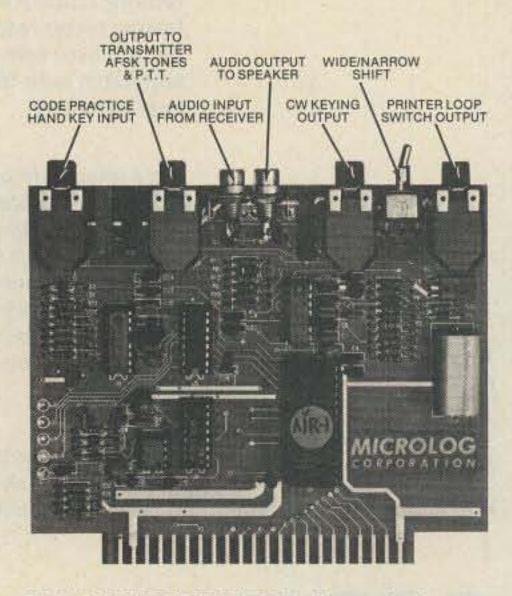
RTTY DEMODULATOR: True dual tone computer enhanced demodulator circuit on standard 2125/2295 Hz tone pair compatible with HF RTTY and VHF FM operation. Switch selected wide and narrow shift.
