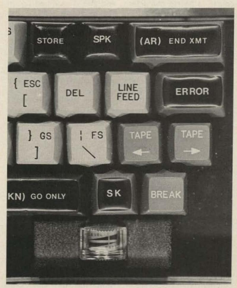
Photo D. Keytops and meter (black keys have new tops). 73 Magazine • July, 1983 59
