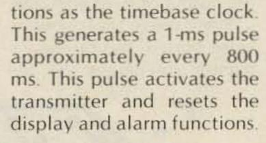
IC1a, part of an MC3401 quad op amp, is wired as an astable multivibrator which
