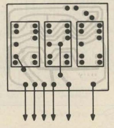
Fig. 7. Parts placement for the display PCB.
