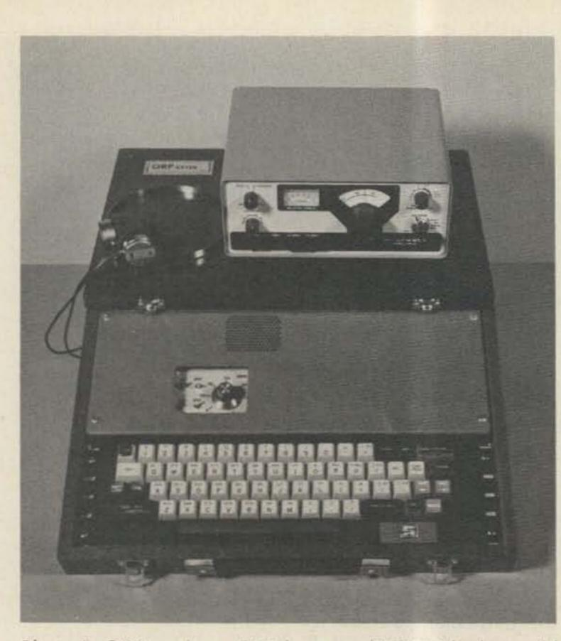
Photo E. QRP station – QRP keyer and HW-8 (the keyer lid was removed to make a base for the transceiver).
