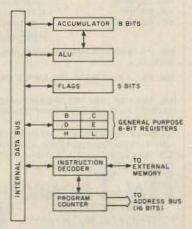
Fig. 1. 8080 block diagram. 73 Magazine • July, 1983 107
