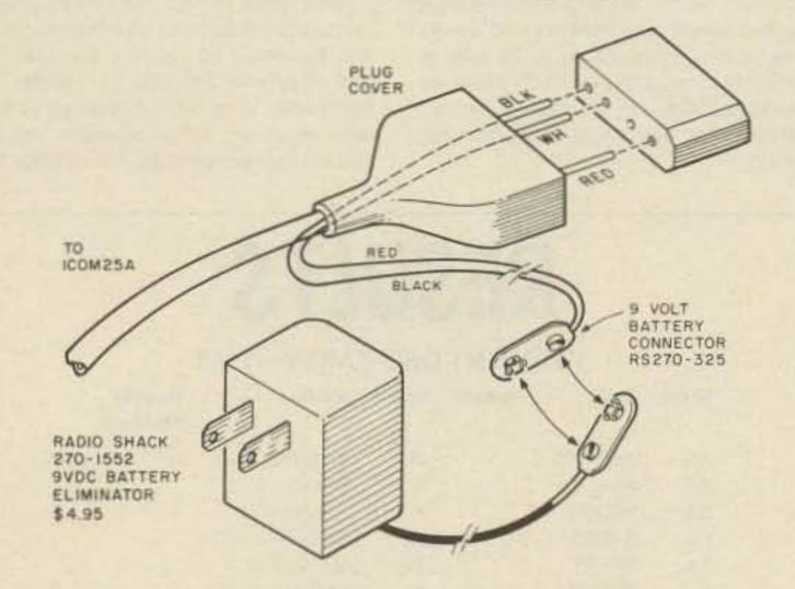
MEMORY BACKUP FOR THE ICOM 25A: To retain the memory in the Icom 25A when the power is disconnected, slip back the cover of the power plug and wire a 9-V battery connector to the white (positive) and black (negative) leads. When removing the
