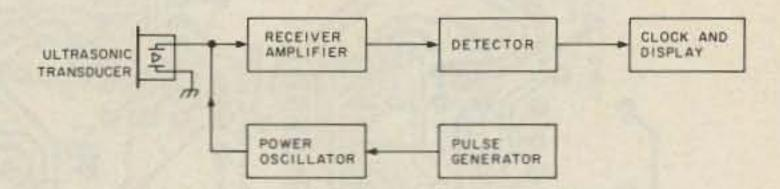
Fig. 1. Basic scheme for an ultrasonic depth-sounder circuit.
