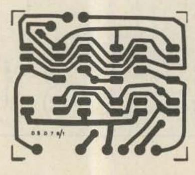
Fig. 6. PC board for the display.
