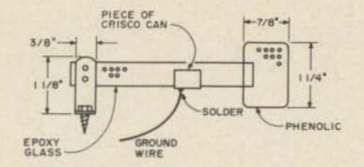
Fig. 3. Details of paddle-arm assembly.
