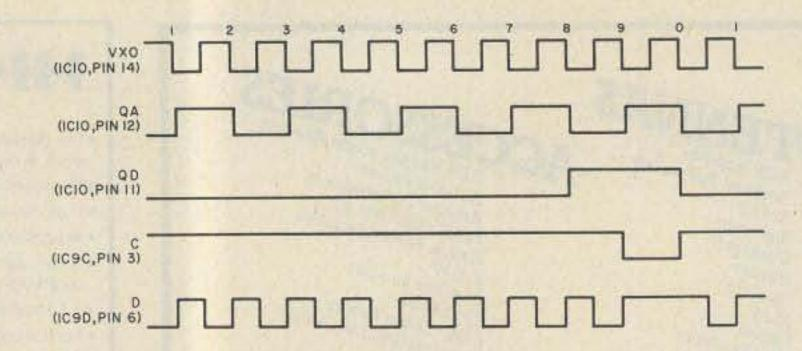
Fig. 4. Operation of the divide-by-1.111 ... module as explained in the text.
