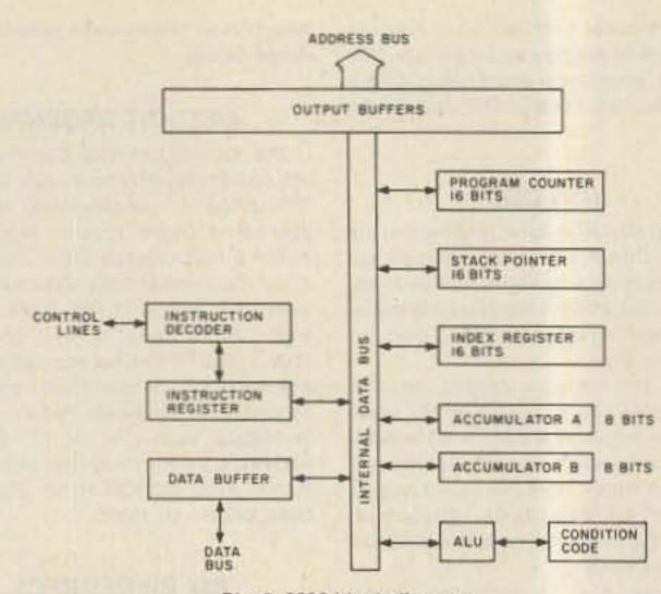
Fig. 2. 6800 block diagram.
