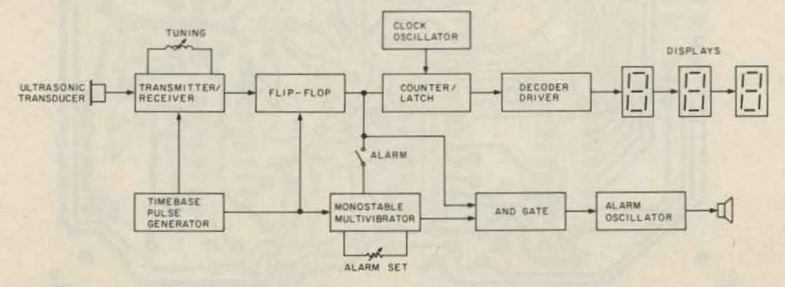
Fig. 2. Block diagram of the complete depth-sounder circuit. The transmitter/receiver is based on a single IC.
