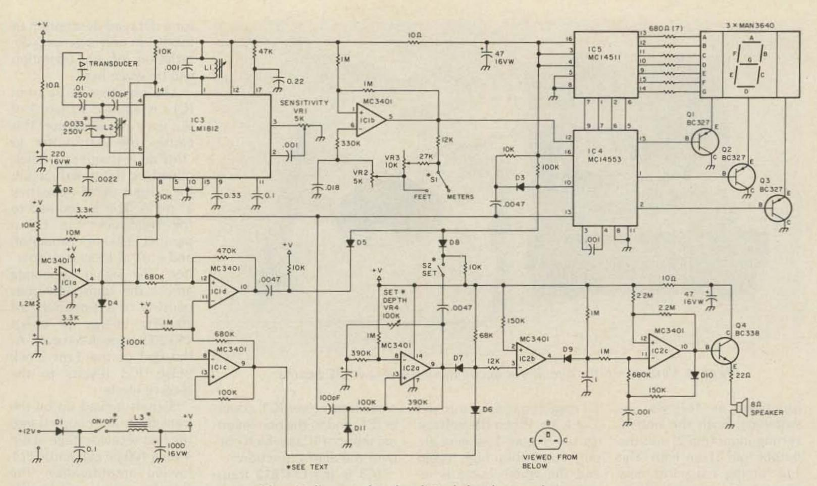
Circuit diagram for the digital depth sounder.
