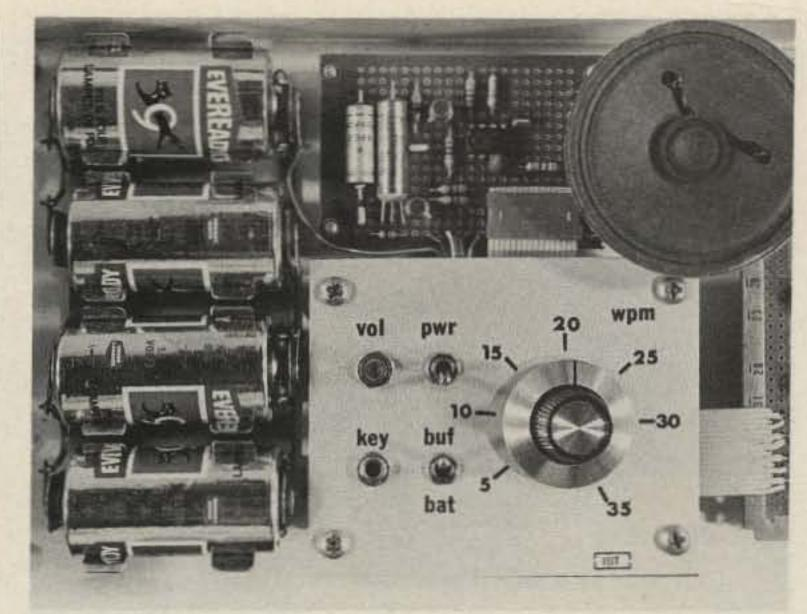
Photo C. Control panel, speaker, batteries, and sidetone/ relay board.
