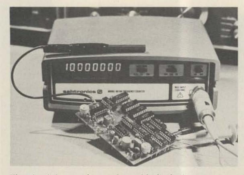
The circuit in actual operation, with the ferrite antenna on top of the counter. Output frequency is 10 MHz, phaselocked to a selectable AM-broadcast station. tual accuracy due to the aging process in the crystal—and they cost 50 dollars or more.
