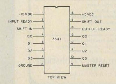
Fig. 3. 3341 connection diagram.
