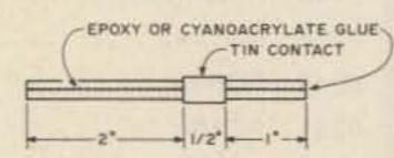
Fig. 1. Paddle construction. Clamp glued ends together until cement has cured. Use same technique for tin-plate ground contact.
