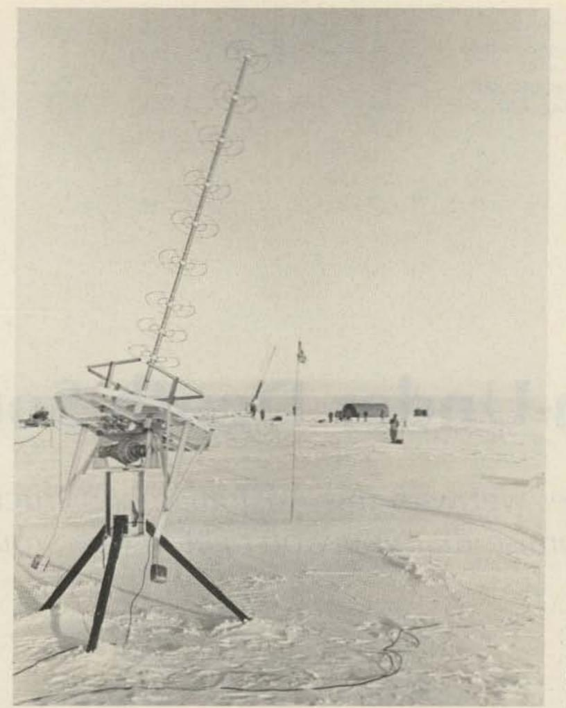
The P-Band antenna at Siple Station, Antarctica, is used to receive data from Nike-Tomahawk rockets launched into the magnetosphere (US Navy photograph).
