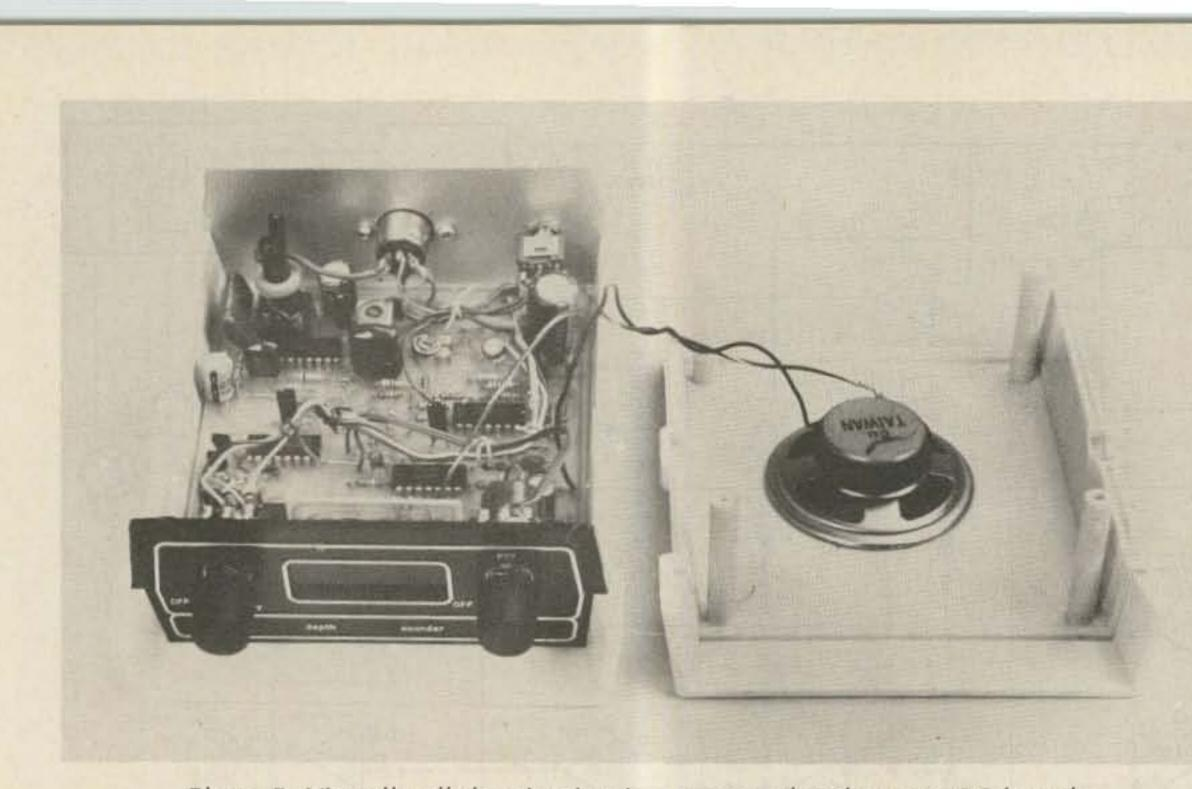
Photo B. Virtually all the circuitry is accommodated on two PC boards.
