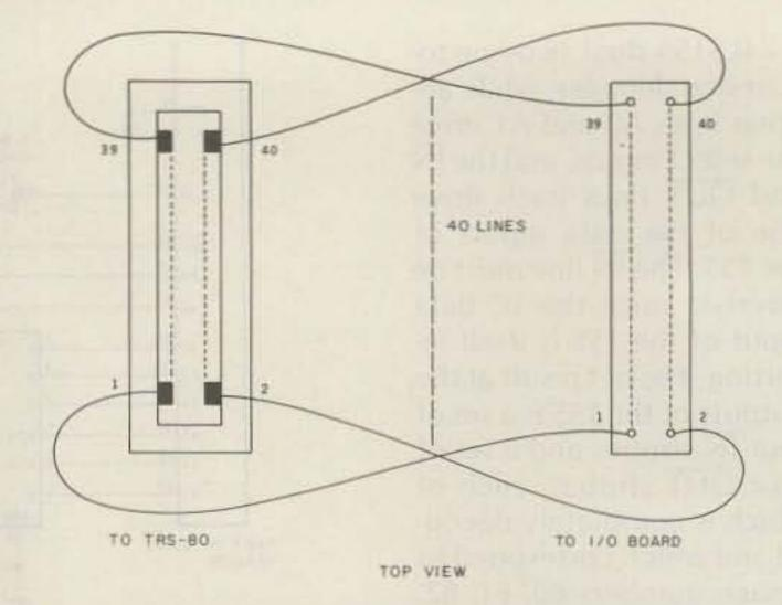
Fig. 4. Schematic of interface connector. Viewed from the rear of the TRS-80, pin 1 is the upper-left finger and pin 40 is the lower-right finger on the PC board.
