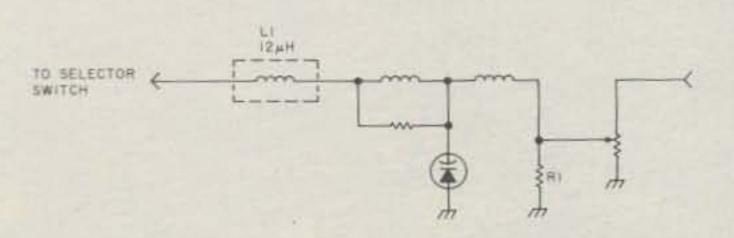
Fig. 1. SBE-12CB clarifier circuit. L1 is added to extend range to 15 kHz. R1 is 1-4k Ohms and controls linearity. All other components are existing.
