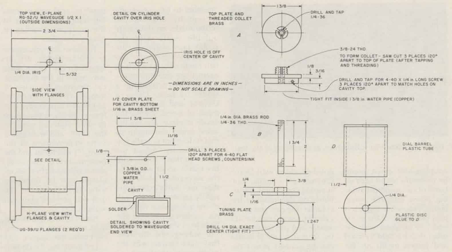
Fig. 3. Construction details for cavity wavemeter.
