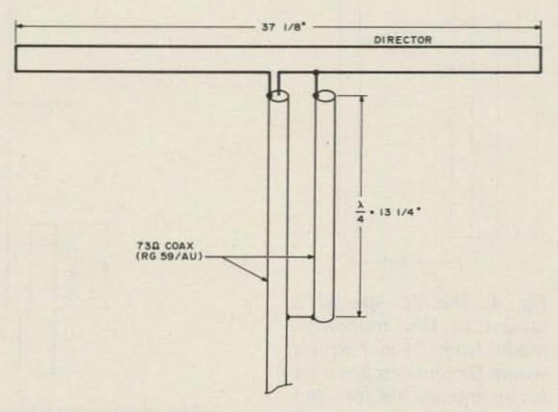
Fig. 3. Dimensions given for the 1-to-1 balun are for 146.5 MHz using coax with a velocity factor of .66. For other frequencies, balun length in inches is calculated from 2952 × .66 ÷ MHz.
