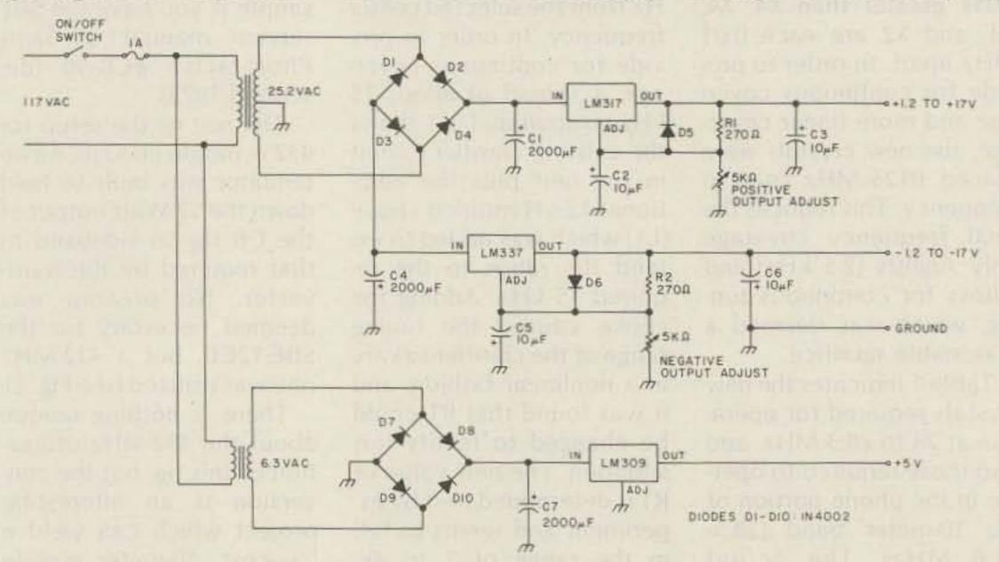
Fig. 1. Tri-voltage power supply schematic.
