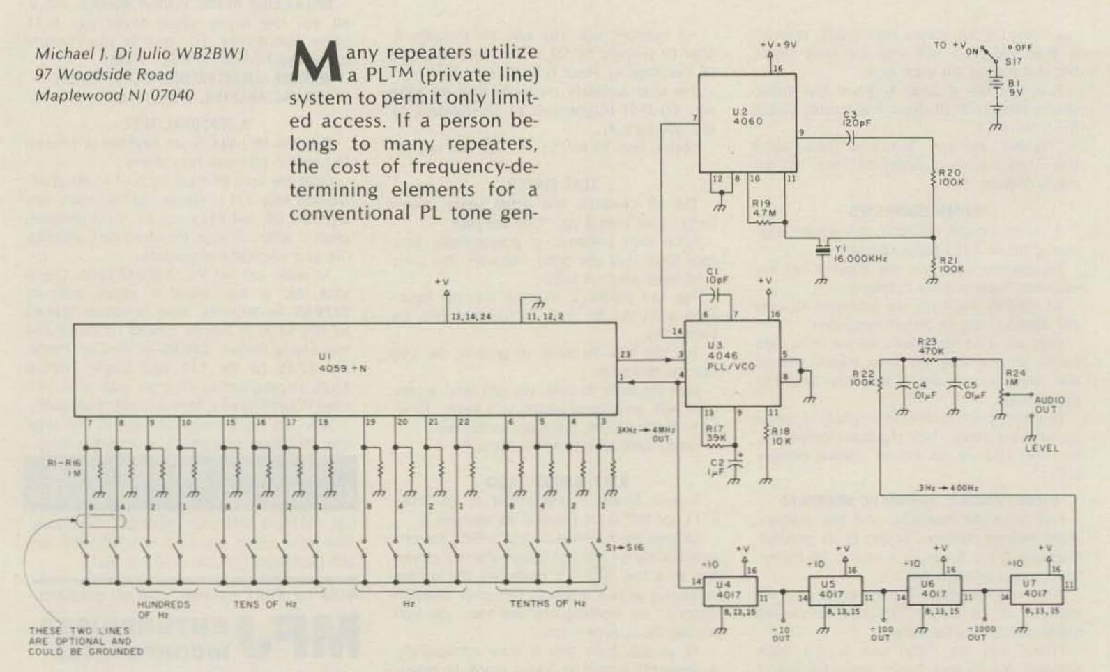
Fig. 1. Synthesized tone generator schematic.
