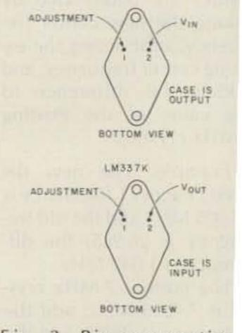
Fig. 2. Pin connection for the LM309, LM31 and LM337 voltage reg lators (TO-3 packages).
