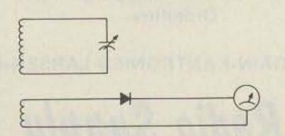
Fig. 1. Parallel resonant equivalent circuit of wavemeter.
