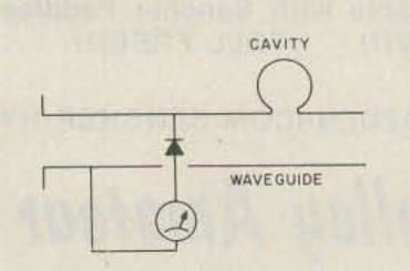
Fig. 2. Cavity wavemeter circuit diagram.
