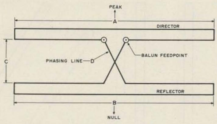
Fig. 2. The ZL Special is composed of two phased driven folded dipoles made from 300-Ohm twinlead. The driven director is 4.4% shorter than a half-wave element and the reflector 1.7% longer. Formulas for dimensions in inches: A = 5446 ÷ MHz; B = 5794 ÷ MHz; C = 1266 ÷ MHz; D = 1266 ÷ MHz. Dimensions for 146.5 MHz are: A = 37-1/8"; B = 39-1/2"; C = 8-5/8"; D = 8-5/8".
