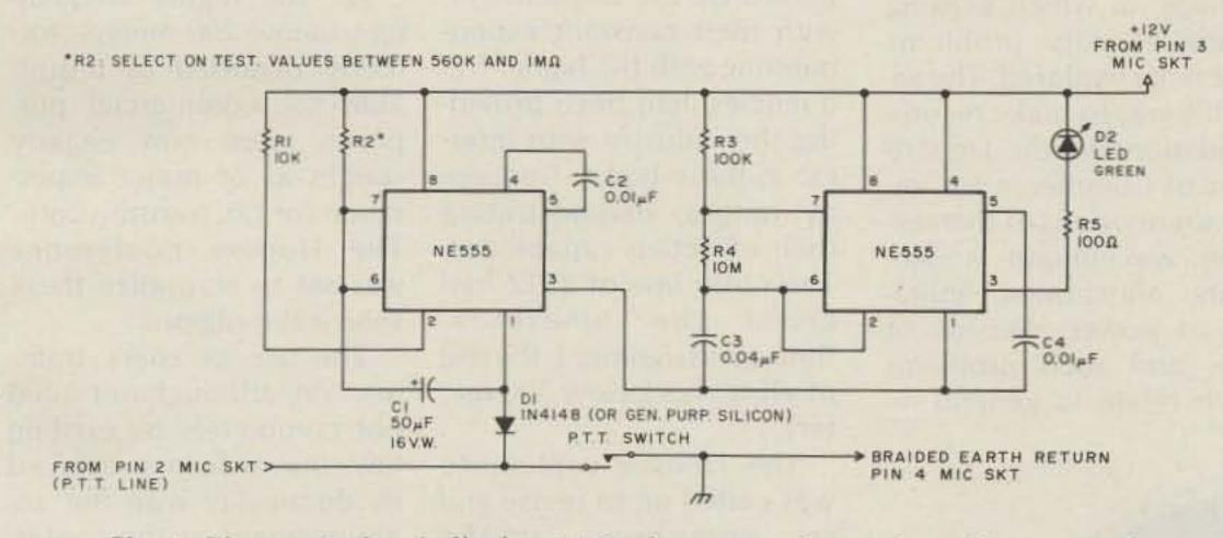
Fig. 1. Time-out circuit flashes LED after one minute, forty-five seconds.
