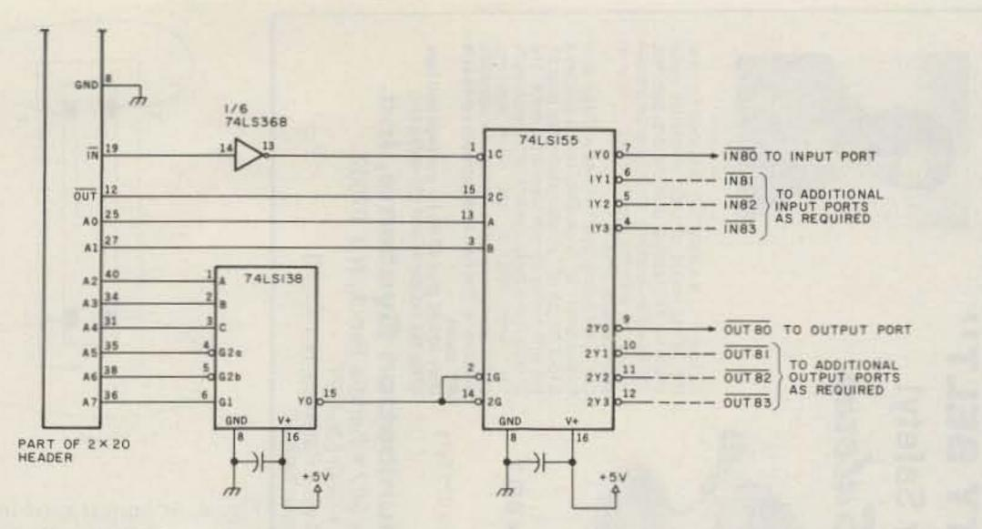
Fig. 1. Schematic of strobe generator circuit. Unmarked capacitors are 0.1-uF, 25-volt disc ceramic.
