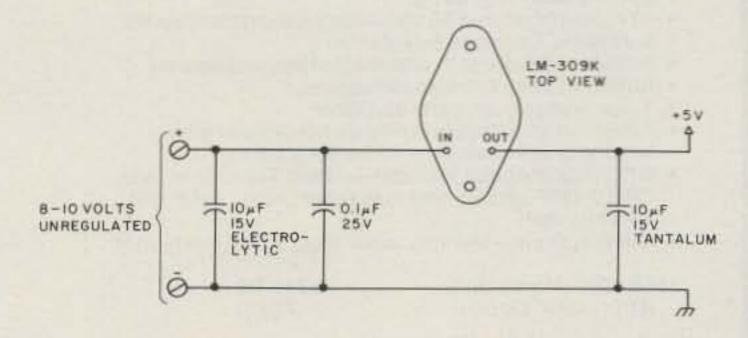
Fig. 3. Schematic of power-supply regulator. The 10-uF capacitors are tantalum and electrolytic; the 0.1-uF capacitor is disc ceramic.
