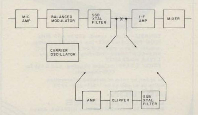
Fig. 4. Rf clipping can be added to most SSB transceivers by breaking the i-f chain after the SSB filter and adding the stages shown.
