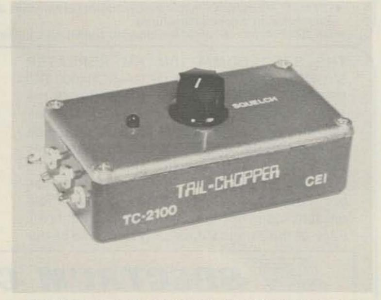
Tail-Chopper squelch-tail eliminator from Circuit Electronics.
