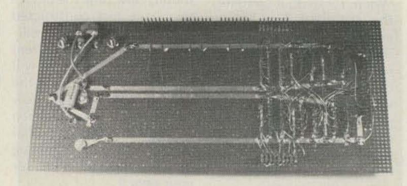
Photo B. Bottom view of the I/O board. The 2 × 20 header is at the right. The electrolytic and ceramic capacitors for the regulator circuit are at the left. Power buses are 1/8"-wide adhesive copper strips made by Circuit-StikTM. Small white spots are paint used to mark correct positions for the sockets and headers. Terminating resistors (input port) were added after the photograph was taken.
