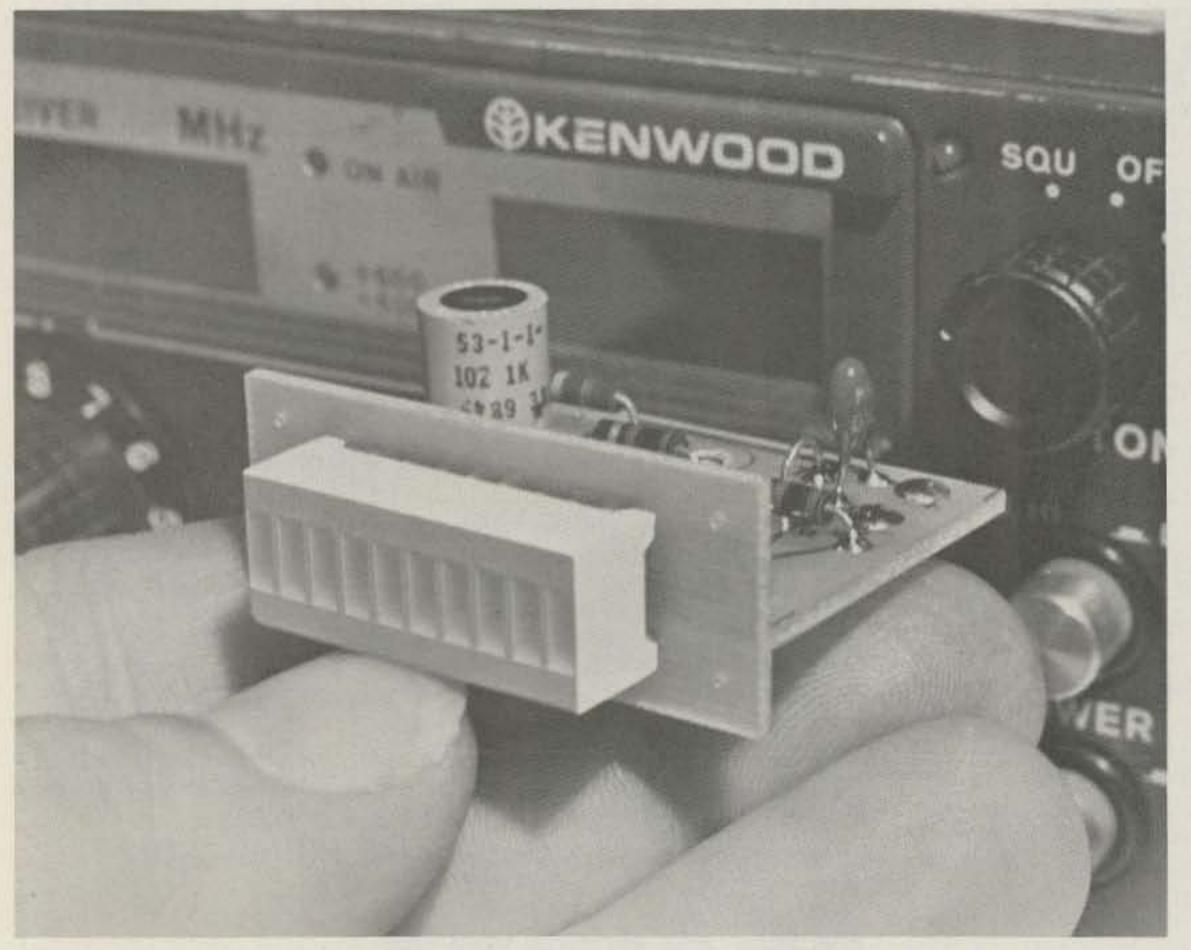
Photo A. Completed unit ready for installation. Note the two-board construction.
