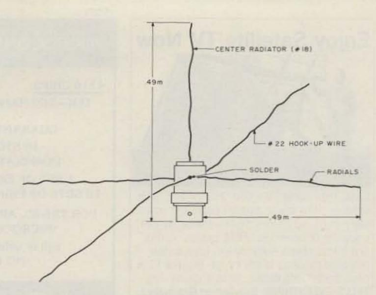
Fig. 1. The Flexi-Plane with BNC connector.
