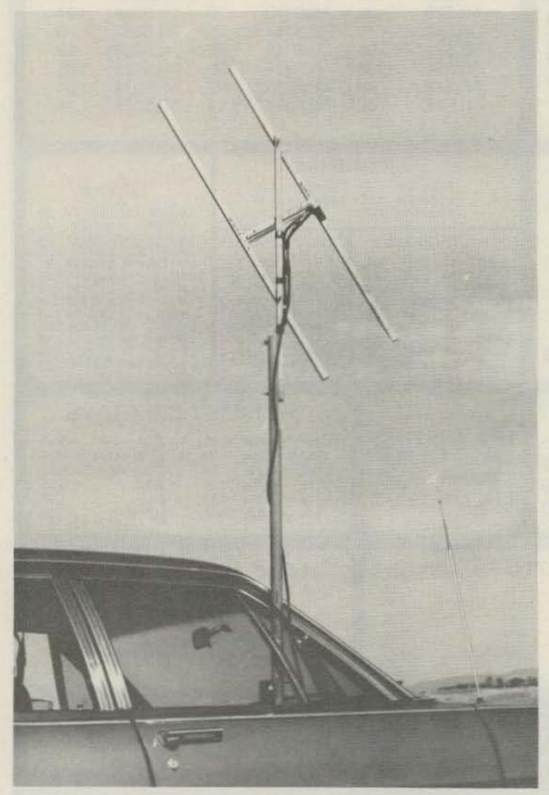
The completed antenna is mounted through the wind-wing of a car.
