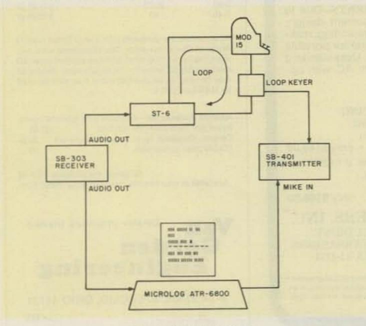
Fig. 1. Station wiring.
