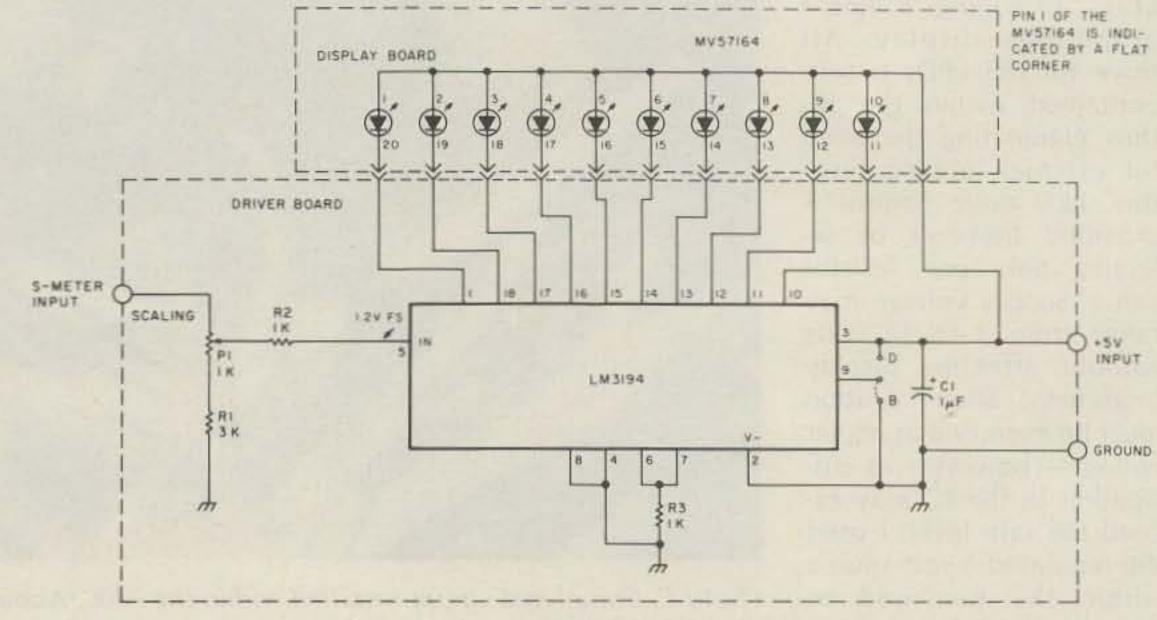
Fig. 1. Schematic of bar-graph S-meter.
