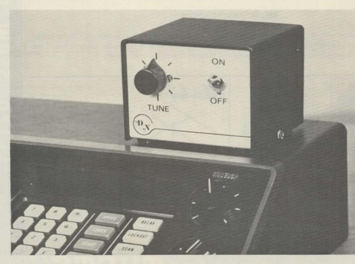
Photo A. The D-12 scramble decoder shown working here with a Bearcat 210 scanner.
