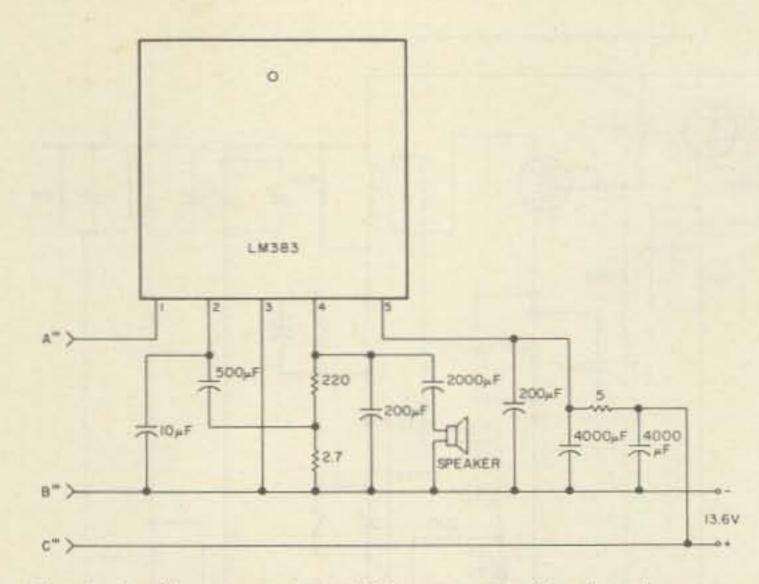
Fig. 4. Audio power amplifier uses Radio Shack LM383.
