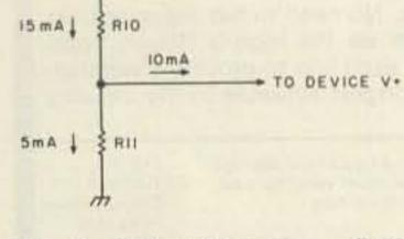
Fig. 1. 510 V/15 mA = R10 + R11 = 34k. R10 = (510 volts - 10 volts)/15 mA  $\approx$ 33k; R11 = 34k - 33k = 1k. Therefore, R10 = 33k and R11 = 1k.
