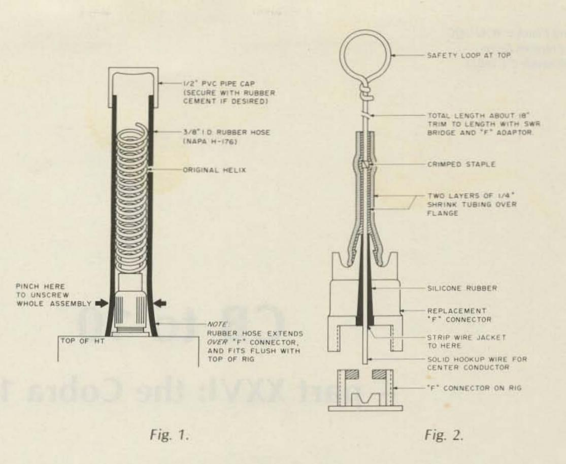
resulting antenna can be rolled up to about the size of a stick of gum (see Photo B) and tucked away in a corner of the HT case until needed. Performance is dramatically better than with the rubber ducky, and the antenna can easily be taped to a bus or train window for operating while traveling. Cost is negligible; the connectors come in packs of two for 59¢ or so at stores like Radio Shack.
