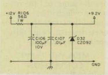
Fig. 6(a). Original regulator circuit.
