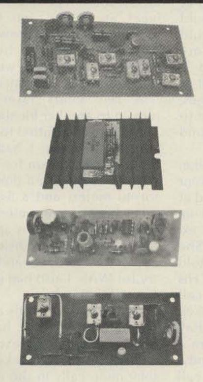
TXA5-3 ATV EXCITER/MODULATOR ..... \$85 ppd This wired and tested module is designed to drive the Motorola MHW-710 module in the PA5 10 watt linear amp. The crystal in the 100 mHz region keeps harmonics out of two meters for talk back. The video modulator is full 8 mHz for computer graphics and color. Requires 13.8 vdc reg @ 70 ma. Tuned with xtal on 439.25, 434.0, or 426.25 mHz. Two Freq version add \$30.
