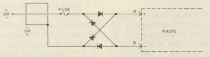
Fig. 3. Depolarizing circuit. Diodes should have a current rating greater than the fuse value.
