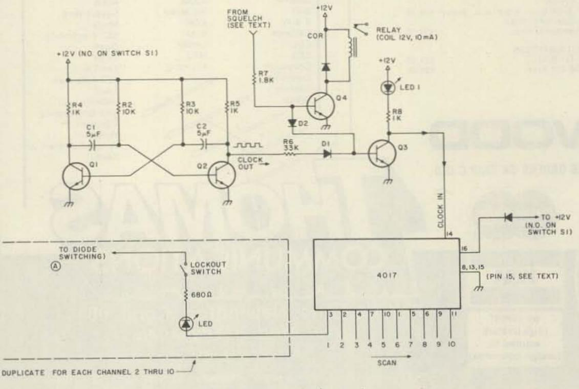
Fig. 2. Scanner schematic.
