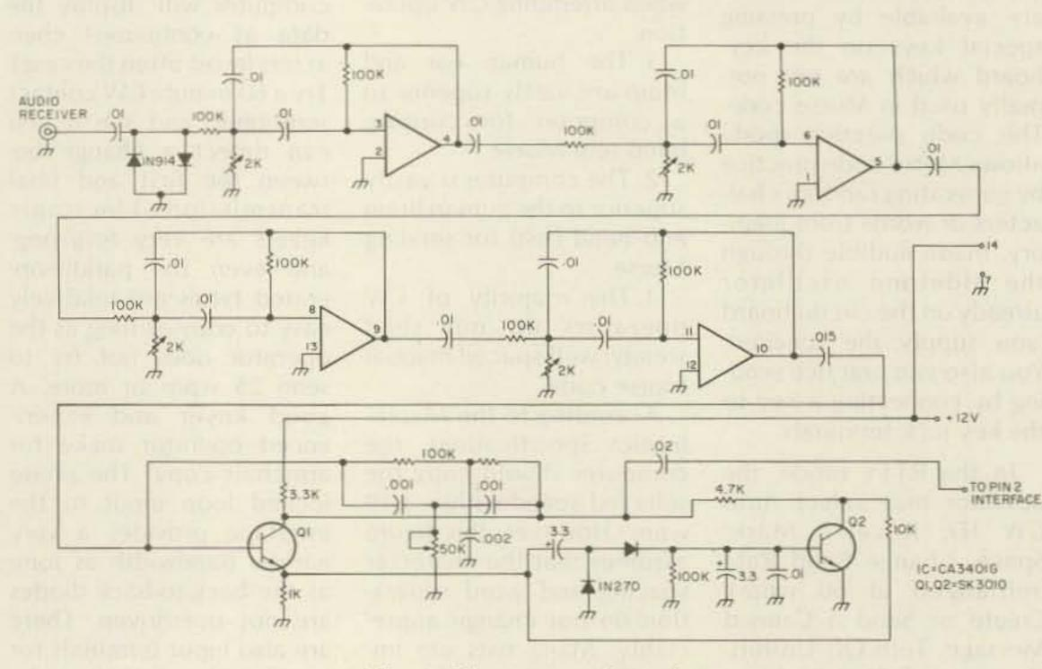
Fig. 3. Filter/amp schematic.
