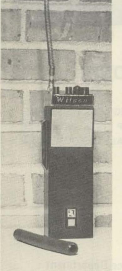
Photo A. Before. The beatup rubber ducky before installing the replacement covering.
