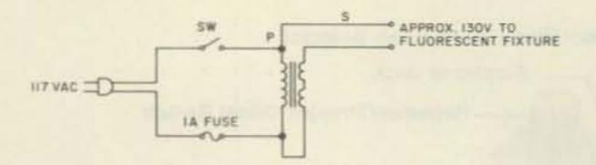
Fig. 1. The transformer can be any spare transformer that will supply approximately 10 to 12 volts ac. This can be accomplished by using a single winding, or by using two windings in series, such as 6.3 and 6.3 volts. In order to "add up," the windings must be properly polarized. Otherwise, a lowered voltage will result. was in the middle of a DX contest, and the stores were closed for most of the contest weekend.
