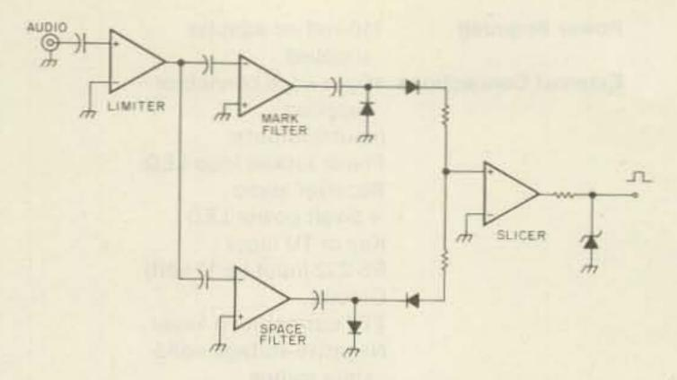
Fig. 2. RTTY terminal unit.
