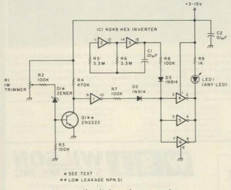
Fig. 2. Pilot light/voltage monitor.
