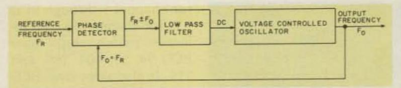
Fig. 1. Block diagram of a simple phase-locked loop.
