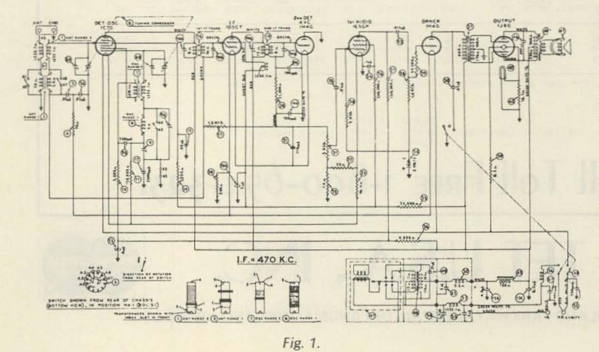
As shown, the original converter tube was replaced by two transistors, one as the "first detector" (as we used to call them) and the other as the local oscillator. The original coils, padders, trimmers, and variable capacitors were used without modification. And that created a problem!
