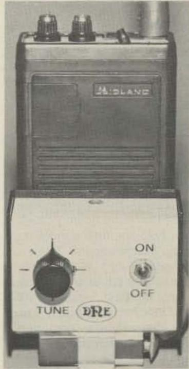
The descrambler is powered by a standard nine-volt transistor radio battery which is held to the back of the decoder cabinet by a small spring clamp. A three-conductor cable protrudes from the back of the cabinet to allow attach-
