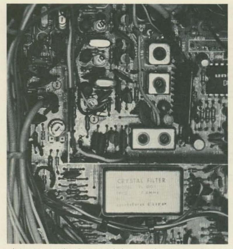
Photo E. Details of some of the President Grant changes show here. Arrow #1 points to L13, #2 to L12, and #3 to where jumper JP11 was located originally. D38 is located between L12 and the shield.
