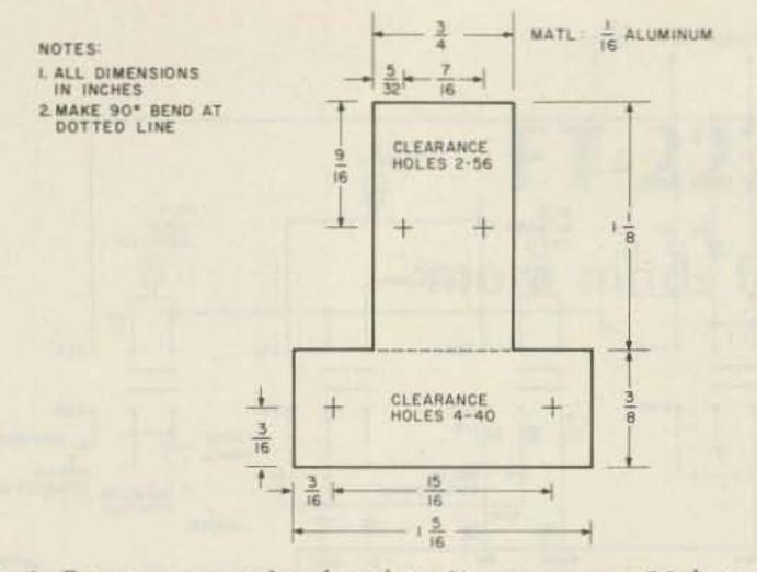
Fig. 6. Battery mounting bracket. Keystone no. 93 battery clip required.
