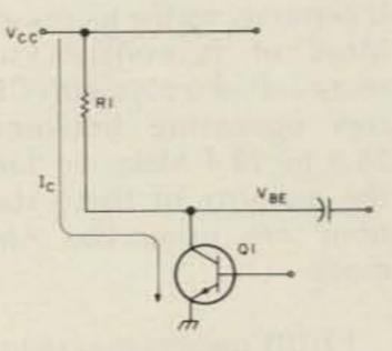
Fig. 6. Too much current through R1 when Q1 is conducting will blow Q1.
