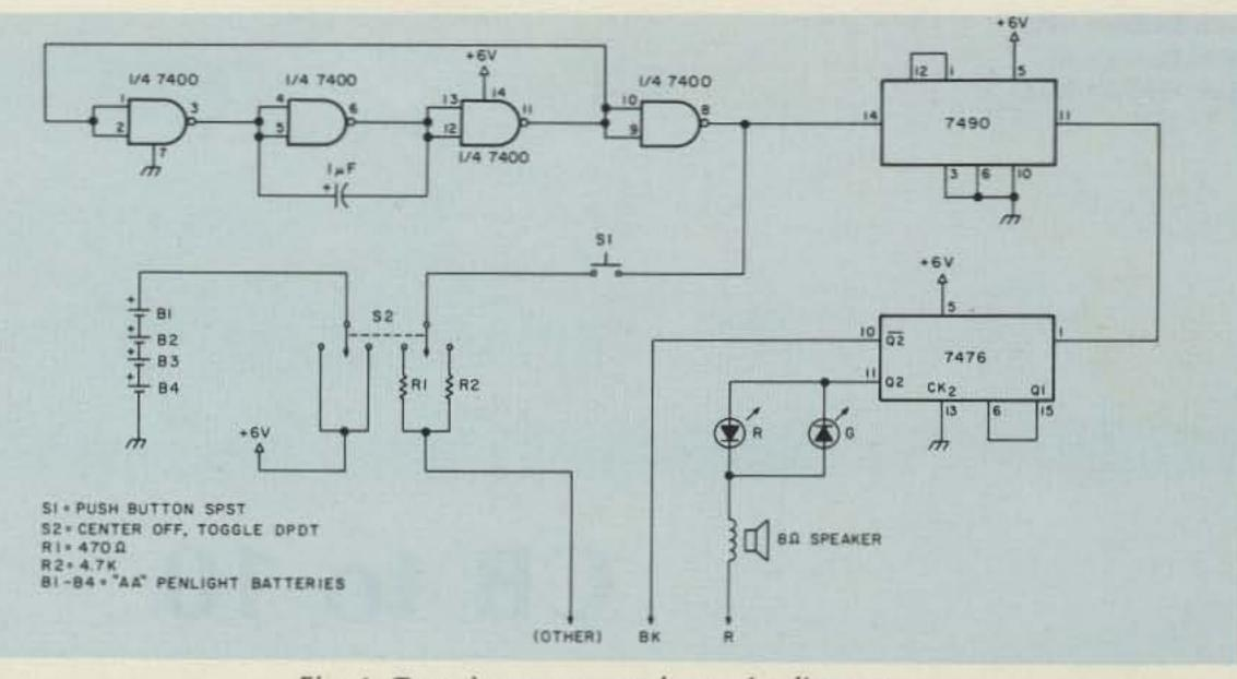
Fig. 1. Transistor tester schematic diagram.
