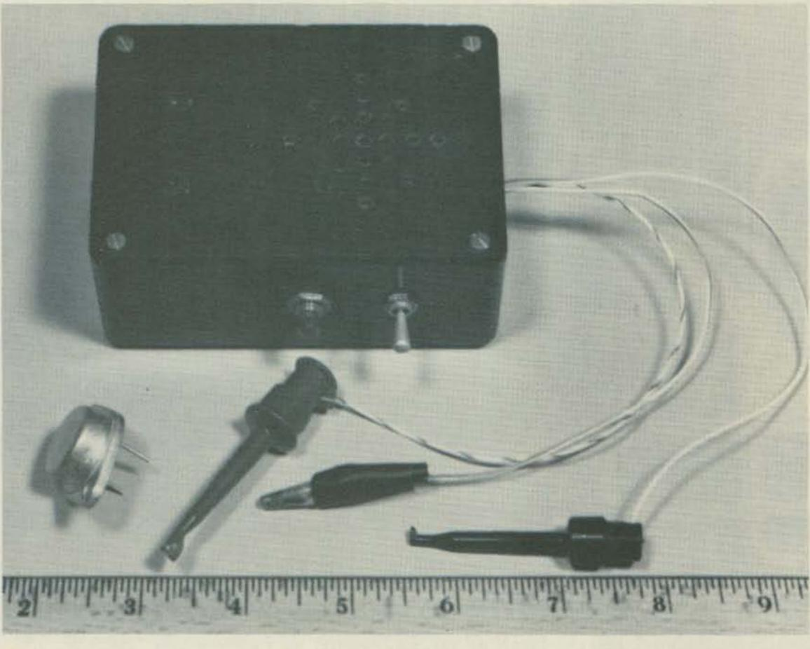
The finished transistor tester.
