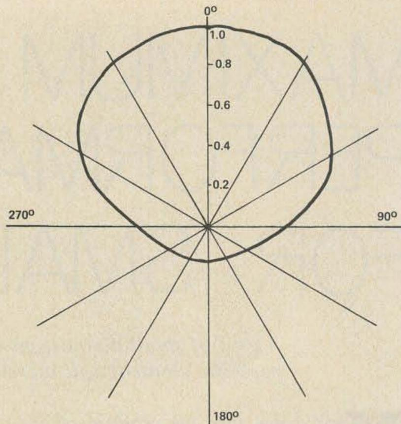
Fig. 3. Typical horizontal radiation pattern.
