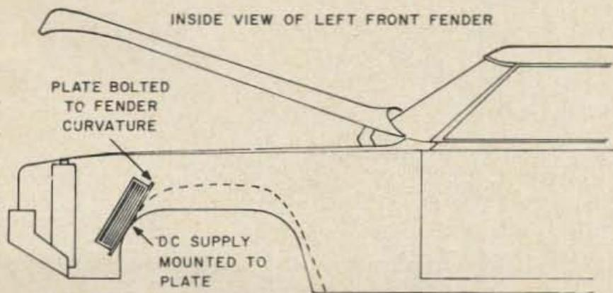
Fig. 1. Power supply mounted against metal car body for maximum heatsinking.
