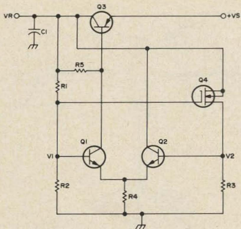
Fig.3. MOSFET improves power supply regulator.
