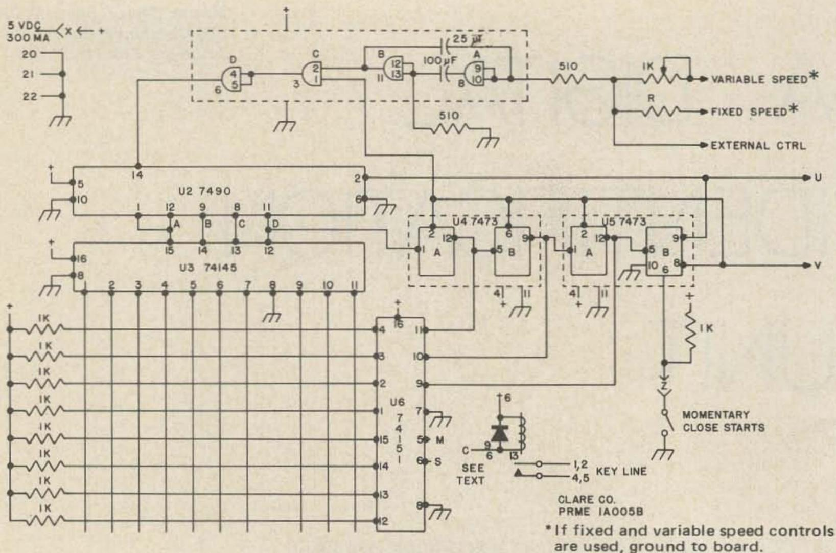
Fig. 1. K1OZS diode programmed CW identifier.
