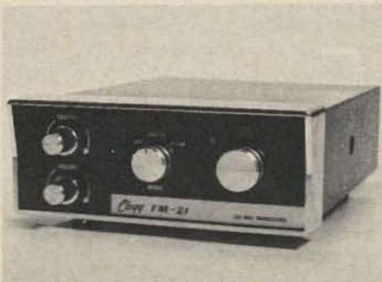
When the Clegg engineers sat down to design a 220 rig, they most certainly at one point went the route that is the industry standard - one crystal controlling the transmitter and another for the receiver. That the
