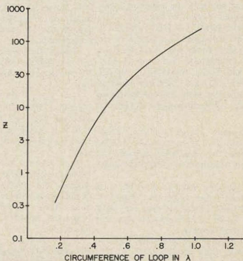
Fig. 3. Radiation resistance of a loop as a function of its size.
