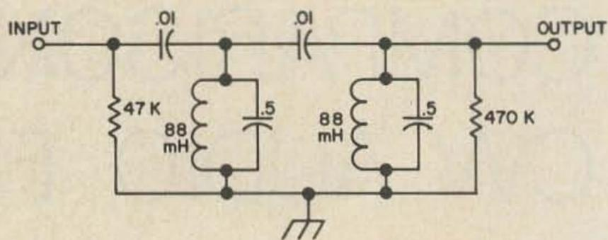
Fig. 2a. Schematic of the 88 mH toroid filter.
