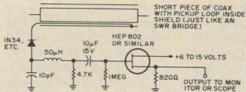
Fig. 3. Transmission line video detector.
