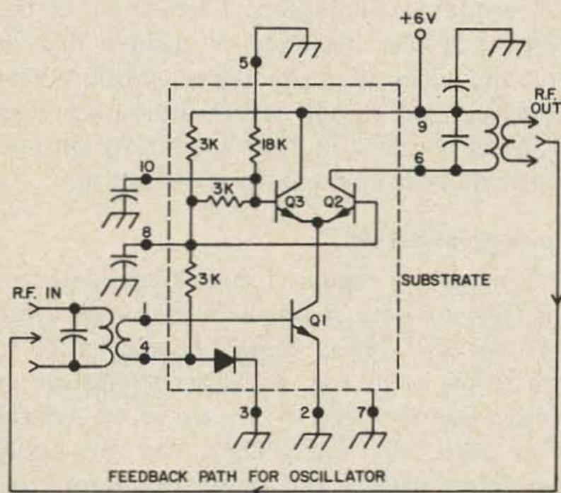
Fig. 3. Internal connections of the HEP590 and the feedback path used for oscillation.
