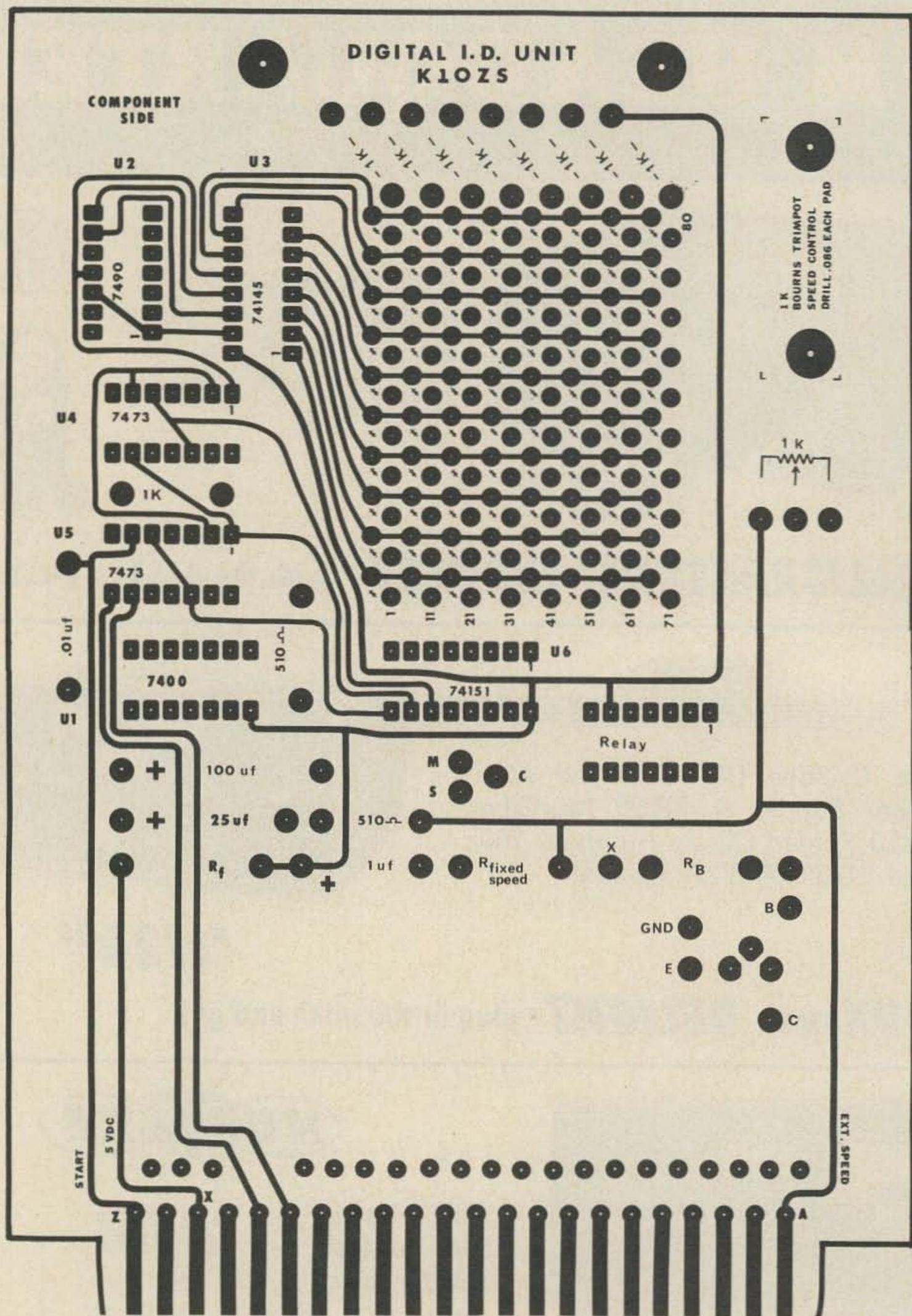
Circuit board, component side (full size).
