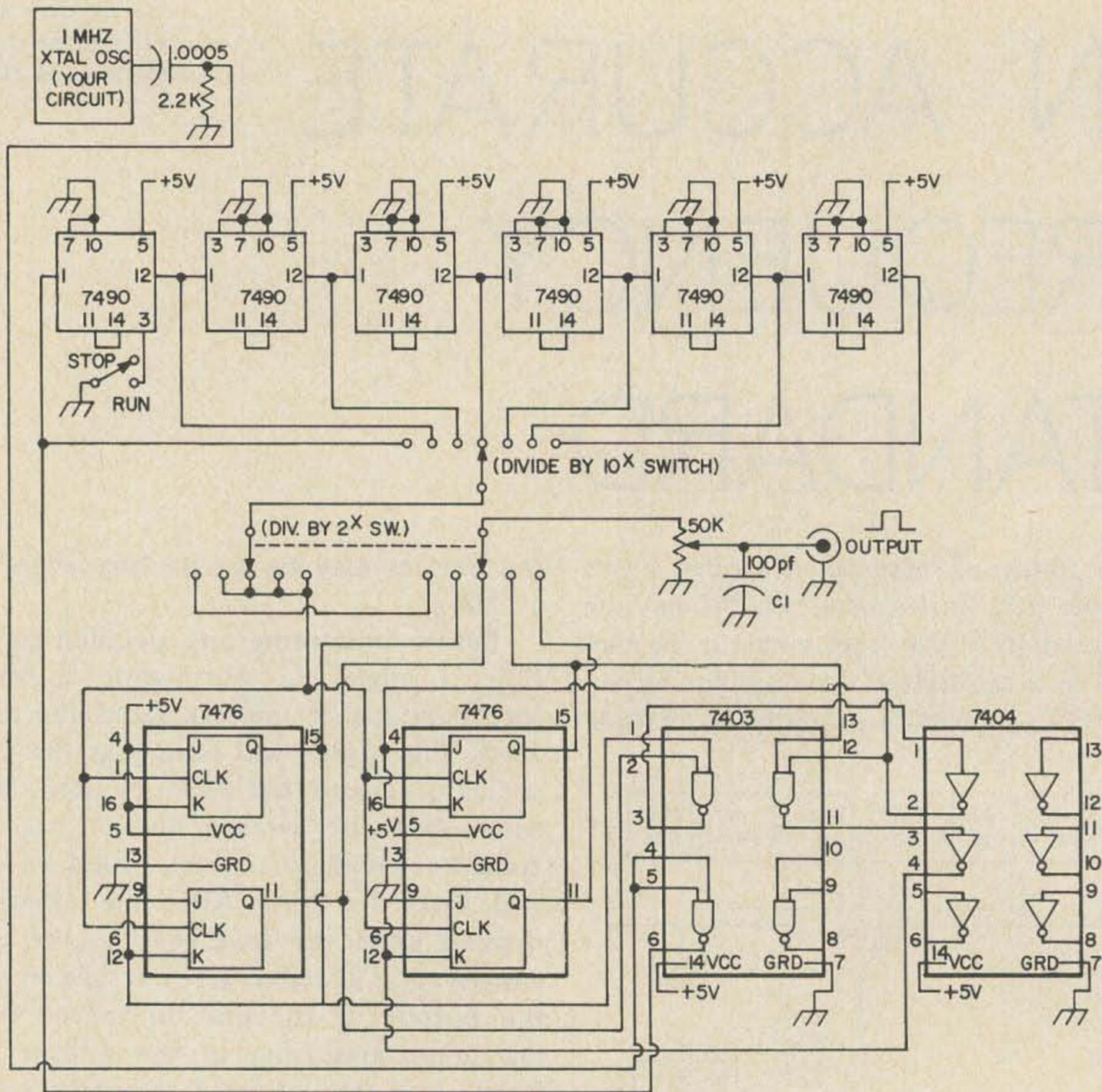
Fig. 3. Frequency standard wiring diagram.
