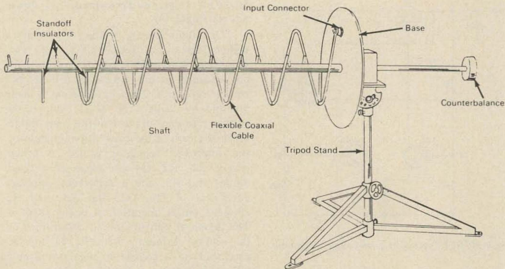
Fig. 5. Economical weatherproof helical antenna.
