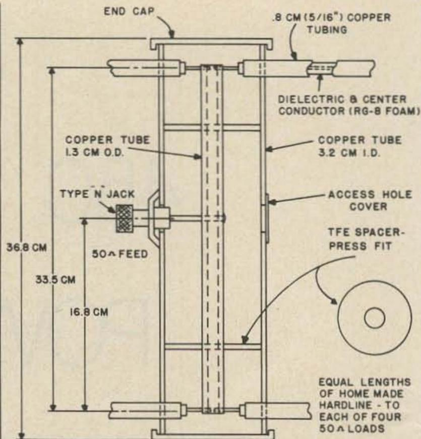
Fig. 2. Construction details of the 450 MHz power divider.
