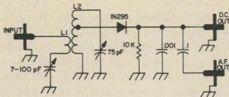
Fig. 4. Tuned diode detector (21-75 MHz) used for checking oscillator and doubler output. L1, 2T movable near L2; L2, 7T No. 3003 miniductor (16 TPI, 1.3 cm diameter), diode tap at 2T from top.
