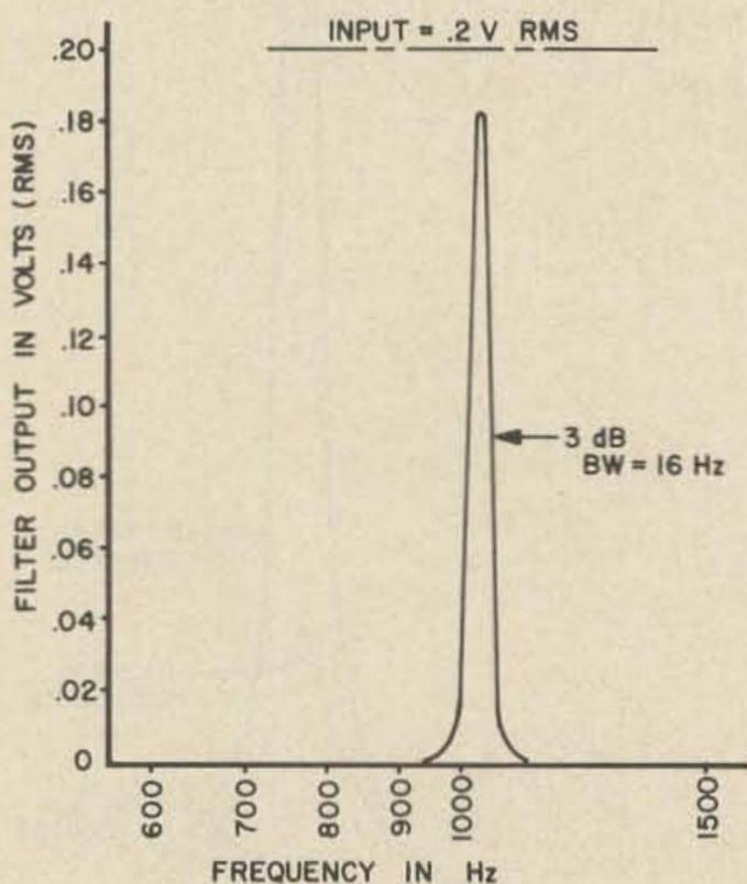
Fig. 6b. Response of filter with threshold detector.
