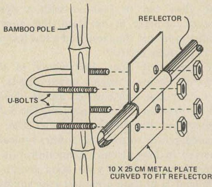
Fig. 4. Mounting of the vertical member on the reflector.
