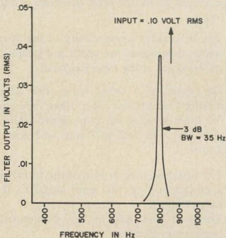
Fig. 2b. Characteristics of the passive toroid filter.
