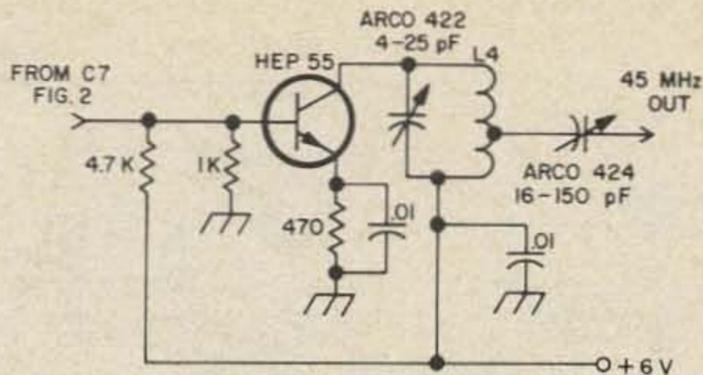
Fig. 5. Doubler for 45 MHz output. L4, 7T No. 24, 2.3 cm long, 2 cm I.D.
