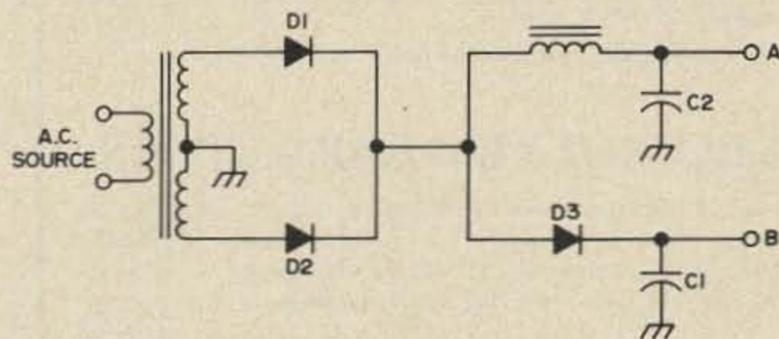
Fig. 1. Dual-voltage power supply with increased efficiency.
