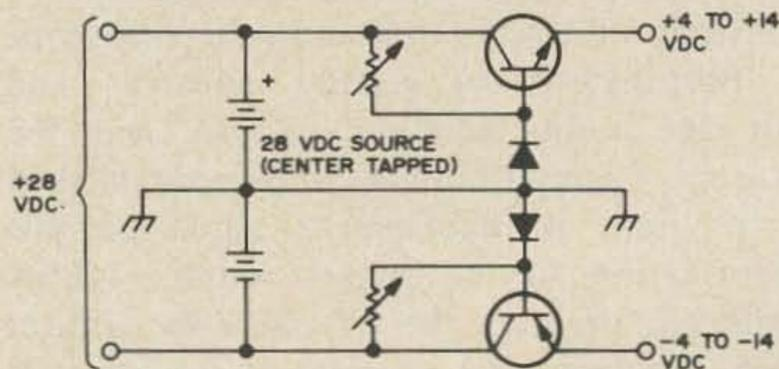
Fig. 2. Dual polarity power supply.
