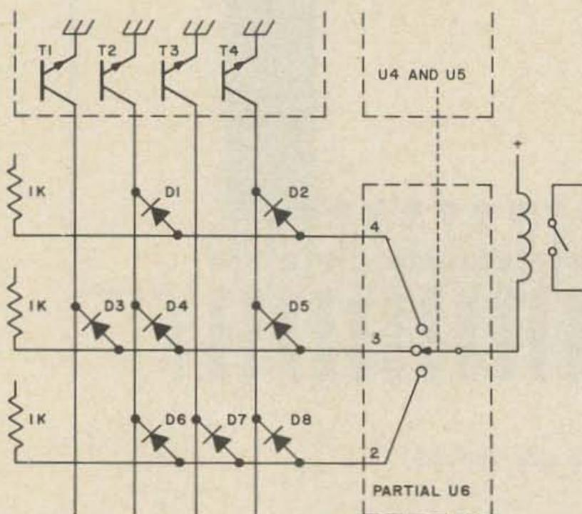
Fig. 4. Simplified version of the matrix. It is read from left to right, a horizontal row at a time, and is programmed to send dit dah dit dah. D1 is the first dit, D2, 3, 4 is the first dah, D5 is the second dit, etc. The blank areas between the bits are spaces.
