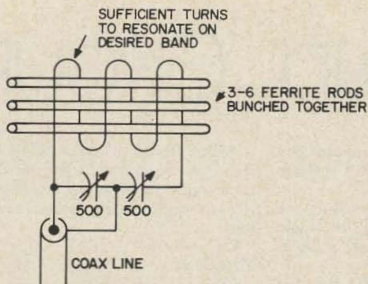
Fig. 2. Ferrite loop antenna for single band operation.
