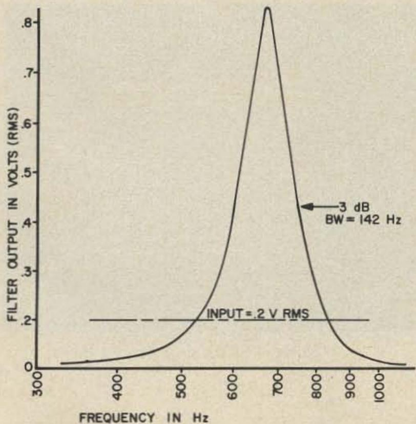
Fig. 3. Characteristics of the 4 section, Twin-T active filter (Ref. 2).
