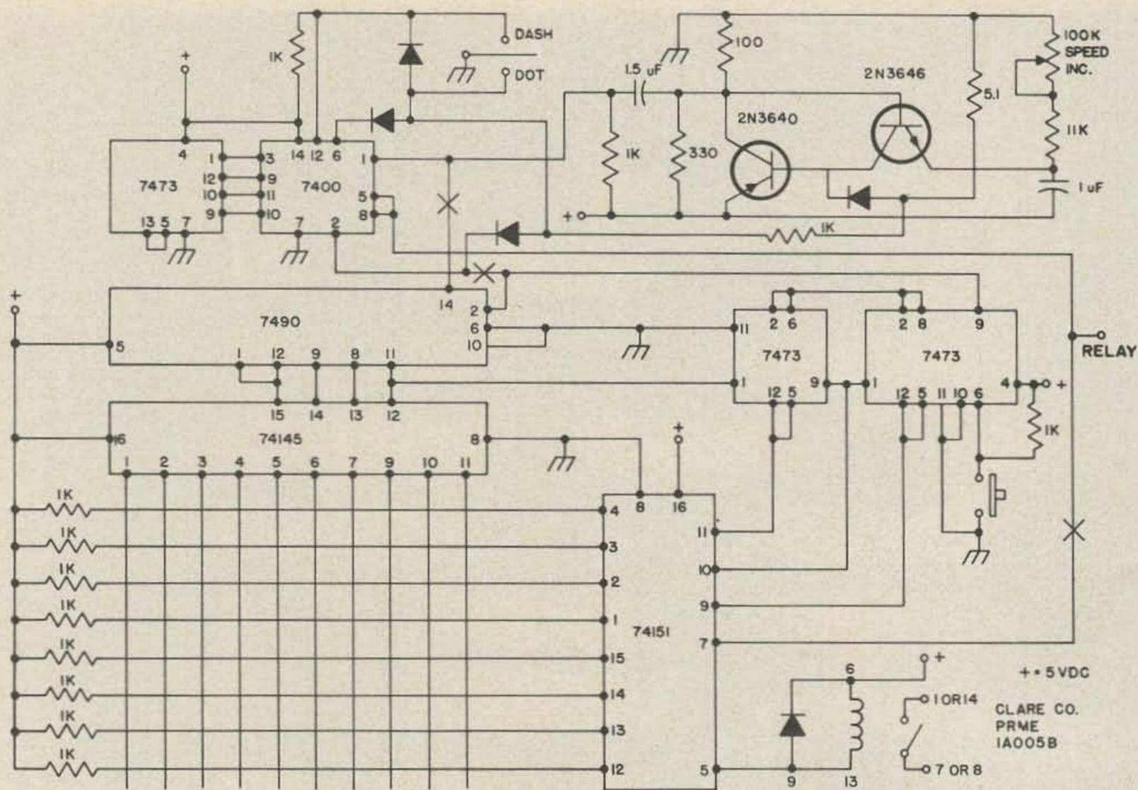
Fig. 6. One chip and two transistors add an electronic keyer to the ID unit at the three points marked with an "X."
