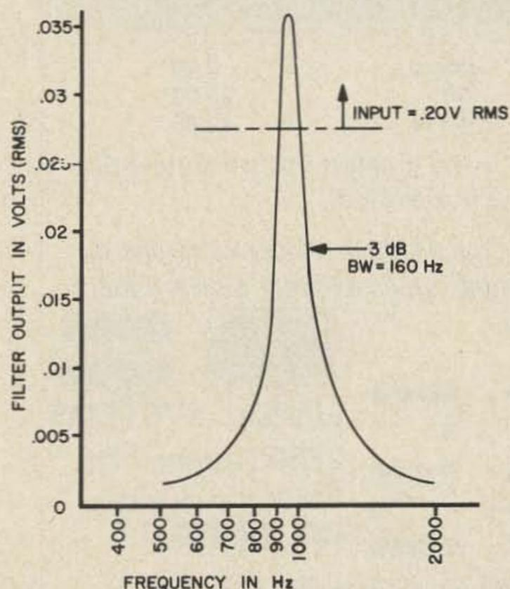
Fig. 1. Filter characteristics of the passive surplus range filter.
