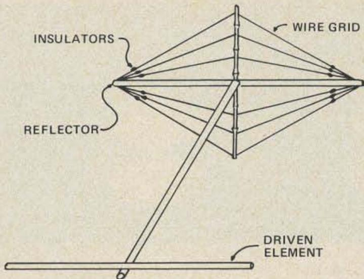
Fig. 5. Possible alternate configuration for lower frequency bands.
