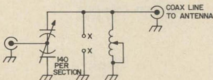
Fig. 6. Simple transmission line tuner to couple coax line operating at a high swr into a transmitter requiring 50–70Ω load at a low swr.
