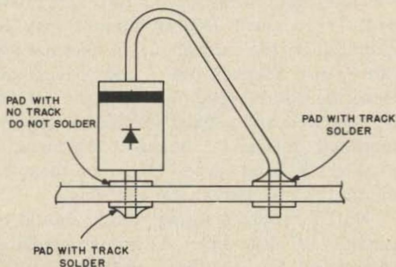
*Fig. 5. Method of mounting the matrix diodes.*
