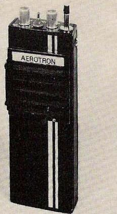
of 146 to 174 MHz. Test jacks make possible all important measurements: RF power output, deviation, frequency, receiver sensitivity, audio output and distortion... without the need to open the case. The "600" series features "crystal lattice filtering." The transmitter section is available in power output levels of 100 mW, 1.8W and 50W. Options include continuous tone squelch and up to 6 channels capability. AEROTRON, INC., P.O. Box 6527, Raleigh NC 17608.
