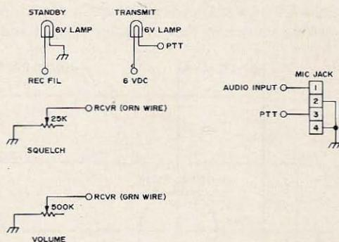
Fig. 5. Front panel schematic.
