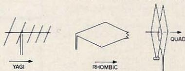
Fig. 2. Directional antennas must be pointed toward the station you're communicating with.
