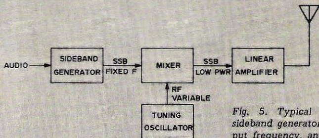
Fig. 5. Typical SSB transmitter consists of sideband generator, provisions for changing output frequency, and linear amplifiers. See Figs. 6 and 7 for details of sideband generators.
