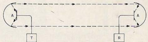
Fig. 1. The parabolic antenna concentrates virtually all the radiation into fairly tight beam.
