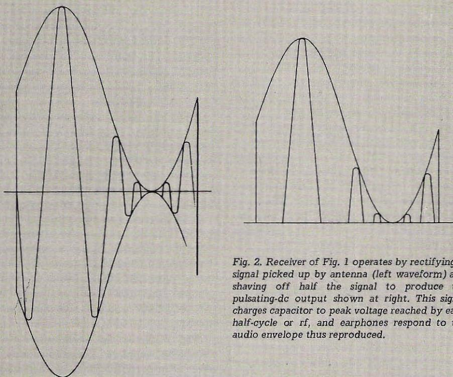
Fig. 2. Receiver of Fig. 1 operates by rectifying rf signal picked up by antenna (left waveform) and shaving off half the signal to produce the pulsating-dc output shown at right. This signal charges capacitor to peak voltage reached by each half-cycle or rf, and earphones respond to the audio envelope thus reproduced.
