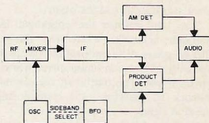
Fig. 8. Selectable sideband receiver shows great similarity to ordinary receiver (Fig. 3), but with added extras to facilitate SSB reception. Actually, any receiver capable of receiving CW can tune in SSB, but extra features shown here are needed for extended use.
