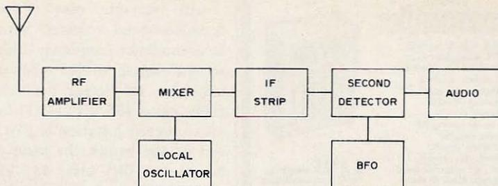
Fig. 3. Basic stages of a conventional superheterodyne receiver are shown here and described in text. Rf amplifier and bfo are not normally included in non-communications superhets for entertainment use, but are considered essential in quality communications receivers.
