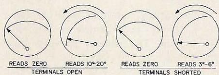
Fig. 4. A simple test can tell you a lot about a questionable meter.
