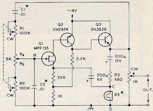
Fig. 4. Variable frequency oscillator. All resistors 10% 1/4W. \*See text for tolerance.
