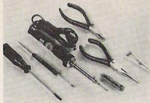
The tool kit consists of long-nose and diagonal cutting pliers, screwdriver, soldering iron, soldering aid tool, heatsink tool, and a coil of rosin-core solder — the most-needed items for the hobbyists' tool chest.
