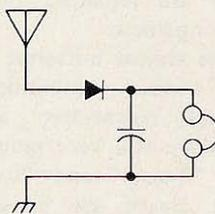
Fig. 1. Simplest radio receiver consists only of antenna, ground, diode, capacitor, and earphone connected as shown.
