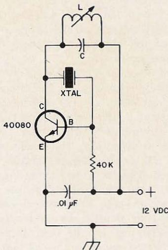
Fig. 1. Schematic diagram of simple oscillator.
