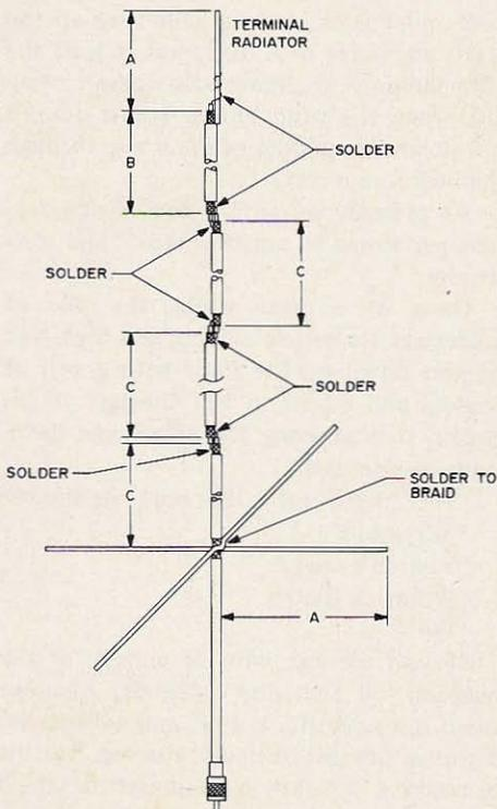
Fig. 1. The collinear gain antenna is made up of coaxial sections connected in a phase-reversal configuration. The bottom section (from the radials to the first joint) and the upper section (which joins the antenna to the shorted radiator) are half the size of all other sections.
