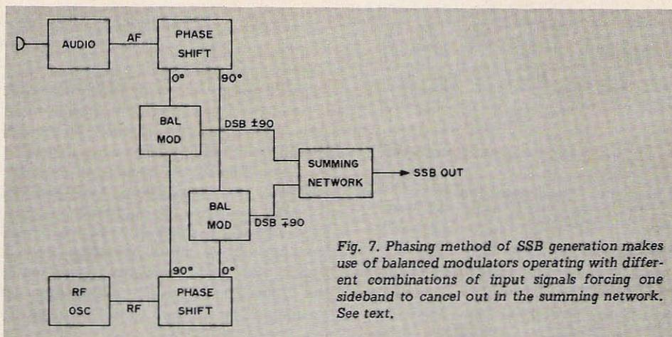
Fig. 7. Phasing method of SSB generation makes use of balanced modulators operating with different combinations of input signals forcing one sideband to cancel out in the summing network. See text.
