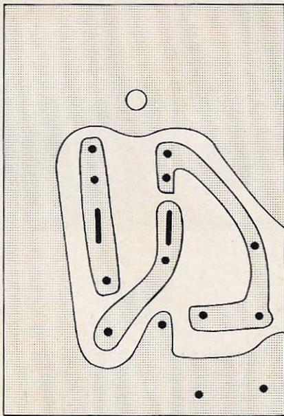
Fig. 2. 42% printed circuit layout; refer to the schematic and picture for parts placement.
