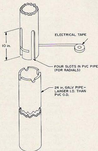
Fig. 5. Long slots in the PVC pipe will hold the radials in place with the antenna inserted. Wrap the bottom well with electrical tape after the antenna is installed in the fiber tube. Notch four matching places on a 2 ft length of galvanized pipe to seat, and try for a snug fit.
