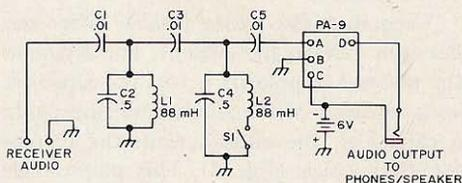
Fig. 6. Schematic of CW Audio Filter.
