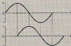
Fig. 3. Current lags voltage by 90° in an inductor.
