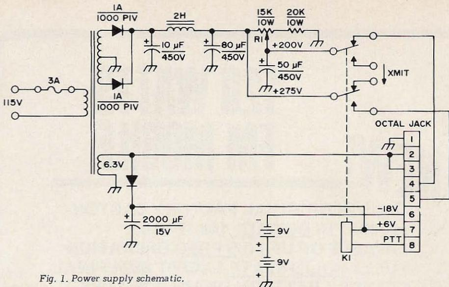
Fig. 1. Power supply schematic.
