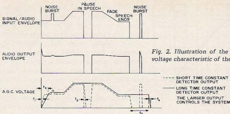
Fig. 2. Illustration of the input/output and agc voltage characteristic of the processor.
