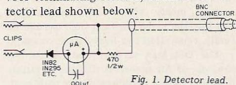
Fig. 1. Detector lead.
