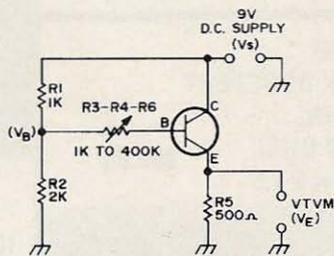
Fig. 1. Simplified Beta Test Circuit
