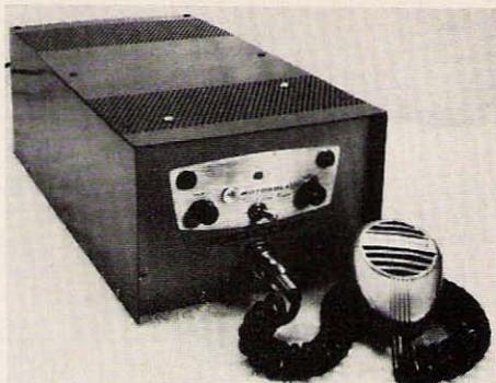
Simple U-shaped cabinet is made of scrap aluminum. The speaker is mounted behind the perforated part of the cabinet at the top front of the cabinet. Choose your own color combinations, and refinish mike to match unit.
