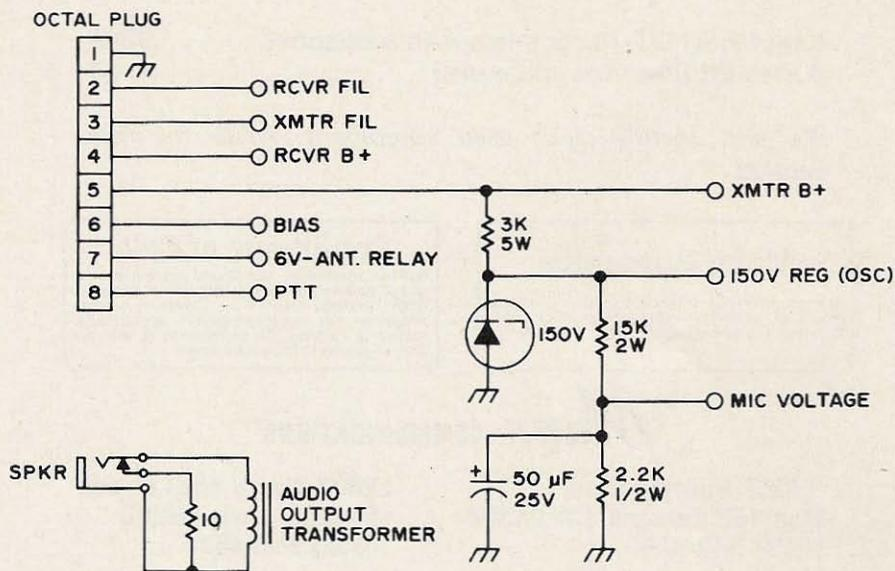
Fig. 2. Conversion chassis schematic
