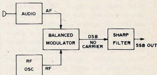
Fig. 6. Filter-method sideband generator converts audio and fixed-frequency rf into double-sideband suppressed carrier signal using balanced modulator, then filters away one sideband to produce SSB. Filter may use crystals or mechanical technique, and may operate at frequencies from 17 kHz up to 9 MHz.
