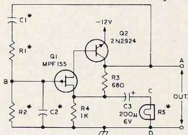
Fig. 2. Fixed frequency oscillator. All resistors 10%  $\frac{1}{4}$  W. \*See text for values and tolerance.
