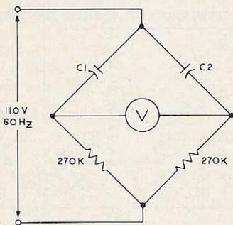
Fig. 3. Capacitor comparison bridge.
