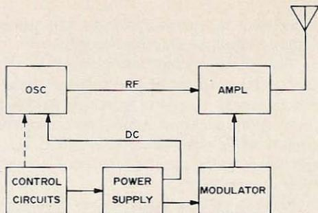
Fig. 1. Every radio transmitter contains these five basic functions, as explained in text. Even a CW transmitter has a modulator.
