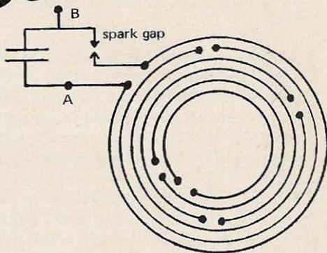
Fig. 1. Tubing may have balls or disks on their ends or strips may overlap for slight fixed condenser effect. Connect the high voltage either to A and B or to A and C. Practically there is no difference.
