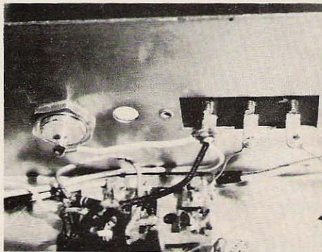
Inside of chassis showing connection of coax receptacle. Third wire on antenna terminal comes from calibrator.
