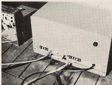
Rear of HQ100 ready for action. Notice 90° elbow on coax. Speaker plugs into phone jack — no change of impedance.
