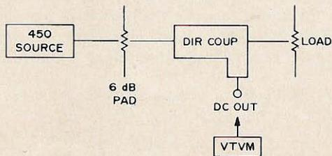
Fig. 7. Reversing the coupler should make an order of magnitude change in the voltage.
