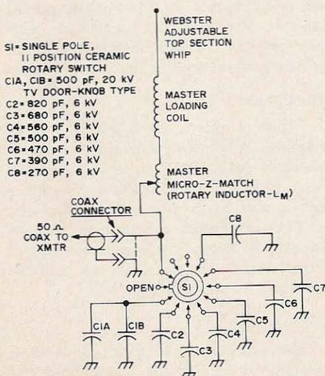
Fig. 9. Schematic of antenna circuit.
