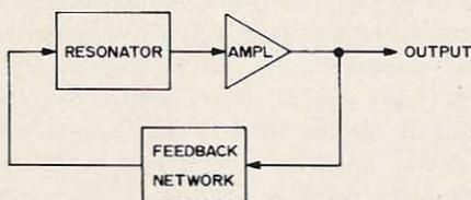
Fig. 3. Addition of resonator to feedback arrangement of Fig. 2, with proper phase of feedback and feedback fraction large enough to eliminate any need for external input, produces a tuned oscillator. All rf oscillators in common use share these three components, and the differences between one type of oscillator and another all lie in the manner in which one or more of the three basic functions is achieved.
