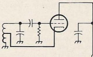
Fig. 7. The Hartley oscillator is always identified by a cathode tap on the coil.
