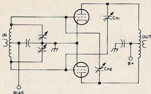
Fig. 10. Neutralization techniques for push-pull amplifiers differ somewhat from that shown in Fig. 9. Here two neutralizing capacitors are used; they connect from plate of one tube to grid of other and vice versa. Since two tubes always operate out of phase with each other, feedback still works out to be negative. The two neutralizing capacitors interact with each other, and adjustment of both must be checked whenever either is adjusted.
