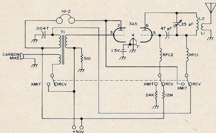
Fig. 1. Circuit diagram of what may be the world's most inexpensive 144 MHz transceiver.
