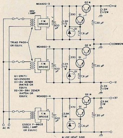
Fig. 8. Solid state power supply for 450 MHz transmitter.
