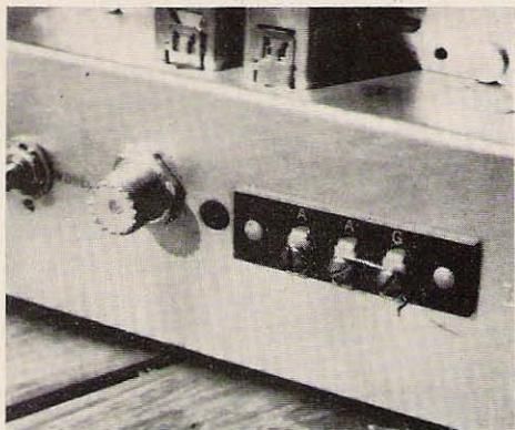
Rear of chassis showing coax connector installed.
