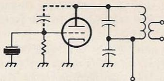
Fig. 6. Miller crystal oscillator is simply a crystal version of TPTG circuit (Fig. 5), with a crystal replacing the grid tank circuit.
