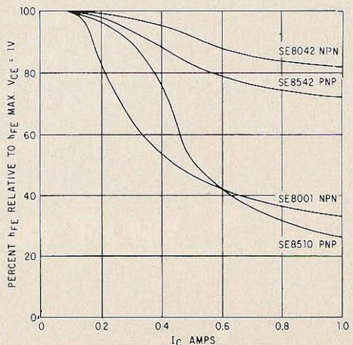
Fig. 1. Beta linearity vs collector current.
