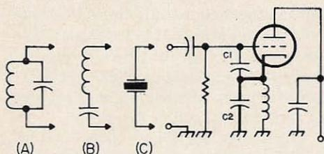
Fig. 8. Capacitance feedback circuit goes under various names, depending on the tuned-circuit arrangement.
