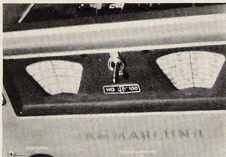
Front of receiver showing calibrator switch.
