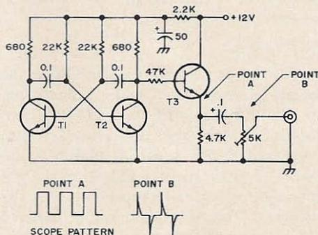
Fig. 2. Speech simulator schematic.
