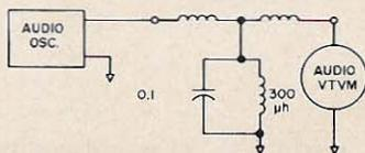
Fig. 3. Audio generator schematic.
