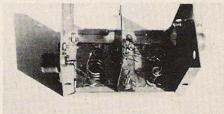
**A**n rf preamplifier is a handy thing to have when there is a desire to improve the sensitivity of older receivers or to complete the construction of modern ones. The availability of dual-gate FETs makes it possible for the average experimenter to build a good front end for his receiver. This article describes such an FET amplifier that can provide about 20 dB of voltage gain to improve the sensitivity of fair or poor receivers. This preamplifier can also improve the signal-to-noise ratio.
