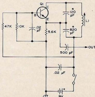
Fig. 1. 455 kHz beat frequency oscillator.
