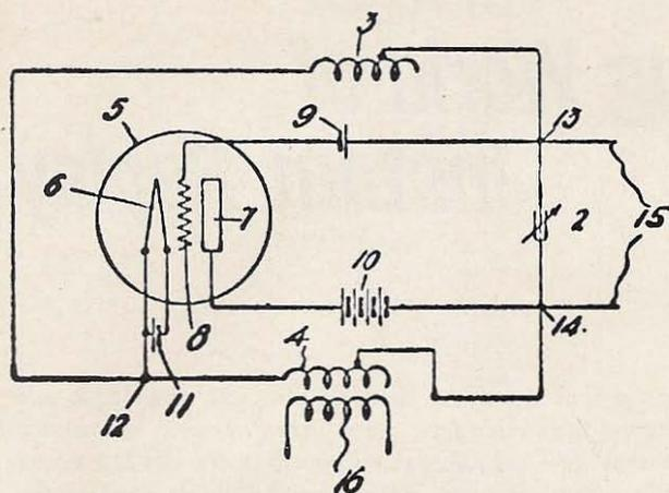
Hartley's oscillator as it appears on his patent granted Oct. 26, 1920. It took more than 3 pages of very small type to describe the operation of the oscillator. The device, granted patent 1,356,763, was called an "oscillation generator."
