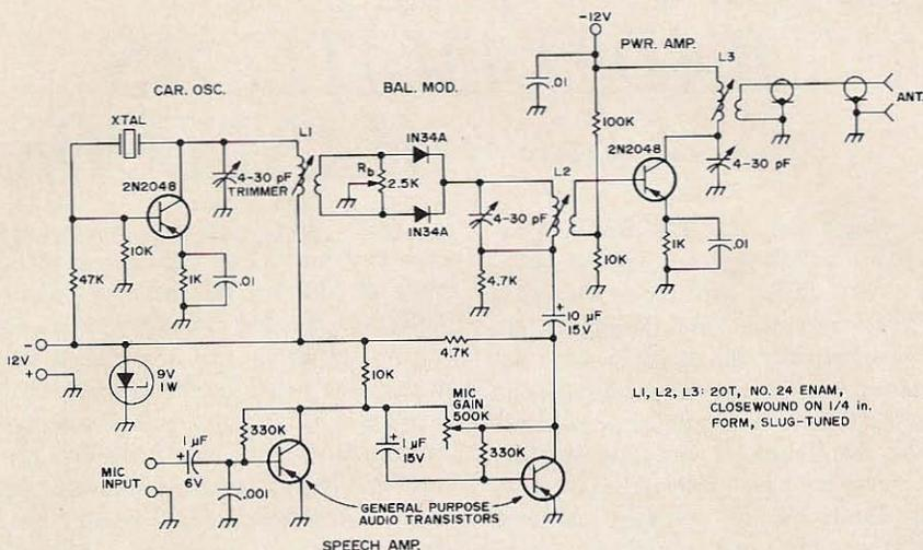
Fig. 2. Schematic diagram of DSB transmitter for 10m.
