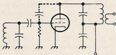
Fig. 5. Tune-plate tuned-grid oscillator feedback path runs through the grid-plate capacitance of tube.
