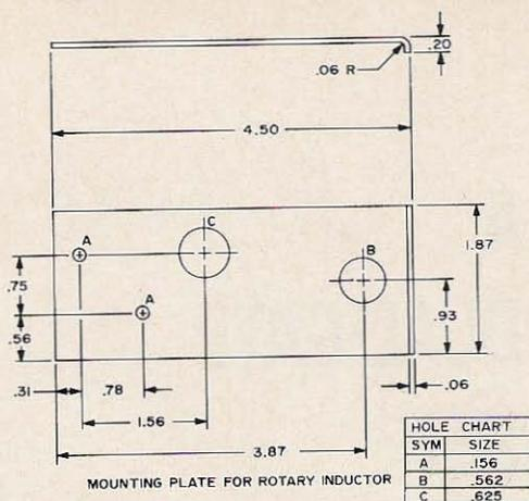
Fig. 10. Dimensions of mounting plate for rotary inductor.
