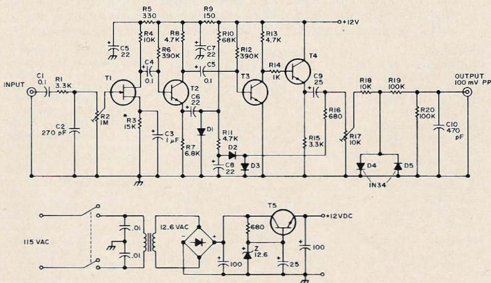
Fig. 1. Compressor schematic.
