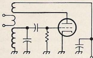
Fig. 4. Armstrong oscillator; feedback is via a  $r''$  "tickler" coil.
