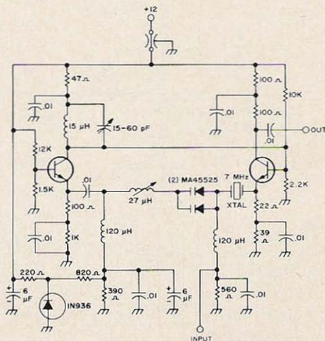
Fig. 2. Variable crystal-controlled oscillator circuit.
