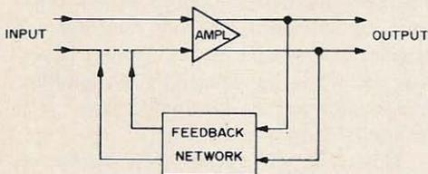
Fig. 2. When a part of the output of an amplifier is fed back to the input, effective characteristics of the amplifier are greatly changed. Normally, only a small fraction of the total output is fed back; function of feedback network is to cut total output down to desired "feedback fraction" for feeding back, and to determine phase of feedback signal with respect to that of input signal.
