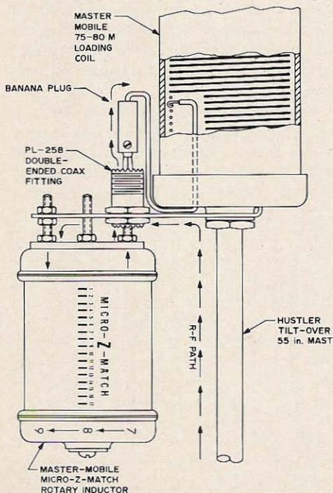
Fig. 4. Rotary coil detail.
