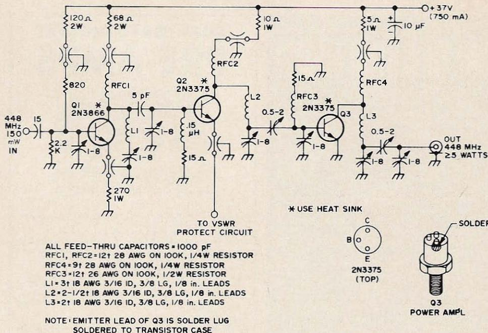
Fig. 5. Rf power amplifier stages. With a 150 mW input, a signal of at least 5W is produced.
