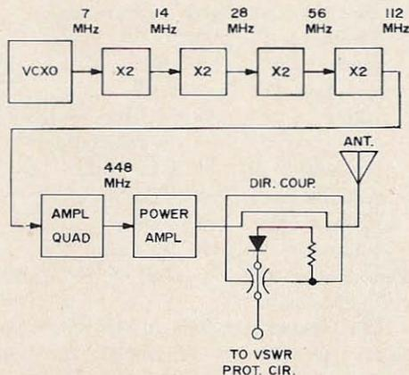
Fig. 1. Block diagram of 450 MHz transmitter.
