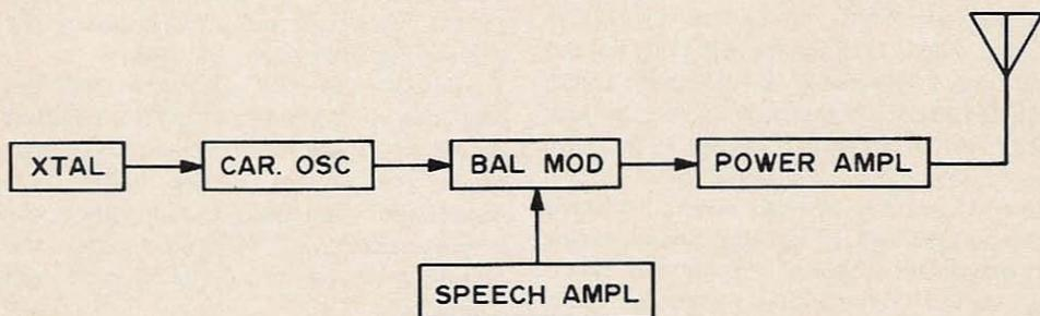
Fig. 1. This block diagram shows the simplicity of the homebrew 10m DSB transmitter. The tenth-watt unit can be used to drive a low-power linear or, for QRP fun, it can be used barefoot.
