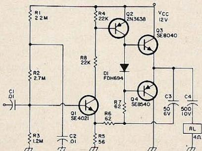
Fig. 4. Gain linearity is unimportant for distortion determination because of feedback.
