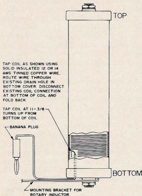
Fig. 3. Loading coil detail.
