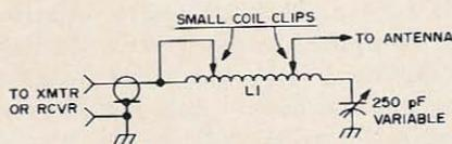
Fig. 2. Wide-range, single-wire antenna coupler for transmitter or receiver.
