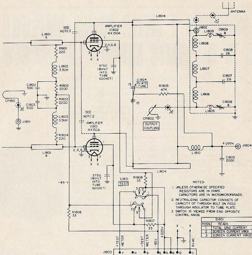
Fig. 2. Radio frequency amplifier, schematic.
